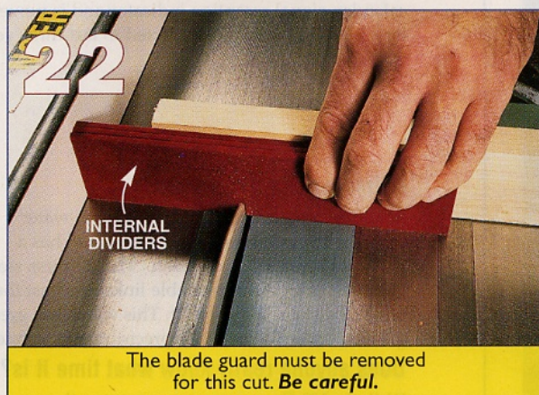
Cut the internal dividers in a gang to guarantee that the cuts line up. A sacrificial fence on the miter gauge prevents excessive velvet fraying.
