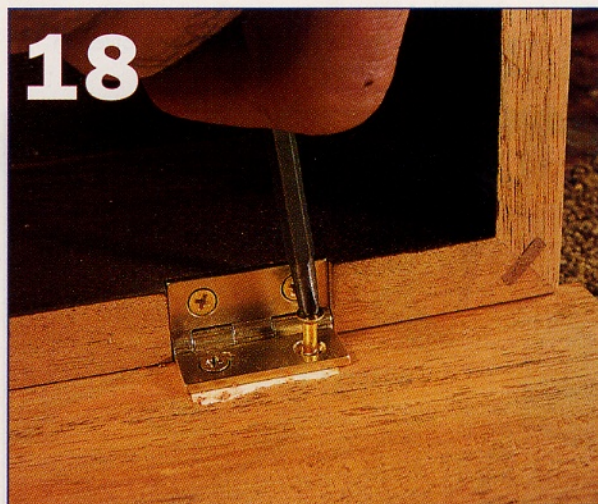
Carefully flip over the box , with the taped-on lid, and mark the screw locations. Then, predrill and screw the hinges to the lid. Protect the top of the lid with a carpet pad on the bench. Warning! Don't use the screws that come with the hinges. They're too long and will run right through the top! Replace them with #4 x 1/2-in. screws.
