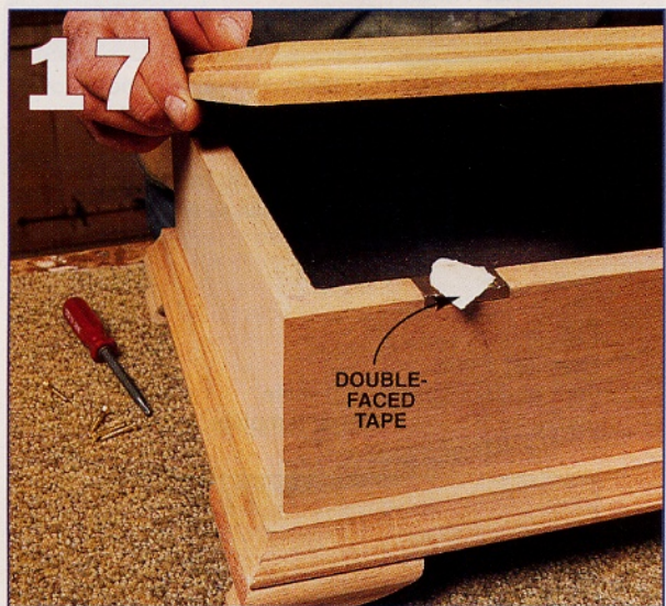
Put double-faced tape on each hinge leaf. Then position the lid flush with the back of the box and press it down on the tape.
