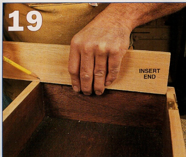
Mark and cut the insert ends 1/16-in. shorter than the interior dimension of the box, so they can slide in.
