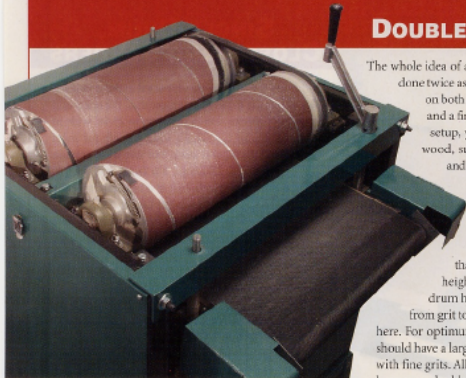
13 Double-drum sanders save sanding and set-up time by using two different grits in one pass.
