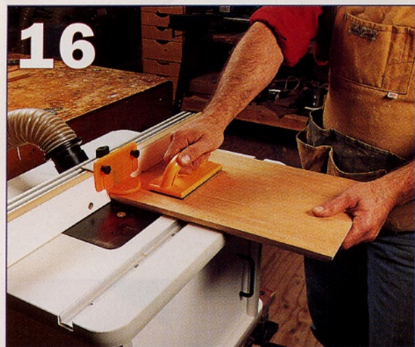
Rout the second pass in the lid using the 1/4-in. round-over bit as shown in Fig. F.
