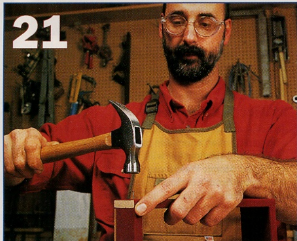
Hand-nail the insert together with 4d brads. With a brad nailer, it's too easy to blow a nail out through the narrow sides.
