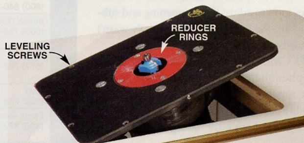
Photo 13 Mounting plates allow you to easily lift the router and mounting plate out of the table for bit changes and hand-held work. On the downside, you need to level the plate with the top, and the large cutout can weaken the top.
