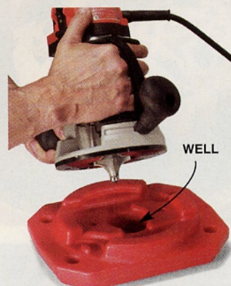
The case includes a removable base with a deep well, so you can store the router upright on your workbench.
