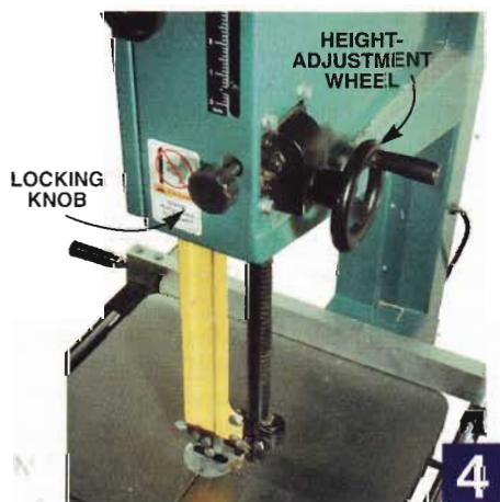
Rack-and-pinion height adjustment makes raising and lowering the guard easy.
