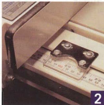
2 Direct-read cursors almost eliminate measuring on the tablesaw.
