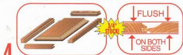
4 ASSEMBLE STILES, RAILS AND DOOR PANEL.
