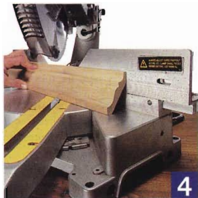
A tall fence makes it easier to cut crown molding.
