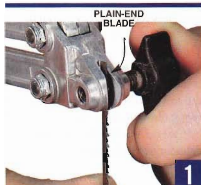
1 Tool-free blade changes make scrollsawing easy.
