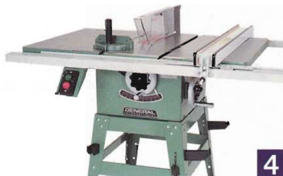
4 Solid, cast-iron tables are preferable to webbed or stamped tables. They're flat, with no holes to catch your fingers in.
