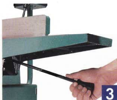
Lever adjustments are fast, but can be difficult to use for fine adjustments.
