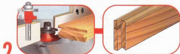
2 ROUT STILES & RAILS. SHOWN: STILE BIT FROM FREUD SET #99-260.
