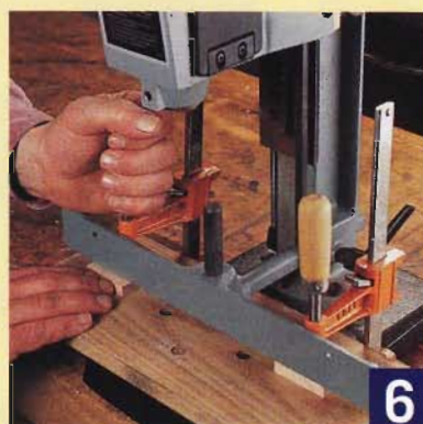
Clamp the fence to the table so it stays put.
