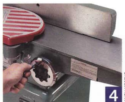
Wheel-style adjustment offers control of table height.
