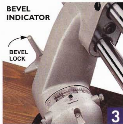
Angle and bevel indicators should be easy to read.
