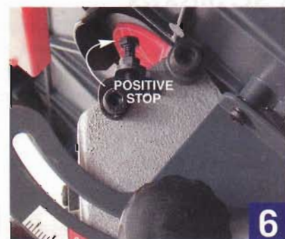
6 Tables should tilt 45 degrees in one direction and at least 15 degrees in the other.
