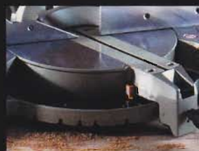
Large miter scale with precision machined positive stops in 9 positions
