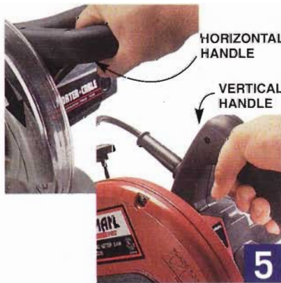
Miter saws come with horizontal or vertical handles. The choice is personal.
