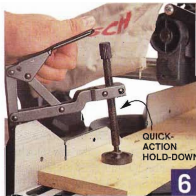
Quick-action hold-downs make it easier to clamp material to the saw.
