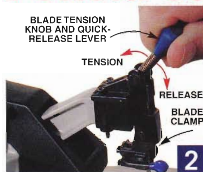
2 Quick-release blade tensioners simplify blade changes even further.
