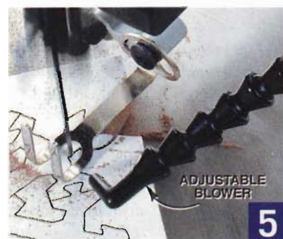
5 Adjustable dust blowers help keep your work area clear.
