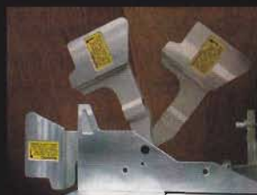
Adjustable pivoting flip fence for supporting taller stock
