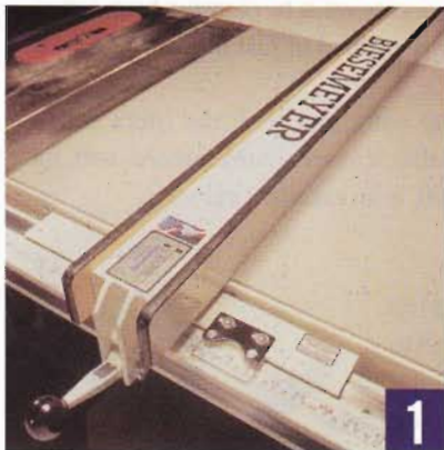
1 T-square fences lock rigidly at the front of the saw.
