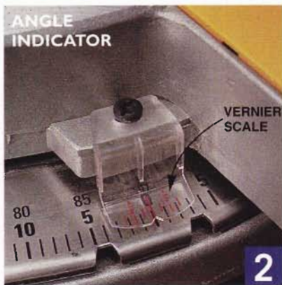
Angle and bevel indicators should be easy to read.
