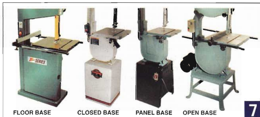
There are four basic bandsaw base styles.
