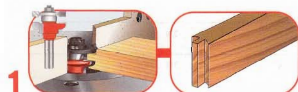
1 ROUT RAIL ENDS. SHOWN: RAIL BIT FROM FREUD SET #99-260.
