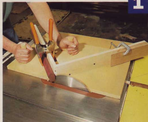
Cut the first miter by clamping the stock on the fence that faces the operator.
