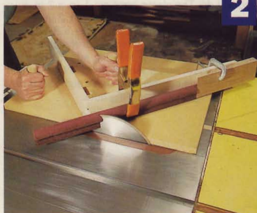
Cut the second miter on the opposite fence with the newly mitered end locked into the mitered stop block.
