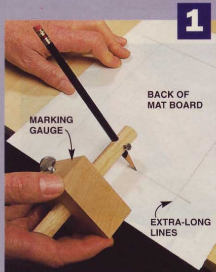
1 Lay out the mat opening with a marking gauge. You can easily make your own from a block of wood and some 5/8-in. dowel.
