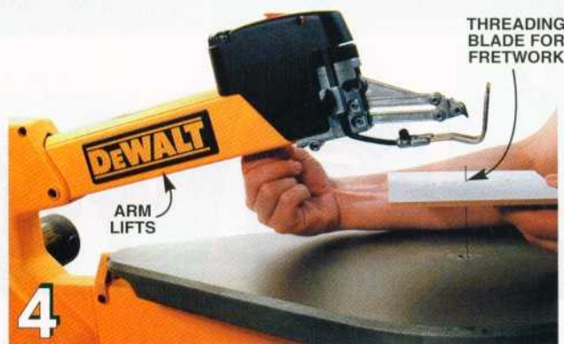
4 You just can't beat the lifting upper arm on the DeWalt for threading blades. Release the blade from the upper holder, lift the arm, thread the workpiece over the blade, lower the arm, reattach the blade and you're ready to go.
