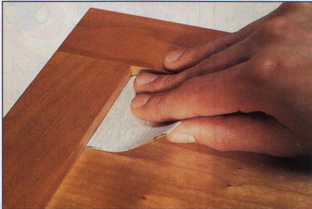
SAND INTO TIGHT CORNERS. This folded sandpaper pad lets you put sanding pressure just where you want it.
