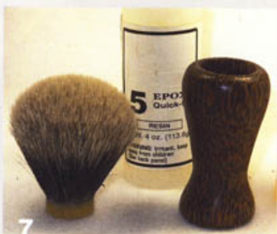
7 After a dry fit test, the handle is ready for the knot to be glued in.
