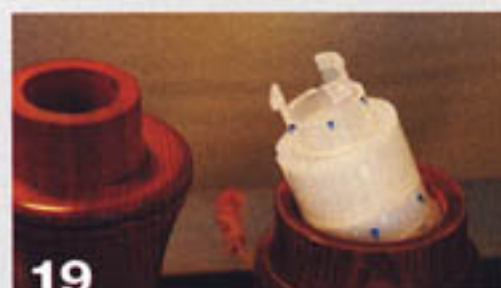
19 Apply blue marker to the ends of each little "fin" of the grinder mechanism. The blue ink will be transferred onto the inside of the hole on bottom of the bottom section and onto the inside of the hole in the bottom of the middle section.
