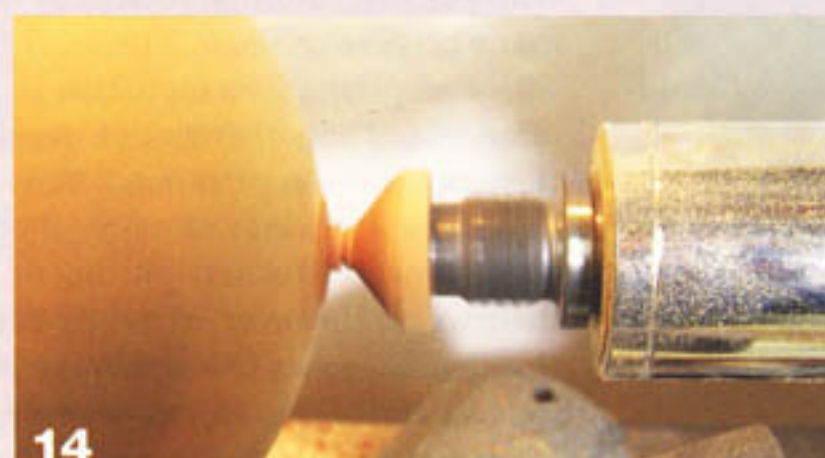
14 Cut away the tenon from the top part of the newel post and sand that area.
