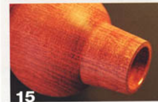
15 Shape the outside of the top. Sand and apply finish to that part before later reversing it.
