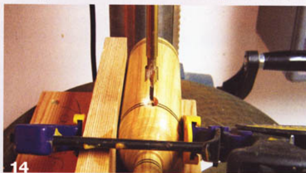
14 Drill a \frac{3}{8} " (10mm) hole at the end of each cut line.
