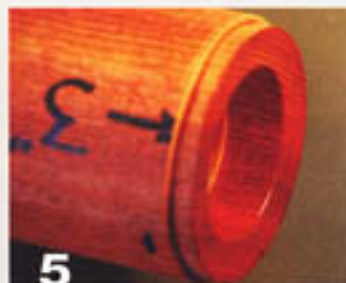
5 Sand and apply finish to the inside of the hole that is drilled on the other end of the bottom section.
