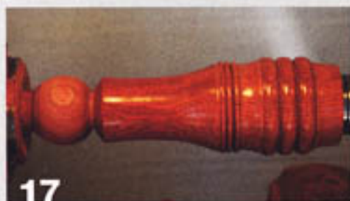
17 Turn the assembly to a pleasing shape. Then, sand and apply finish to the middle and bottom sections.
