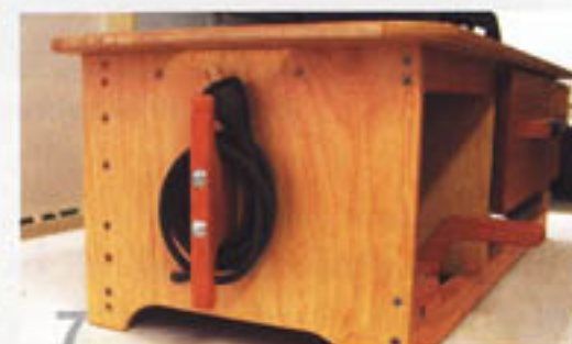
7 A power cord storage bracket is bolted to the outside.
