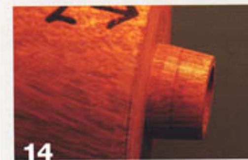
14 Taper the tenon so that it fits into the tapered hole in the middle section.
