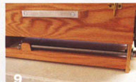
9 The axle for the wheels is stored on the other end of the cabinet underneath the drawer when not in use.
