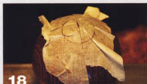
18 Using masking tape and a compass, mark a circle where the holes for the salt will be drilled.
