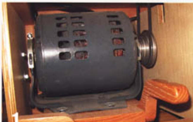
A handle allows easy lifting of the motor to change the pulley belt.
