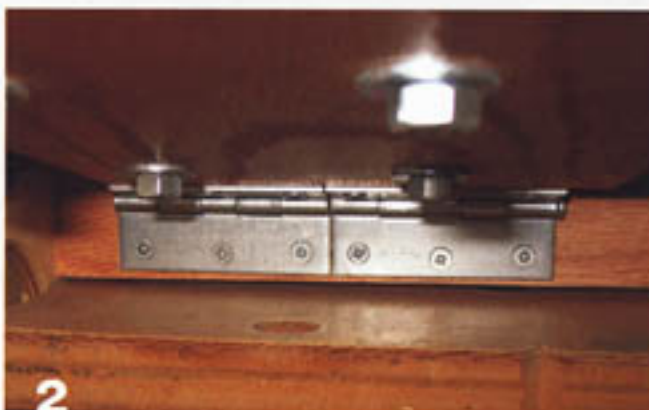
Motor is mounted on a board that is secured to the cabinet with two hinges.
