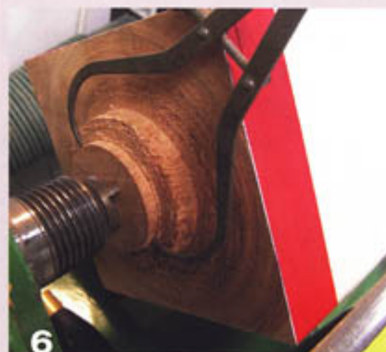
6 Use calipers to size the tenon. Make sure the lathe is off when measuring next to a square shoulder such as this.
