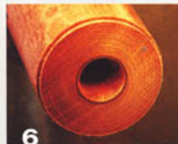
6 After drilling a 1"-diameter (25mm) hole, mark a line about 1/16" (1.5mm) outside the hole and enlarge the hole so that it has a slight taper.
