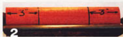
2 Measure and mark the three sections of the peppermill/saltshaker: top, middle, and bottom.
