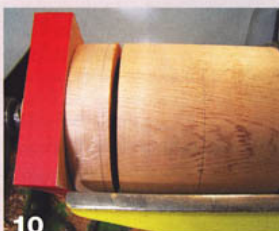
10 Layout lines are marked and the first key dimension is created using a parting tool.
