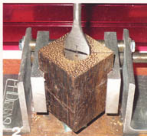
Drill the first hole in the handle using either a spade or Forstner bit.
