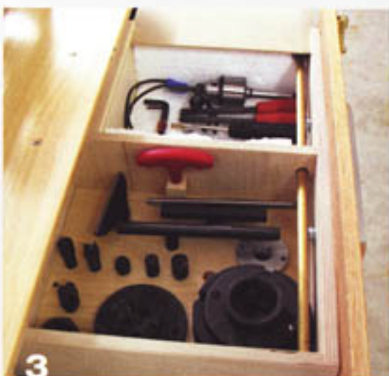
A two-section tool drawer with full-extension drawer slides is installed.
