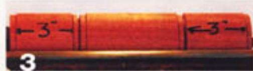
3 Begin parting the three sections to create tenons for mounting in a chuck.
