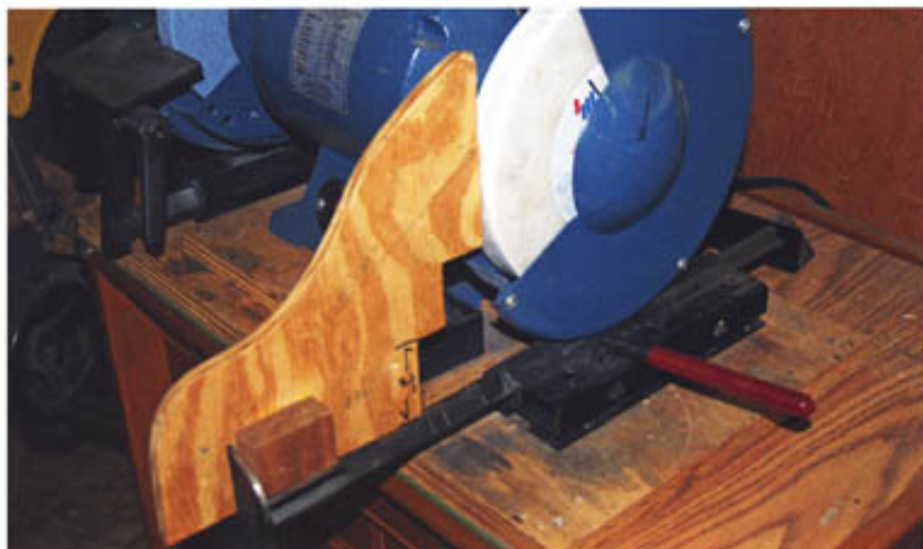
Using a simple shopmade template to set up your sharpening jig for repeatable distances saves time and tool wear.
