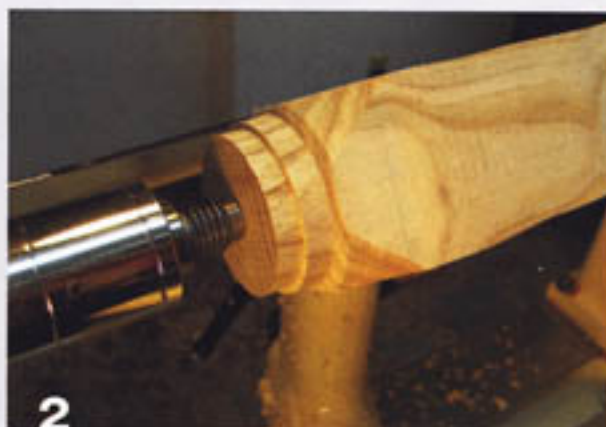
2 Form a tenon at the tailstock end.
