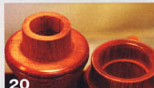
20 Carve small V-grooves at all the marked locations. The grooves will lock the fins in place when the mechanism is inserted.
