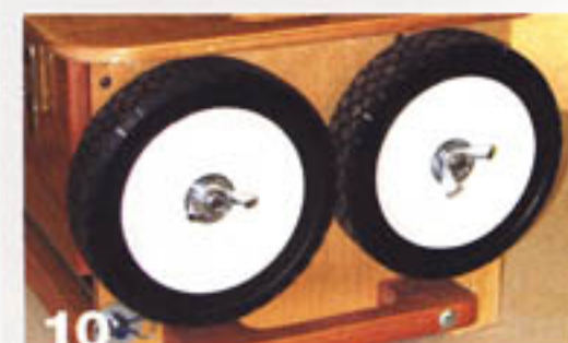
10 The wheels can be stored out of harm's way when not in use. Two carriage bolts with wing nuts and washers hold them in place.
