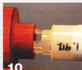
10 A small groove will be turned inside the middle section's tenon to accept the "ears" of the grinder mechanism.
