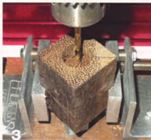
Drill the pilot hole for the tap.
