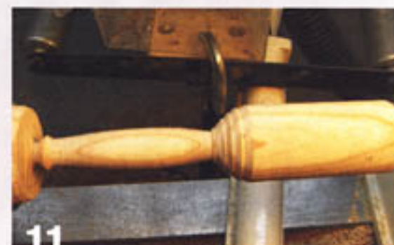
11 Form the handle and sand the taper.
