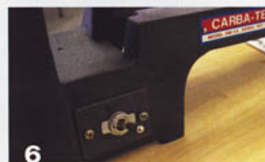
6 A toggle switch is mounted to the front of the lathe to provide a power switch.
