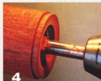
4 With the bottom section mounted in a chuck, clean up any torn grain, then drill the first hole.
