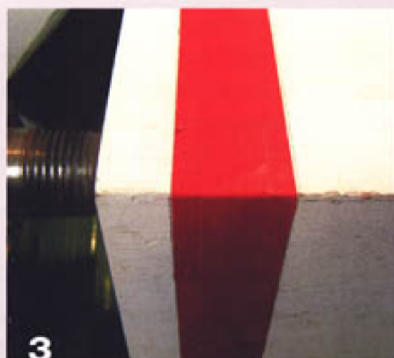
3 Affix red painters' tape to the square shoulders to help reduce tearout of the wood and to provide a warning sign.
