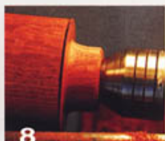
8 Use the rotating cone of the live center to steady the wood while turning the tenon.
