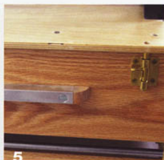
A brass barrel bolt is mounted to the front of the drawer to keep it secure while moving the stand.
