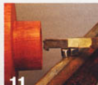
11 The author's shopmade tool that is used to cut the groove for the ears of the grinder mechanism. A small-profile round-nose scraper can also be used.
