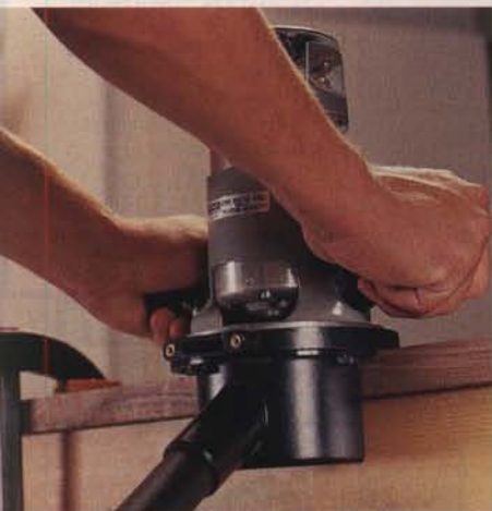
For edge routing, a plastic shroud fastens to the bottom of the Porter-Cable dust collection subbase.
