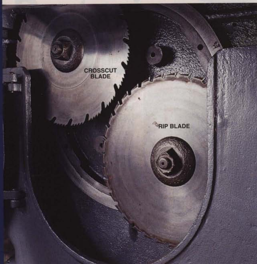
This mid-1920s American Machinery tablesaw has two arbors, one with a rip blade, one with a crosscut. You turn a crank to switch between them.
