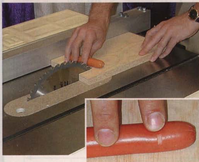
The SawStop is demonstrated here by allowing a hot dog to contact the blade. The blade stops almost instantly so the hot dog is barely nicked.
