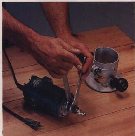
Bit changing is particularly easy with the motor removed from the base.
