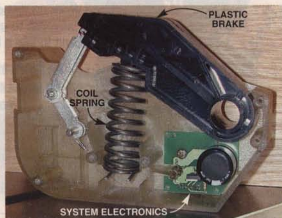
The SawStop cartridge consists of a heavy spring, electrical circuits and a plastic brake pad. If your finger contacts the blade, the electronic circuit releases the spring, stopping the blade.
