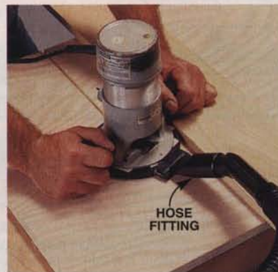
For surface and plunge routing, the hollow subbase connects to your vacuum with an angled fitting.
