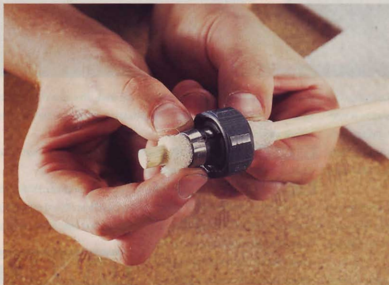
CLEAN rusty router collets with a dowel and synthetic steel wool.
