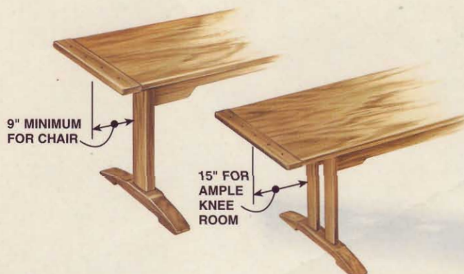
FIG. F A trestle table limits knee clearance at the ends. A large overhang may not look as well proportioned, but it affords plenty of legroom.
