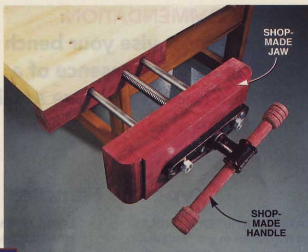
2 A WOOD-JAW VISE requires assembly. Make your own jaws and turn a handle of any length (or buy one). The front of the bench doubles as the upper half of the rear jaw.
