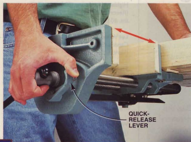
3 SQUEEZE THE LEVER on this quick-release mechanism to slide the front jaw in or out. The spring-loaded lever is connected to a bar that releases the nut from the vise's screw. We prefer this type of quick release.
