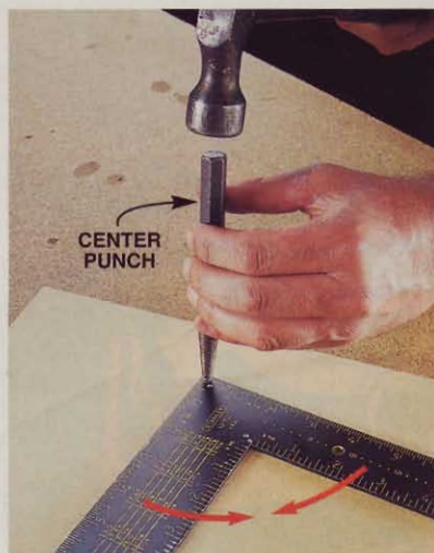
PEENING THE OUTSIDE CORNER "closes" the square.
