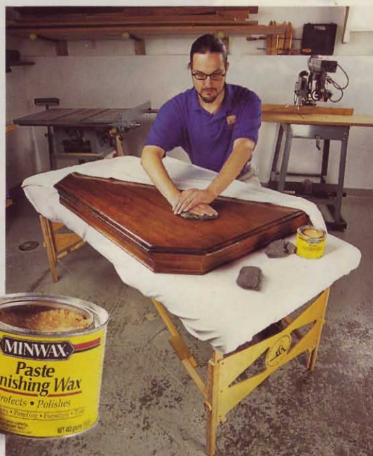
GIVE YOUR WORK a final rubdown with wax and extra-fine steel wool.
