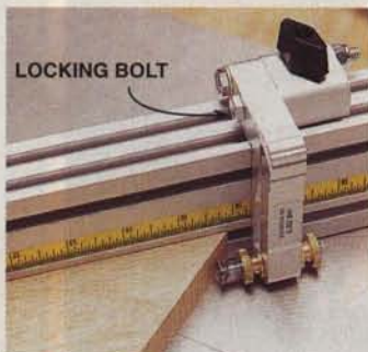
5 WOODHAVEN'S FLIP STOP can be locked down so it doesn't climb up miters.
