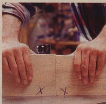
5 WOODHAVEN'S FLIP STOP can be locked down so it doesn't climb up miters.
