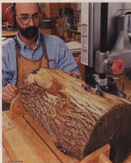
6 DRAW A LINE down the middle of the log using a pencil and straightedge, or snap a chalk line. With the log secured into the sled, saw the log in half.
