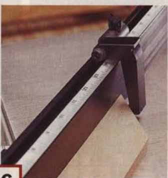
6 ALL OTHER FLIP STOPS will climb on miters, making uniform length impossible, unless the stop is clamped.
