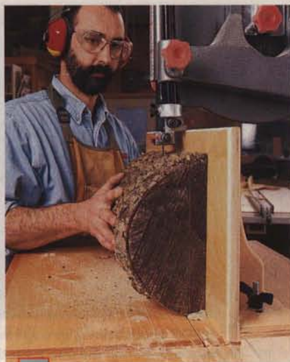
7 SET UP A FENCE to resaw the boards. Run one face of your halved log against the fence, and keep going until you've cut the entire log.
