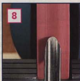
Fig. B THE DETAILING GOUGE is commonly formed into a fingernail shape (as viewed from above) and with a 30- to 35-degree bevel angle.
