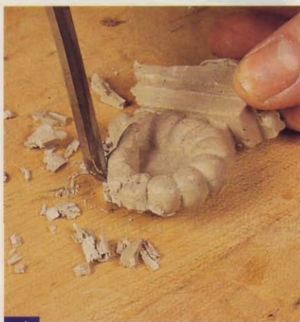
4 CLEAN UP THE CASTING and cut to fit with an X-Acto knife or chisel.
