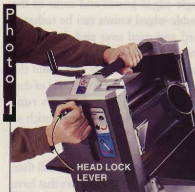
A HEAD LOCK minimizes the amount of snipe but won't eliminate it. The Delta 22-560 head lock shown here is easy to use.
