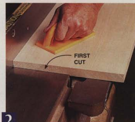
2 REMOVE THE SHIM and make the first cut.
