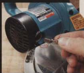
Externally accessible brushes allow job-site serviceability
