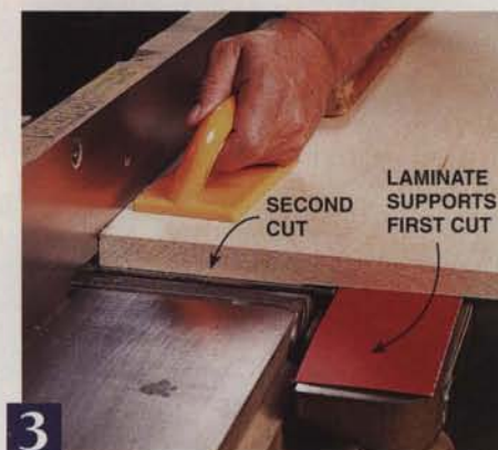
3 REPLACE THE SHIM, turn the board end for end and make the second cut.
