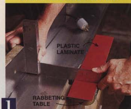
1 SET THE DEPTH of cut equal to the thickness of the shim.
