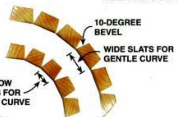
FIG. D A TIGHT TURN requires small slats. The sharpest turn in a roll-top desk is the one you can't see, right behind the pigeon holes. Beveled slats work as well as half-round slats in an S-curve.
