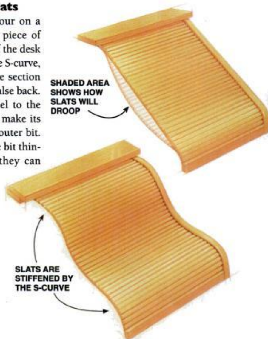
FIG. B THE S-CURVE DESIGN has more to it than good looks. The slats won't sag if they're held in a bent shape.
