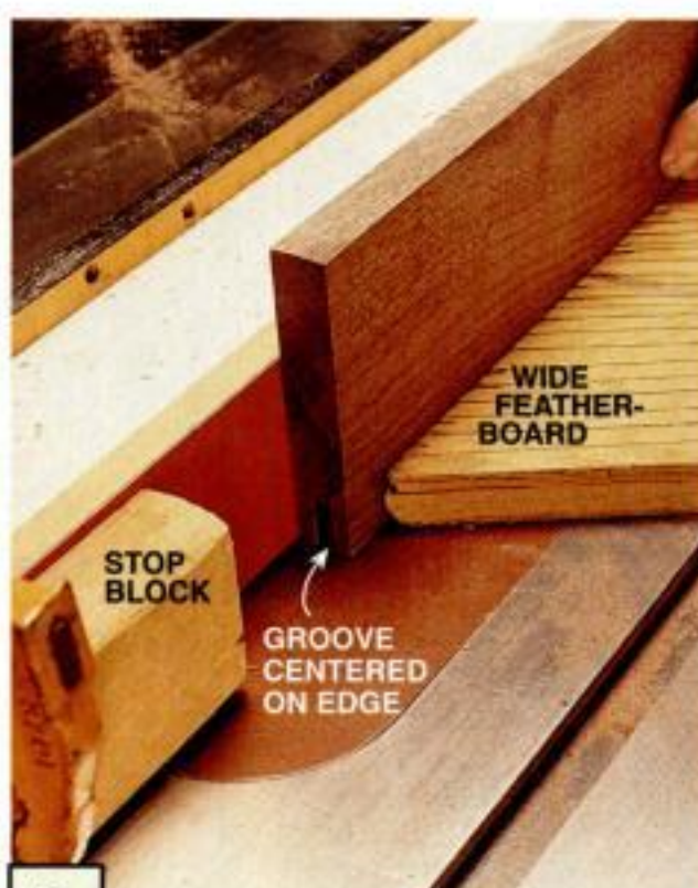
2 USE STOP BLOCKS to limit the length of the deeper grooves at each end of the stiles where the tongues of the rails will fit. Use a dado blade to cut panel grooves in the stiles and rails. Raise the blade and make the deeper grooves for the rails.
