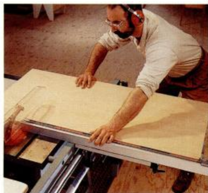
FOR EVEN GREATER CAPACITY, move the fence to the front of the table.
