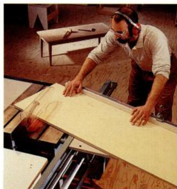
DELTA'S SLIDING TABLE attachment makes it easy to crosscut wide material, especially at an angle.
