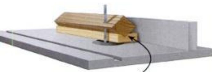
V-GROOVE IN SLED HOLDS STOCK AT 45 DEGREES
