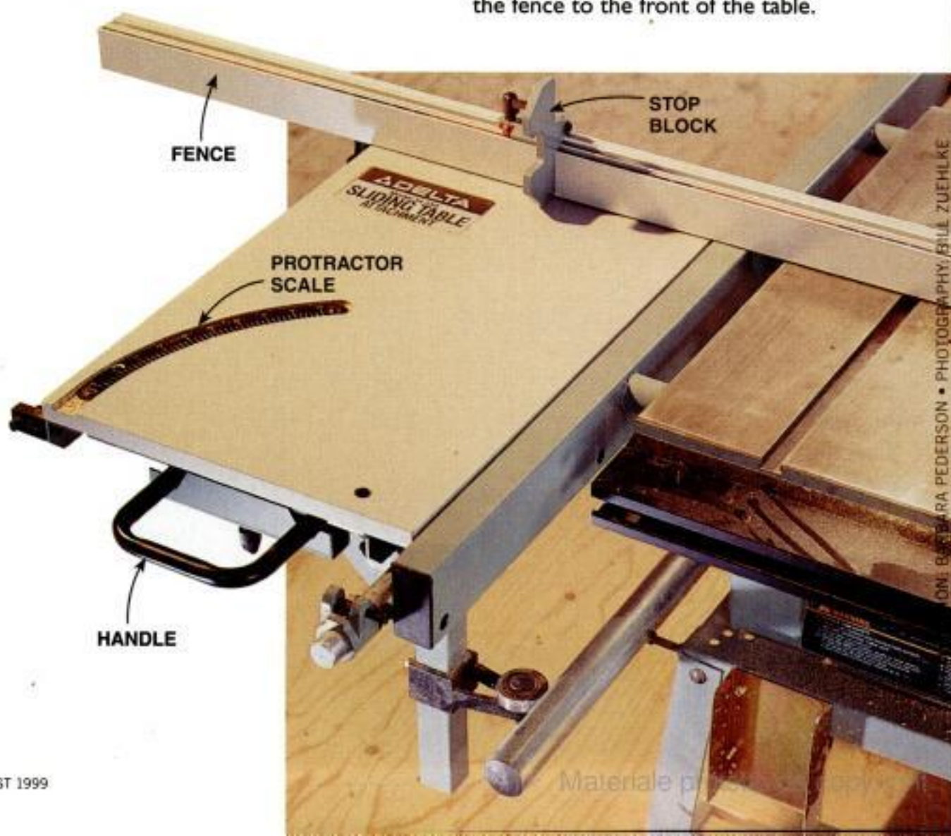
FOR EVEN GREATER CAPACITY, move the fence to the front of the table.
