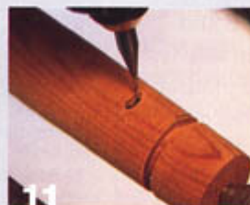
An alternative method is to start the slot with a Dremel tool and a small \frac{1}{32} " or \frac{3}{64} " milling cutter or drill.
