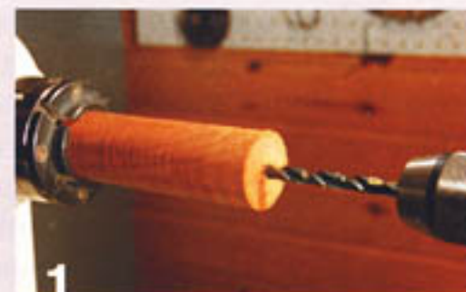
1 By inserting a Jacobs chuck in the tailstock, the lathe becomes a drill press. Drill a hole that will accept the bolster on one end and the chisel on the other.
