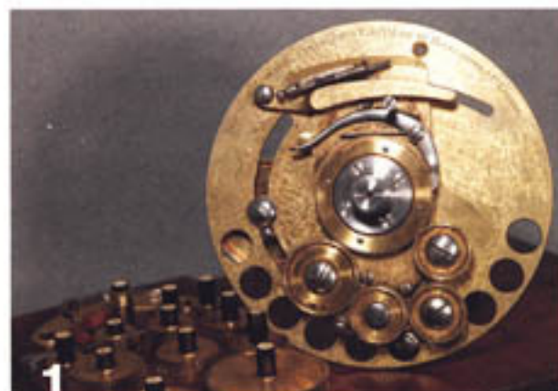
1 Single-stage geometric chuck from the Victorian era of OT.
