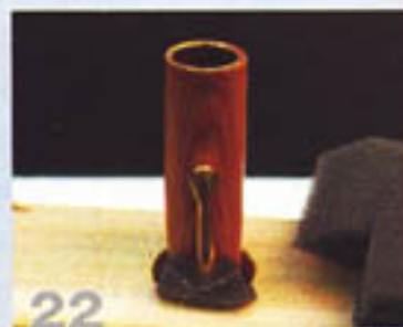
22 Hold the cap inverted until the glue has had at least 30 minutes to set.
