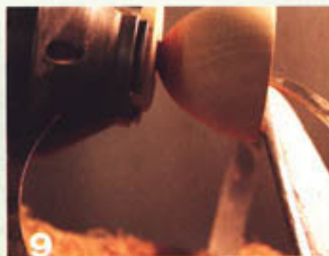
9 Using calipers, check the thickness of the bottom of the egg. Make sure to account for the thickness of the spigot.
