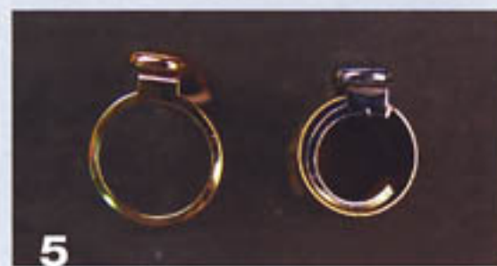
If the ring is larger than the tube, it has to be clipped and reshaped until it fits as shown here with the Baron clip in a Baron cap tube.
