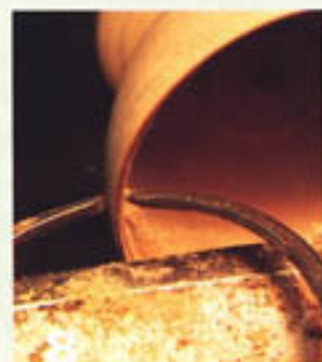
8 Check the thickness of the wall using a caliper. Make sure the thickness is uniform throughout the egg.
