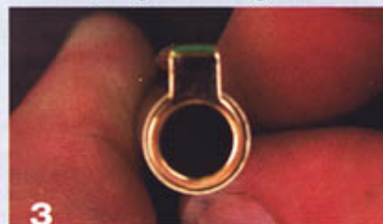
Using the brass tube as a sizing gauge, the ring must fit inside of the tube, as the El Grande shown here with the Baron cap tube.
