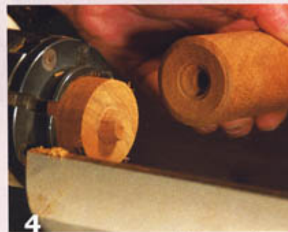
4 Turn a knob on the remaining stock to be used as a jam-fit chuck. After parting off the handle, I rotate it 180° and place the bolster opening onto the knob. Support the other end of the handle with a live center in the tailstock.
