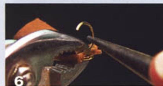
Bend the large ring after removing a 90° section. Use two pairs of pliers and hold the clip in a piece of leather to prevent damage to the plating.
