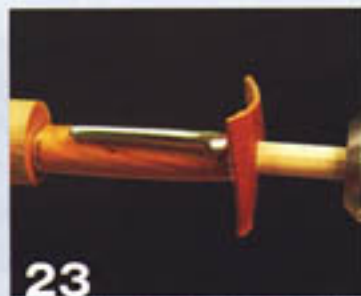
23 Push the center-band and threaded sleeve into the cap. The leather prevents damage to the finish. The cap is finished. Now make the other end of the pen.
