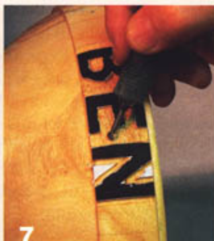
7 A micro motor carver is easy to control and works well for carving between the letters.
