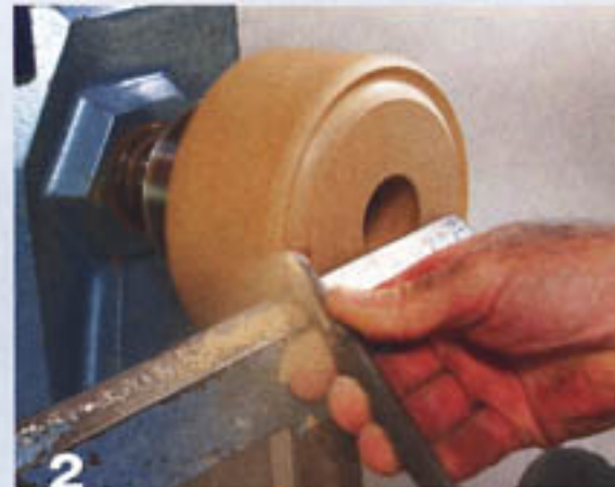
2 Turn the outside of the lidded doughnut form from the tailstock side first. Reposition the toolrest to turn the headstock side of the form.
