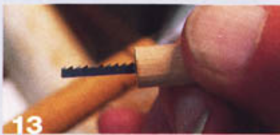
This slot-cutting tool is a piece of a coping saw blade, about \frac{1}{32} " wide.
