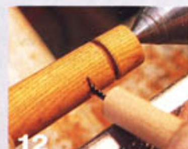
Continue cutting the slot with a small saw blade held in a piece of dowel.
