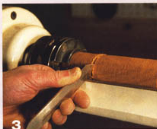
3 Part off a 4" length of the cylinder for the chisel handle.
