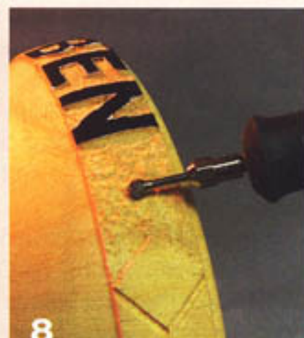
8 For more aggressive carving, a Dremel tool with a 3/16"-diameter spherical burr is used.
