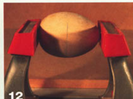
12 Glue the two halves of the egg together.
