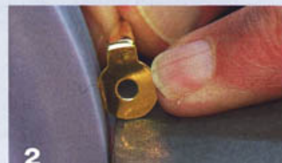
Grinding the flat washer. Keep it cool, and always hold it in the trailing position as shown. Make sure your toolrest is as close as possible to the rotating wheel.
