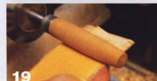
19 Sand and finish the cap.
