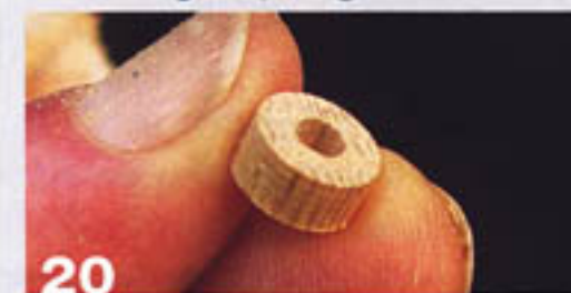
20 The plug that will hold the clip in place is ready to place in the hole.
