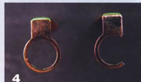
If the ring fits inside the cap tube, the only modification is to remove a section of the ring so it may be threaded to the inside of the cap, as with this El Grande clip in a Baron cap tube.
