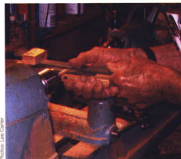
Doc "turning" a small spindle with a hinged rasp, one of his unconventional turning techniques.
