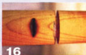
The burned area around the slot can be turned and sanded off.
