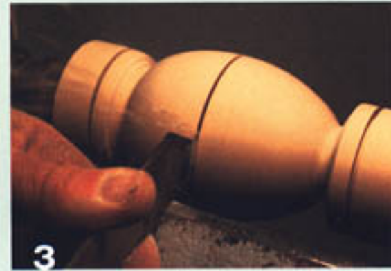
3 Use a parting tool to make a slight cut, indicating where the egg will be parted in half.
