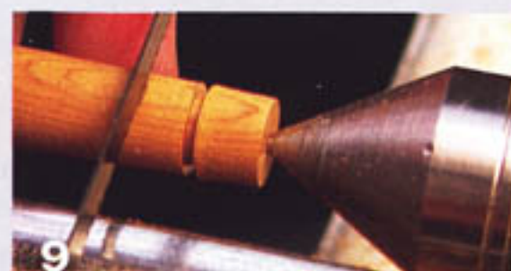
Locate the slot for the clip with a small saw that leaves a \frac{1}{32} " kerf.
