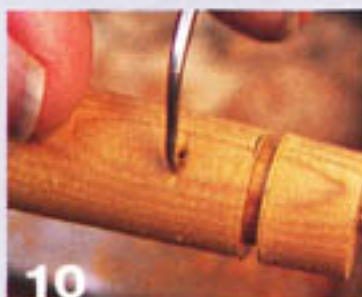
Start the slot with a sharp dental pick.
