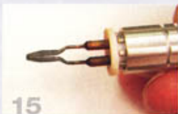
The slotting tool is a Detail-Master No. 2D calligraphy pen.
