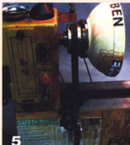
5 A band clamp is placed around the chuck and the lathe bed to stabilize the workpiece while doing the carving.
