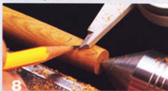
Mark the location of the clip slot and the end of the pen.
