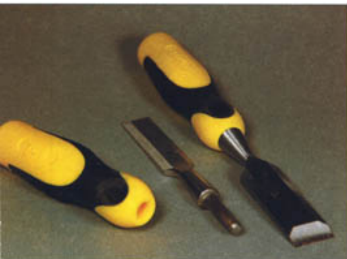
I separate the plastic handle from the steel chisel by placing the handled chisel in boiling water. The hot water softens the glue and makes it easy to separate the two.
