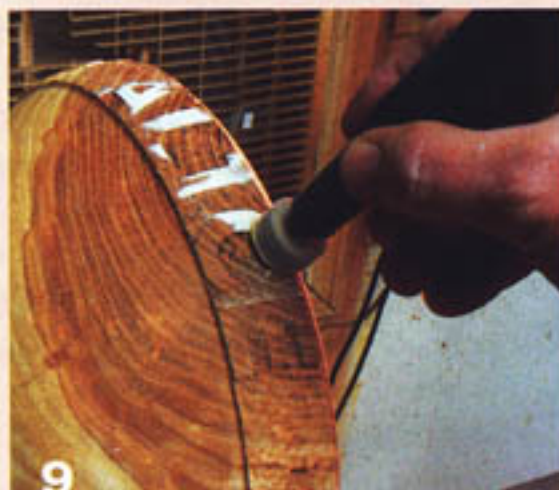
9 Using a shopmade 1"-diameter sanding arbor, sand the paper off of each letter.
