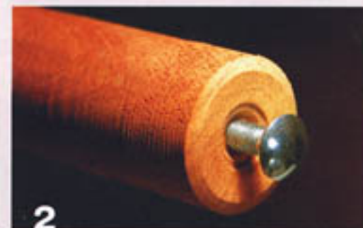
2 A carriage bolt becomes the bolster on the butt end of the chisel.
