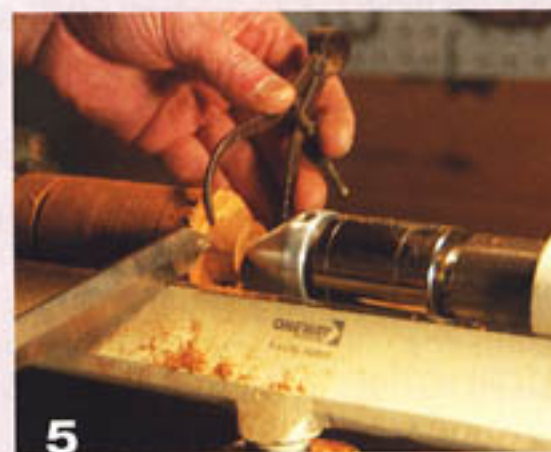
5 Turn a tenon on the handle for the ferrule and measure the diameter using outside calipers. I turn this tenon so that the ferrule fits loosely, leaving space for glue between the ferrule and the wood.
