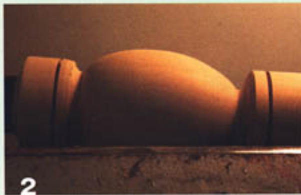
2 Turn the egg shape and leave spigots on each end to mount into a chuck. If your chuck has a large body, you will want to use the entire length of the spigots.
