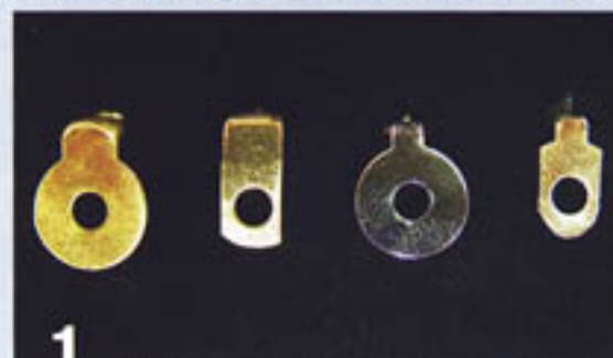
Left pair is the clip attachment for the Ameroclassic pen kit and its modification. The right pair is the Berea Perfect-Fit Convertible and a similar modification.
