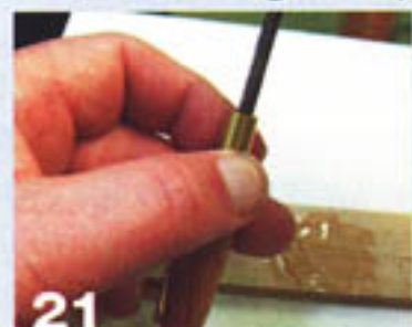
21 Mix and drop 5-minute epoxy glue into the bottom of the hole. Use a smaller brass tube to keep the glue off of the cap tube. DO NOT use CA glue.
