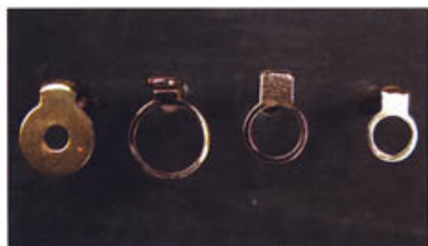
The shape of the clips, left to right: flat washer, large ring, small ring, and the hybrid which is a large ring on its parent kit, but becomes a small ring when used on a larger kit.
