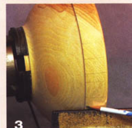
3 Draw vertical guidelines around the band to aid in placing the letters.
