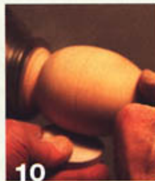
10 With one half still in the chuck, fit the second half to it, holding it in place with one hand. Sand the body of the egg where the two halves meet.
