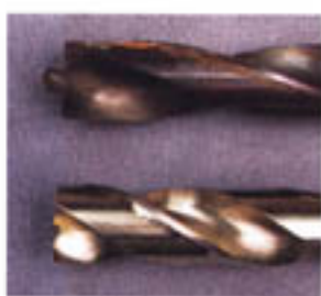
The cap blank is drilled with a \frac{29}{64} " or \frac{15}{32} " drill bit to achieve a square bottom. Use either a pilot point drill bit, or grind a bottoming drill.
