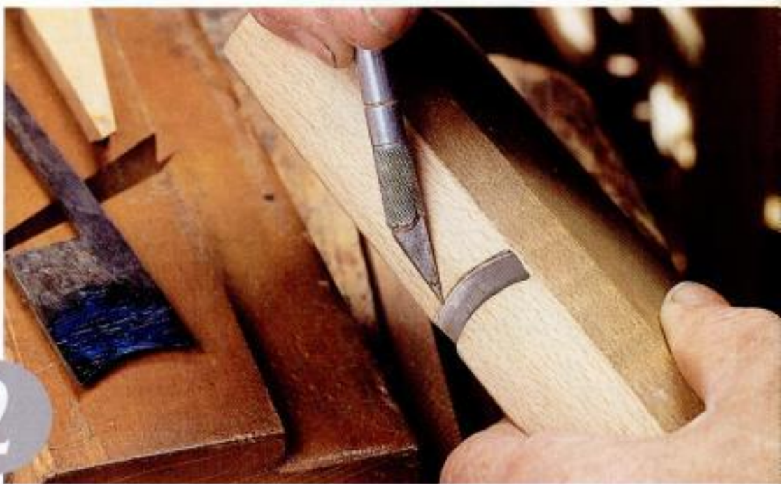
2 SCRIBING A ROUND IRON. To transfer the shape of the sole to the plane iron, coat the iron with machinist's bluing, then scribe it with a knife.
