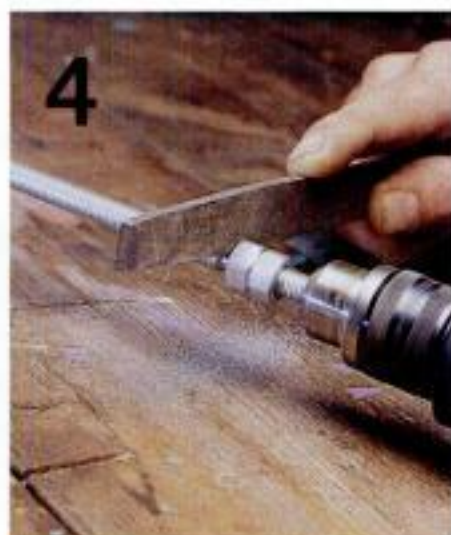
4 A GROOVED, THREADED ROD is at the heart of the adjustment mechanism. The groove is made with a file while the rod is turned slowly in a drill or drill press. Two nuts tightened against each other make a stop to help control the file.
