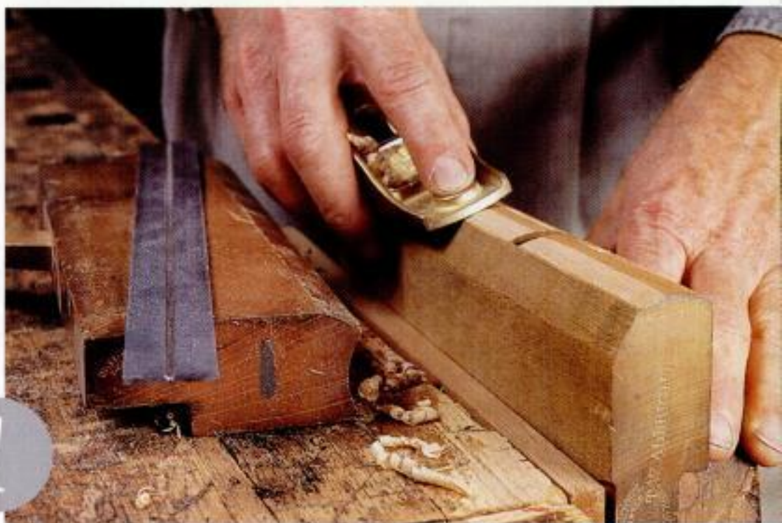
1 PLANING THE PLANE. The bottom of an old plane often needs to be reshaped. I used a block plane to true up the bottom of this round plane before smoothing the contour with sandpaper.
