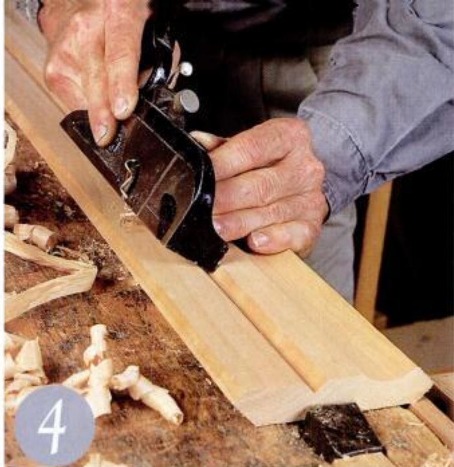
PLANING THE SHOULDER. A rabbet plane cleans up any saw marks left on the molding's shoulder.
