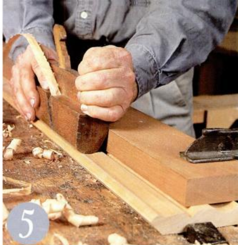
STARTING STRAIGHT. Guide the first few hollowing passes with a wooden straightedge that's clamped along the workpiece.
