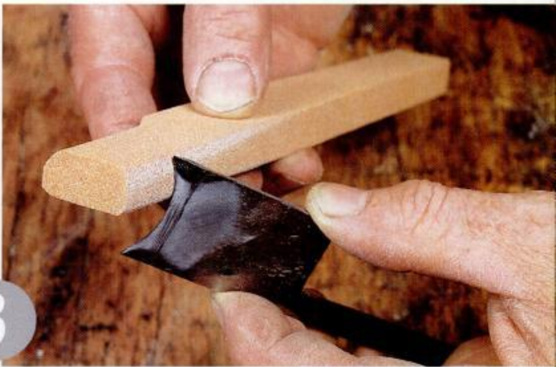
3 HONING A HOLLOW IRON. After grinding the iron, I bring it to final shape using a modified "roughing" stone.
