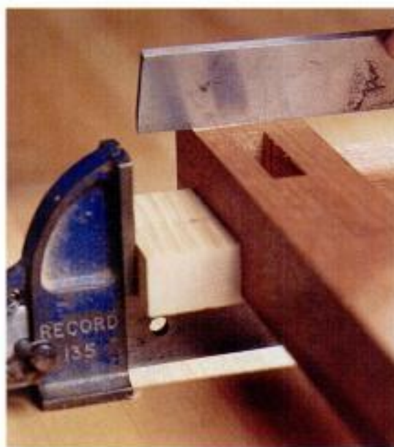
CAREFUL ALIGNMENT of clamps and blocks keeps your work flat and square.
