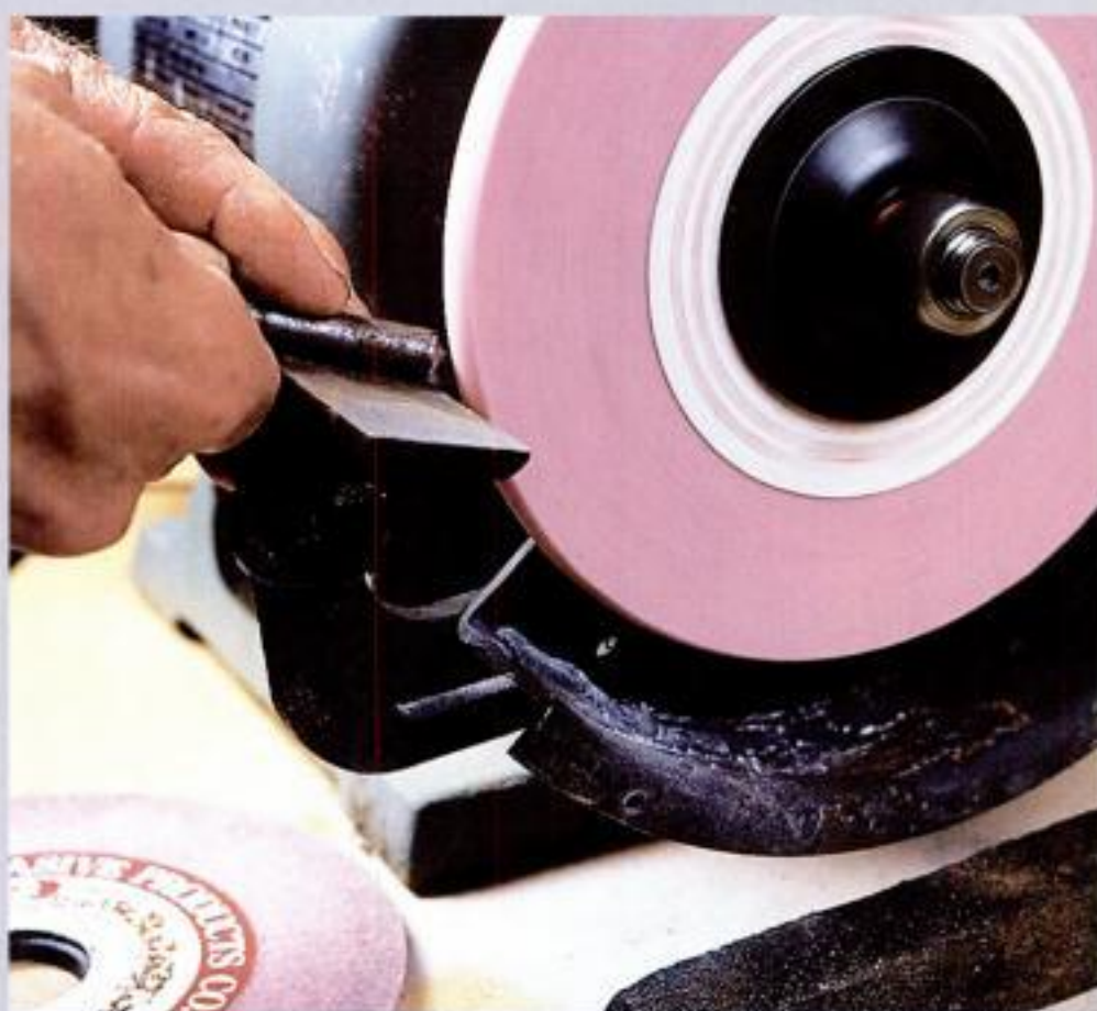
DRESSING A WHEEL. A diamond-point dresser will shape a soft grinding wheel to any profile you need for grinding concave plane irons.
