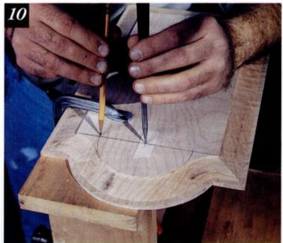
MARK THE INSIDE CORNERS that the panel-raising bit couldn't reach, by extending the shoulder using a compass and small square.
