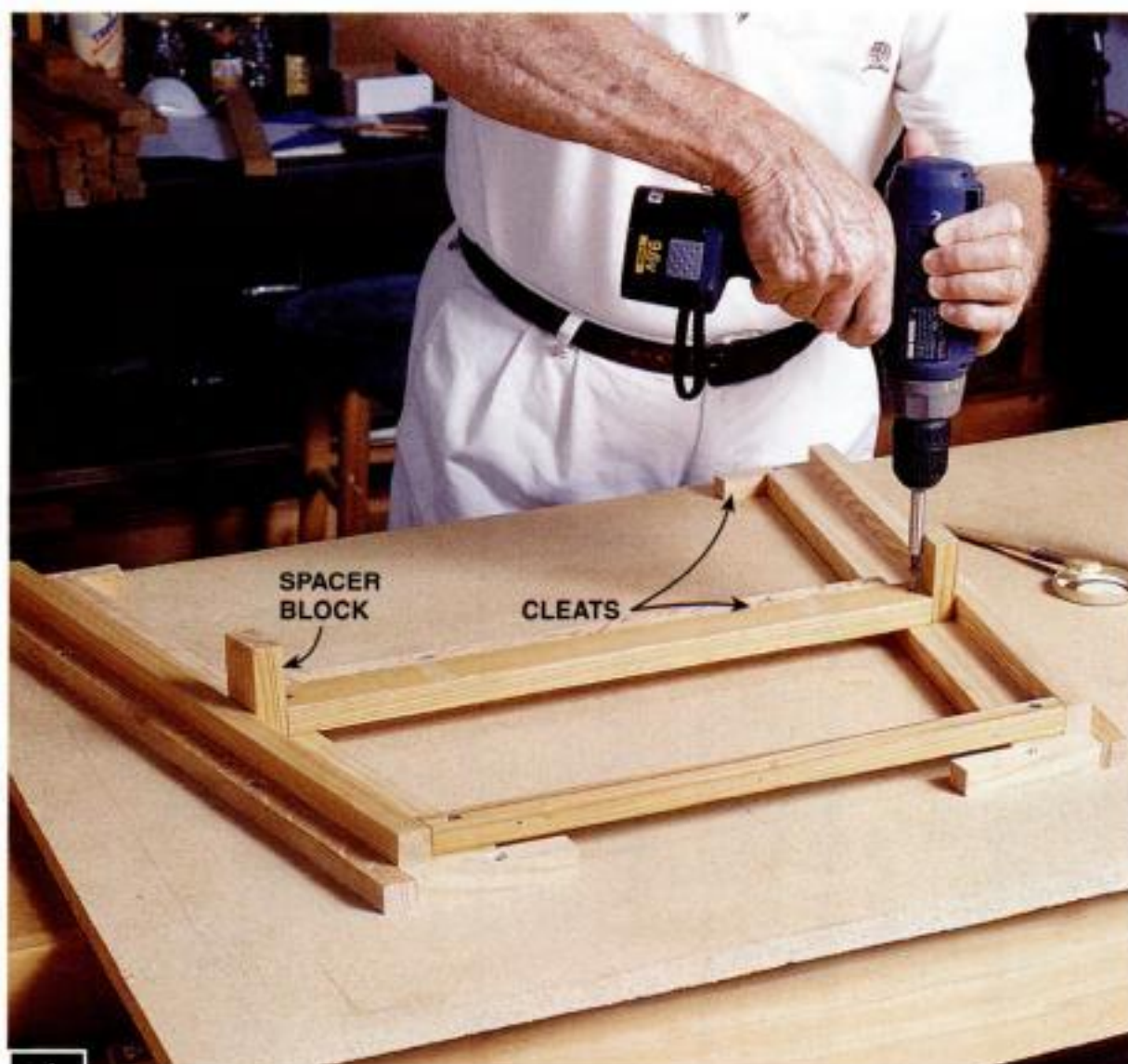
1 ASSEMBLE THE SIDES on a jig to keep the legs in position. The side rails are cut to fit, using spacer blocks to stand for the front and back rails.
