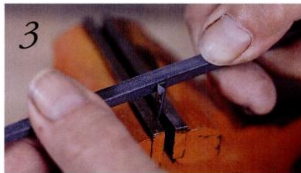
FORM THE CUTTING EDGE with a file and diamond hone, then straighten the shank. If this is the only tool you're making, proceed to heat-treating (Photos 10 and 11) and attaching a handle (Photo 12).
