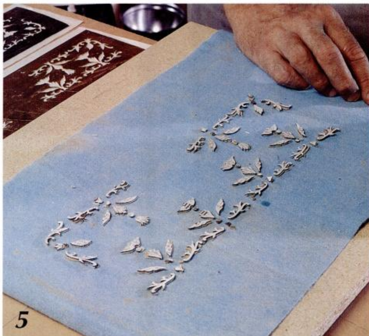
ARRANGE THE CUTOUTS on a felt-covered board that is larger than the finished sheets will be. When you're done, separate the packet and you'll have a wood background and a brass background, each with the pattern cut in it.
