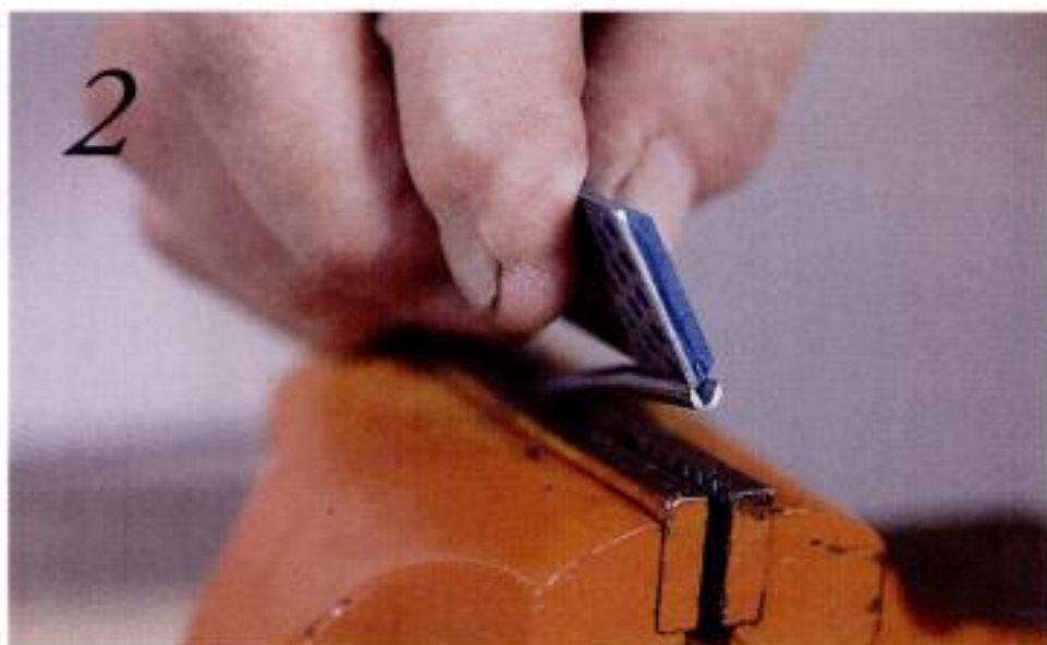
REFINE THE INSIDE with a diamond hone ($10). You may need to file down the plastic sides of the hone so it will fit in the tiny V.
