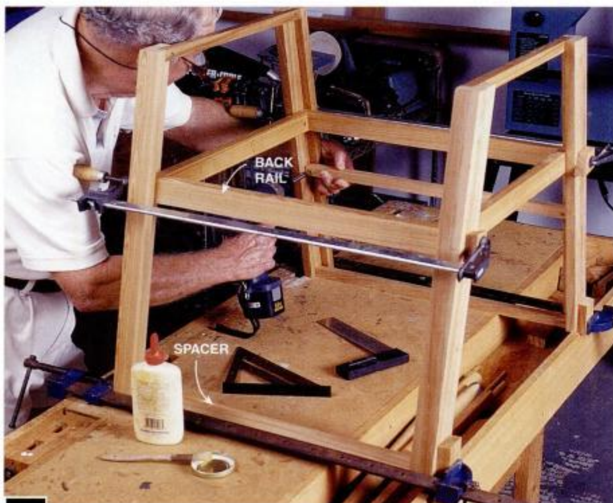
2 CONSTRUCT THE FRAME by attaching the front and back rails to the two side assemblies. A couple clamps and a spacer between the back legs will help.
