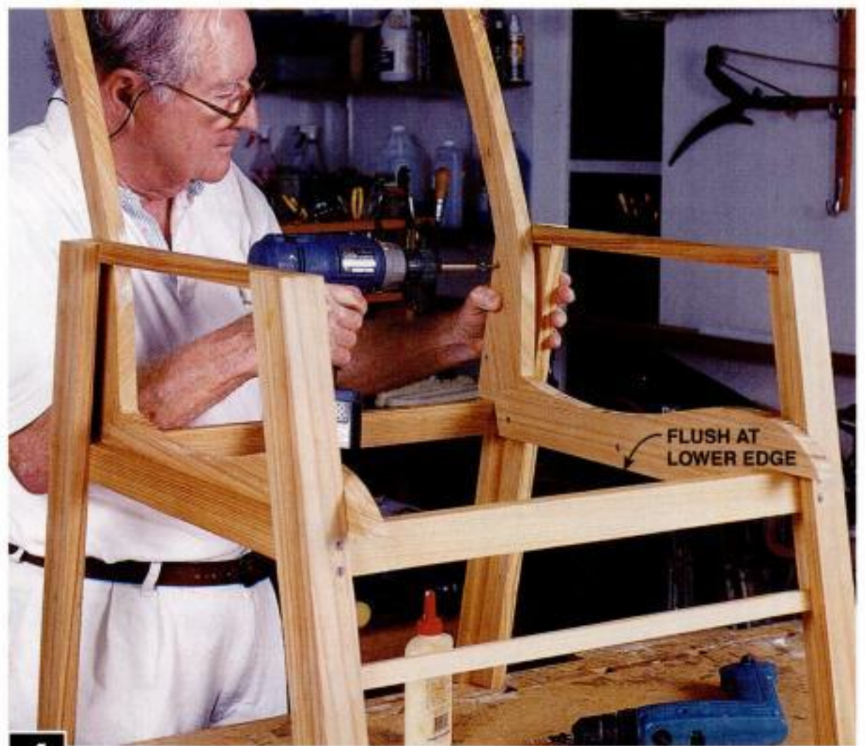
4 SCREW THE SEAT SUPPORTS to the seat rail and the rear leg, checking to make sure they are parallel and 1/8 in. in from the back edge of the leg. Shape the armrests, then glue and screw them on.
