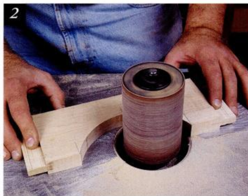
2 SAND THE CURVE SMOOTH and to your layout line using a spindle sander or sanding drum in a drill press. Be sure it's a fair curve without dips or flat spots.
