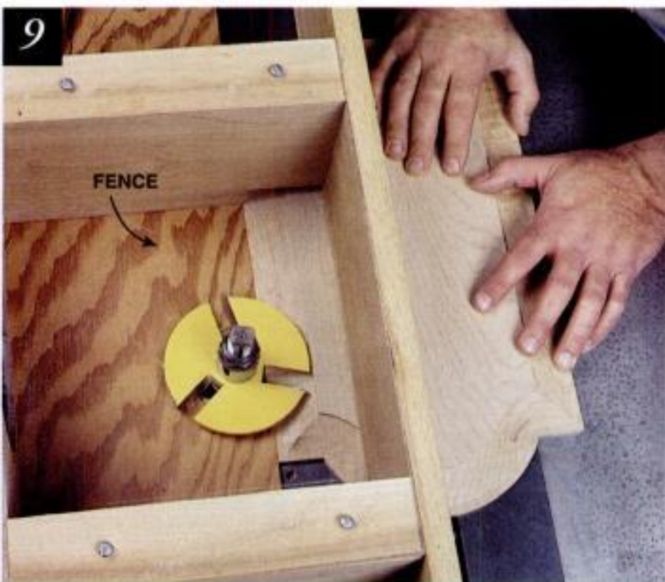
RAISE THE STRAIGHT EDGE of the panel with a similar jig, but use a fence instead of the guide bushing or pilot bearing.
