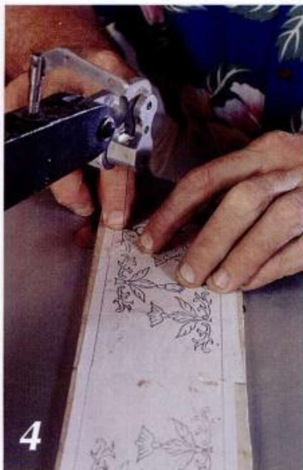
CUT OUT THE PATTERN using a scrollsaw with an extremely fine blade. Cut directly on the lines.
