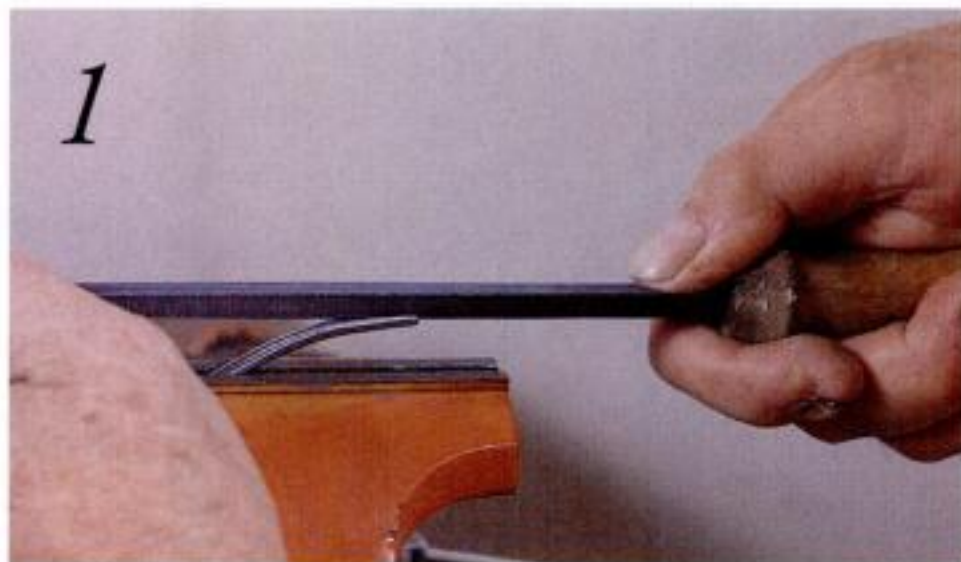
FORM A V-SHAPE with a triangular file on the end of an 18-in. piece of 5/32-in. drill rod. Bending the tip of the rod will give you room to work.
