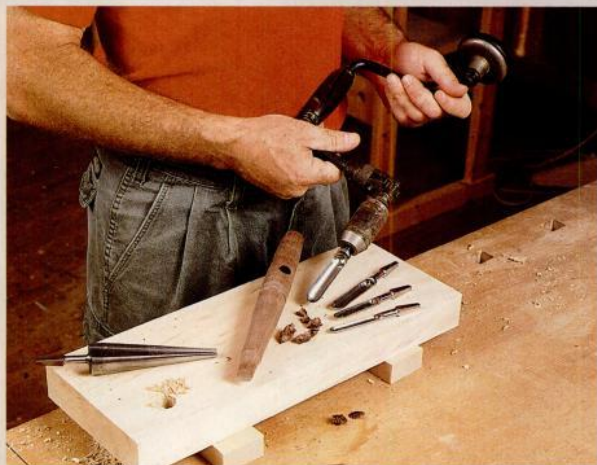
Chair tools. Spoon bits, shown here in sizes ranging from 3/8 in. to 5/8 in. (right), let you cut angled, round-bottomed holes. A tapered reamer (at left) cuts a tapered hole for a snug fit to a tapered tenon.
