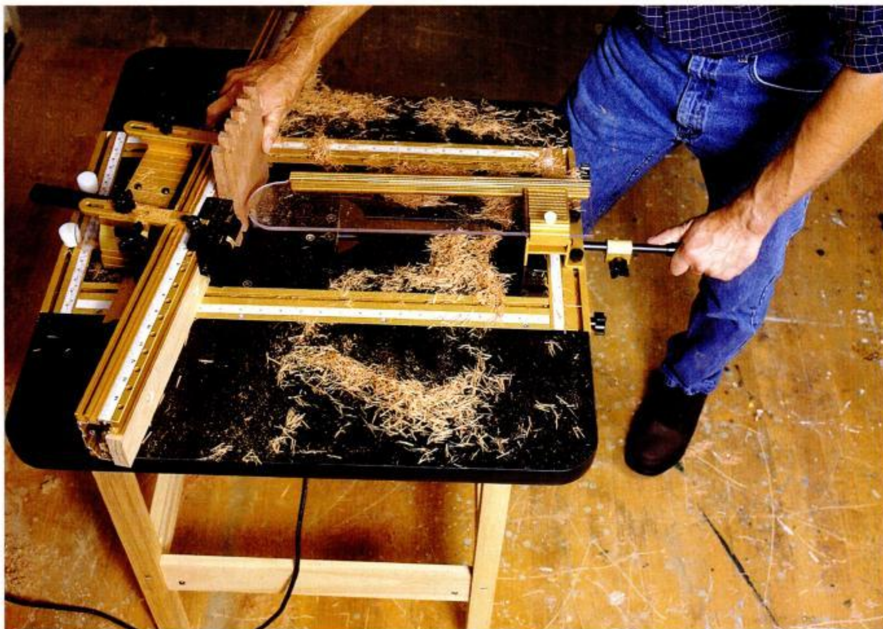
Sliding action. Rout-R-Slide lets you make dead-straight cuts by pushing or pulling a handle to move the router.
