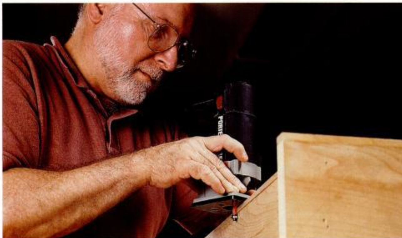
Flush-trim the edging. Strips of hardwood milled slightly thicker than the case sides are glued and nailed to the plywood edges, then routed flush.
