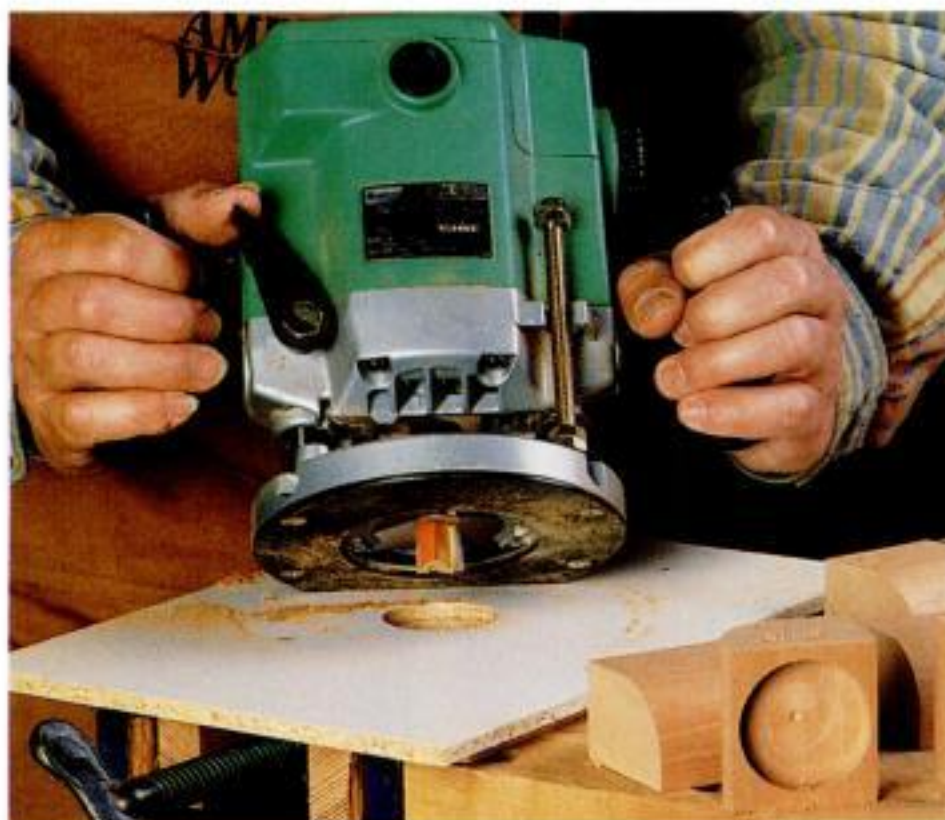
Rout the lid mortises. A shop-made template clamped in a vise makes routing the lid mortises fast and accurate.
