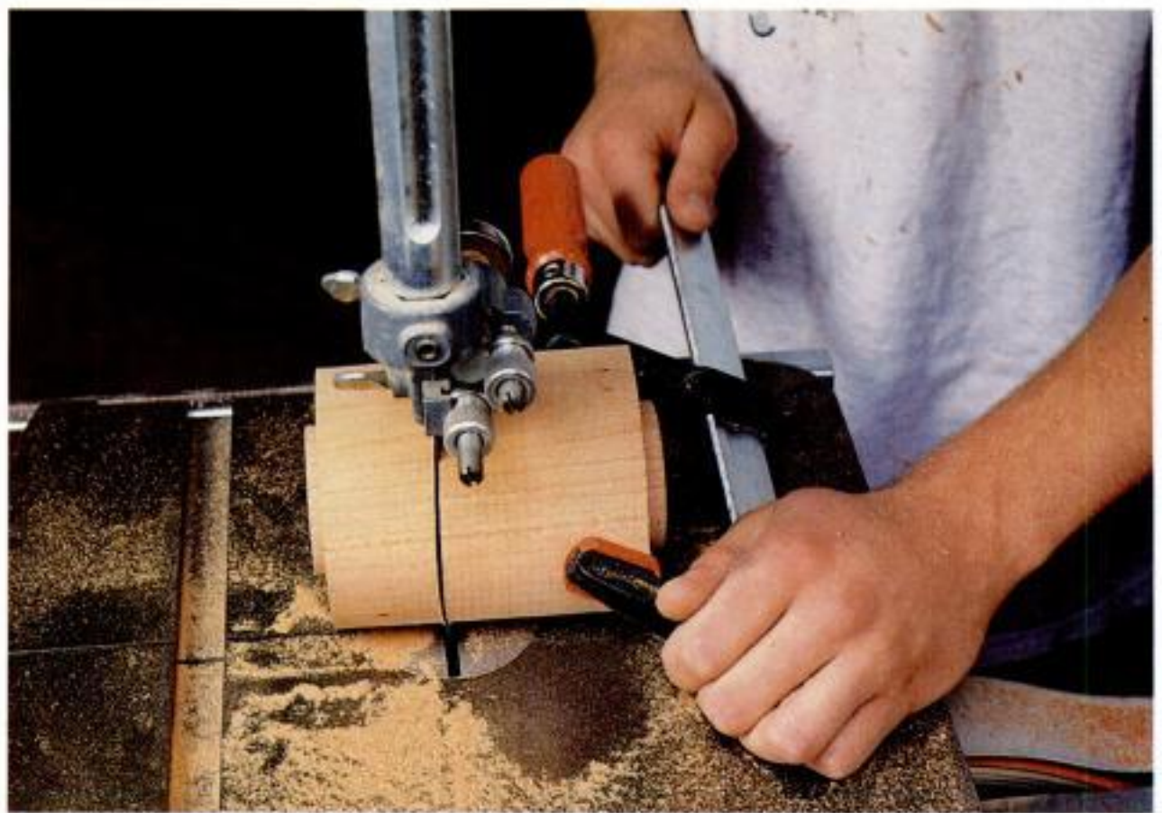
Safe separation. After you turn a cylinder, cut the lid and body blanks apart on the bandsaw. A quick-action clamp helps to hold the cylinder safely—be sure the clamp rests on the table.
