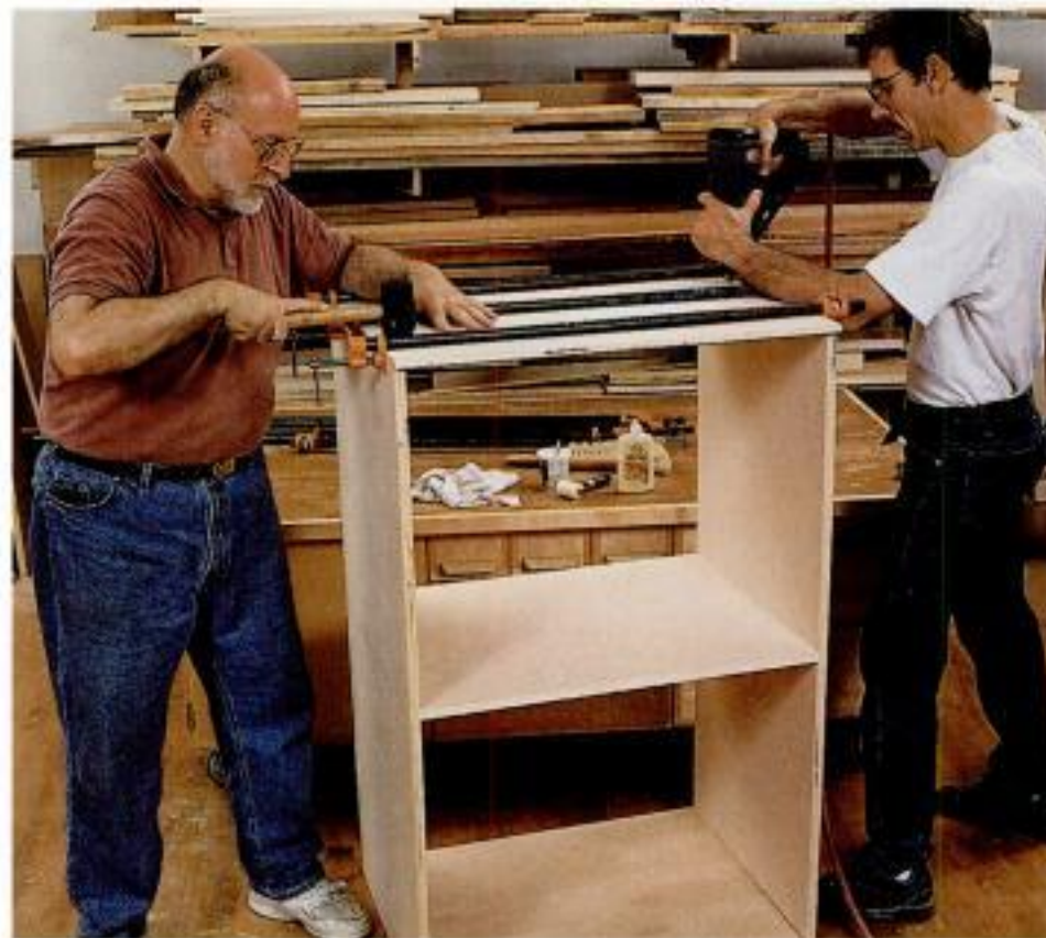
Assemble the case. Pipe clamps and a rubber mallet coax glued joints snug. The clamps can be removed after nailing.
