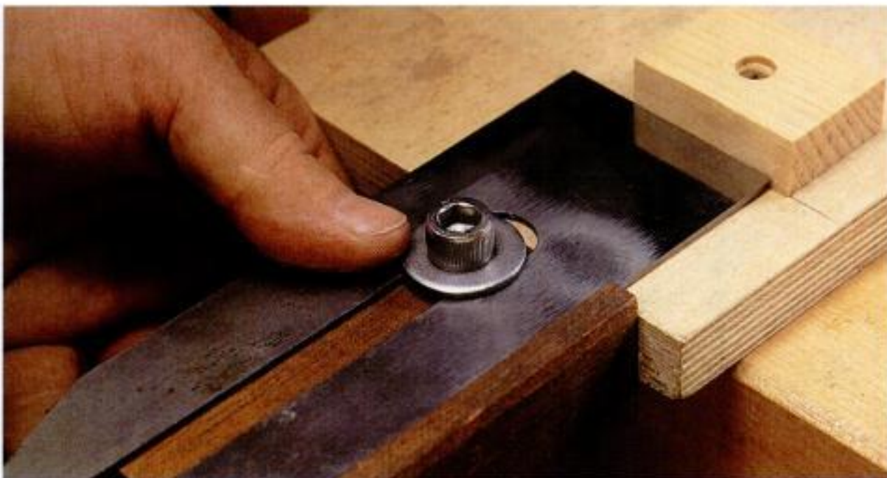
Set the angle. How far the plane blade projects from the holder determines the grinding angle. Find the angle by trial and error, then lock it in with a stop block on the grinder baseplate.
