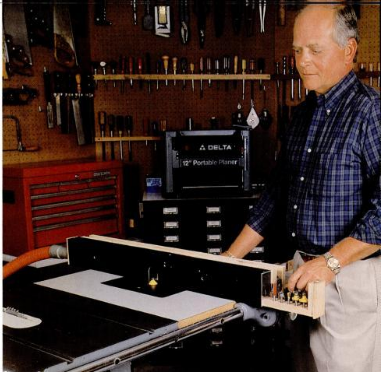
Space saver. This detachable router fence offers bit storage and dust collection in a compact package.
