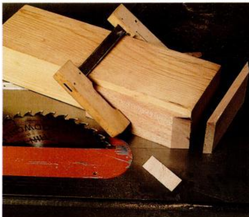
Cutting the roof miters. To cut an angled roof piece, the author clamps it to either the side or the end of a right-angled block that slides in his table saw's miter gauge slot.
