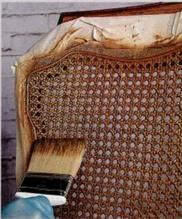
Step 3: Imitate wear. Drag a dry, soft-bristle brush over the wet color coat to highlight areas of normal wear, such as around edges and high points. Seal with two coats of spray shellac.
