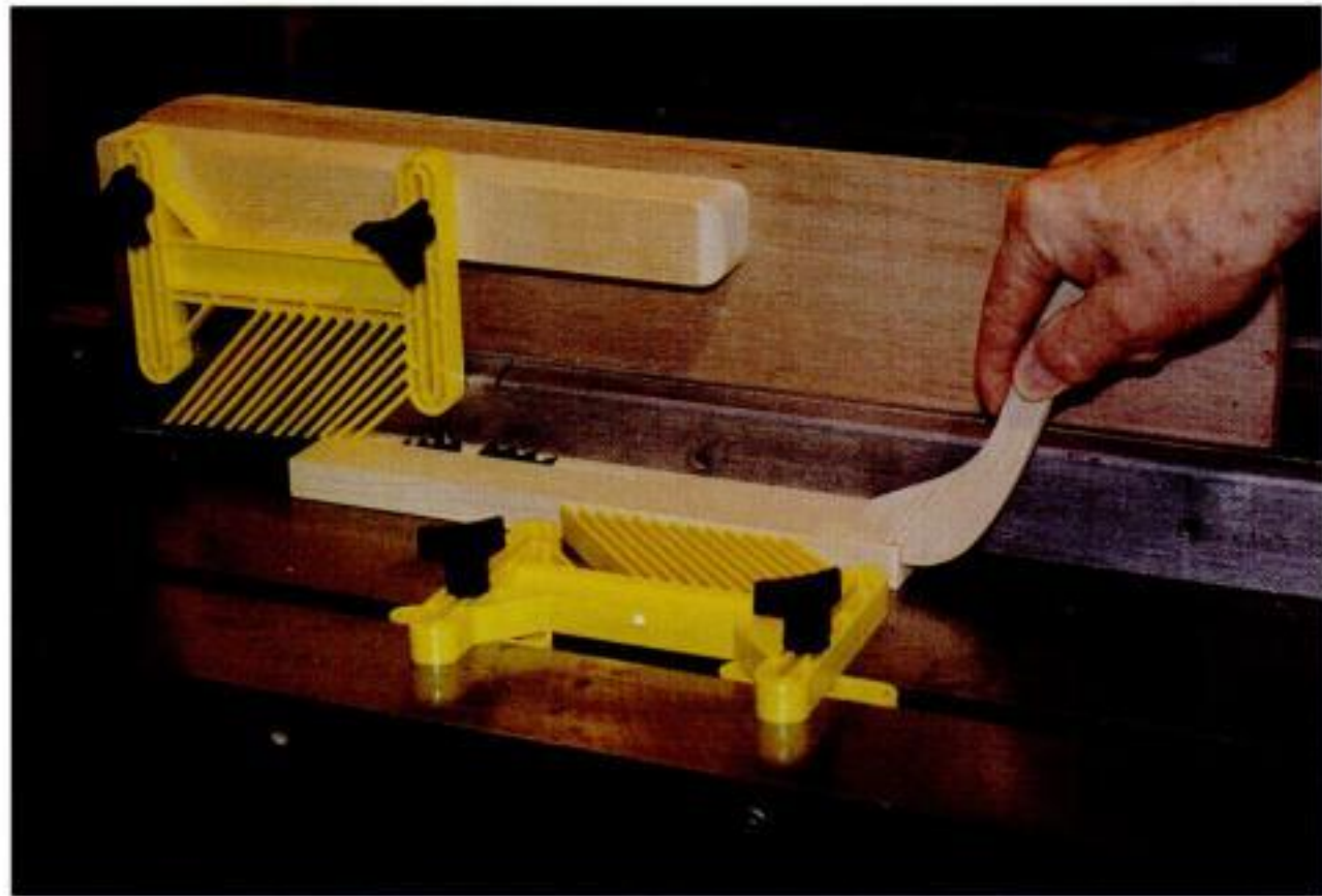
Factory-made featherboards. Inexpensive (about $10) and easy to use, these plastic featherboards can work horizontally and vertically.
