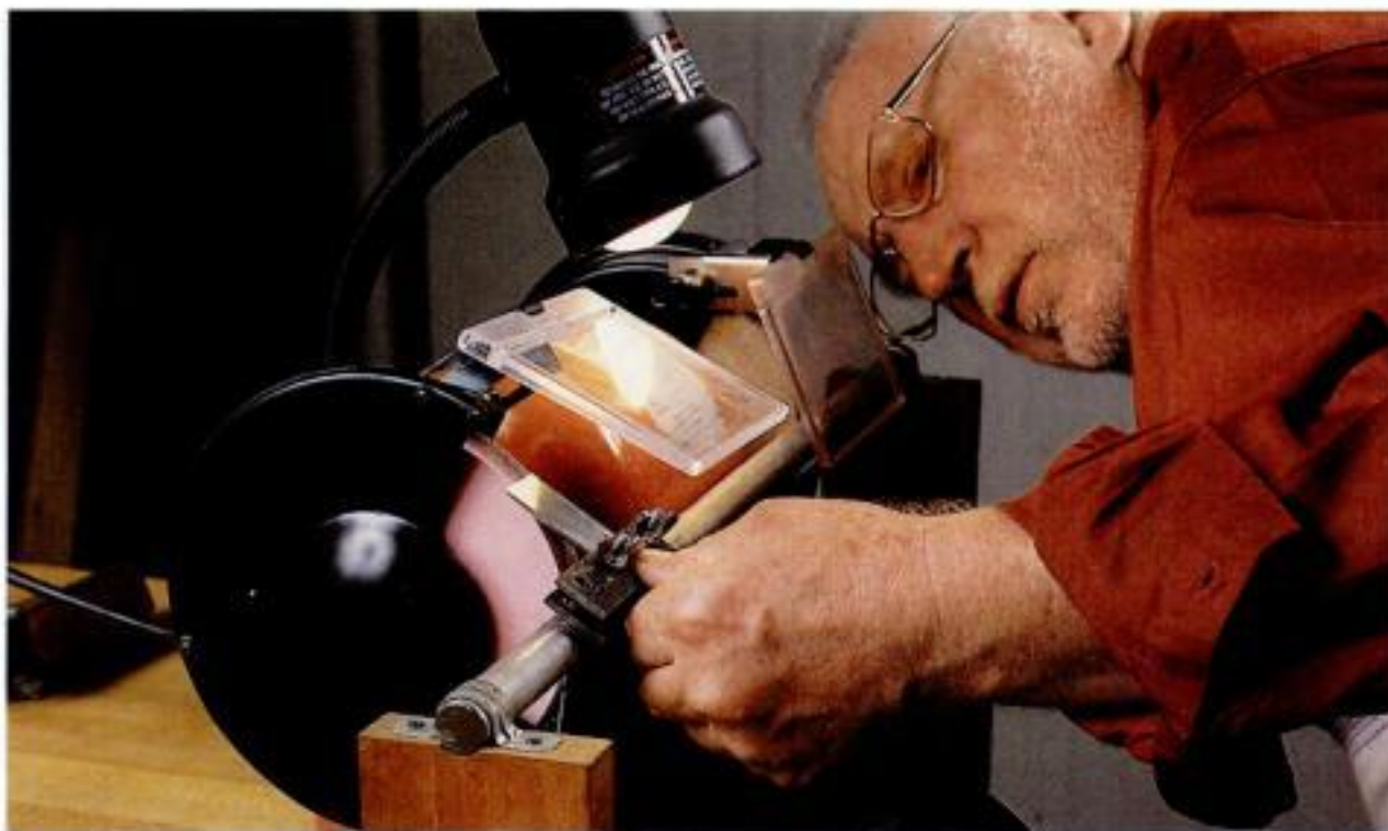
Check the angle. Load the chisel into the holder and pivot it onto the grinding wheel. Adjust the grinding angle by changing the chisel's position in the holder.
