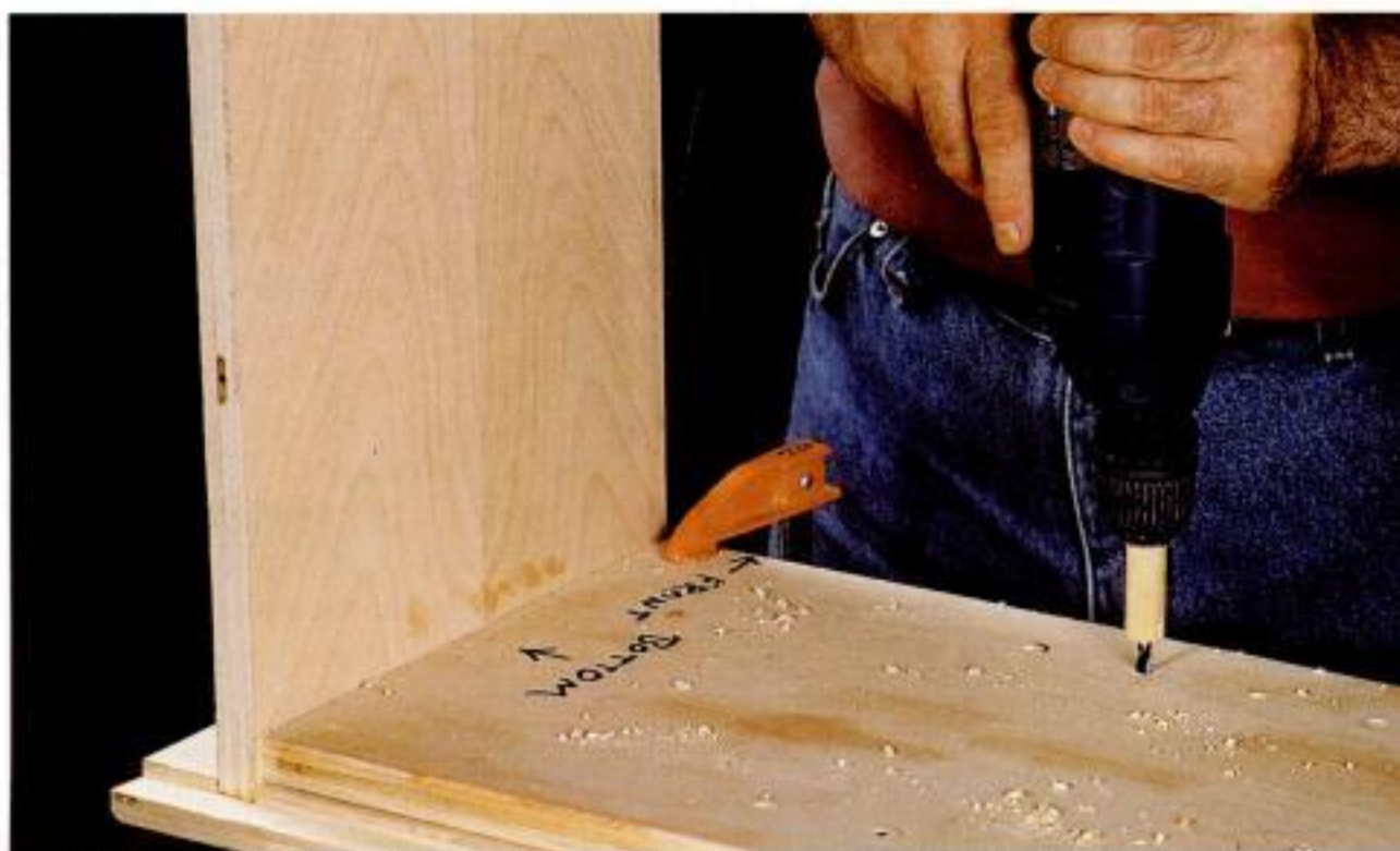
Drill the shelf pin holes. A shop-made jig simplifies drilling the holes. A 1/2-in.-dia. dowel serves as a drill depth stop.
