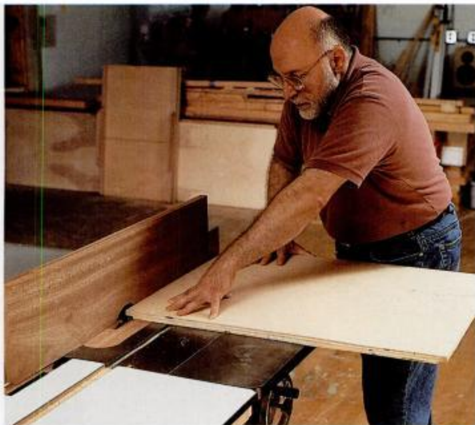
Cut the case joints. When rabbeting case pieces, use a notched, wooden auxiliary fence to protect your rip fence.
