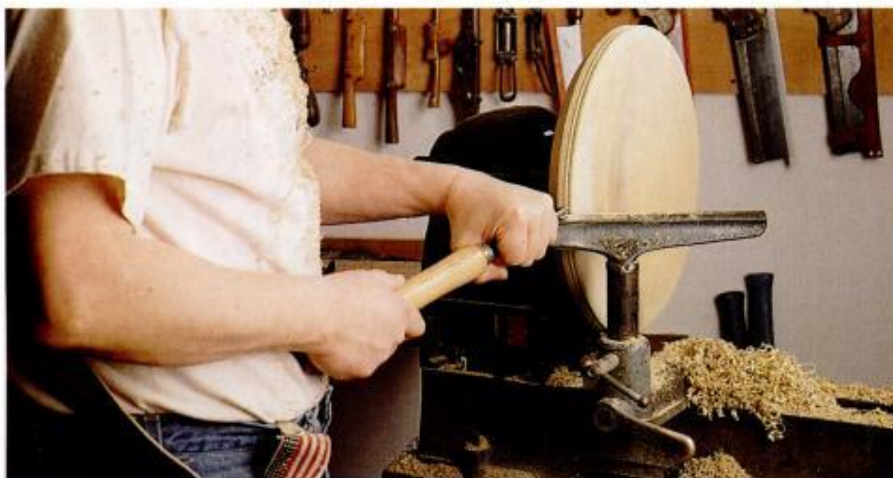
Turn the seat. After dishing the seat and chamfering the underside, Dunbar uses the long point of a skew to cut a decorative bead on the edge.
