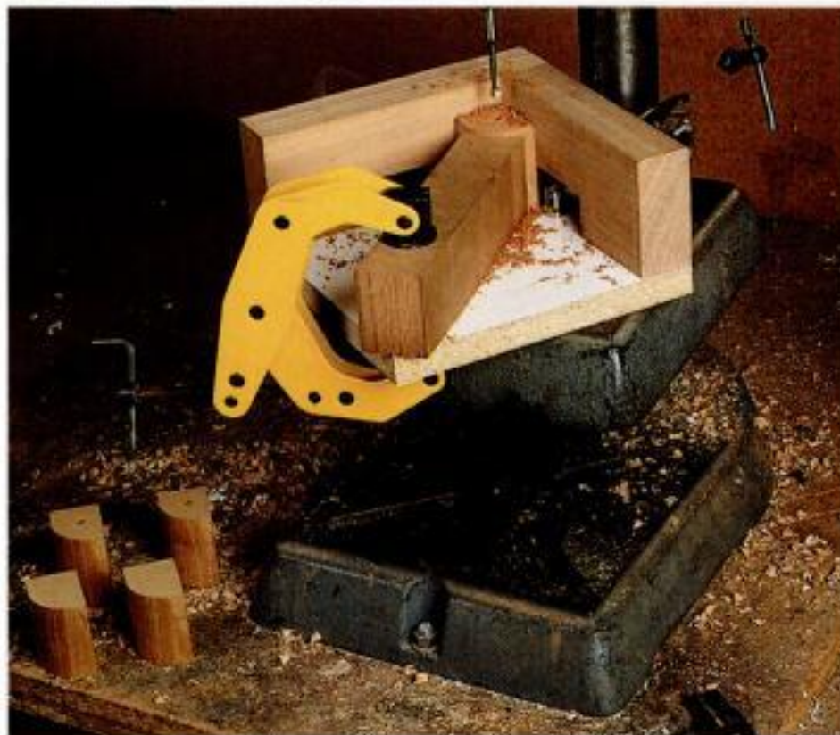
Drill the pivot holes. The author's jig ensures accurately positioned pivot holes. A clamping arm presses the workpiece against the jig's fence.
