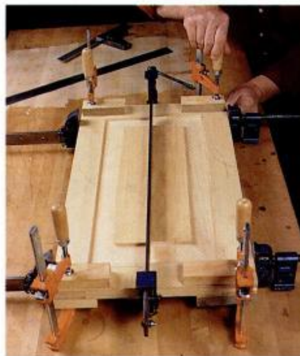
Clamping it up. Long bar clamps pull the frame tight; shorter ones close up the corner joints.
