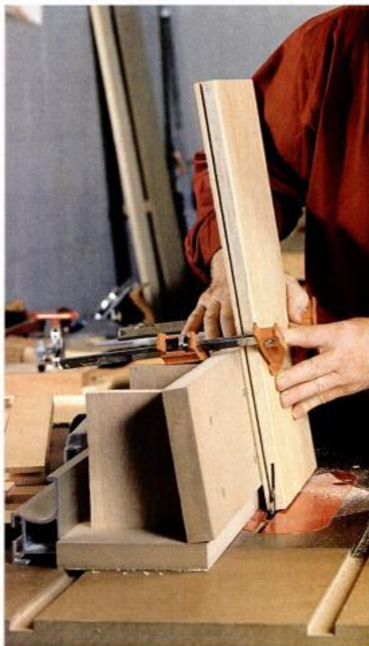
The blade stays vertical. This jig works great because it allows solid clamping and because the workpiece is beveled, not the blade.
