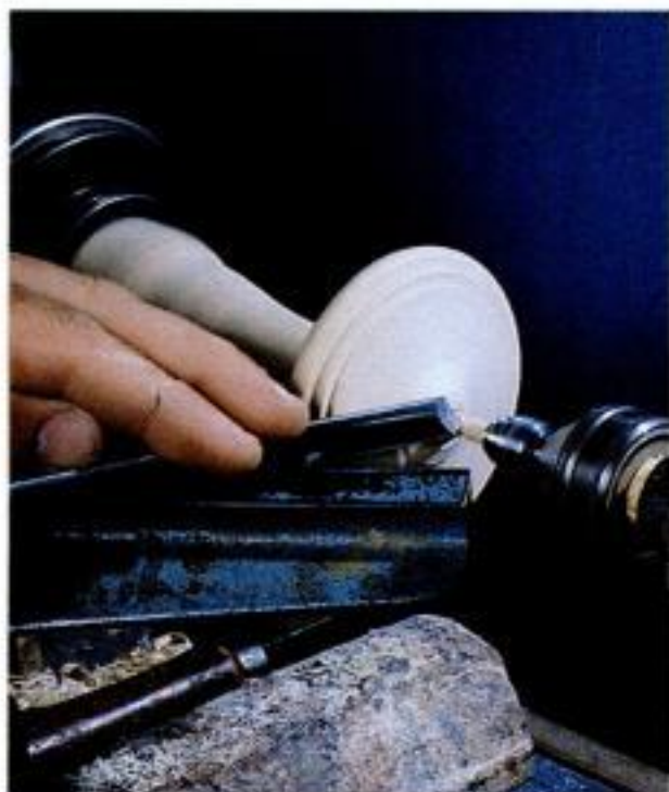
Turn the tip last. For a dead-center tip, turn it after the rest of the body and shaft, using light cuts with a skew's tip.
