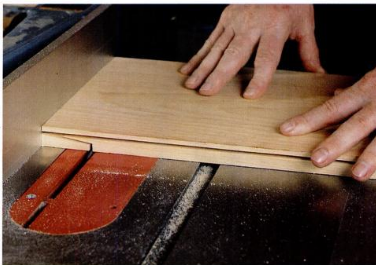
The shoulder cut frees the waste. Blade height equals shoulder depth. The rip fence guides the edge of the panel.
