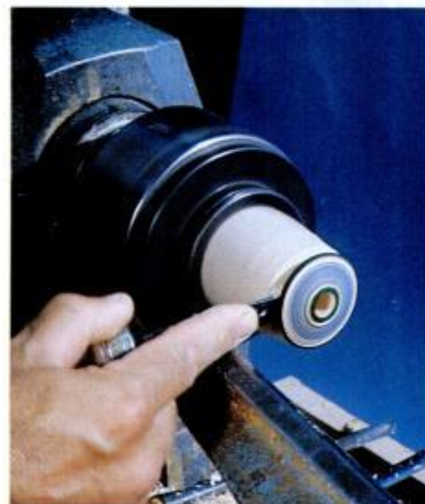
Part a disk. Turn and decorate the outside of the blank, then make a concave parting cut to free the disk.
