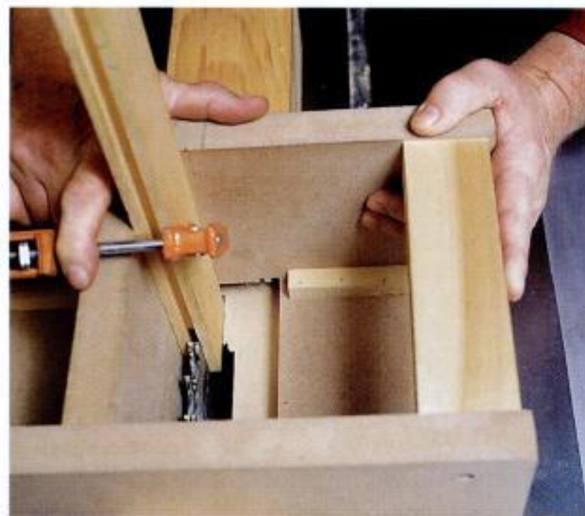
Mortising the stiles. Kirby's tenoning jig is designed to run against the rip fence, and will also cut open mortises.
