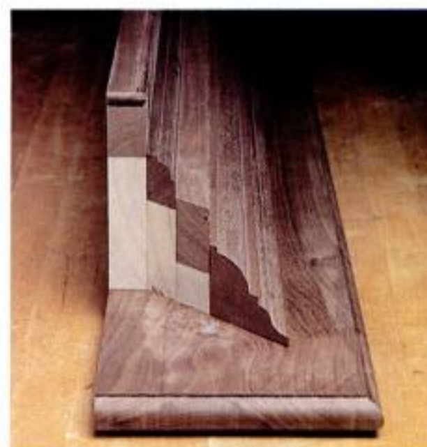
A stack of moldings. Shown upside down, the author's shelf consists of walnut moldings stacked together, with poplar as a secondary wood.
