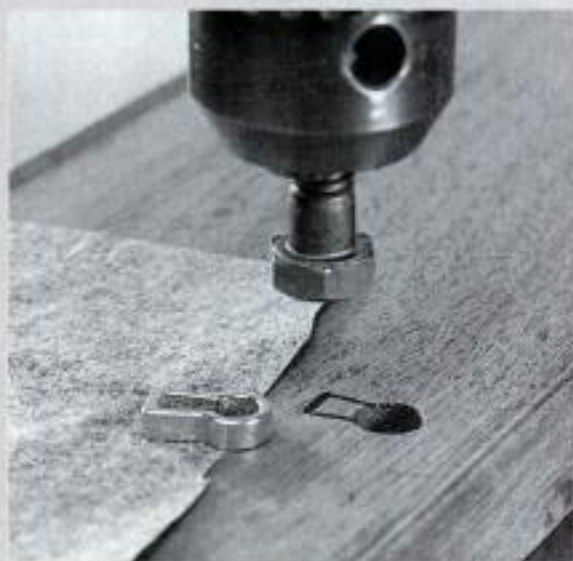
Pressing news. Chuck a bolt in the drill press and press the escutcheon against carbon paper to lay out the skirt mortise.
