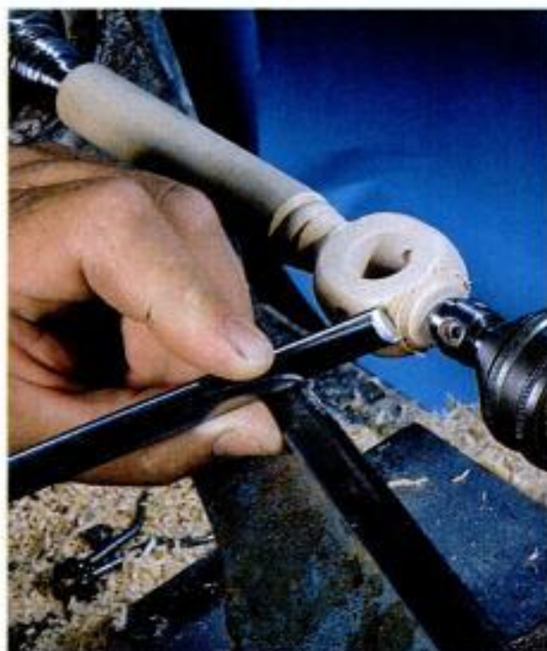
A handle with two holes. Bore the right-angled holes before mounting the blank for rounding.
