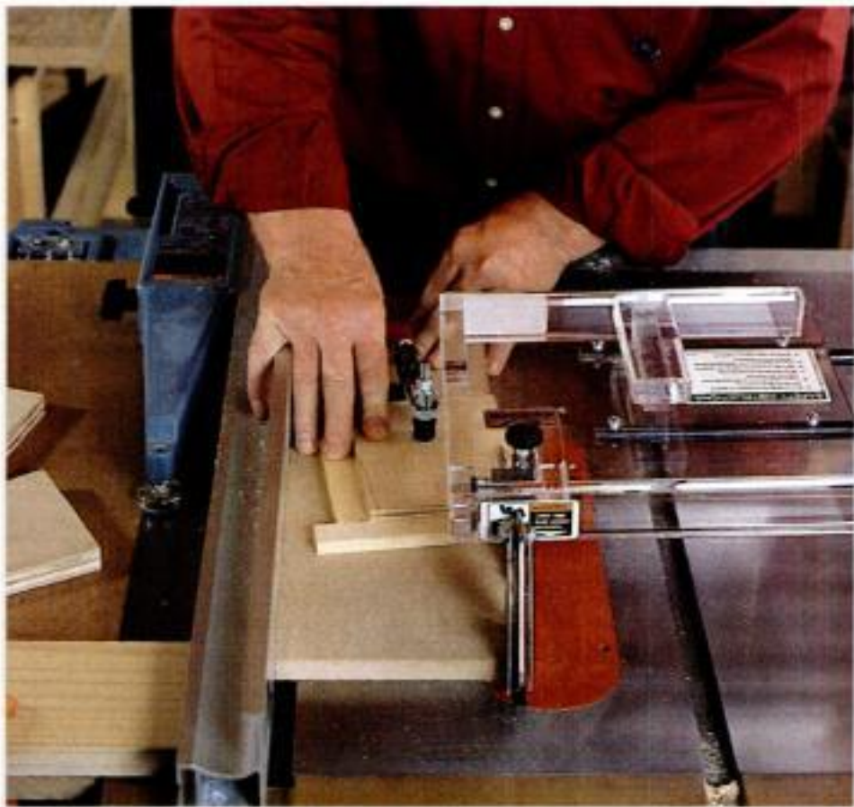
A duplicate parts jig. A slab of MDF serves as the base, which runs against the rip fence. Stop blocks and a toggle clamp keep the buttress blank positioned exactly.
