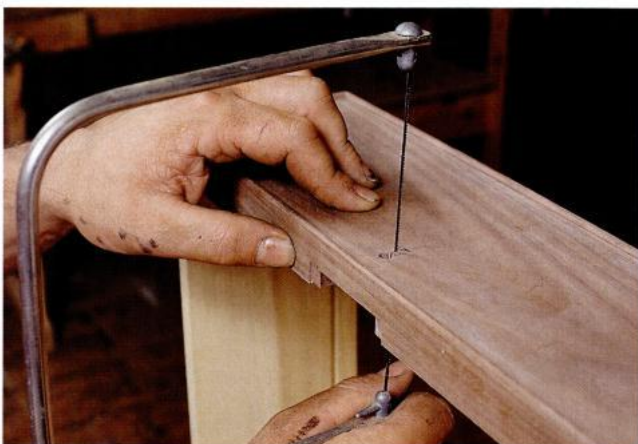
Cutting the keyhole skirt. Use a coping saw to cut out the skirted section of the keyhole, then clean up the edges with a chisel or file.
