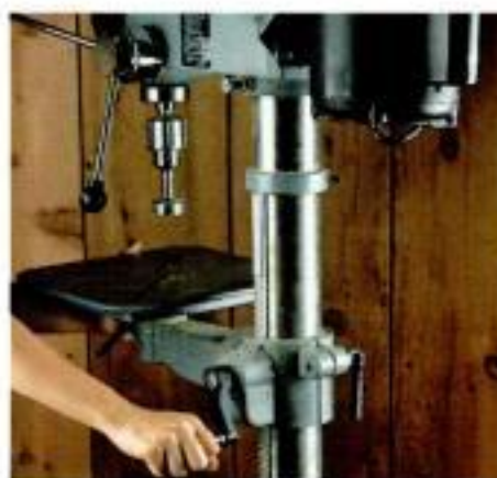
Crank it up. A rack-and-pinion mechanism makes it easier to adjust heavy cast tables.
