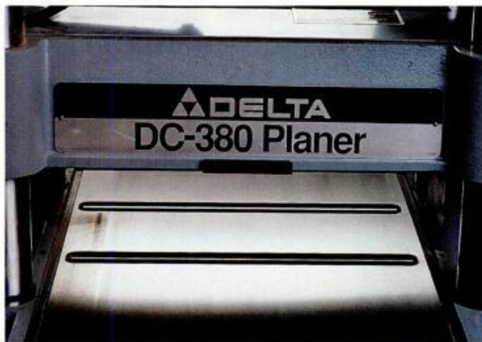
Friction fighters. Bed rollers and a smooth cast-iron bed can handle heavy use and large, long stock.
