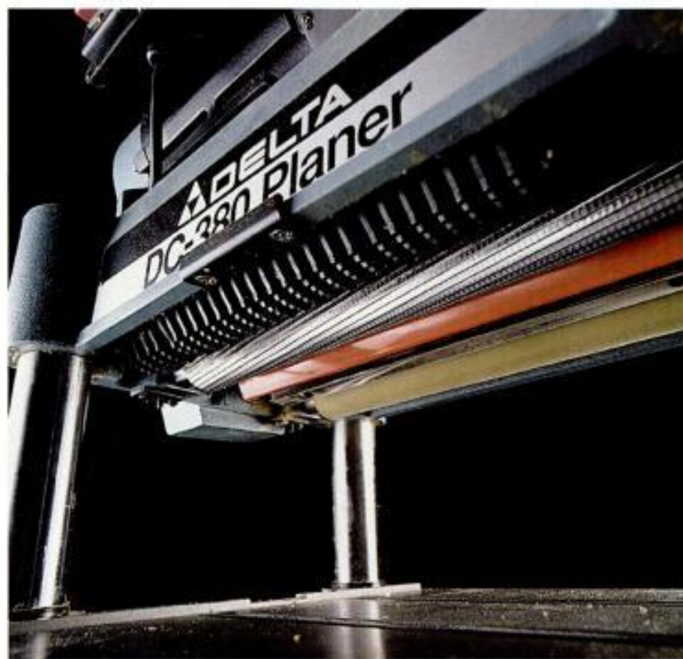
Infeed rollers. Serrated infeed rollers are effective in moving heavy boards through the machine.
