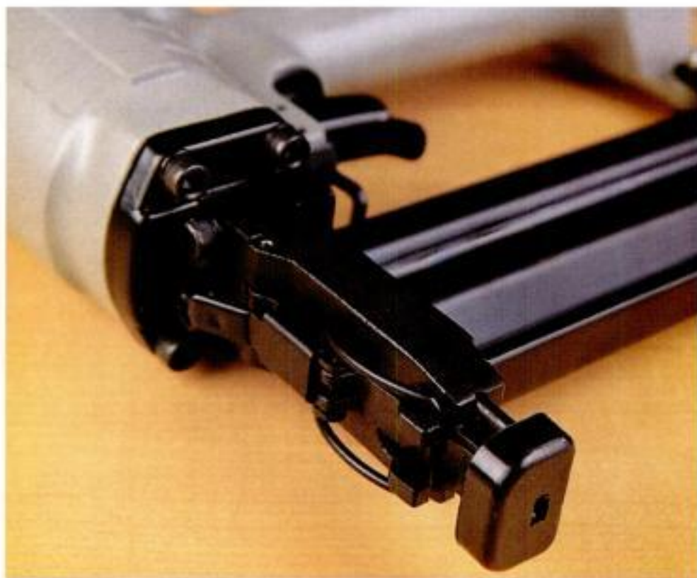
Rubber nose tip. A rubber nose tip keeps wood from being marred by the gun's nose.
