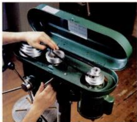
Simple speed control. A step-pulley system regulates spindle speed on most models.
