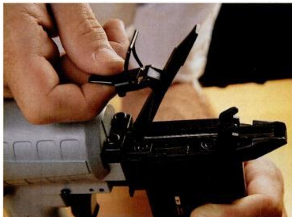
Quick-release nosepiece. A draw-catch release allows quick access to the firing compartment for clearing jammed nails.
