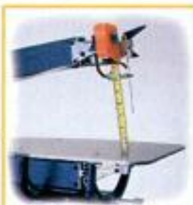
Top arm lifts for easier inside cuts.
