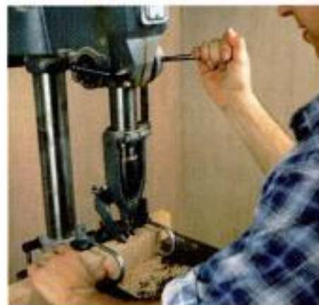
Easy mortises. A hollow-chisel mortising attachment can quickly make square-edged, flat-bottomed mortises.
