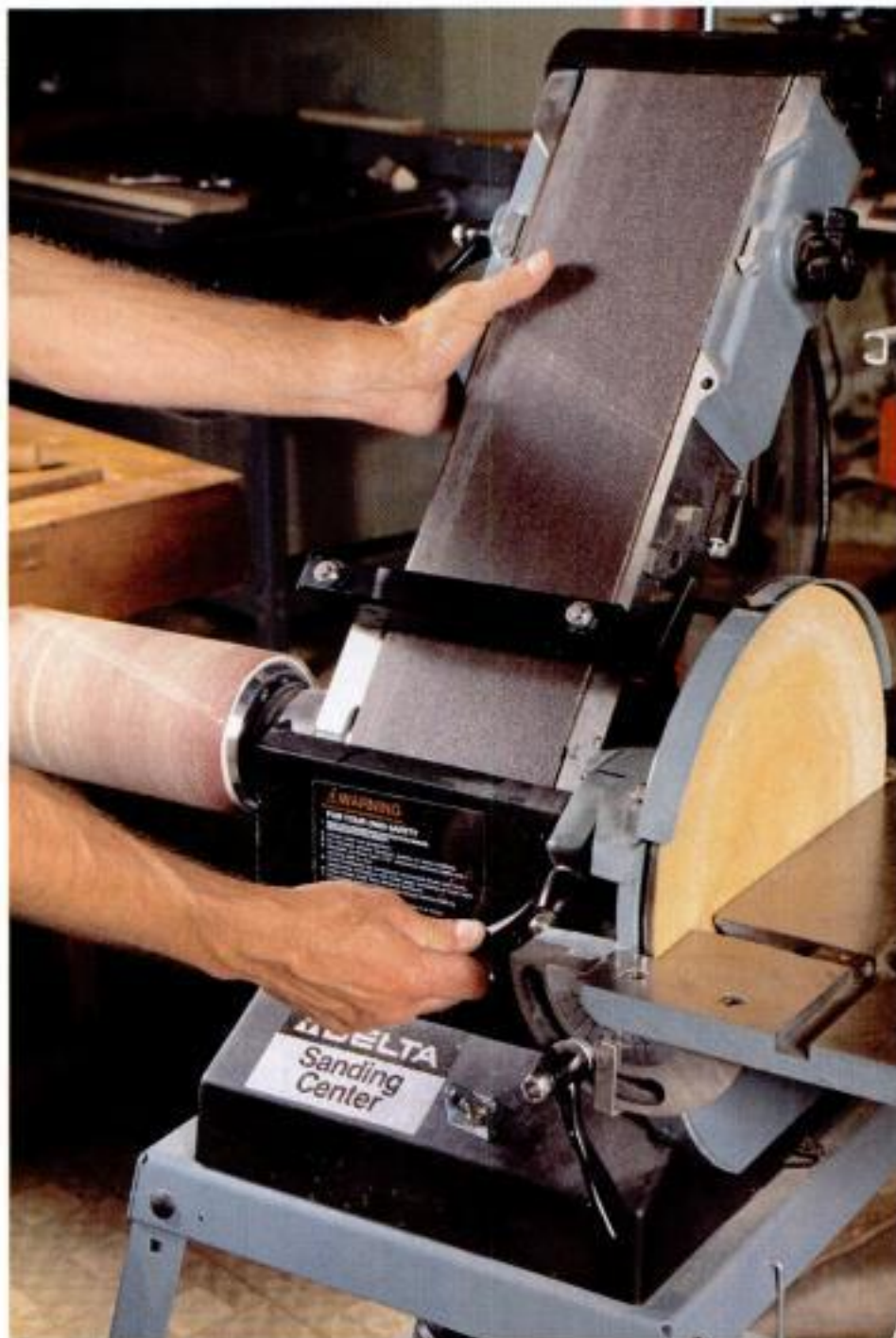
Tilting belt. Some belt-disc sanders let you adjust the belt between horizontal and vertical positions.
