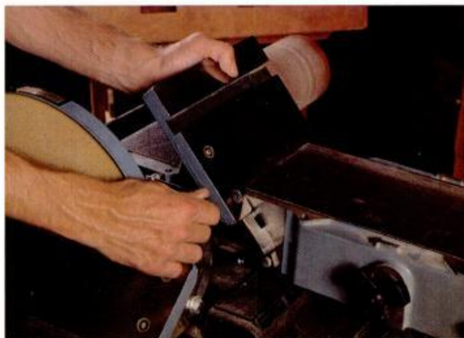
Tilting table. On a quality belt-disc sander, well-machined cast-iron tables and trunnions give solid support for sanding at a variety of different angles.
