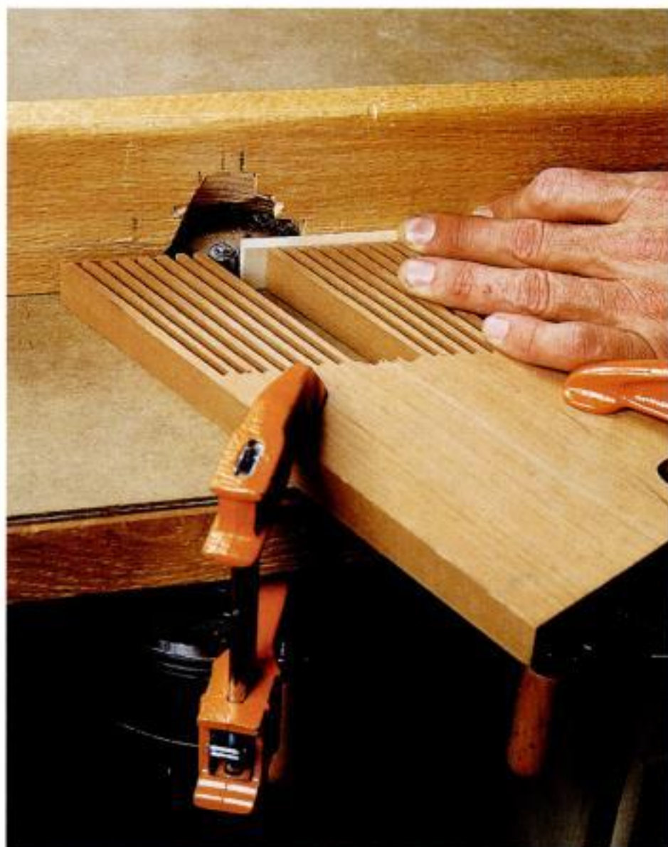
Router-table helper. This short featherboard, wide enough for two-point clamping to a table overhang, presses stock against a router-table fence.
