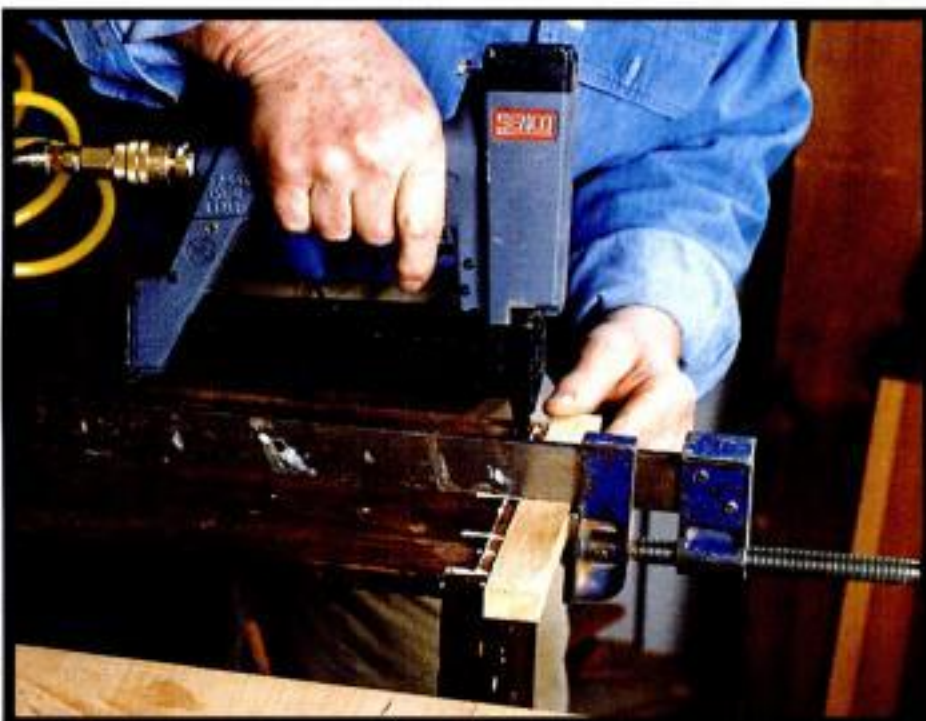
Old joint, new fastener. After regluing one of the dovetailed drawers, Kirby uses a pneumatic nailer to pin a joint fast.
