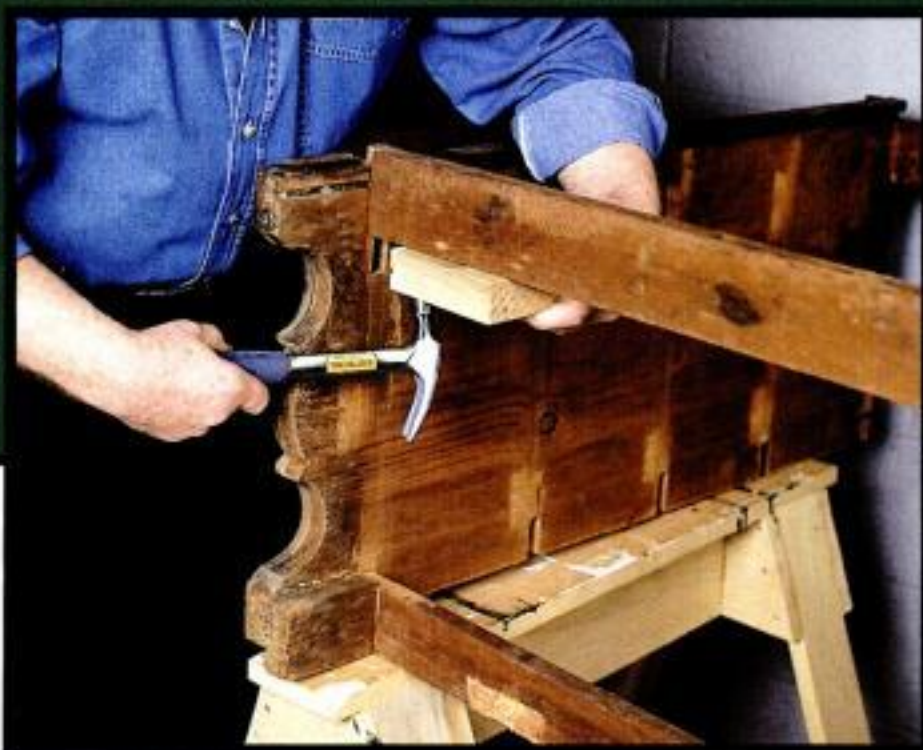
Gentle persuasion. Cushioning the blow with a block of wood, Kirby taps a rail free of a side. Though the joints were well made, the hide glue had failed.
