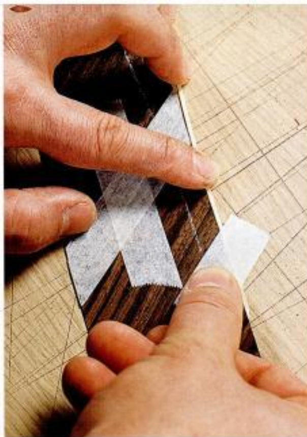
Add the banding. Attach banding to the joined border pieces with short lengths of tape.
