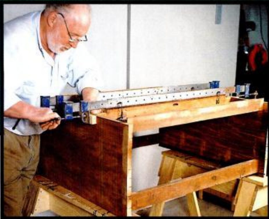
Regluing sides and rails. Kerfs cut on the inside face of each side provide enough flexibility for Kirby to flatten these parts during reassembly.
