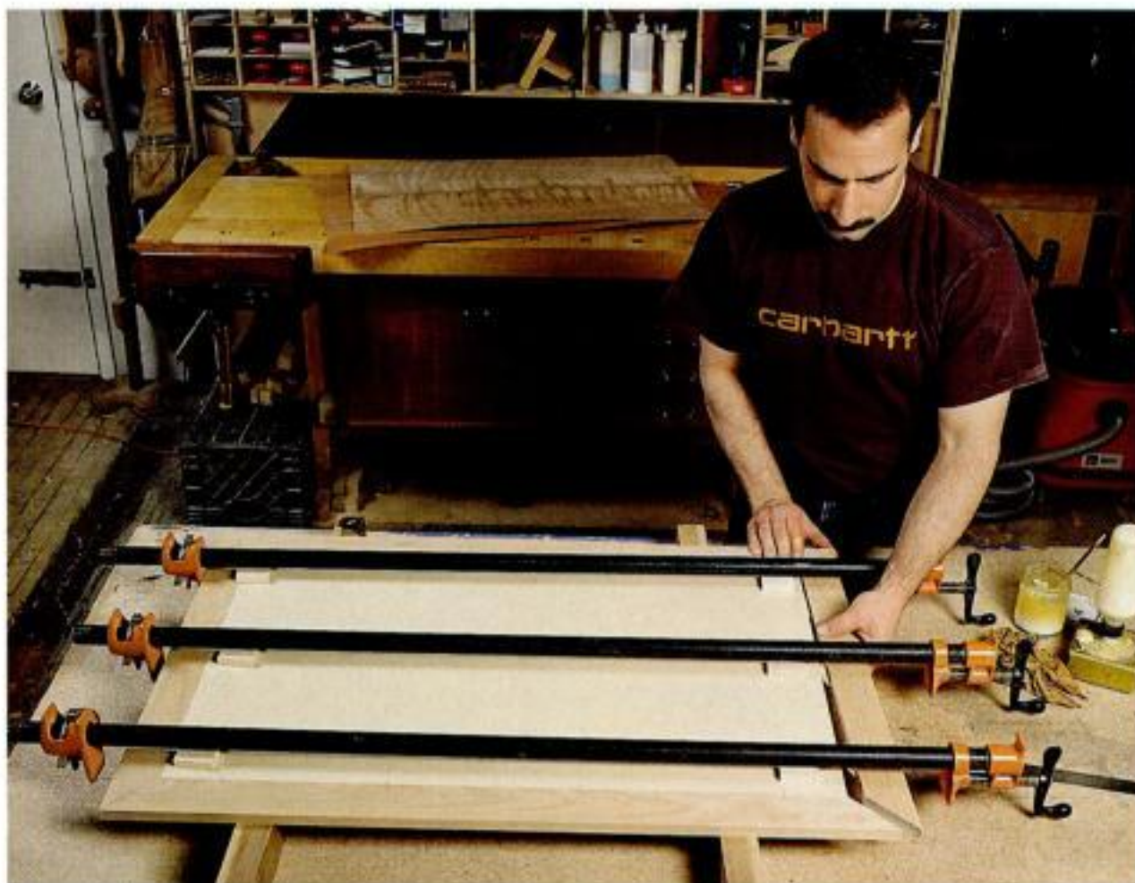
Solid wood edges. Glue and clamp mitered edging to the MDF, using biscuits for good alignment. The author glues up two opposite edging pieces first, lets them dry, then glues up the other two.
