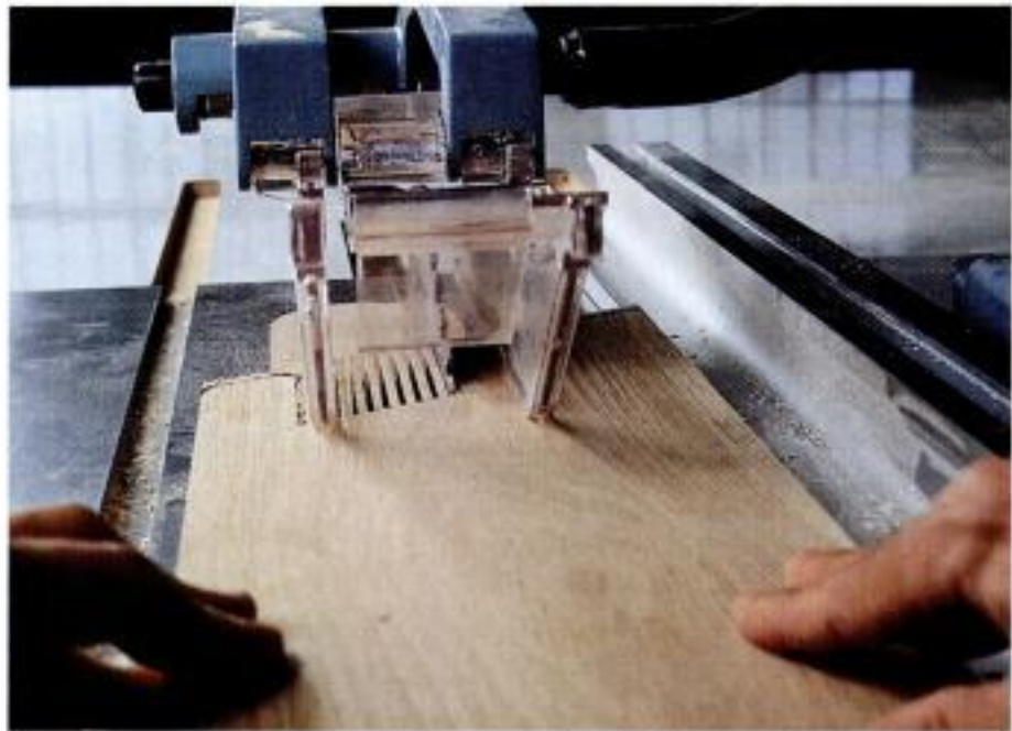
Ripping fingers. Cut the fingers from left to right, with the featherboard's acute angle against the fence and the blade raised to full height. The featherboard in this photo is shown on page 81.
