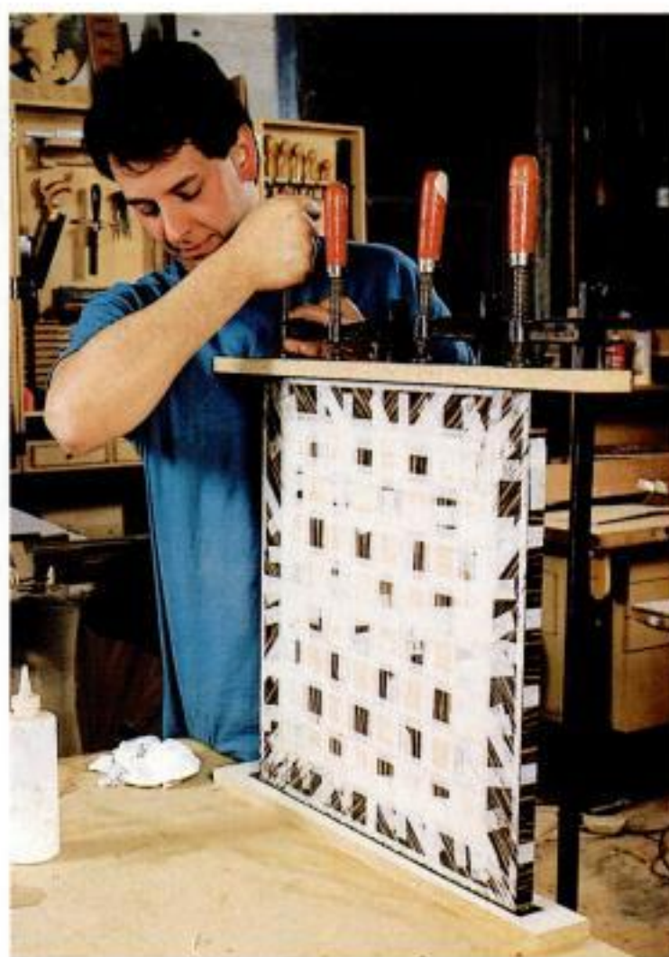
Clamp the edging veneer. Glue on the edge veneer, using tape to position it, and clamp two opposing edges at a time.
