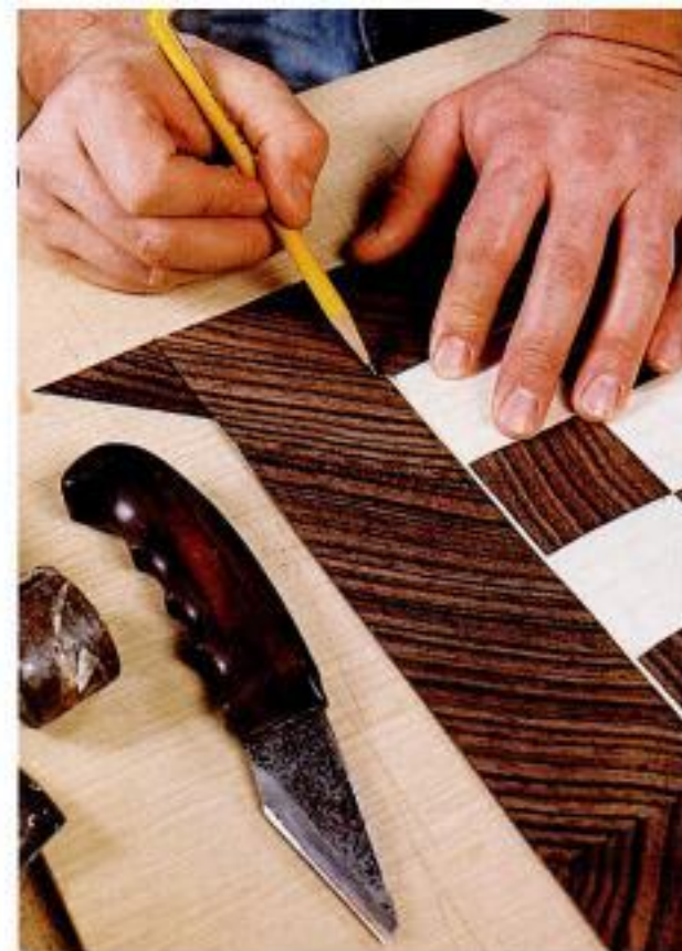
Fit the border. Miter the four border pieces where they meet at the corners of the boards.
