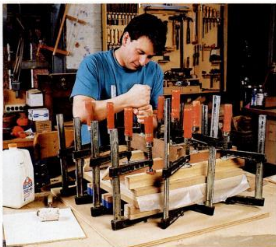
Clamp the veneer to the substrate. Clamp the glued-up assembly between MDF platens and wooden cauls, using waxed paper as a glue resist.
