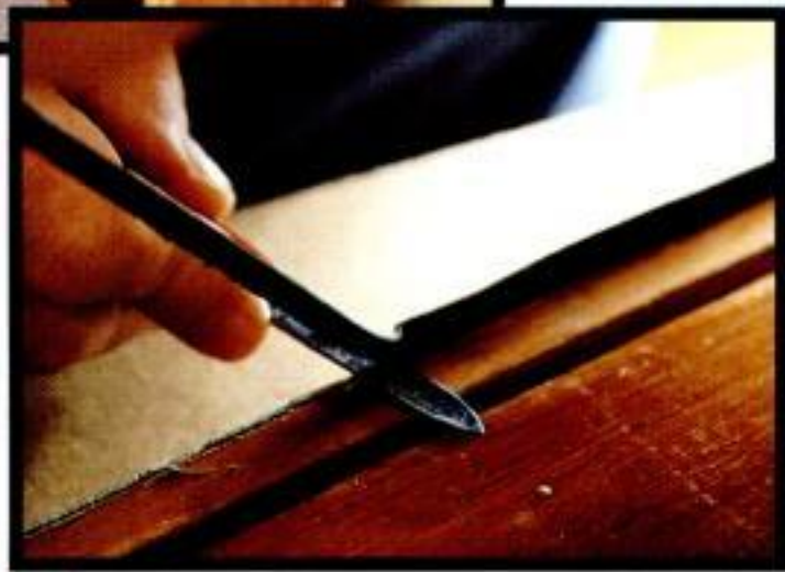
5 The knife trims it. Slice the excess leather along the edge of the wood.
