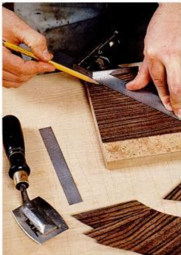
Cut the border pieces. Saw the 45° crossband border pieces from veneer stock trimmed to consistent width.
