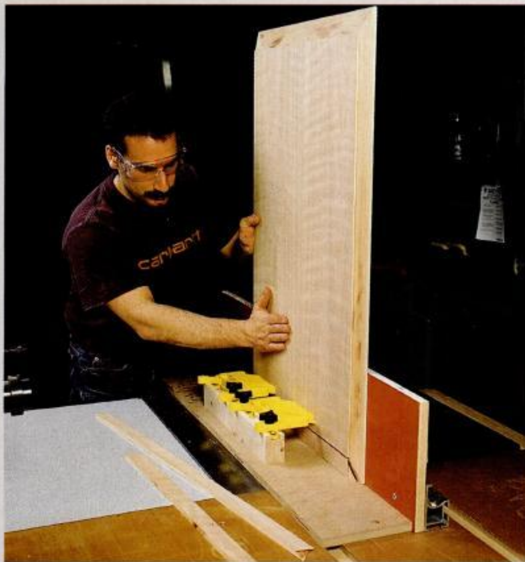
Saw the bevel. The author's jig helps hold the panel vertical while he pushes it through the angled blade. Featherboards contribute stability and safety.
