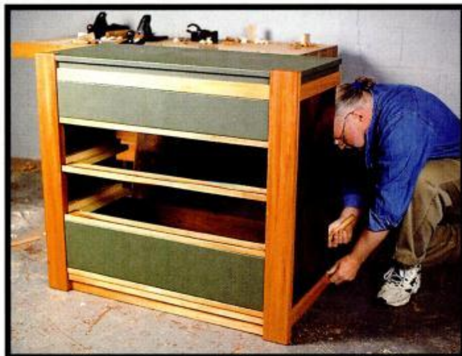
The back goes on last. Leaving the back off makes it easier to install and adjust the drawer guides for a smooth, precise fit with each drawer.
