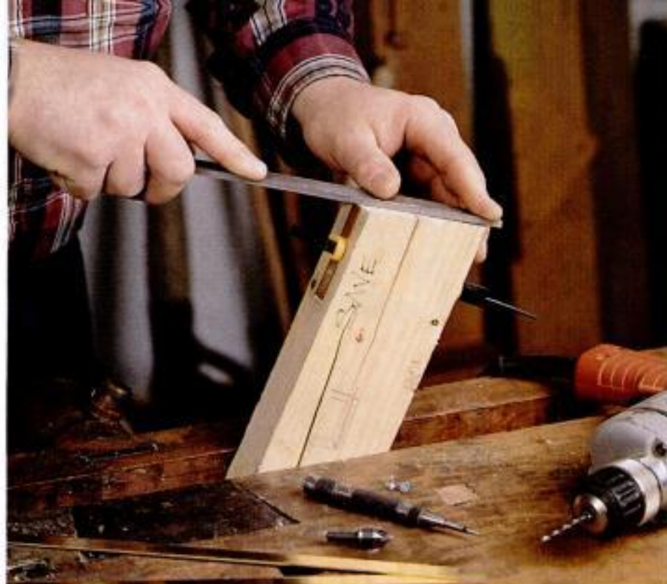
Bevel the brass. The beveled end of a 2x4 guides your file as you bevel the ends of the brass plate. A shallow mortise in the scrap holds the brass securely.
