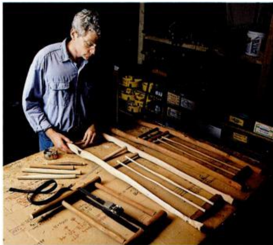
Front and back subassemblies. The back panel is glued up and ready to go. Band clamps hold the front panel in place (foreground) while the glue sets. While you're waiting, you can dry-fit the next chair.
