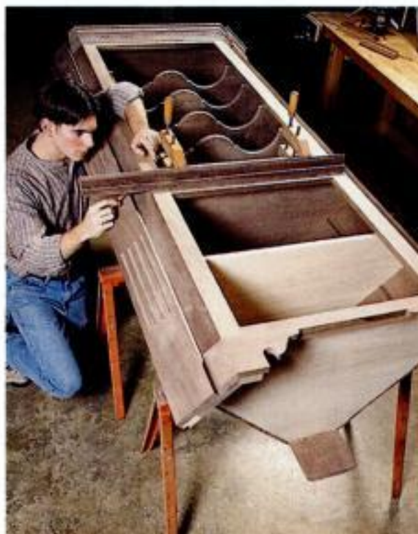
Working on the waist. Bird's assistant, Jeff Coffman, clamps a length of waist molding to the case to ensure exact marking for the miter cut.
