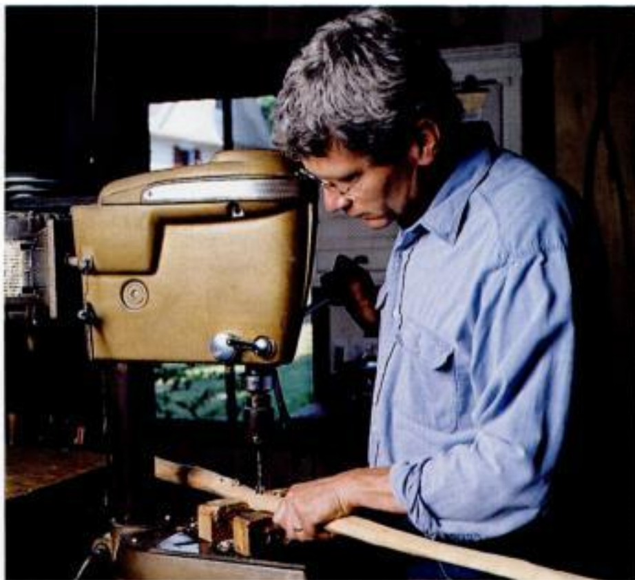
Mortising made easy. A pair of notched wooden blocks cradles the post as you drill. Hold the post steady with your free hand. For angled mortises, tilt the table or rest the blocks on a ramp.
