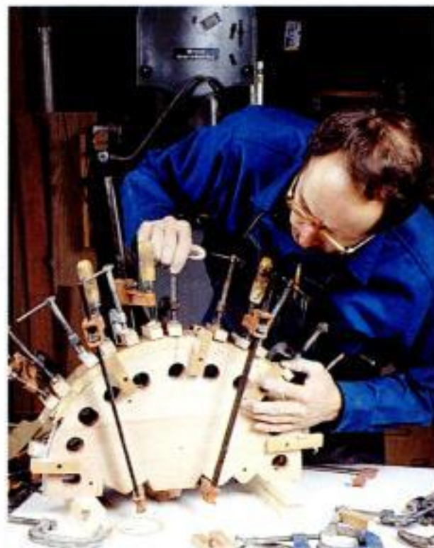
Laminating a rail. Curved rails for the panel's frame are made by gluing thin strips of wood together in a curved form. Clamps pull the laminations together against the form.
