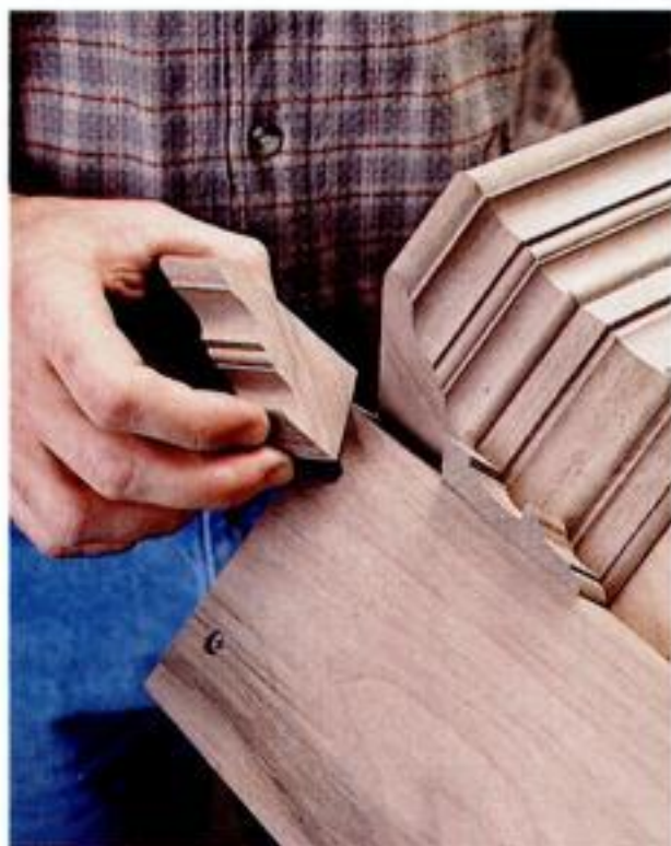
Tight joints to turn corners. Each course of molding runs horizontally, "wrapping" around pilaster and case corners with tight miters.
