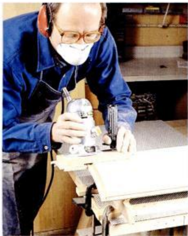
Raising the edge. The router needs a curved wooden base to follow the panel's curve. A wooden fence on the underside of the base guides the cut, which is made with a core-box bit.
