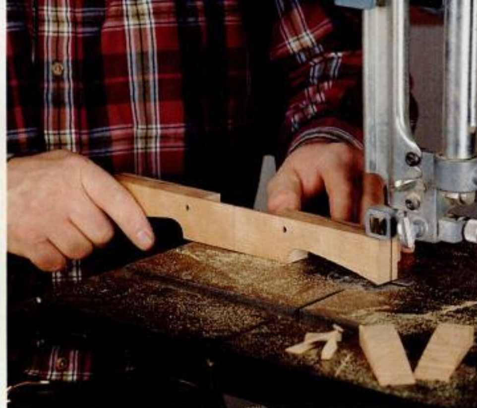
Saw out the rough shape. After roughing out the front of the shave, the author saws the bottom face on the bandsaw using a \frac{3}{16} -in. blade.
