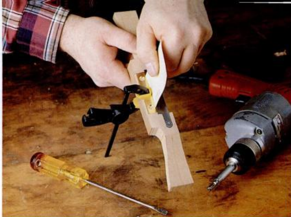
Close your mouth. Determine the correct mouth opening by holding a business card against the blade's cutting edge, then slide the brass plate up to the card.
