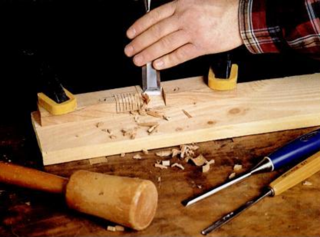
Pare the wear. Use a sharp chisel to pare away the sawn kerfs to define the throat, or wear. A small gouge takes care of the mortises for the cutter's ears.
