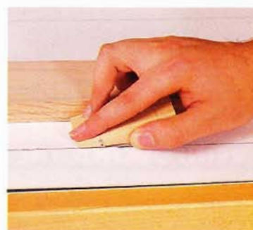
Inexpensive cutter. Sultan's simple mat cutter uses scrap-wood and a mat-cutting blade to cut the bevel in the mat.
