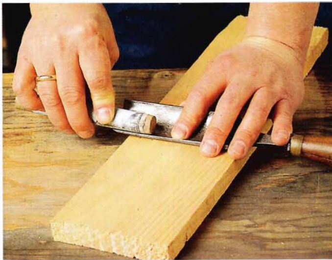
Inside curves are easy, too. Wrap sandpaper around a dowel to smooth and polish the inside face of a gouge.
