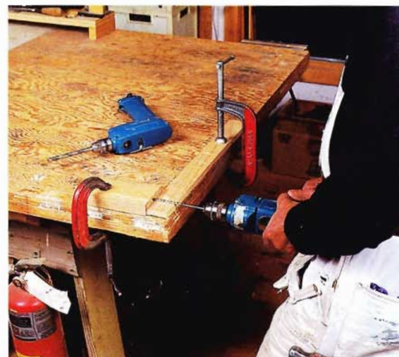
Drill it straight. McArthur uses a wide scrap board to keep his drill bit parallel to the stock as he drills the deep hole in the front post.
