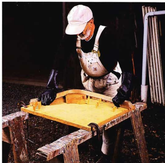
Steam and bend. Gloved for protection, the author pulls out a hot seat slat from the steam box (left). Working quickly, he bends the hot piece between dowels and wood blocks in his bending jig (right).
