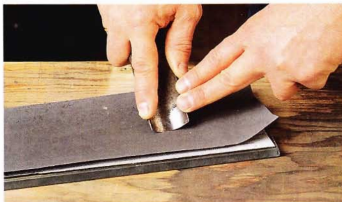
The gouge bezel. A side-to-side motion works for honing the bezel on the outside curve of the gouge. Turn the blade to sharpen the curved surface evenly.
