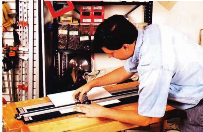
Cutting system. A mat-cutting system holds the mat firmly while you slice a beveled opening with a mat cutter. Prices start at around $50.
