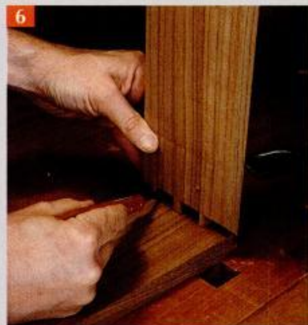
Use the pins to lay out the tails. Scribe your tail lines by holding the adjacent pins carefully against the baseline.
