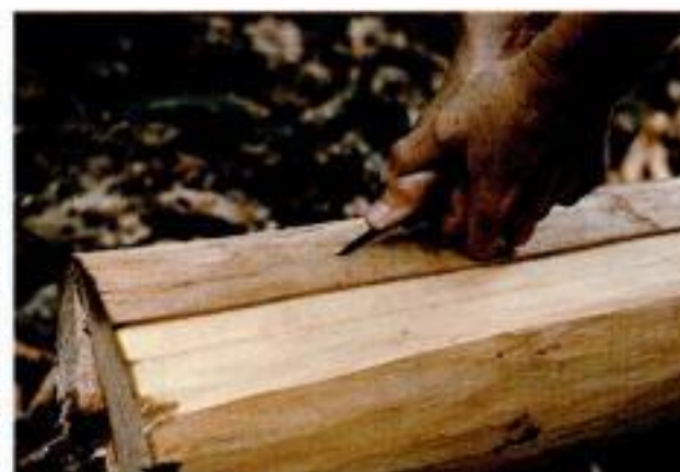
Slice the inner bark. Score the inner bark into \frac{3}{4} - to 1-in.-wide strips that run down the length of the log.
