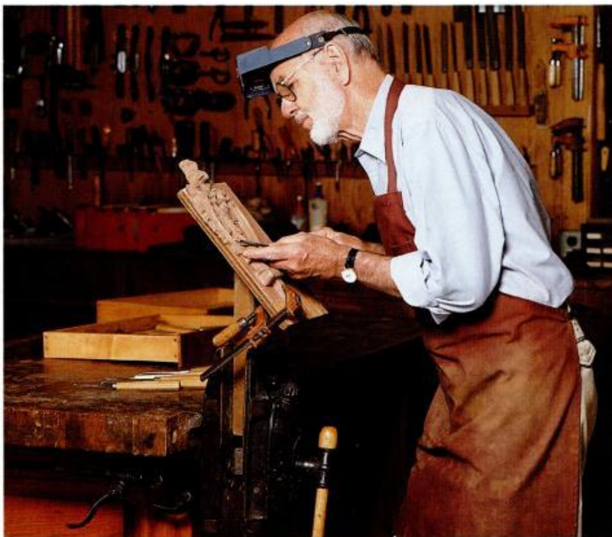
Versatile vise. To hold delicate work at a comfortable height, Whitley orients vise jaws vertically and grips an abrasive-backed work board.
