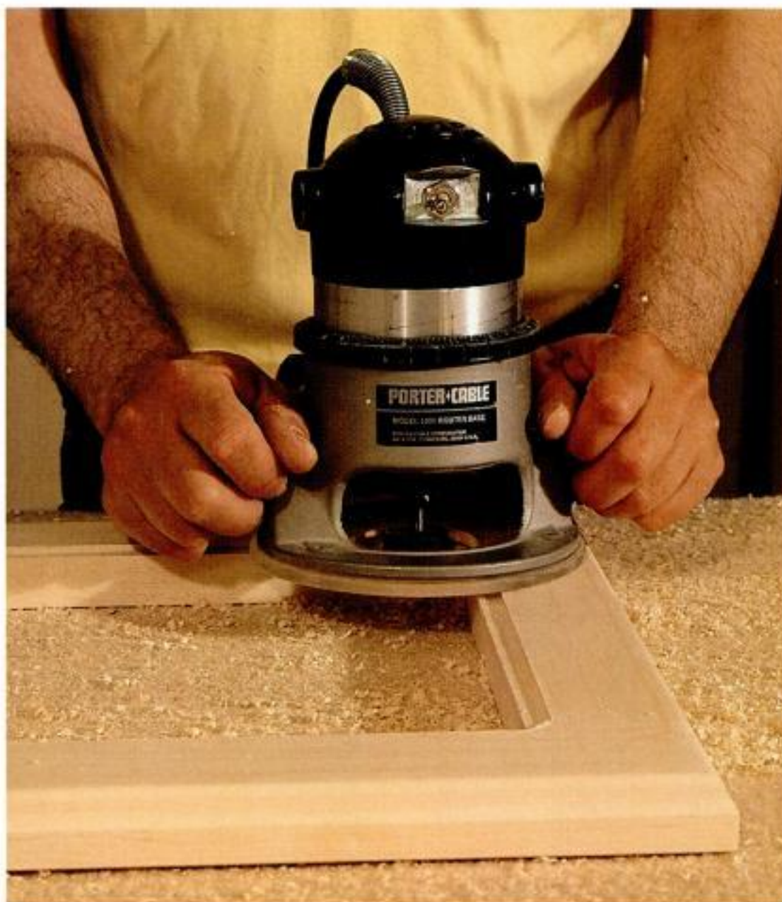
Rabbeting the frame. Once the frame is together, it's quick work to rabbet the frame's inner edges. Then chisel the four corners of the rabbet square.
