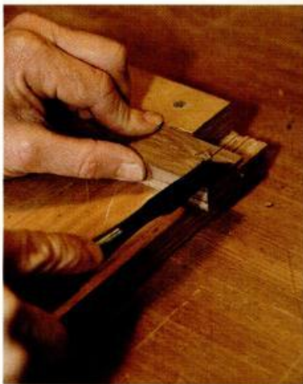
Groove along the tenon shoulder. A shallow groove pared along the tenon's shoulder line will help keep your saw square.
