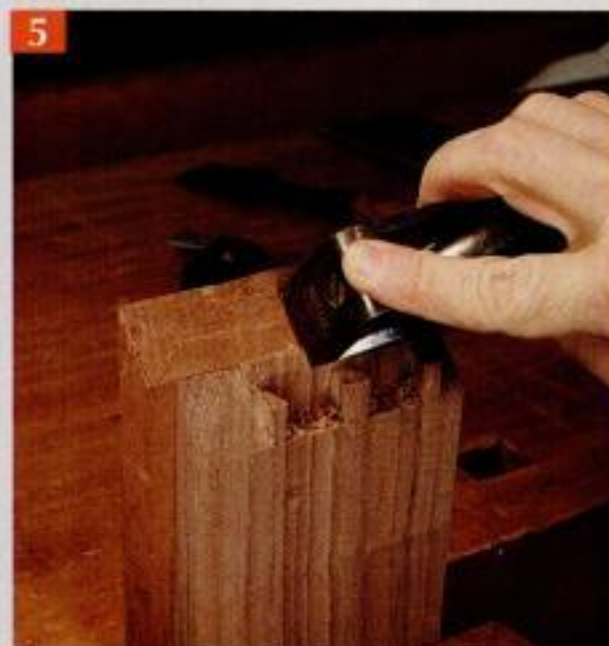
Miter the middle. Another template guides the rabbet plane as you miter the length of the rabbet lap. This removes stray saw marks on the lap.
