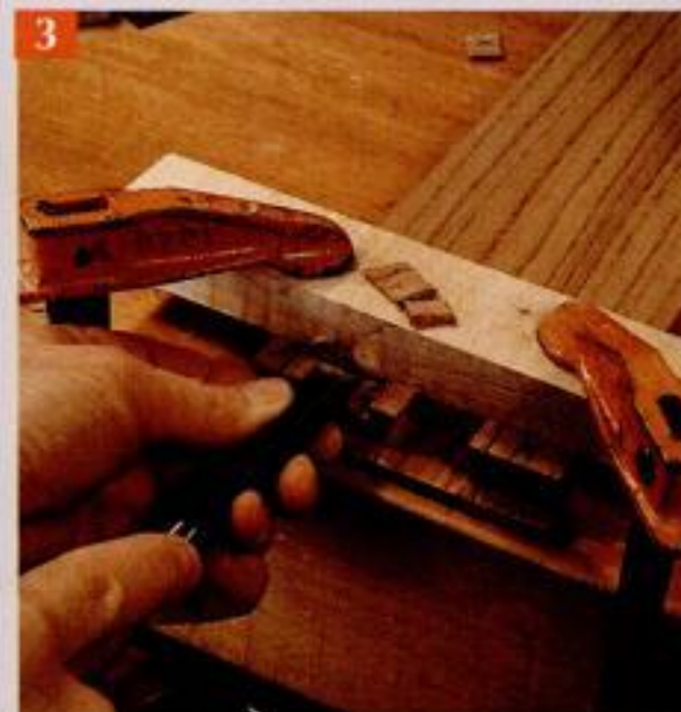
3 Pare to the rabbet lap. Carefully pare down to the thickness of the rabbet lap. The clamped-down board supports the chisel on downward cuts.
