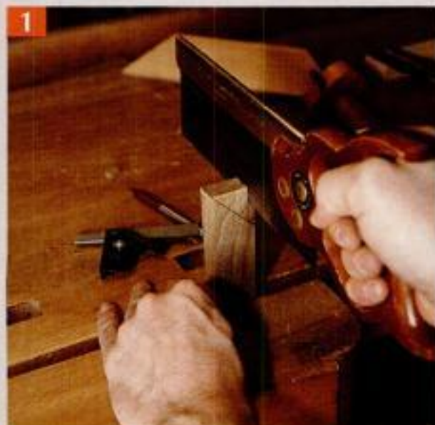
Saw the bulk. Use a handsaw to trim away most of the excess molding on the end of the mortised stock. A diagonal line will help you miter the molding accurately.
