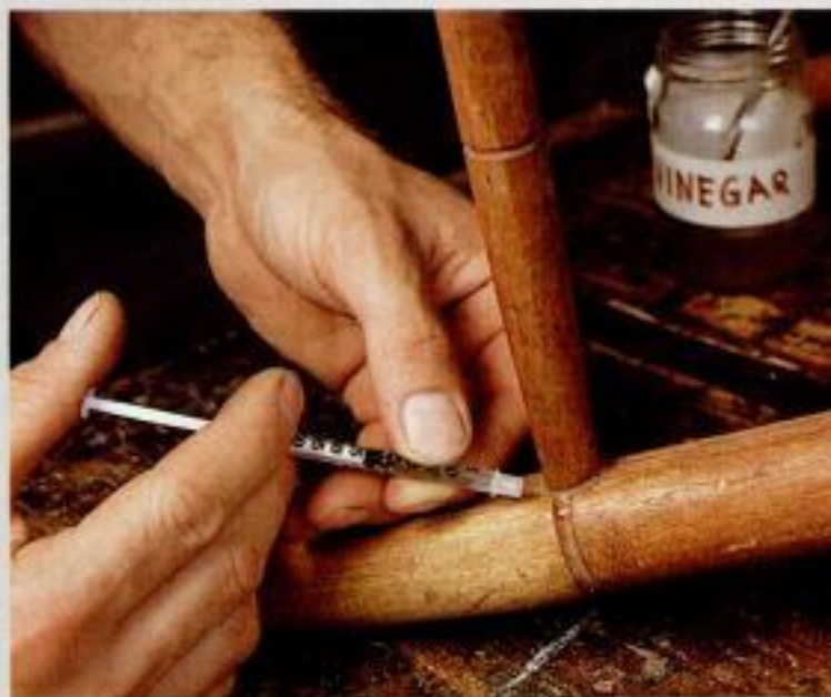
Loosen up. To undo an old hide-glue joint, inject warm water into the crevice. In five to 10 minutes, pull it apart. If water doesn't work, try vinegar—it's more aggressive.
