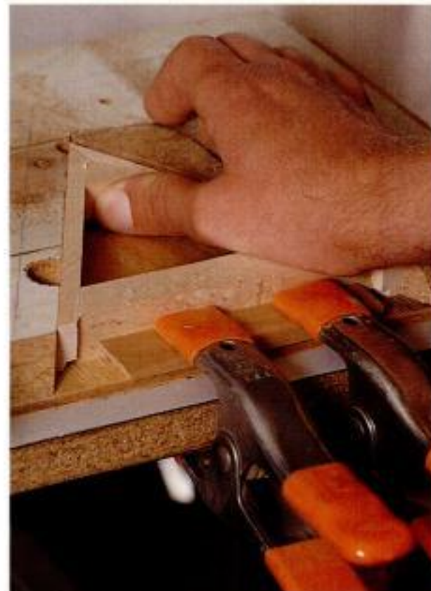
Rod support. Glue a rod-support wedge into each back corner. Hold it with your thumb for about 10 seconds.
