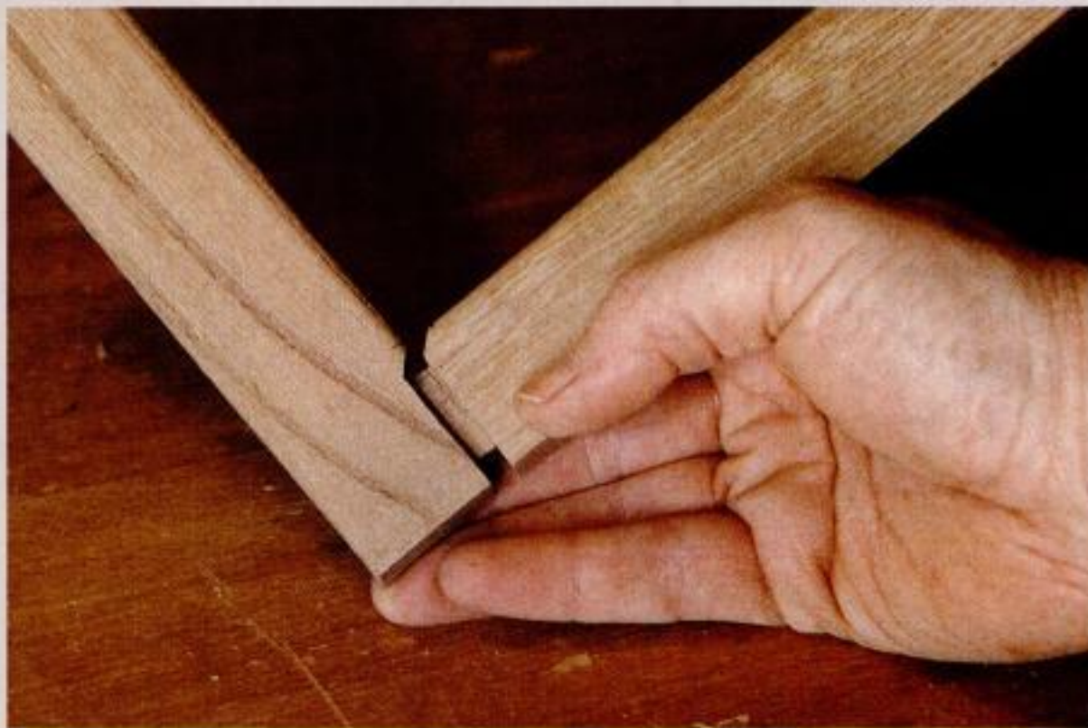
A perfect fit. Mitering the integral, or "stuck," molding on adjoining stiles and rails is a traditional doormaking technique.
