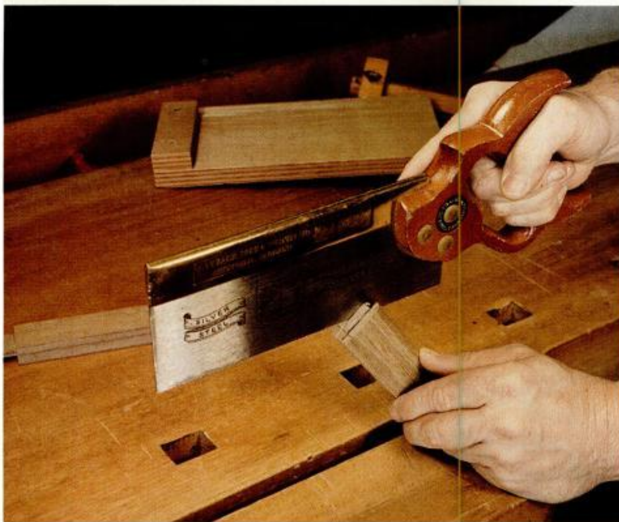
Saw the tenon cheek. Make the first cut with the work pointing away from you. Then flip the work so it points toward you. Complete the cheek cut with the work clamped vertically.
