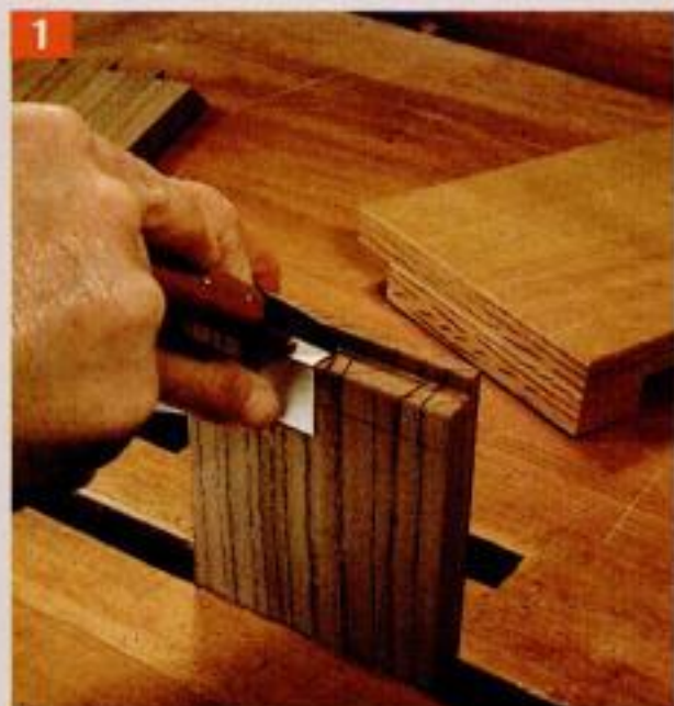
1 Lay out the pins. Make a stiff paper template to lay out the pins first. Note the lap left behind the pins—evidence of the rabbet cut before joint layout.
