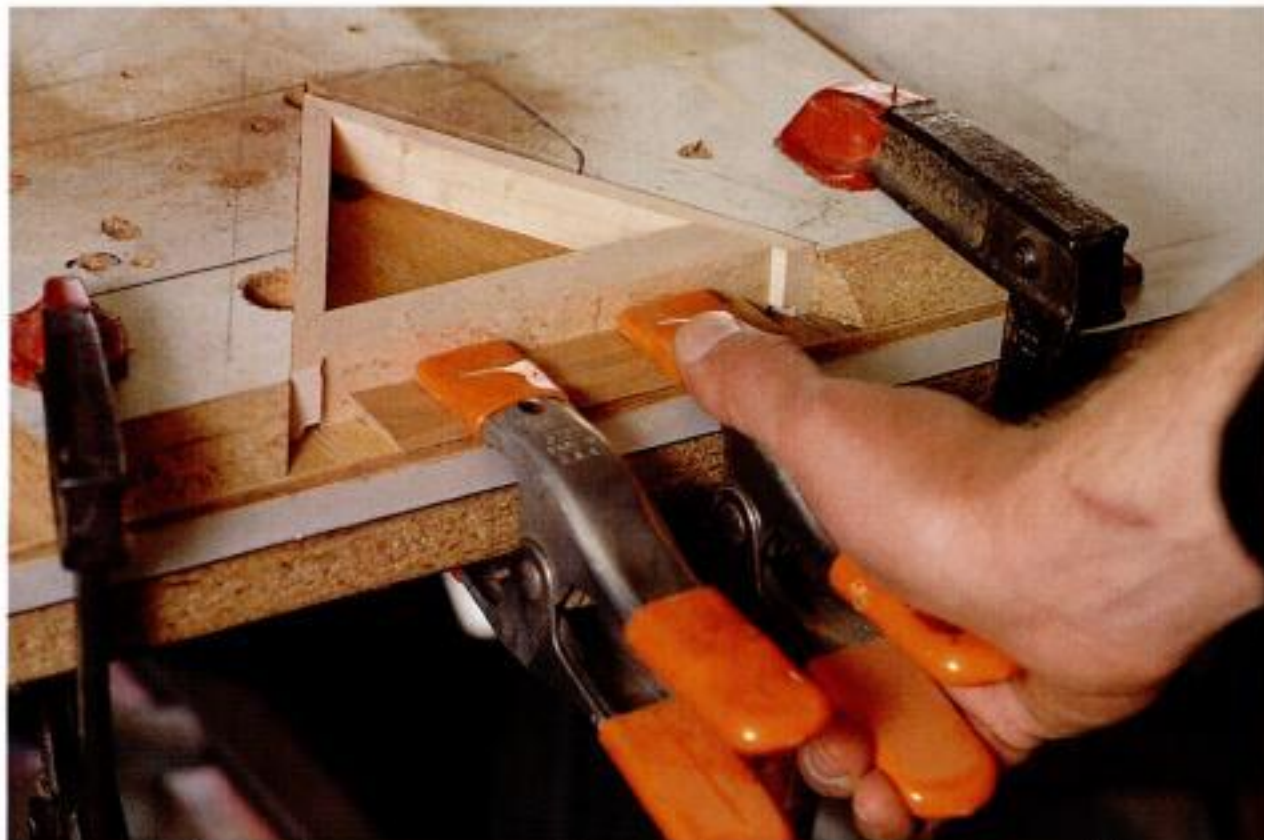
Tray assembly. Glue each tray's sides together using a simple assembly jig. Two spring clamps hold the front tightly against the sides. The thin sides can run long; you'll trim them to final length later.
