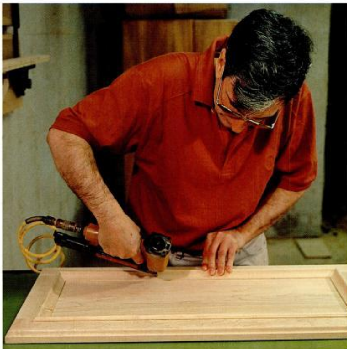
Trapping the panel. Four pieces of mitered molding fit over the panel and cover the rabbet in the door frame. The door is done.
