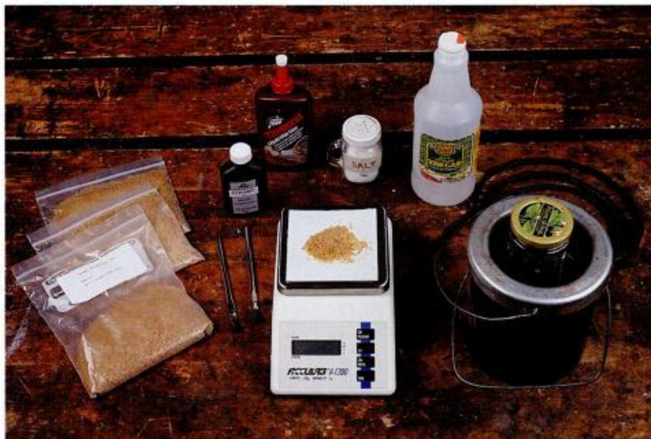
Important ingredients. Shown clockwise from left: hide-glue granules, glycerin, premixed liquid hide glue, table salt, distilled white vinegar, glue pot and lidded glass jar, metric scale, and brushes.
