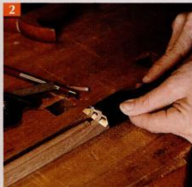
Pare the rest. Clamp the mortised stock in your bench vise, keeping the molding depth line flush with the benchtop. Then pare to the line with a chisel.
