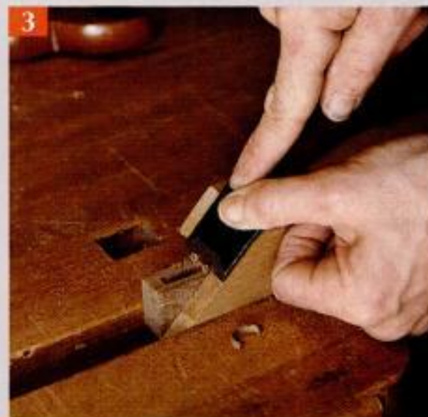
Miter the molding. Clamp each frame member—mortised or tenoned—to the wraparound mitering template you used on the case joints. Pare the molding flush to the template.
