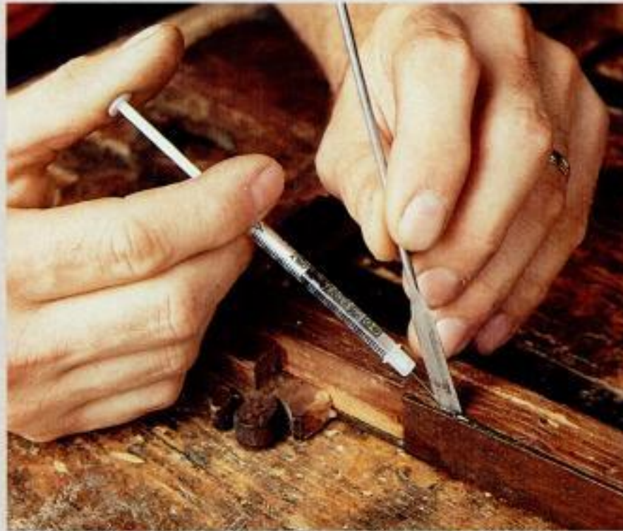
Handle with care. To fix delicate veneer without disturbing the finish, inject warm water or dab on some fresh hide glue.
