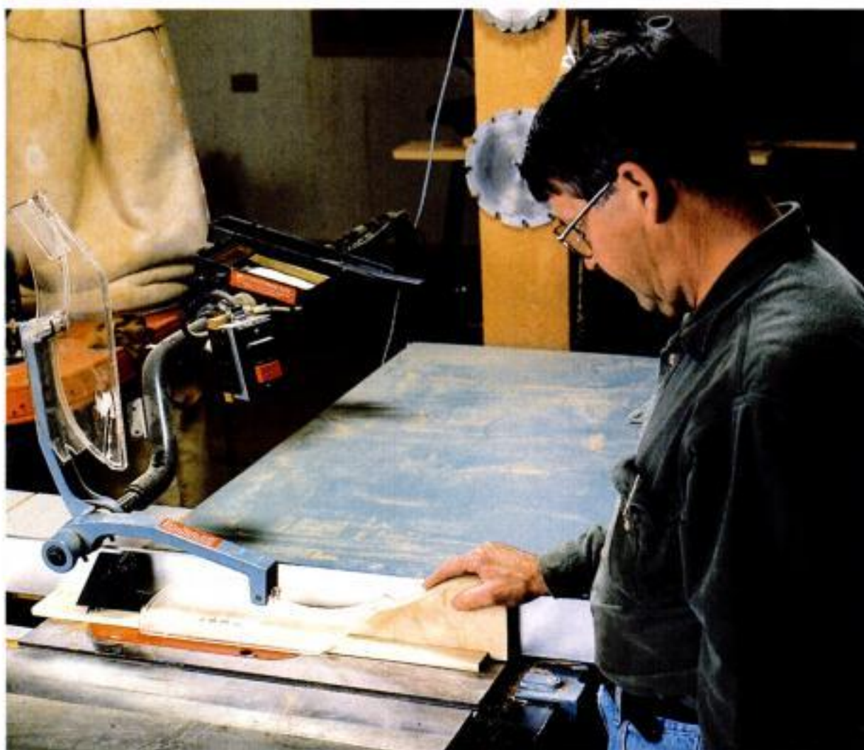
Convenience and security. The blade cover on Conover's Uniguard is suspended from a C-shaped support arm. Two halves of the guard can swing up independently—an advantage when ripping narrow boards.
