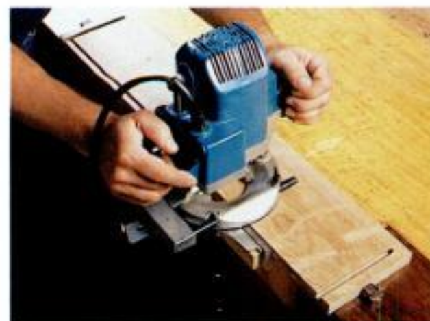
Rout the groove. A straight bit and an edge guide let you safely make the stopped groove in the drawer front.
