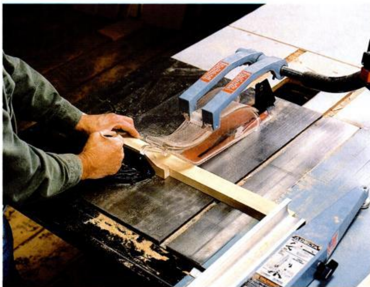
A clear line of sight. Clear, high-strength plastic provides both protection and a good view of the blade. The splitter is attached to the table, independent of the blade guard.
