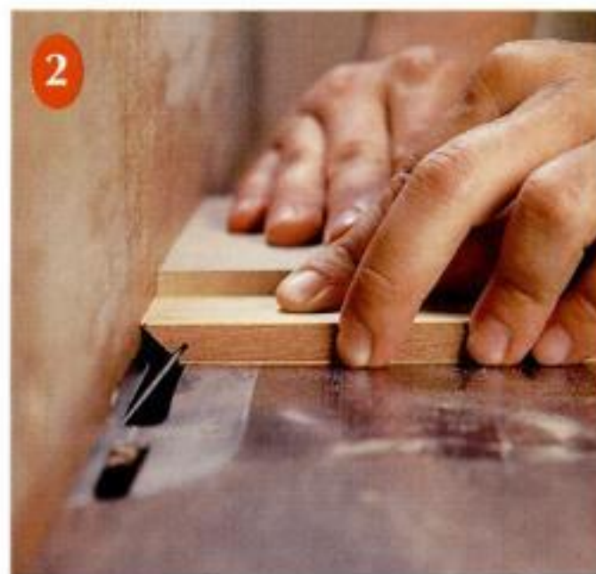
Cut kerfs for spline slots. The rip fence and a square MDF backer block guide the workpiece as Pollaro cuts spline slots in the mitered sides and ends.
