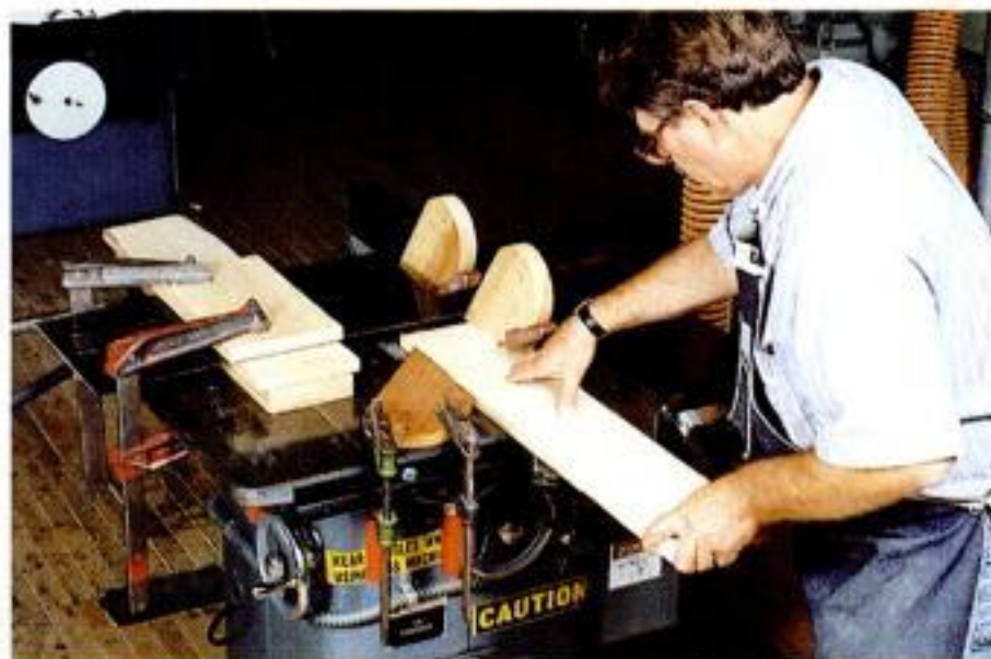
Grooving. A scrap of Plexiglas clamped to a pile of scrap boards covers the dado blade. Pressure from featherboards lets you feed without getting near the blade.
