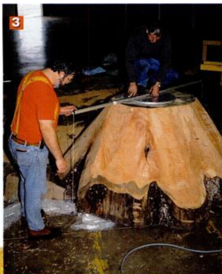
3 Finding center. Mortimer and AW contributing editor Steve Blenk find the center for attaching the faceplate by pivoting a weighted string around the outside of the blank.
