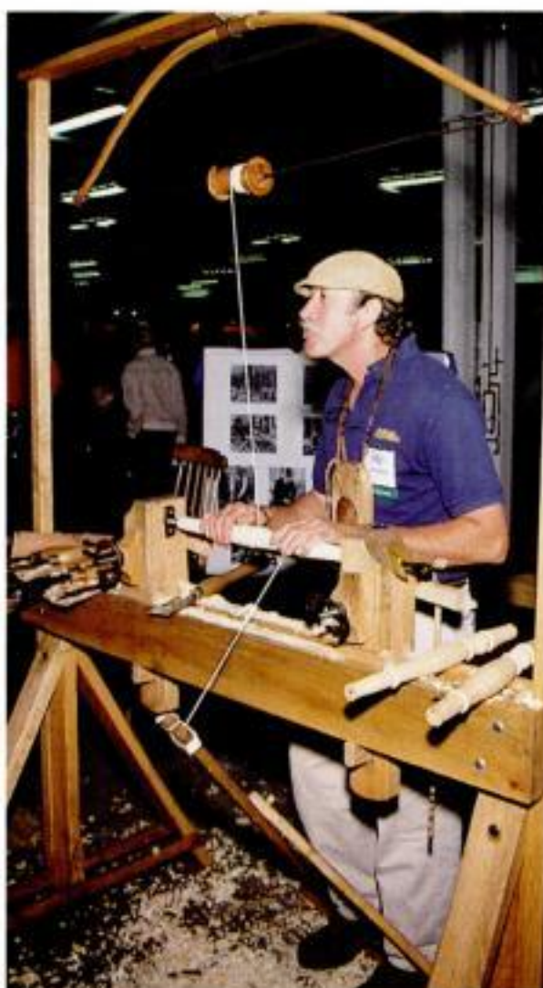
Weber on bodging. Don Weber shows how he makes chair spindles on his pole lathe.
