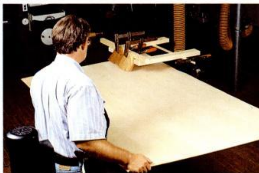
Safe and stable. Maas uses an outrigger for one-man cutting of sheet goods. The fixture not only guards the blade, it holds plywood sheets down on the table.
