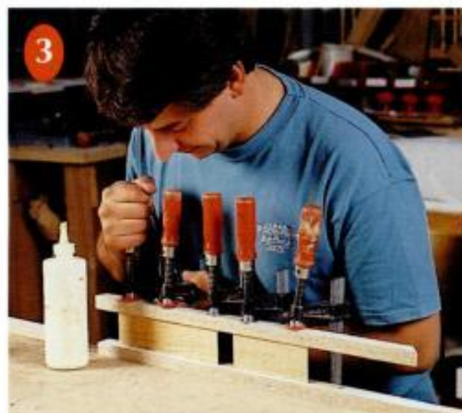
Veneer the edges. Strips of melamine-coated particleboard make good clamping cauls for veneering the edges of side and end pieces.
