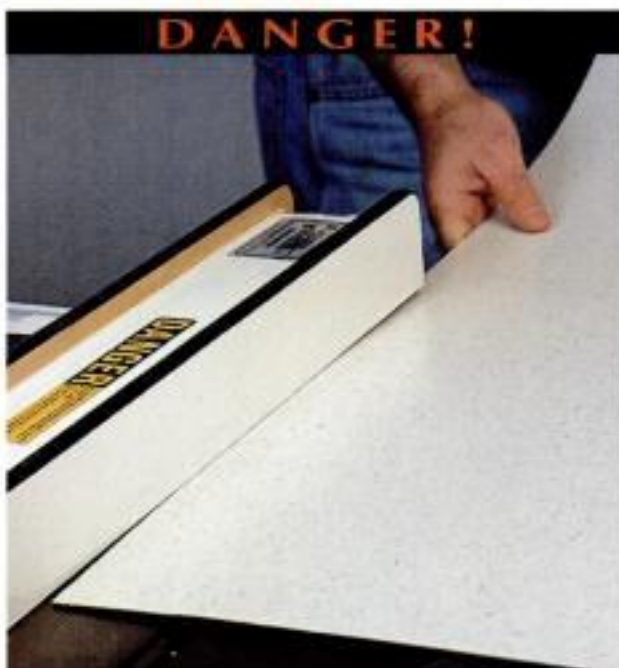
A thin plastic laminate sheet can sneak under the rip fence. It can easily bump the side of the blade and shatter.
