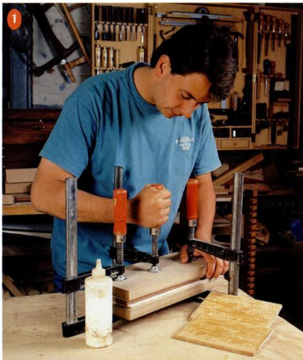
Veneer the core pieces. Pollaro veneers a single mahogany core piece from which the box sides and ends will be cut. This takes less time than veneering parts individually. The outer cauls are 1 1/4-in.-thick MDF. The inner cauls are 1/4-in.-thick, melamine-coated particleboard.
