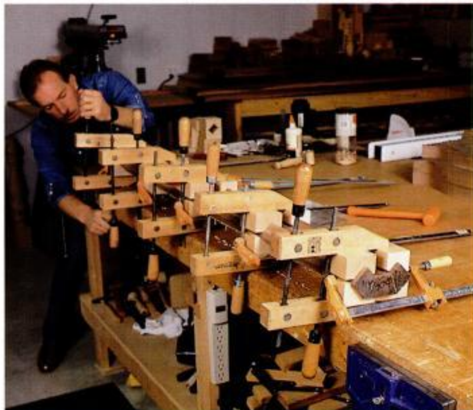
Clamping to a rough curve. Pull each of the three sections of rail together using sets of four clamping blocks, spacing each set about a foot apart.
