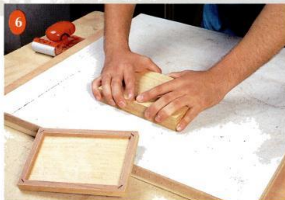
Sand the top and bottom flat. Sheets of sandpaper glued to an MDF base provide a flat abrasive surface. To flatten the mating edges of the top and bottom, apply even downward pressure and move each piece in a figure-eight pattern.
