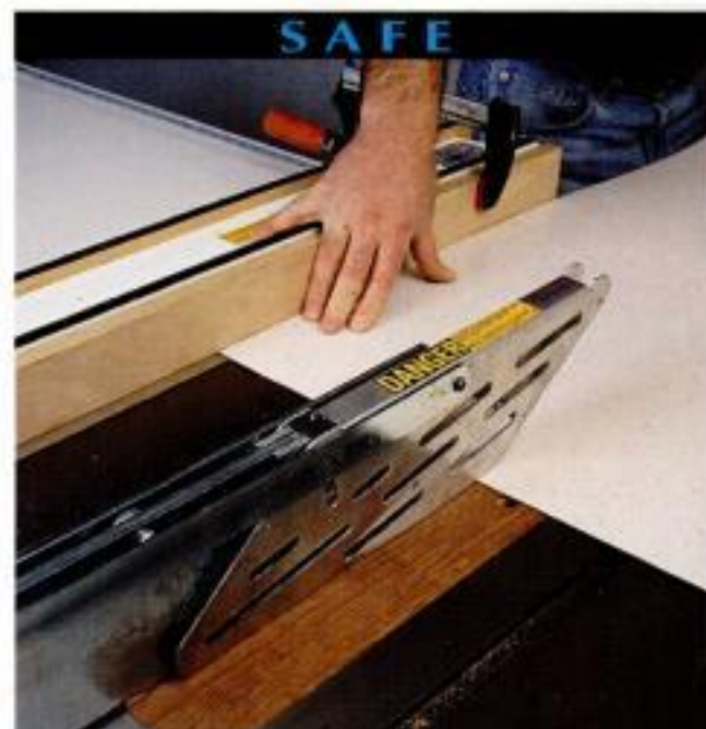
An auxiliary fence closes the gap and prevents laminate sheets from sneaking under the fence.
