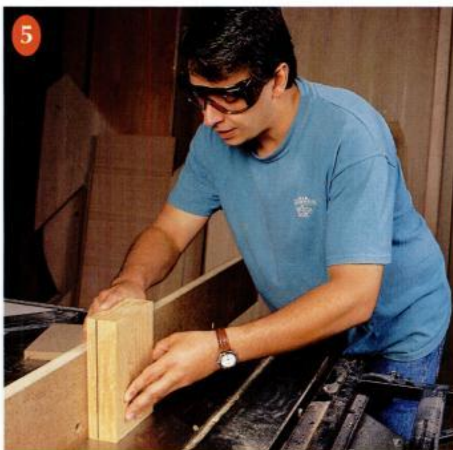
Cut the box apart. A high, flat auxiliary fence promotes control when separating the box top and bottom. Pollaro sets the blade \frac{1}{16} in. higher than box side thickness.
