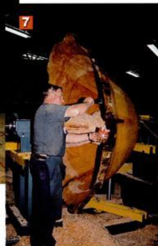
7 Big finish. Mortimer brushes on several gallons of Danish oil to slow down the drying of the green bowl and prevent cracking.
