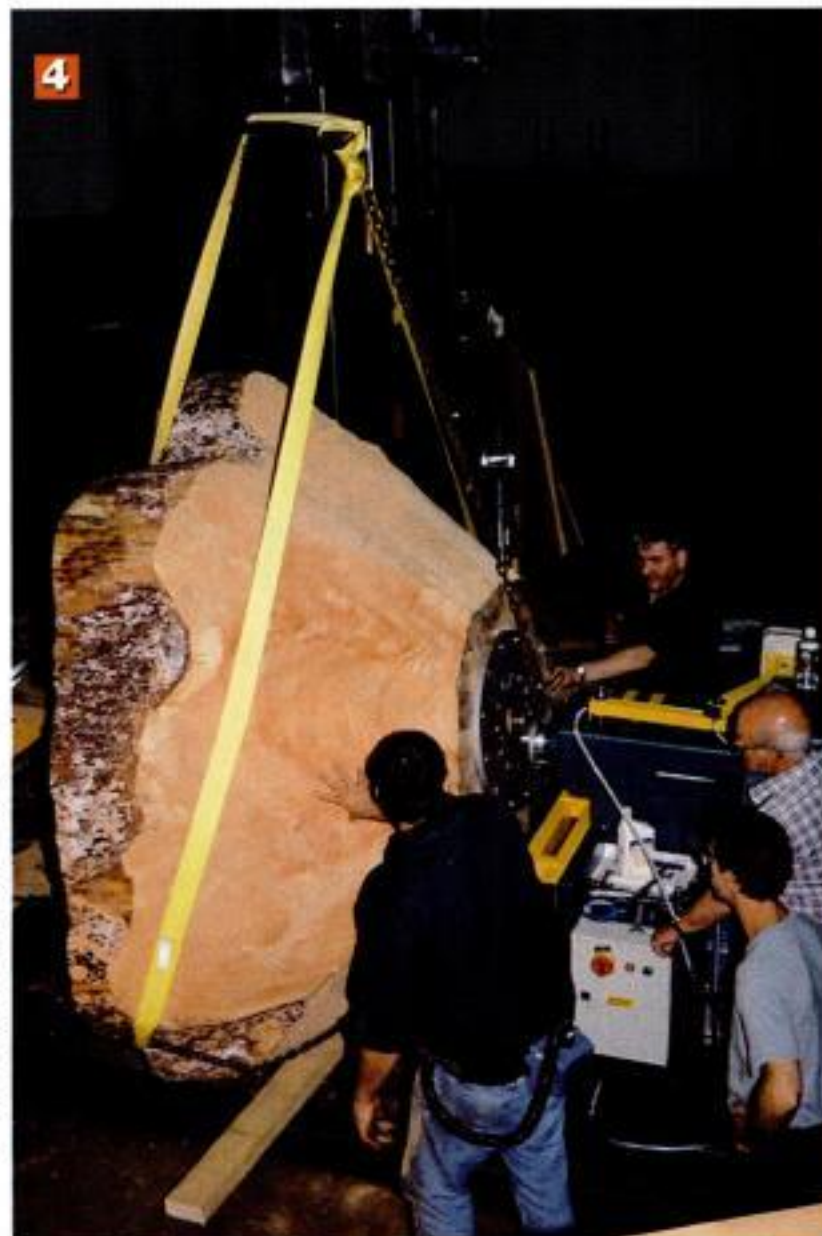
4 Mounting on the lathe. Chains, heavy strapping, and a forklift hoist the big blank onto the headstock. A unique pivoting chuck on the tailstock allows for slight imbalances as the blank spins.
