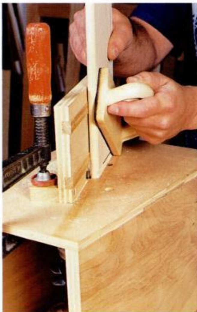
Tails on the router table. With the same dovetail bit used in the jig, rout the full dovetail on each drawer side. Hold the stock vertically against the fence and make one pass on each side of the stock.
