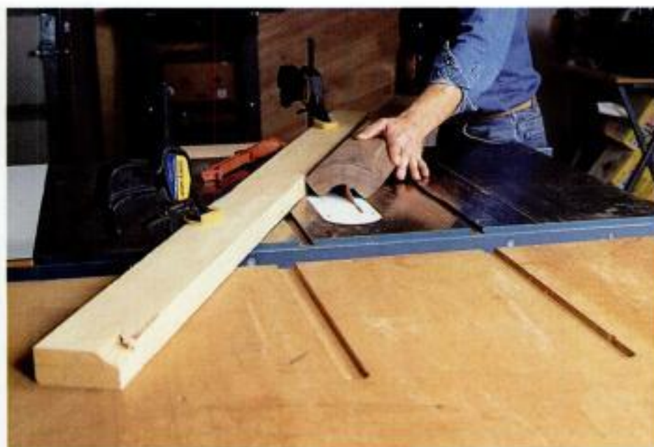
Coving the rail. Cut the curve in the underside of the rail by feeding the work at an angle to the saw blade. A straight-edge clamped to the saw table safely guides the work.
