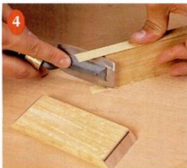
Trim the veneer. A sharp veneer saw is all you need to trim excess veneer from sides and ends.
