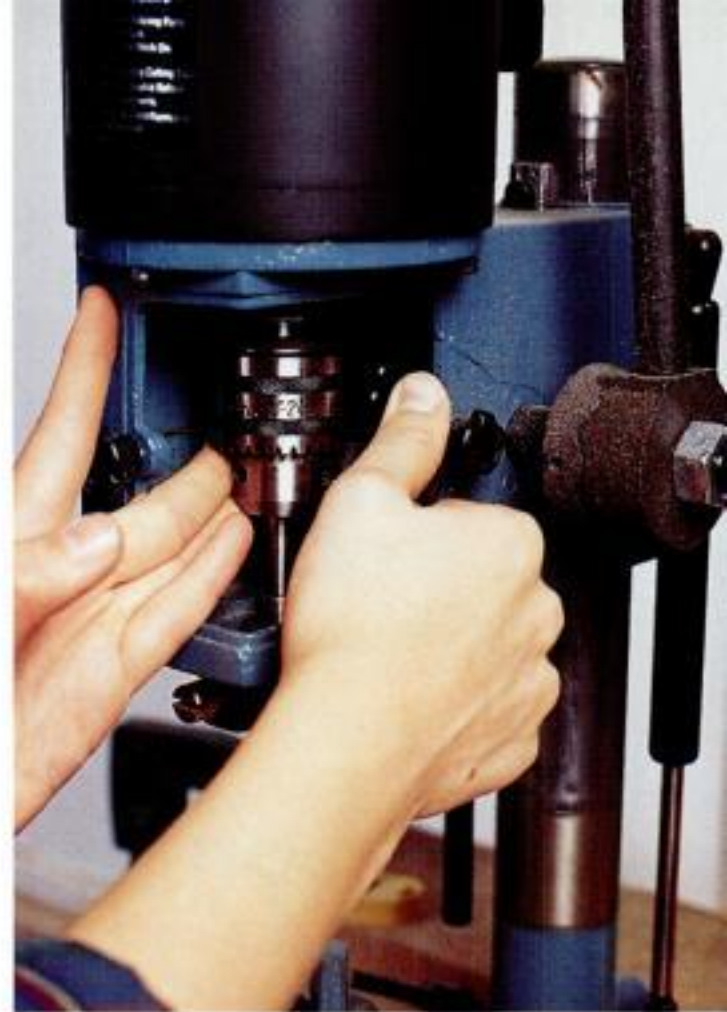
Cramped bit access. It's hard to hold the chuck still on the Bridgewood, Grizzly, Star, and Woodtek machines.
