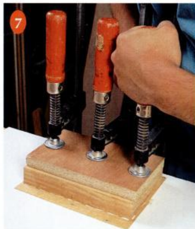
Final veneering. Cover the exposed core edges of the top and bottom assemblies with a single sheet of veneer. After the glue dries, flush-trim the veneer and file the inside corners square.
