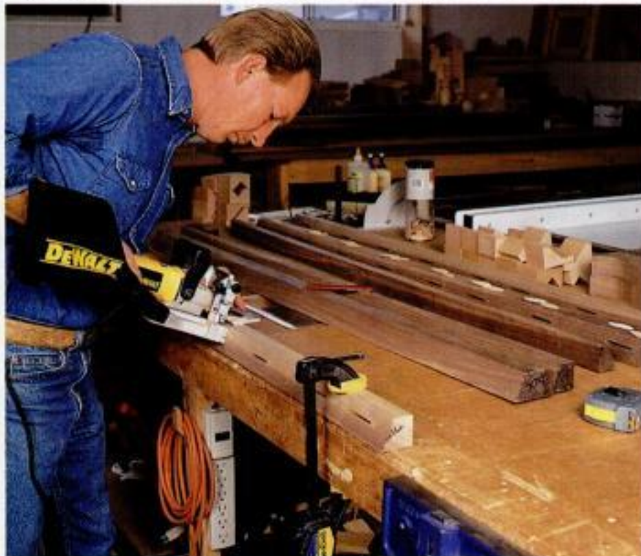
Cutting slots for biscuits. Slot the beveled rails with a biscuit joiner, setting the joiner's fence to 22\frac{1}{2}^\circ and centering the slots in the stock's thickness.
