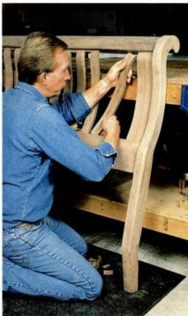
Installing the slats. Slip each slat into place by angling it between the grooves in the rails. Blocks between the slats keep the spacing correct.
