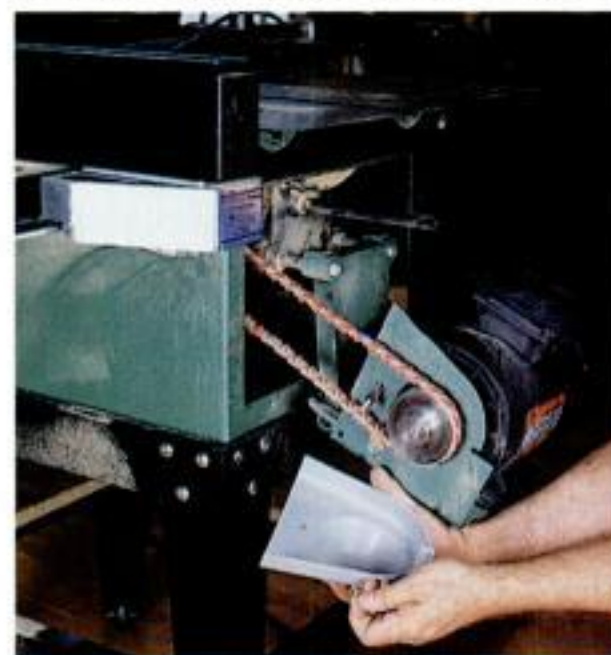
Smooth power transmission. On the Grizzly saw, machined pulleys and a link-belt drive get the spin from motor to blade with minimal vibration.
