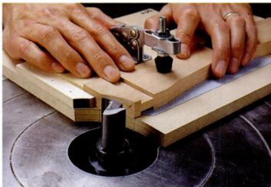
Rout the two end curves. Use another template jig to rout the finished end curves, flipping the workpiece end-for-end between cuts.
