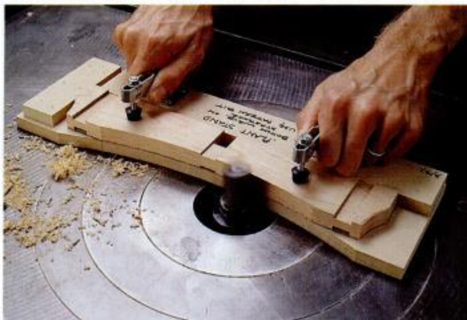
Template-route the bottom curve. After bandsawing the stretchers to rough shape, use a template jig to rout the long curve.
