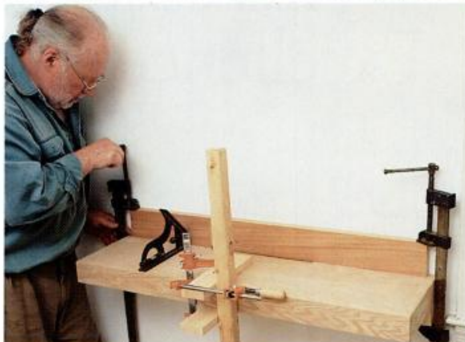
Gluing the shelf. Use a pair of long clamping cauls to clamp the pocket tightly against the top and bottom edges of the ledger.
