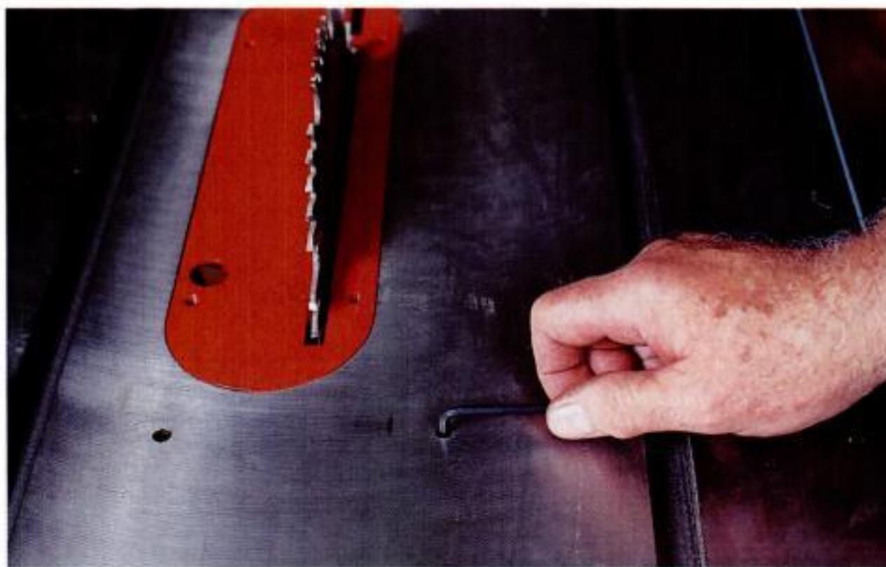
Bevel stops in tabletops. On the Craftsman saw and both Delta saws, a pair of setscrews in the tabletop lets you set stops for 45° and 90° blade settings without reaching under the table.
