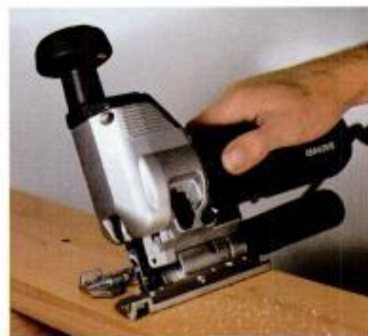
Cut at full tilt. Adjustable-angle baseplates allow you to cut angles up to 45°.
