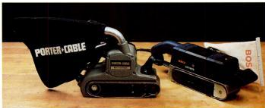
Bag the dust. Front- or rear-mounted bags are generally less obtrusive than side-mounted bags.
