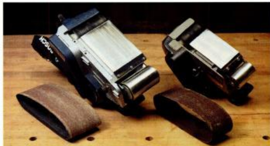
Sanding surface. Larger platens put more of the belt surface in contact with the wood, for faster, flatter stock removal.
