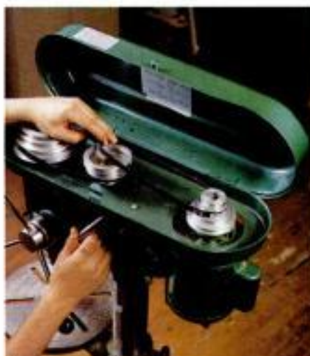
Simple speed control. A step-pulley system regulates spindle speed on most models.
