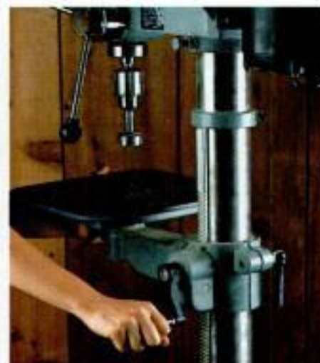
Crank it up. A rack-and-pinion mechanism makes it easier to adjust heavy cast tables.
