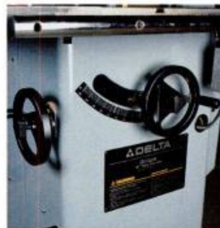
Sturdy, smooth-operating mechanisms. Look for well-made controls that move easily and lock adjustments firmly.
