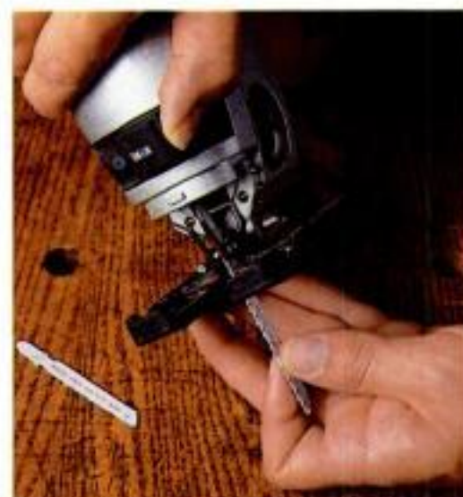
Quick change. A quick-release lever replaces the conventional setscrew for tool-free blade replacement.
