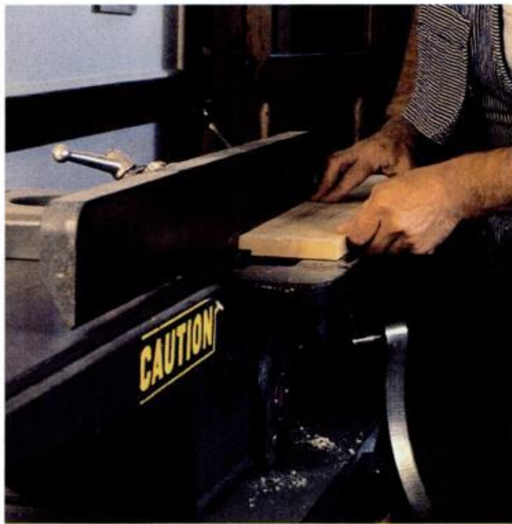
A ledge for rabbets. On a jointer equipped with a rabbeting ledge, you can quickly and easily mill rabbets and tongues.
