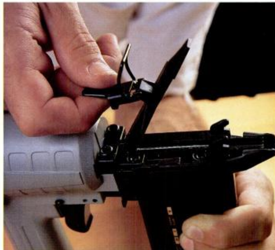
Quick-release nosepiece. A draw-catch release allows quick access to the firing compartment for clearing jams.
