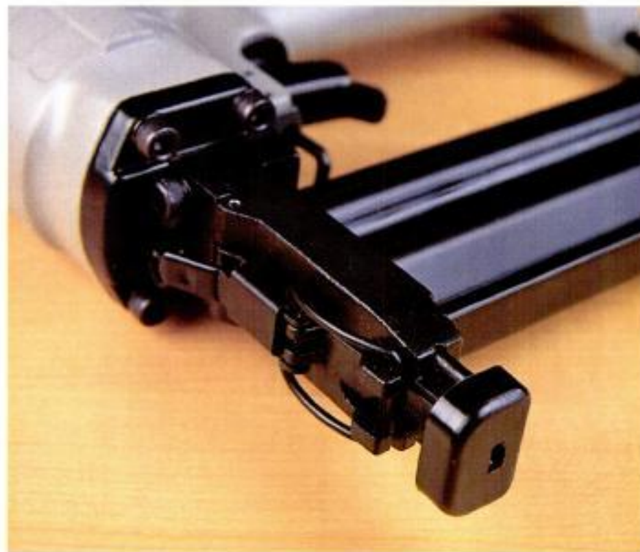
Rubber nose tip. A rubber nose tip keeps wood from being marred by the gun's nose.
