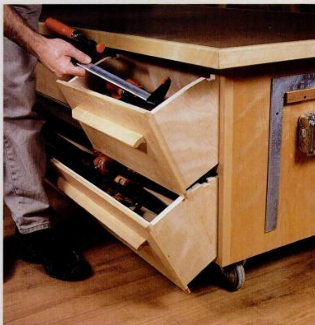
Tilt-out storage. These drawers pivot out and stop, allowing you to quickly access assembly tools such as clamps.
