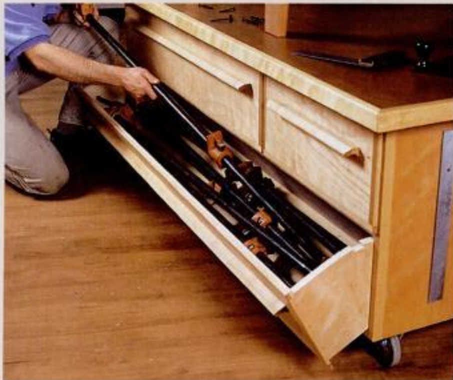
Tilt-out clamp storage. The tilt-out drawers pivot open and stop, making it easy to get to your stash of pipe clamps. (See page 81.)
