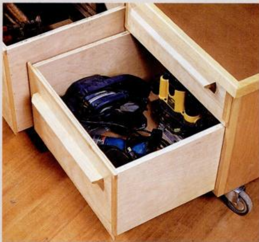
Deep storage drawers. Two tall drawers hold stacks of quick clamps or power tools such as routers, sanders and hand-held planers.
