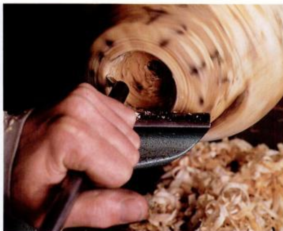
Thin the walls with the bent tool. Angle the bent point down slightly, then raise it to horizontal when entering the wood.
