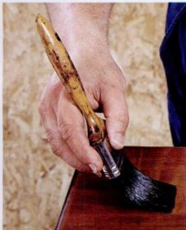
Ending stroke. To get the last bit of finish out of the brush, increase downward pressure without changing brush angle.
