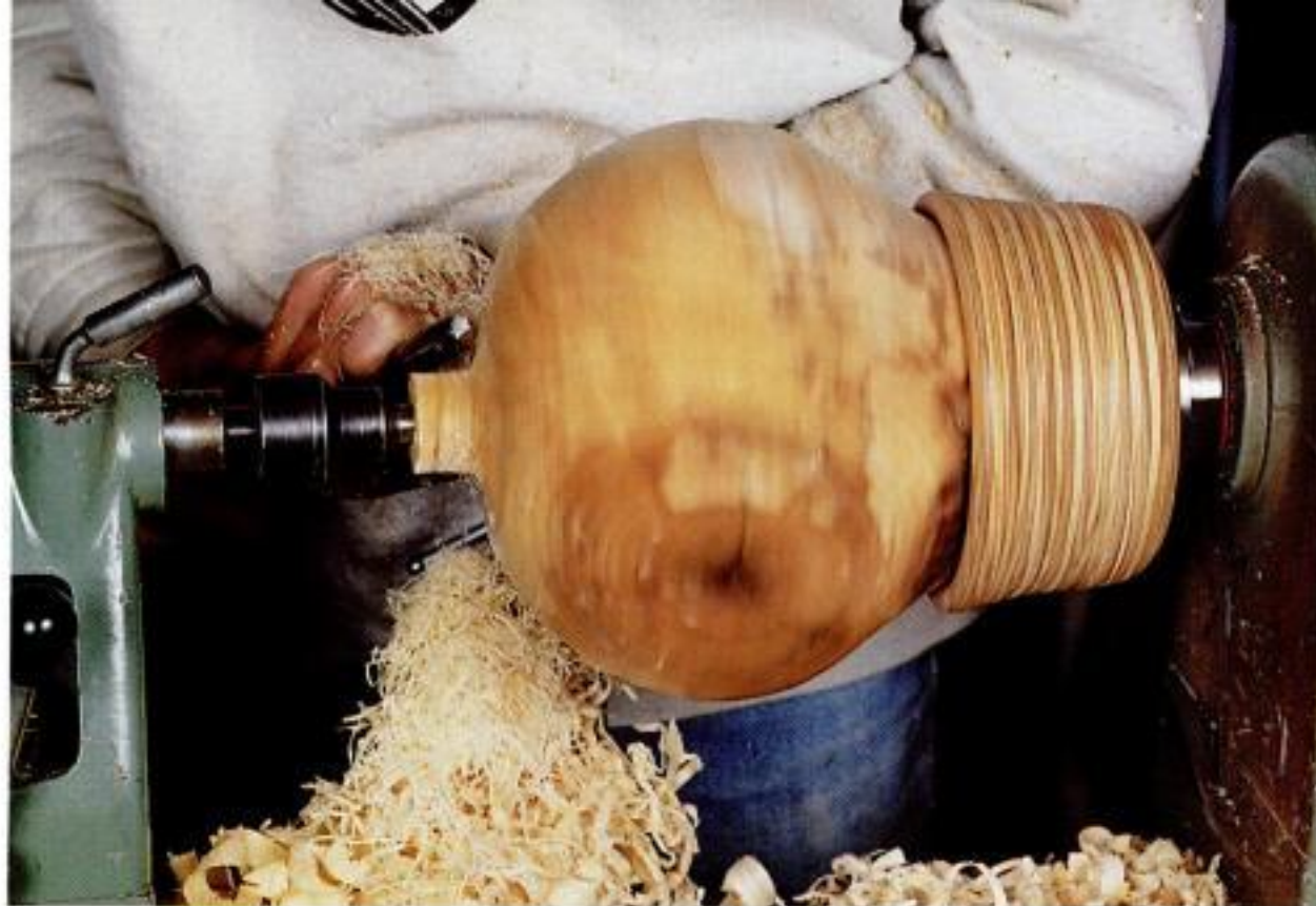
Turning off the base. Fit the hollowed end of the vessel in a jam chuck made from plywood, and center the tailstock in the base to part the vessel free.
