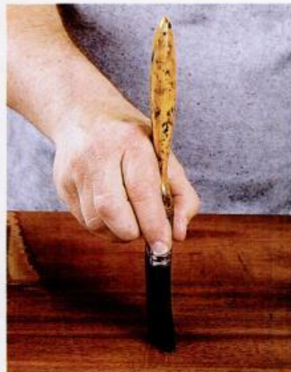
Tipping off. For a smoother finish, hold the bristles at 90° to the surface and run the tips lightly through the finish, moving with the grain.
