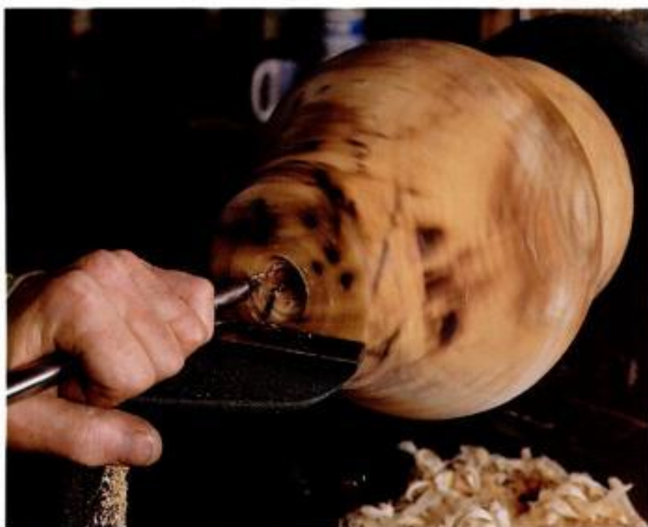
Bore with the straight tool. Keeping away from the walls, excavate into the body of the vessel with a slight sweeping motion.
