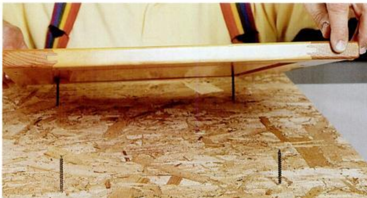
Bed of nails. Protruding nail points provide support when varnishing two sides of a workpiece at once.
