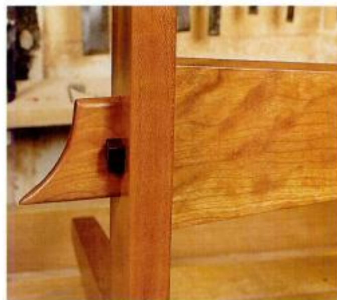
Locked with a wedge. This sturdy knock-down joint is held together with a wedge that slips through a mortise in the tenon.
