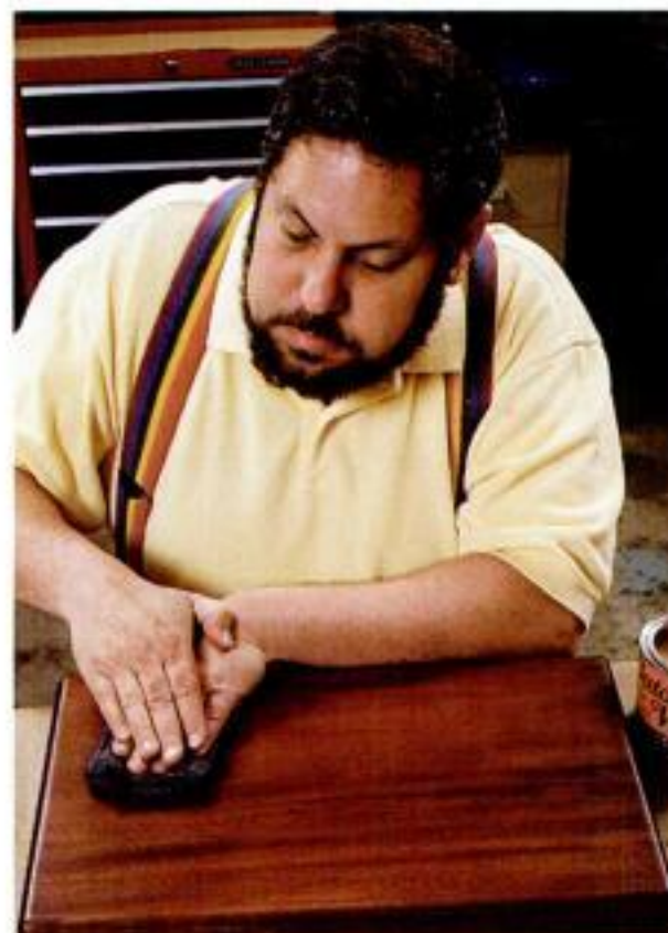
Rub out for luster control. To give the final coat a uniform satin luster, rub it down with some paste wax and a ScotchBrite™ or similar abrasive pad.
