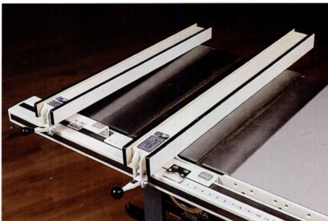
Different size, same performance. "Commercial" fences, like the Biesemeyer shown at right, are longer, taller, and heavier than their "Home Shop" counterparts. But both types perform equally well.
