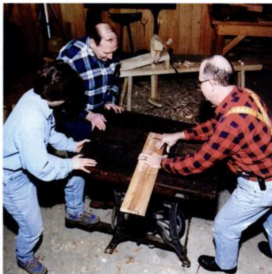
"Please touch" museum. Steppingstone Museum shop master Wade Whitlock (right) cuts a board on a foot-powered tablesaw, while apprentices pump the treadle.
