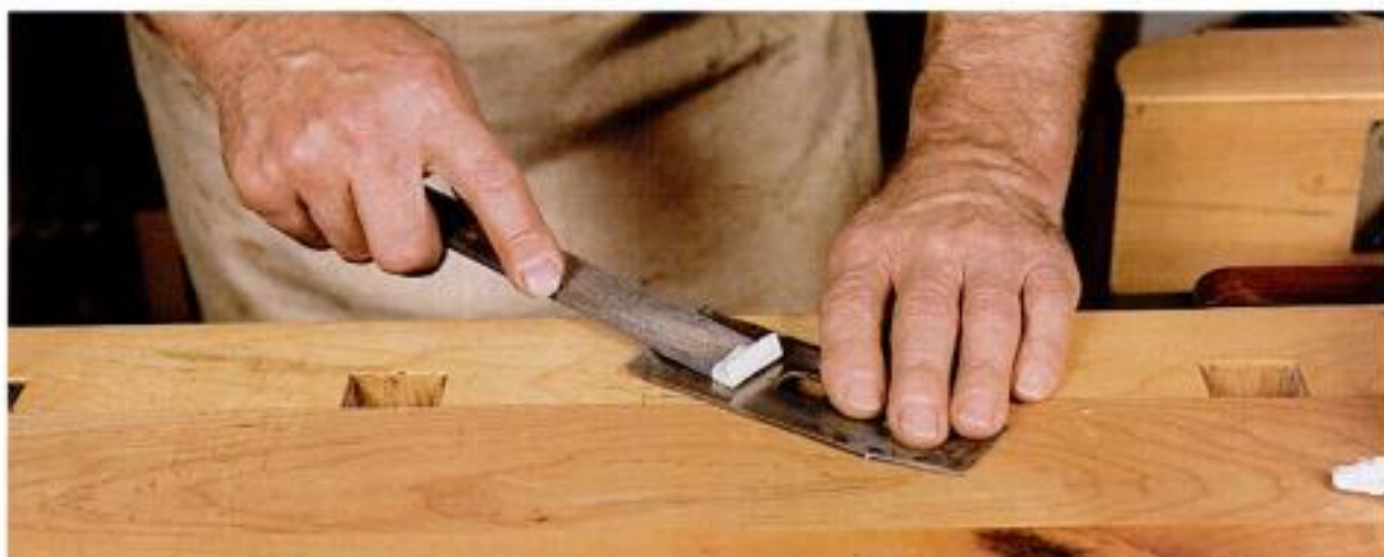
Flat and beveled. Use a mill file to flatten the angled back of the chip breaker. A piece of masking tape on the tip of the file prevents scratches.
