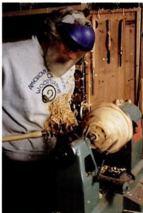
Shape the outside first. Working with the blank mounted between a faceplate and a live center, use a gouge to rough out the form.
