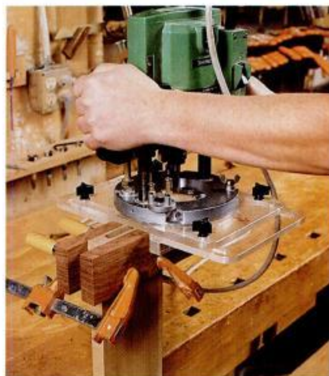
Plunge route the mortise. Staples uses a \frac{1}{2} -in. upcut spiral bit and a pair of fences attached to the router baseplate to route the mortise in the end of the stretcher.
