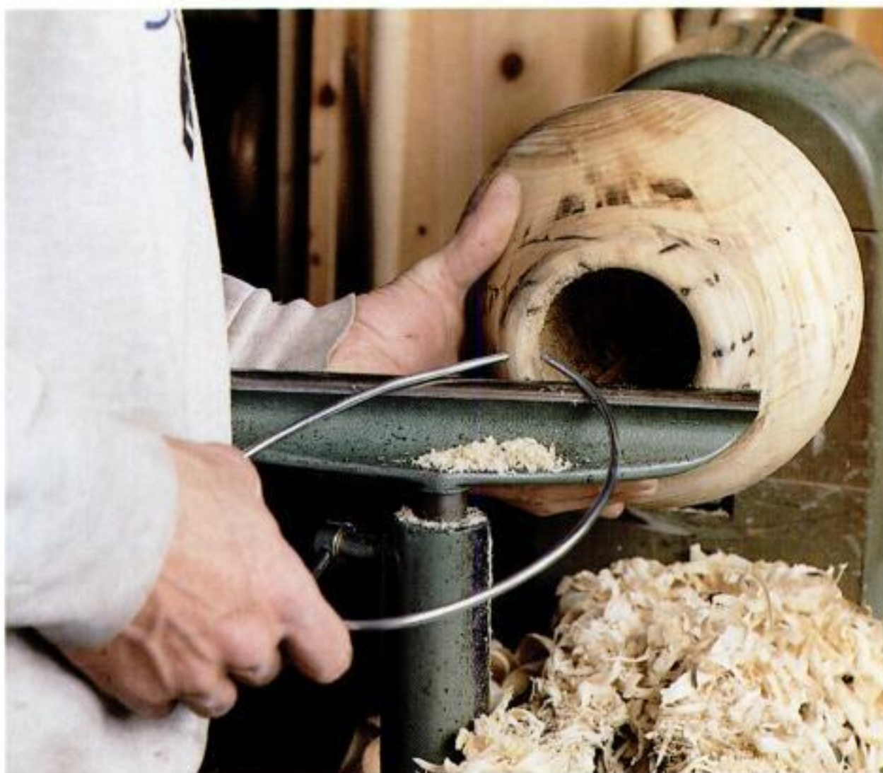
Shop-made calipers. Inexpensive \frac{3}{16} -in.-dia. steel rod can be bent to form an effective tool for measuring wall thickness.
