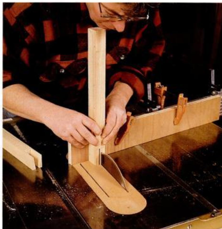
Pins second. With the miter gauge angled at 8°, Staples saws the dovetail socket in the suspension arm by holding the work against a high fence attached to the miter gauge.
