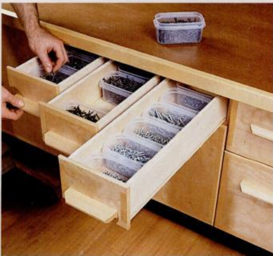
Fastener drawers. Three small drawers fitted with plastic food containers organize assembly hardware and provide convenient access.
