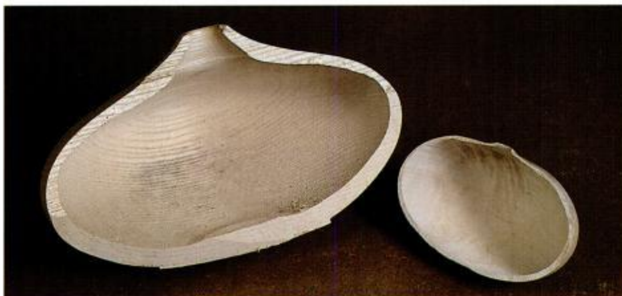
Thick and thin. Bandsawn sections through failed vessels can teach a lot. The larger vessel broke apart while the area near the opening was being worked. Too much material had already been removed close to the base, so support at the rim wasn't sufficient. The walls on the smaller vessel were thinned unevenly, especially at the base.
