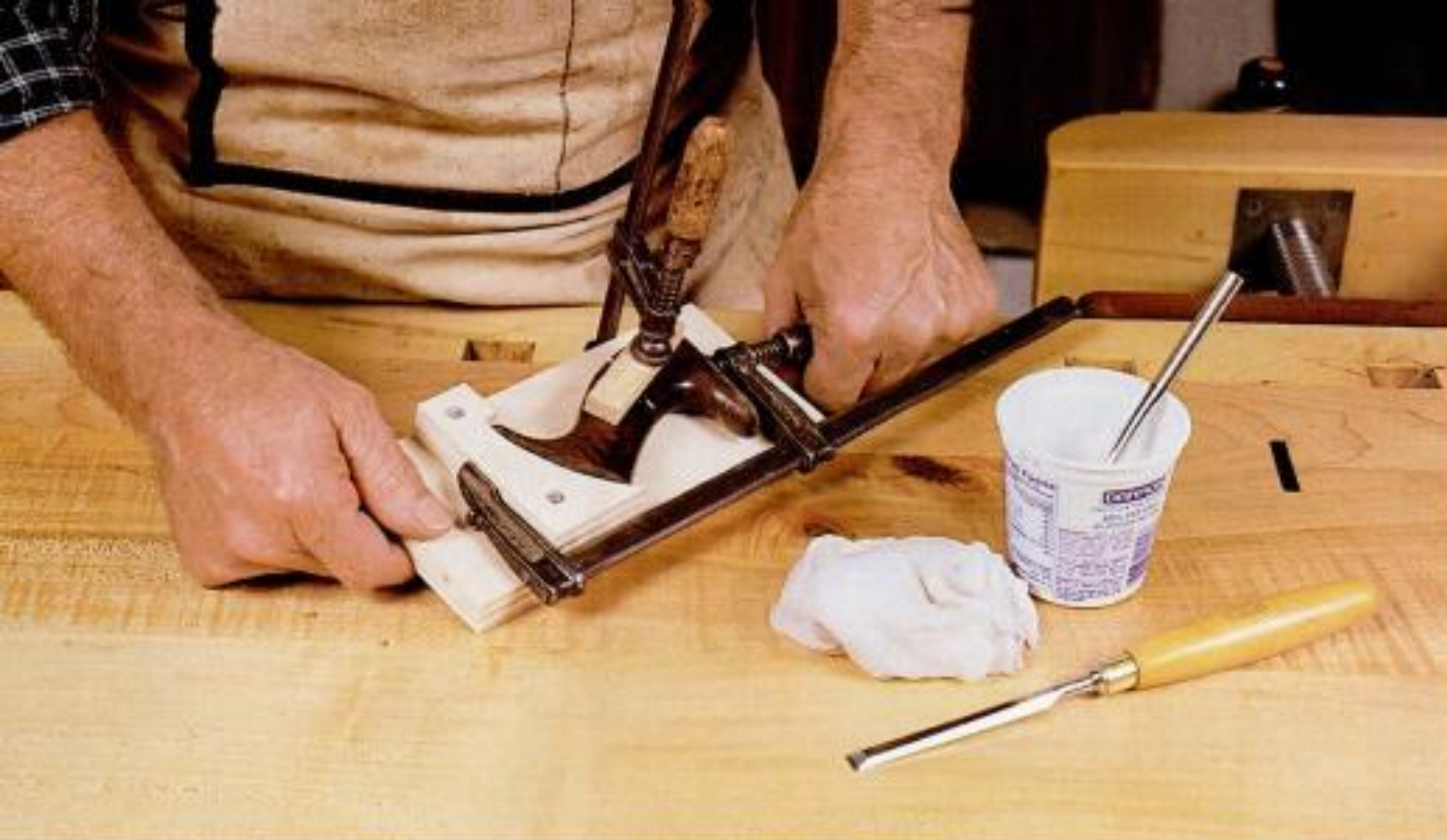
Handle cure. Klausz glues a broken handle back together by clamping it in a simple homemade jig.
