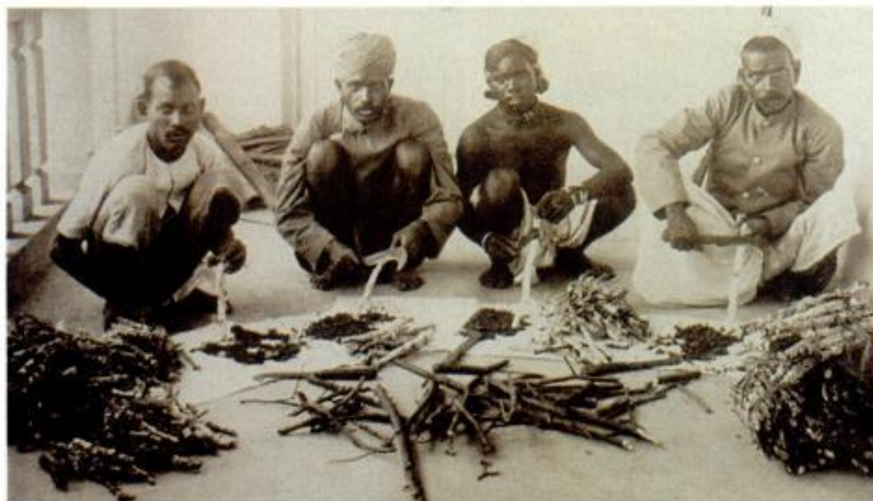
Hand-made shellac. Many cottage industries still produce raw shellac. Here, workers scrape shellac resin from tree branches in India and Thailand.
