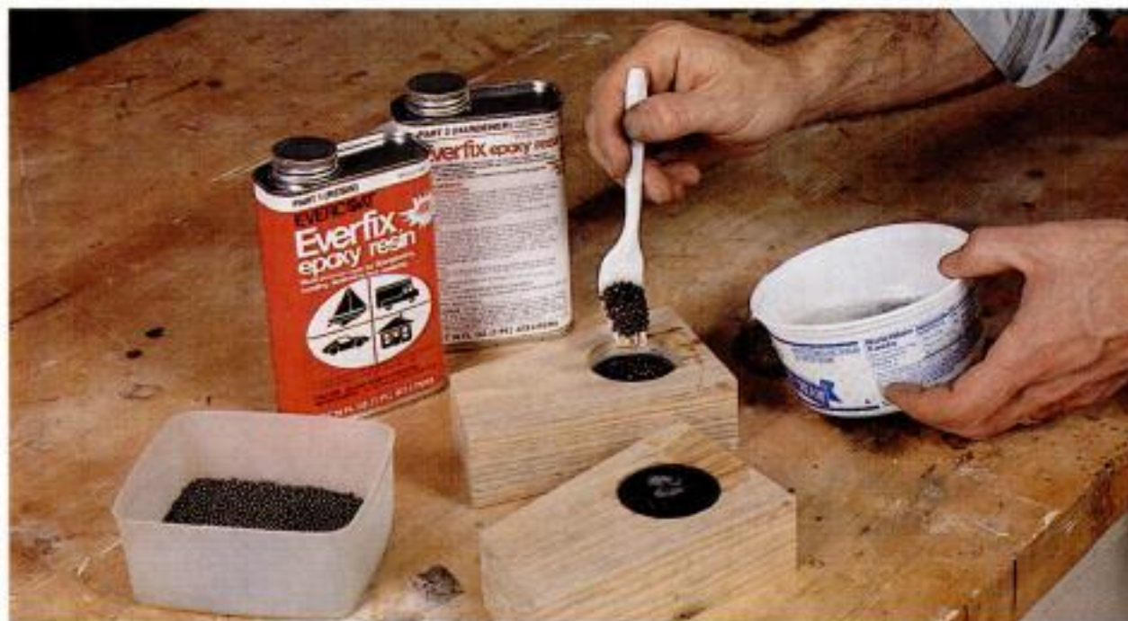
Lead ballast. Fill the cavities in the core pieces with a mixture of lead shot and epoxy resin. Be careful not to overfill the holes.
