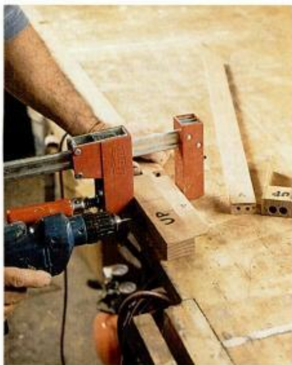
Drilling for dowels. The author uses a pair of homemade jigs to drill pairs of dowel holes in the stiles and rails. Metal drill bushings guide the bit.
