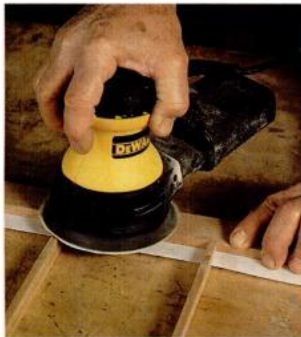
Shim and sand. Use strips of Synskin™ as spacers when installing the removable kumiko. Then sand the kumiko flush to the frame.
