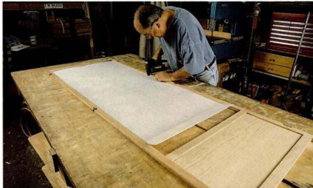
Attaching the skin. Secure the Synskin™ to the fixed kumiko, using staples every 10 in. around the perimeter.
