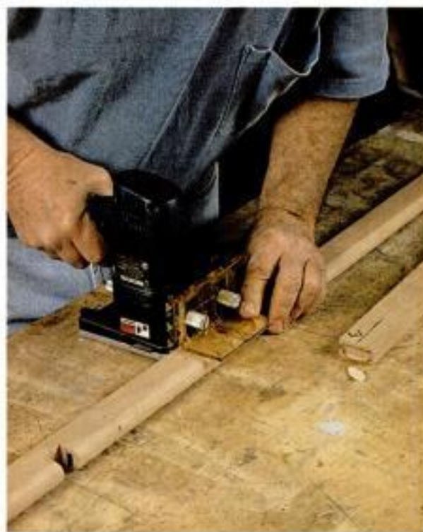
Tiny biscuits. Ryobi's "mini" biscuit joiner is handy for joining the narrow middle rail. Cut double slots in the rail and the stiles.
