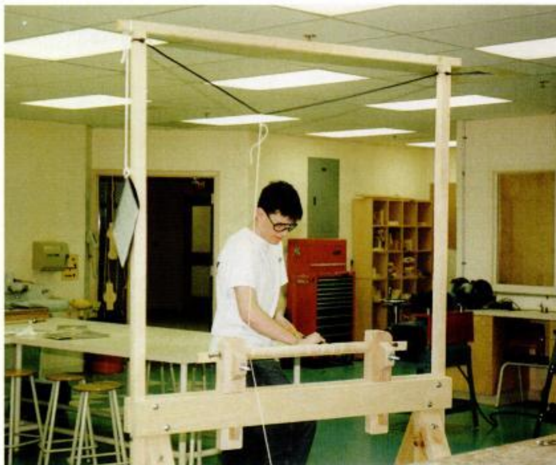
Time-tested technology. Kyle Adam, a 13-year-old Ontario youth, shows off the bungee lathe he built for his school technology project. Good work, Kyle!
