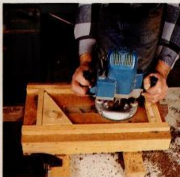
Rout the large compartment. Use the narrow insert and the small angled insert to define the opening size. Plunge cut with a straight bit.
