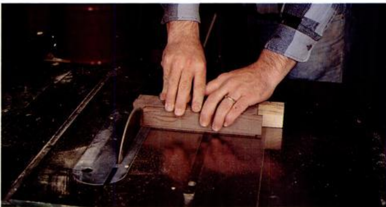
Trimming the ends. Make two cuts on the tablesaw to trim the ends and lid. To complete the box, carve a fingerpull in the lid, then sand and finish.
