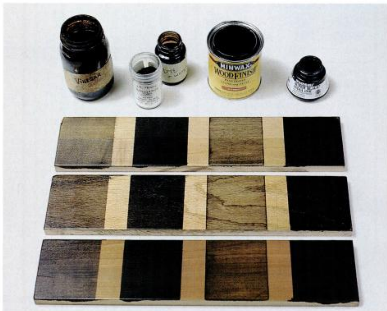
Fade to black. Ebonizing treatments have different effects on different woods. Woods from top to bottom are soft maple, oak and cherry. Treatments from left to right are vinegar and rust, black dye, black pigment stain and India ink.
