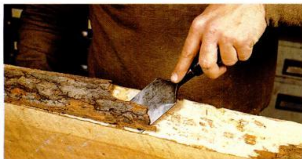
Pop the bark. Pry the bark off natural edges with a dull old bench chisel.
