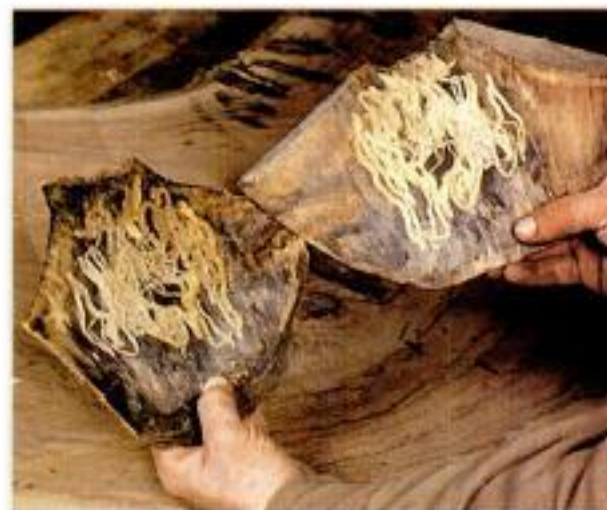
Bug work. When wood is air dried, insect larvae munch tiny tunnels through the cambium layer, creating unpredictable patterns and textures.
