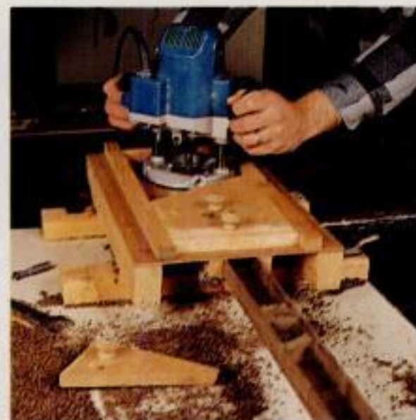
Rout the small compartment. Fit the narrow insert and the large angled insert inside the jig's borders to rout this small opening.
