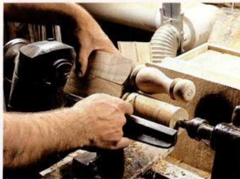
The prototype is the template. To turn a set of four "identical" legs, use your prototype or a single leg as your template.
