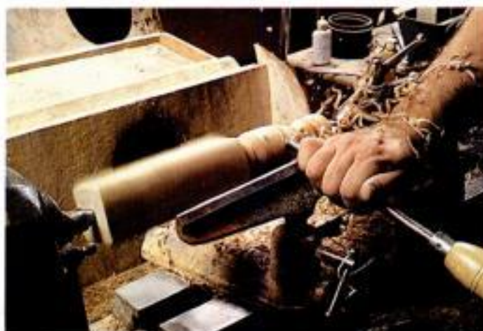
Taper the middle. Remove waste with the gouge, cutting to your parting diameters to form the belly and hollow.
