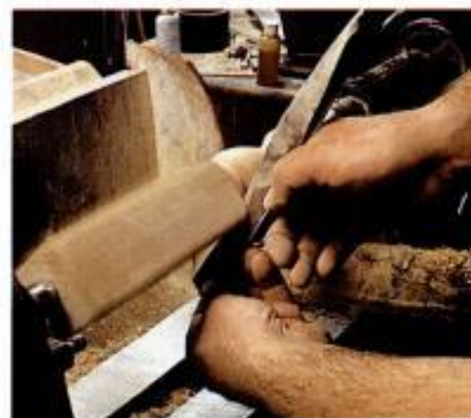
Sanding trick. Fold sandpaper around a flexible plastic ruler to smooth the chamfer.
