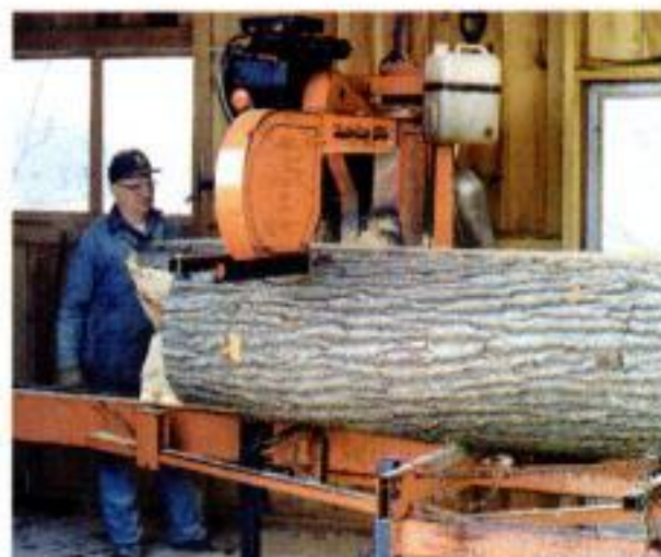
Through and through. Bandsaw mills are your best bet for custom sawing of irregularly shaped logs.
