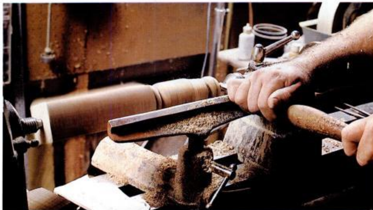
Form the ball. Cut this detail like a large bead, using a beading tool or skew chisel. Work from large diameter to small.
