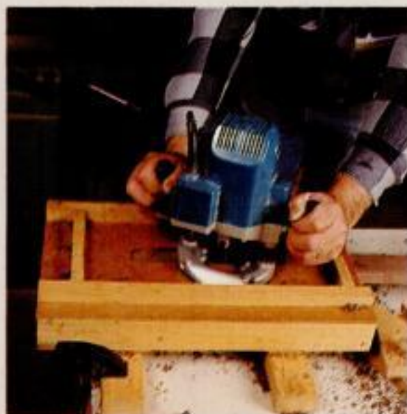
Rout the dovetail slot for the lid. Start and stop the router in the middle of this excavation. No inserts are used in the jig for this first cut.
