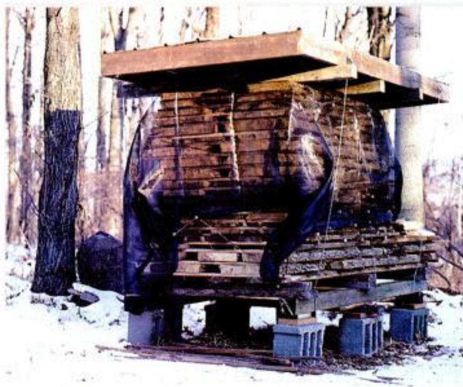
Stack it right. A well-constructed lumber pile keeps water out and allows unrestricted airflow around the boards.
