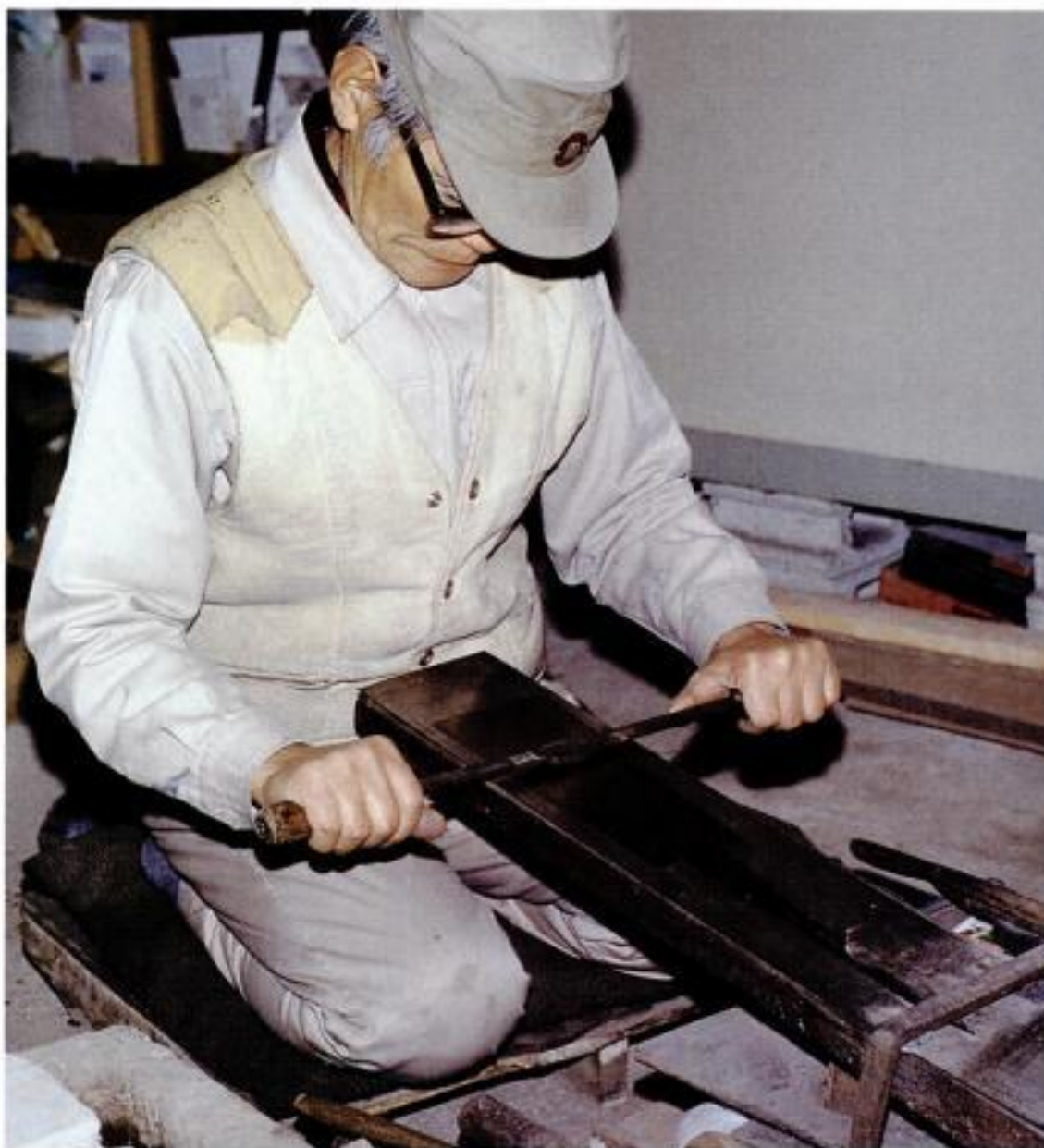
A lifetime of pride and joy. Mr. Hirota is now an elderly man. He has been making Japanese saws all his life. Here, he flattens a saw blade.
