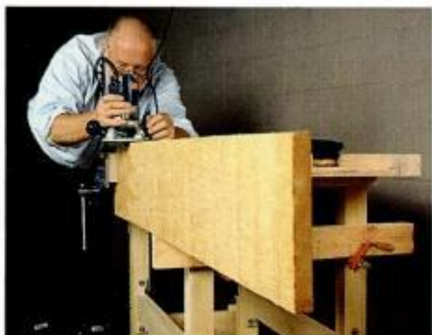
Wide plank. Clamp a beam to the bench legs to support weighty work.
