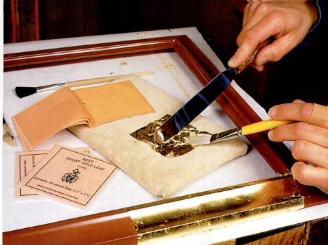
Cutting loose leaf. To cut loose leaf into smaller sections, place it on a shop-made gilder's pillow, or "klinker"—a soft, chamois-covered pad—and cut it with a dull-edged gilding knife.
