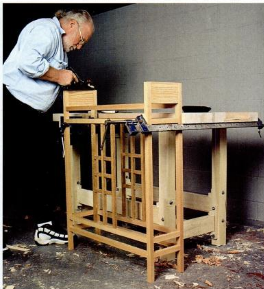
Holds anything. Two clamps and a scrapwood prop bring the joint that needs work tight onto the benchtop (left). Furniture of any size can be backed up to the bench and compelled to hold still (right).
