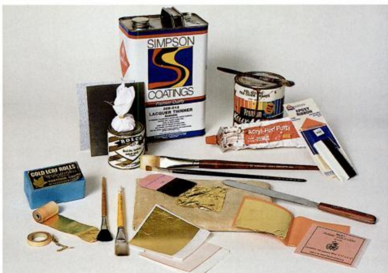
Materials and supplies. Some of the supplies you may need for gilding include gold leaf; special "size" varnish; a cloth "bob" to apply the size; various brushes; putties; and a gilder's knife and "klinker," or chamois-covered pillow.
