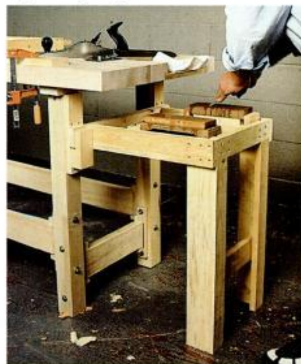
Sturdy support. The workbench can support any number of specialized accessories and stands, such as this removable sharpening outrigger.
