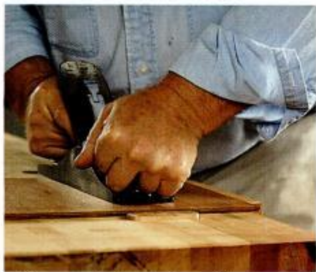
Thin wood. The replaceable stop can be set low enough for any wood.
