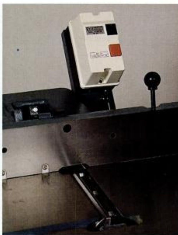
Switch and slide. The Star's switch wins the prize for accessibility. Plastic inserts on the bottom of the fence protect the tables.
