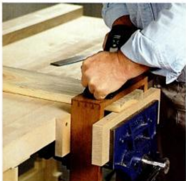
Drawer stop. A plank draped across the bench supports a delicate drawer.
