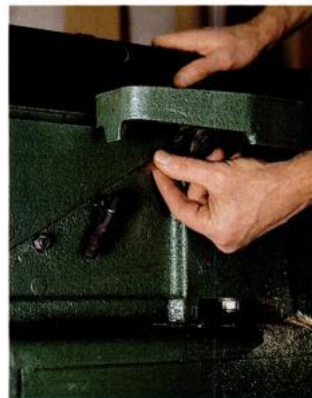
Shim it straight. Correct table misalignment by inserting brass shim stock in the ways of the outfeed table.
