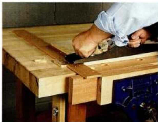
Wide panel. The panel stop, held by bench stop and vise, traps wide work.
