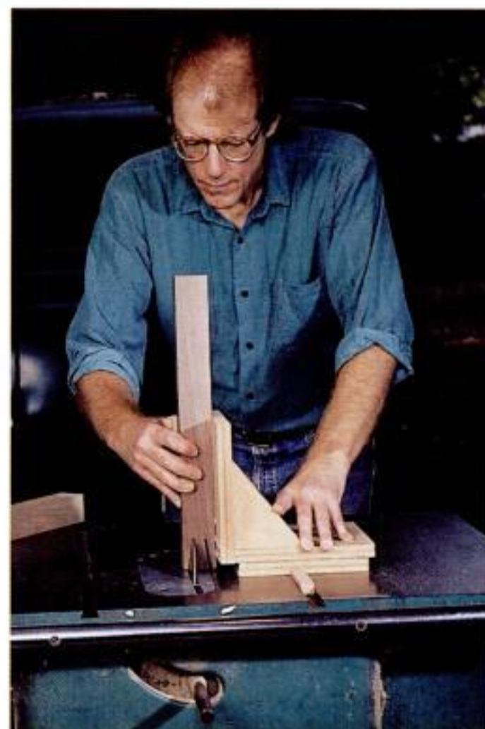
Big dovetail. To cut the dovetail cheek, tilt the saw blade and hold the stock vertically in a tenoning jig.
