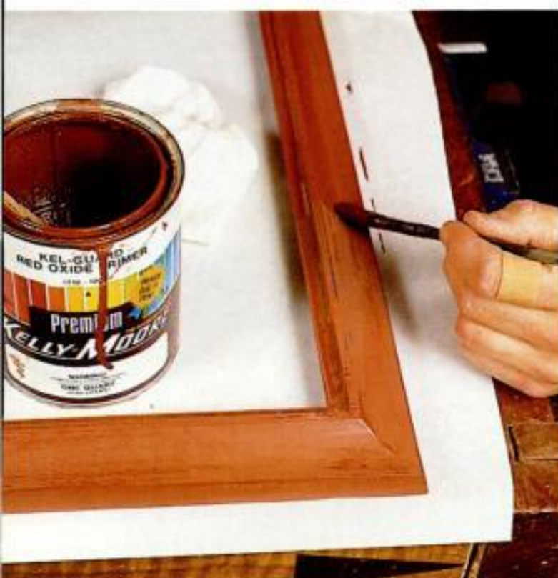
Applying the base coat. Prime the wood with four or five coats of a good quality red oxide or japan paint, sanding between coats to create a glass-smooth surface.
