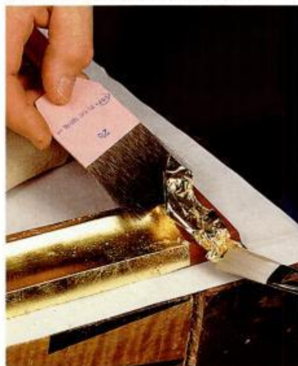
Carrying leaf. Transport cut leaf to the workpiece with a "gilder's tip" brush. You can use another brush to help position the leaf.
