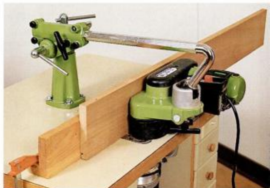
Feeding time. Sunhill's M-3 "Baby" power feeder is ideal for small-shop production runs.
