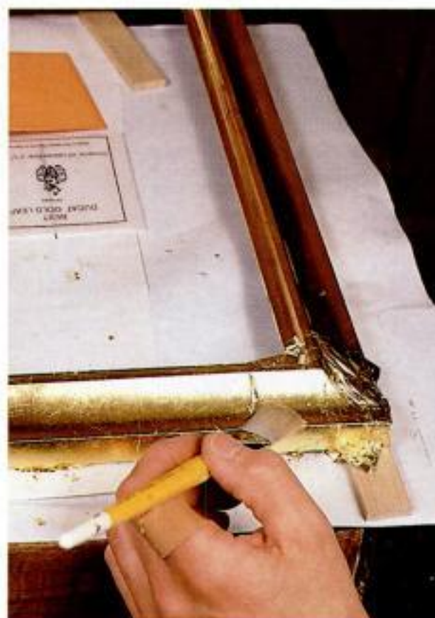
Tamping the leaf. Use a very soft-bristle brush to press the leaf into the tacky coat of size. Brush off excess that overlaps onto adjacent leaves.
