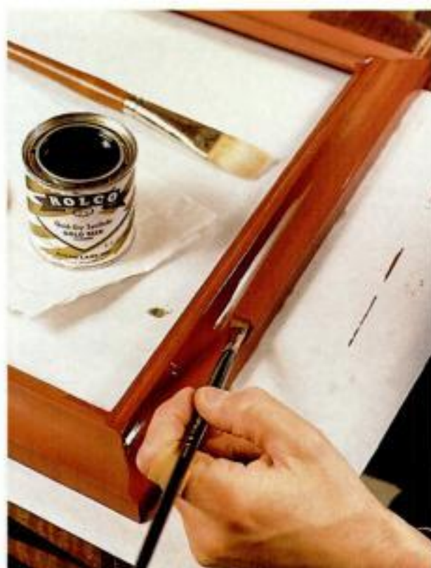
Applying the size. Brush on the "size" varnish with a sable brush. The surface is tacky enough for gilding when your knuckle pulls back from the varnish with a slight snap.
