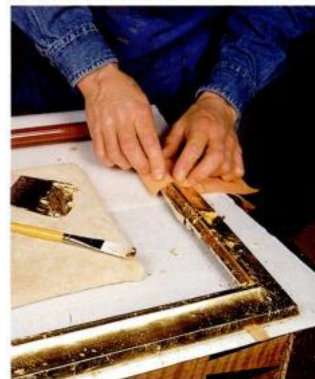
Applying the leaf. One of the easiest ways to apply leaf is to press it into the tacky varnish through the leaf's paper backing.
