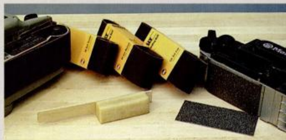
Grits, graphite and a cleaning stick. Belts are sold in coarse, medium and fine grits. To increase belt life, use a belt-cleaning stick (left foreground) and equip the sander with a graphite platen (right).
