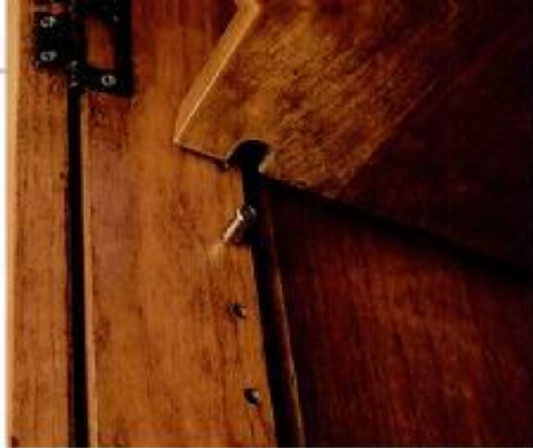
Lift, don't slide. To keep adjustable shelves from sliding forward, rout pockets for pins underneath.
