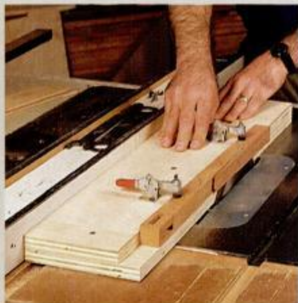
Hands-free tapering. Small toggle clamps hold the work, so your hands never get near the blade.
