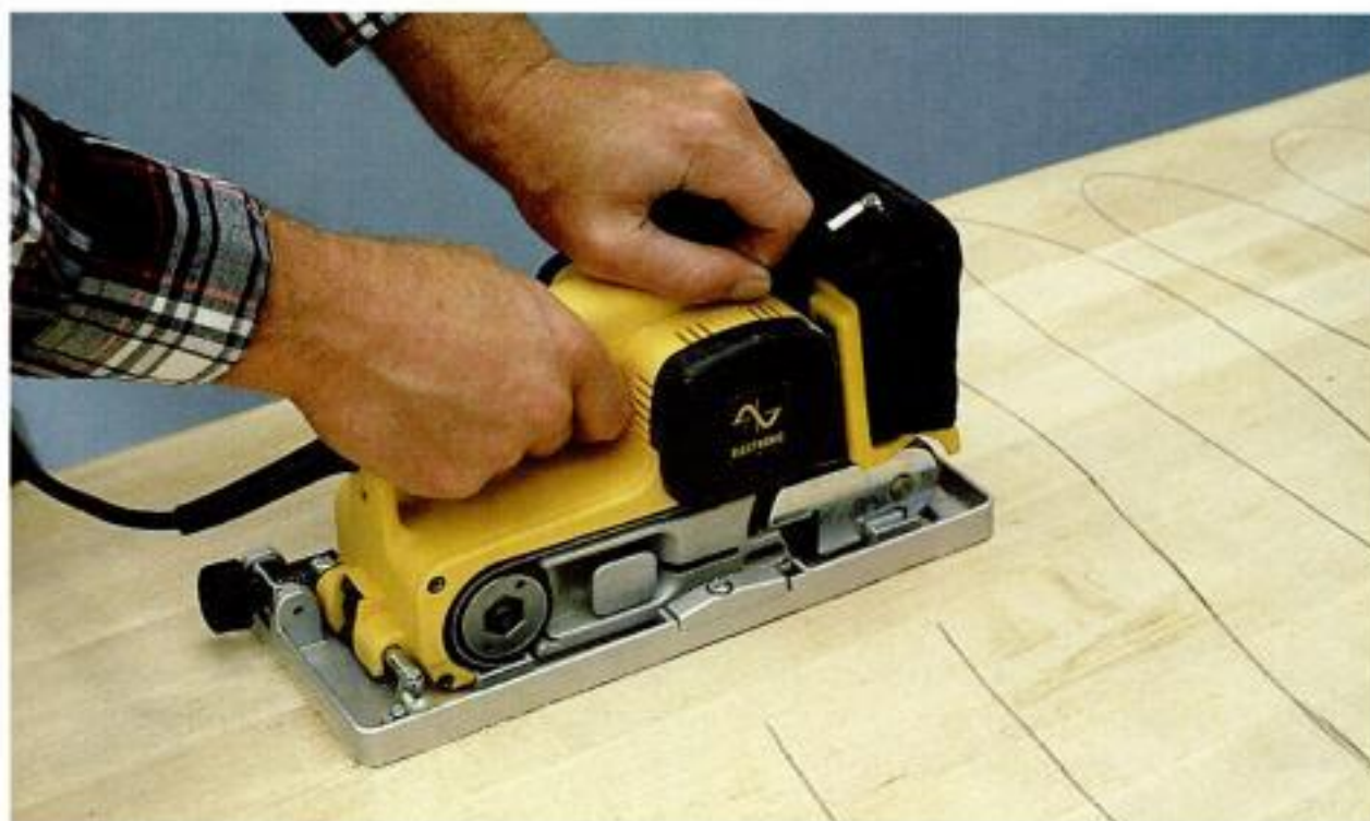
Smoothing a panel. Drawing wavy pencil lines on the stock will help you monitor sanding progress. A sanding frame improves stability.
