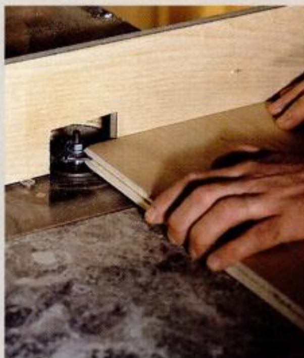
Routing the groove. Use a \frac{1}{8} -in. slotting cutter in the router table to rout stopped grooves in the partition.
