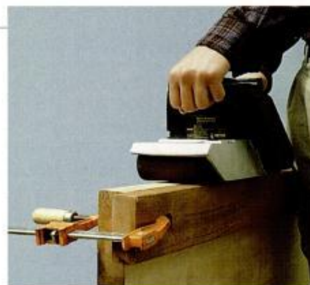
Belt sanding edges. To sand narrow edges, clamp a scrap board to one side of the workpiece for stability.
