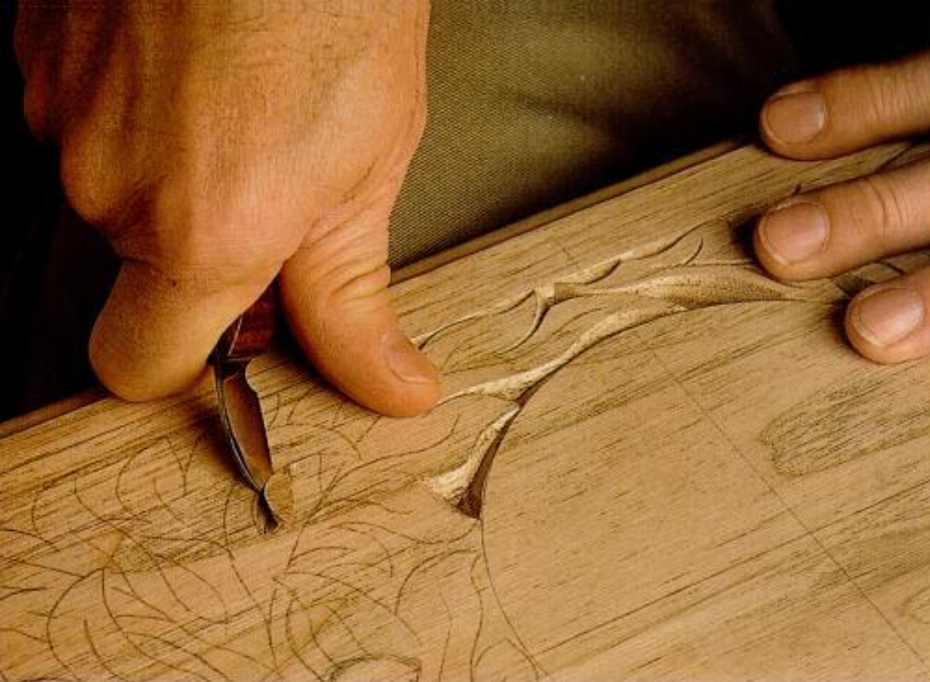
Making a two-sided chip. Leaning the knife at 65°, make two opposing cuts that meet at the bottom, to create a V-shaped chip that lifts from the wood.
