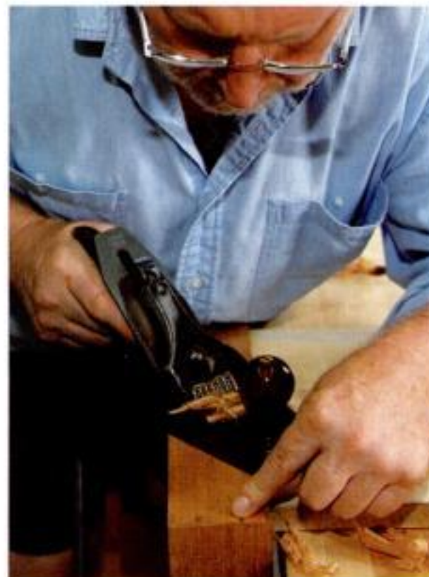
Feel your way. While you may not be able to see how far to plane, you can feel the difference between the dovetail pins and the drawer side. Stop planing when they are flush.
