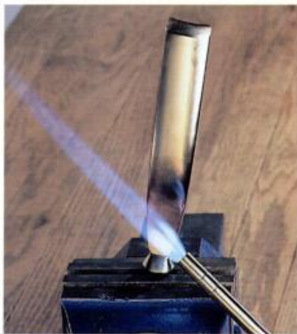
Tempering. To toughen the metal and make it less brittle, temper it by heating it very slowly until it turns straw-yellow.
