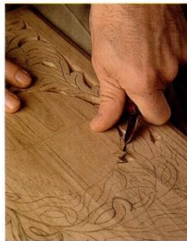
Easy as 1-2-3. All the walls of a chip are cut with the same basic procedure. Cut around short grain first. (See Fig. 2.) Start the cut at an intersection, leaning the knife 65° to its side. Plunge deeper as you approach wide areas, and shallower toward narrow areas. If any bits of wood remain after you've freed the chip, get rid of them with a cleanup slice.
