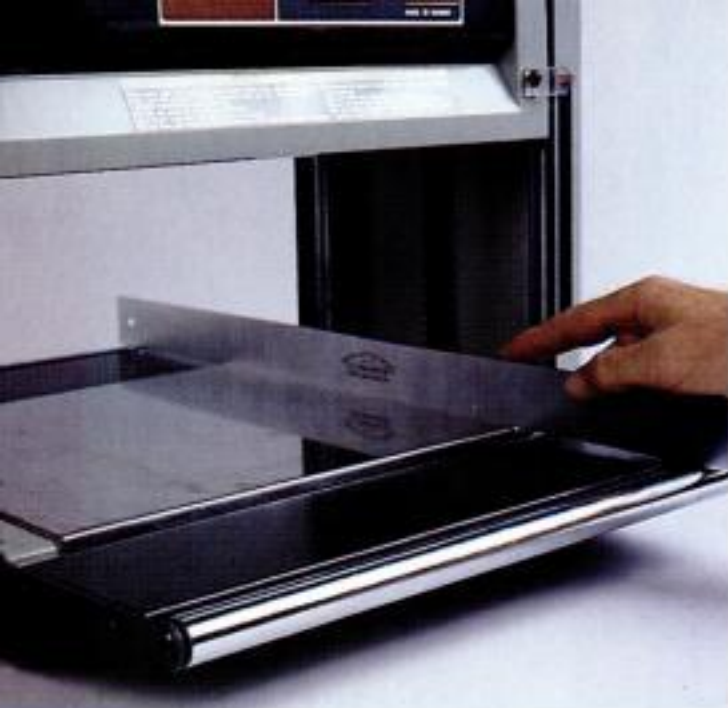
Checking extension-table height. Use a straightedge to set extension-table rollers level with the bed.
