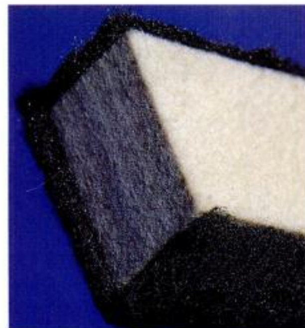
Not just for sandpaper. Use a felt block to back steel wool for more consistent results.
