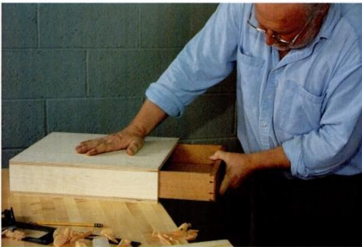
A tight fit. Run the drawer in and out to locate the high spots, and plane them off. When it fits right, the drawer should close with a fingertip's pressure, and the soft whoosh of trapped air.
