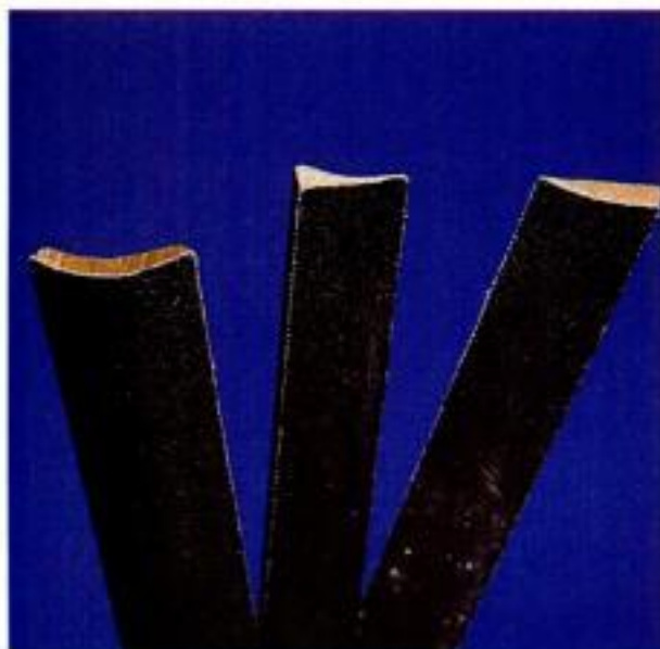
Sanding sticks. Shop-made wooden files are great for tight curves and corners.
