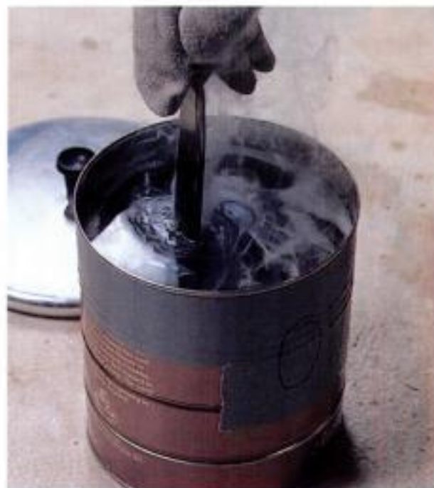
Quenching to harden. After reheating the tool to a cherry-red color, quench it by stirring it in oil. This rehardens the end of the tool.
