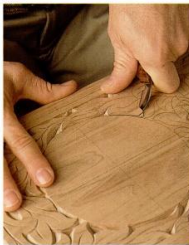
Easy as 1-2-3. All the walls of a chip are cut with the same basic procedure. Cut around short grain first. (See Fig. 2.) Start the cut at an intersection, leaning the knife 65° to its side. Plunge deeper as you approach wide areas, and shallower toward narrow areas. If any bits of wood remain after you've freed the chip, get rid of them with a cleanup slice.
