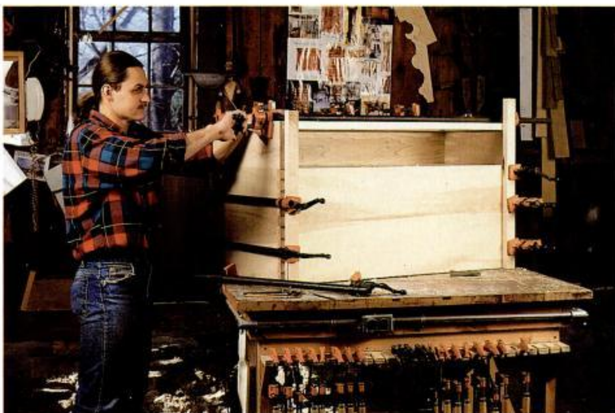
Pulling it together. Slow-setting hide glue is a good choice for a time-consuming glue-up. Clamping cauls pull pins and tails tightly together.
