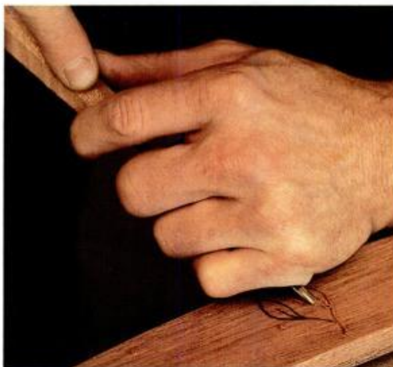
Carving the detail. Carve the leaf detail with a #12, 3mm V-gouge. Come in first from one direction and then from the other, to avoid going against the grain.
