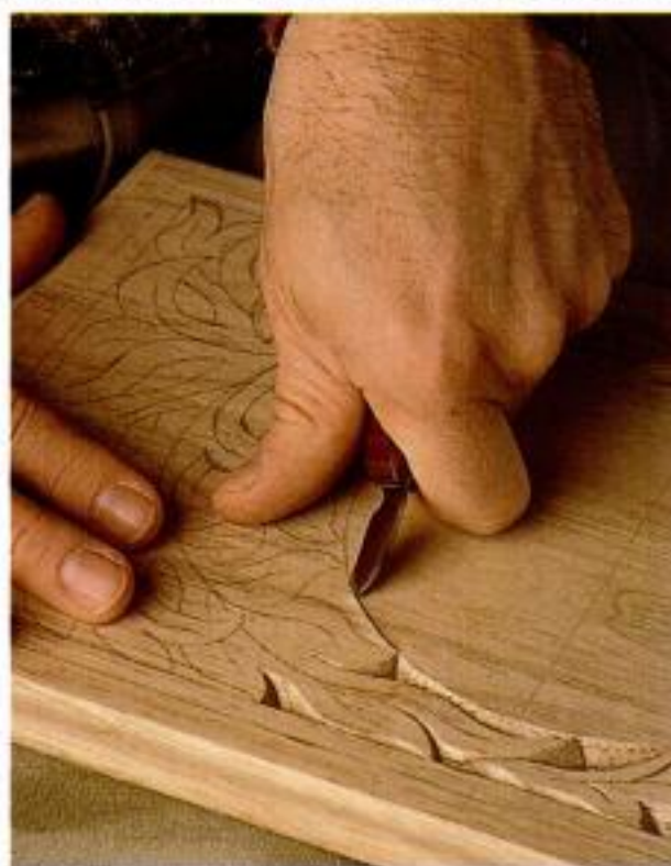
Easy as 1-2-3. All the walls of a chip are cut with the same basic procedure. Cut around short grain first. (See Fig. 2.) Start the cut at an intersection, leaning the knife 65° to its side. Plunge deeper as you approach wide areas, and shallower toward narrow areas. If any bits of wood remain after you've freed the chip, get rid of them with a cleanup slice.
