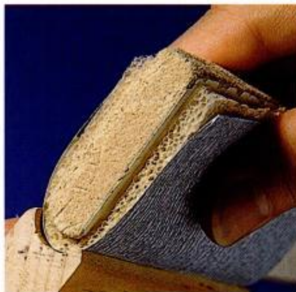
Form follows function. Extra foam padding makes standard-size blocks fit a variety of specialty tasks.
