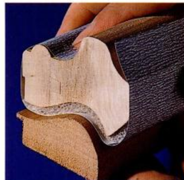
Shapely blocks. Elaborate blocks can be carved to fit wide moldings. Use smaller blocks for single elements.
