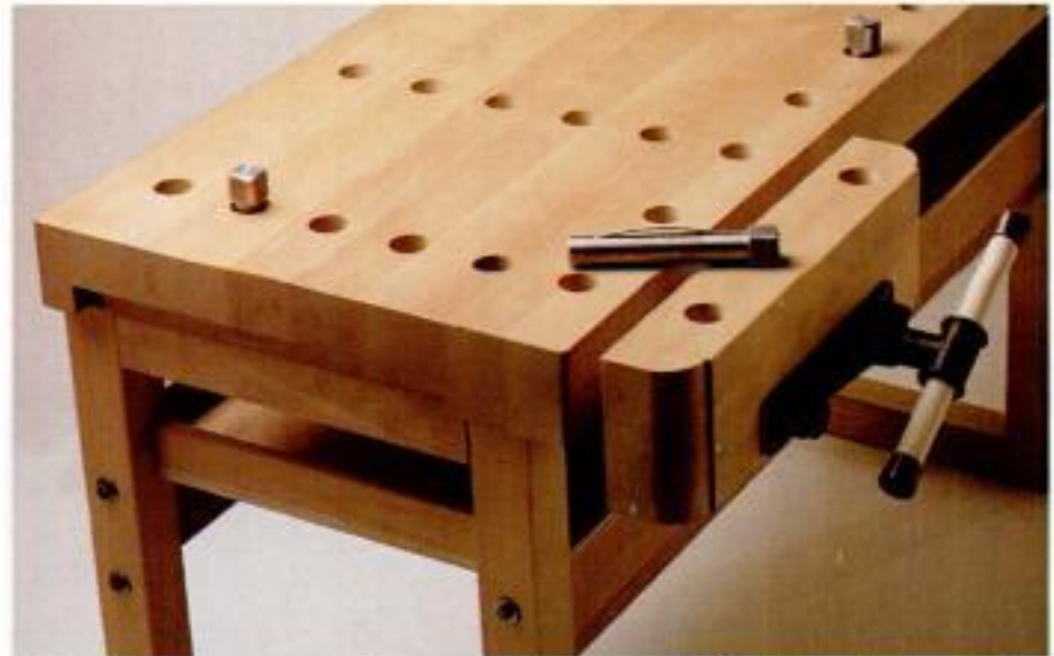
Thick on top. A thick top and an even thicker edge, as on this Ulmia Professional, are indications of a high-quality bench.
