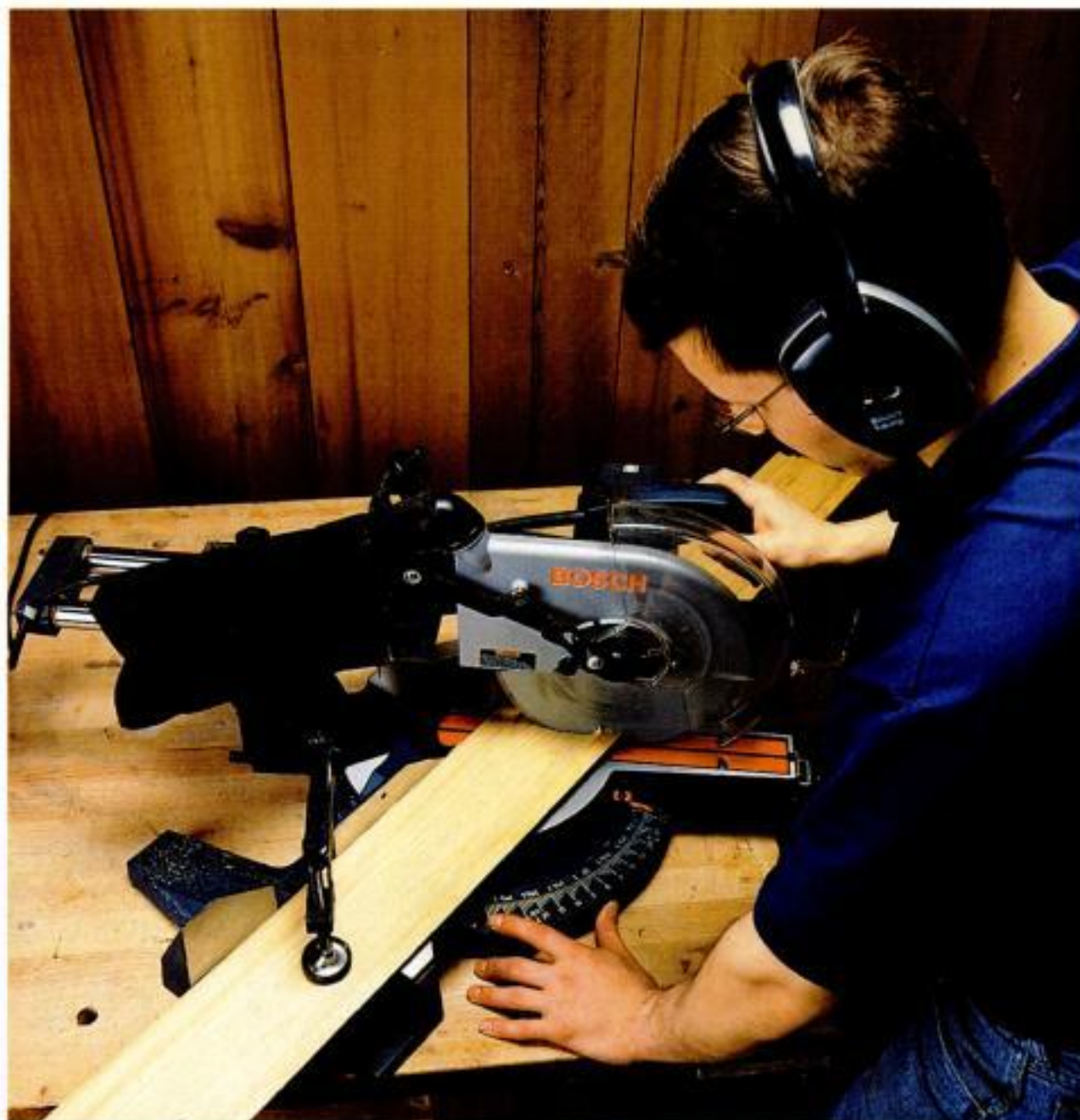
Shop chops. For portability, precision and ease of use, miter saws beat radial-arms. This sliding compound saw can crosscut stock up to 12 in. wide.
