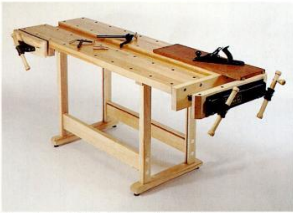
A good vise. This Veritas bench has a twin-screw end vise that lets you clamp wide workpieces without racking.
