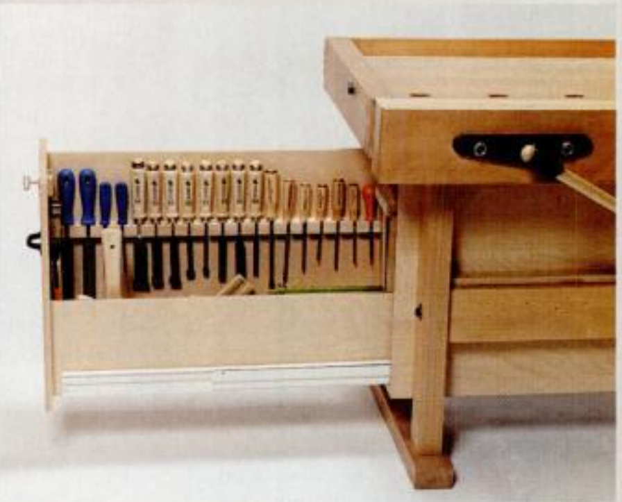
Sliding shelves. Diefenbach's single drawer allows access from the end—a handy feature when work is clamped along the front of the bench.
