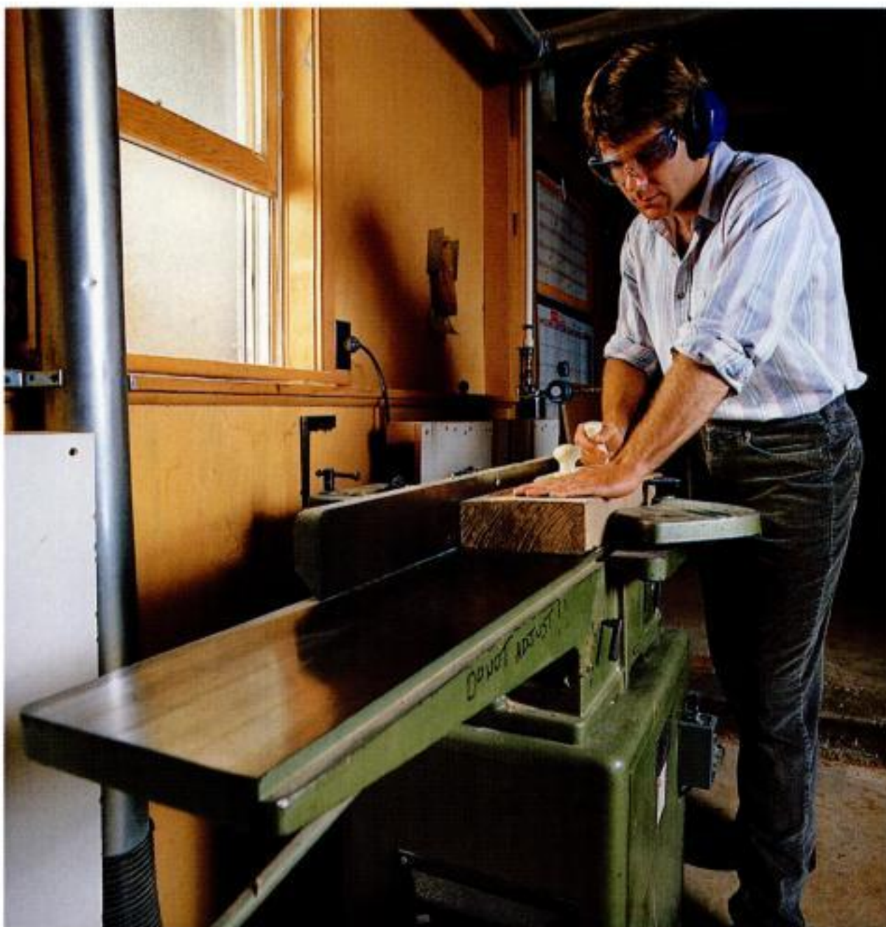
Straight and flat. The jointer can transform boards that are rough or uneven, leaving smooth, straight surfaces and square or beveled edges.
