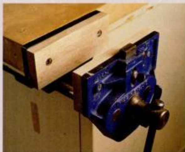
Face vise. The Record vise has a quick-release lever and a sliding dog (Garrett Wade).
