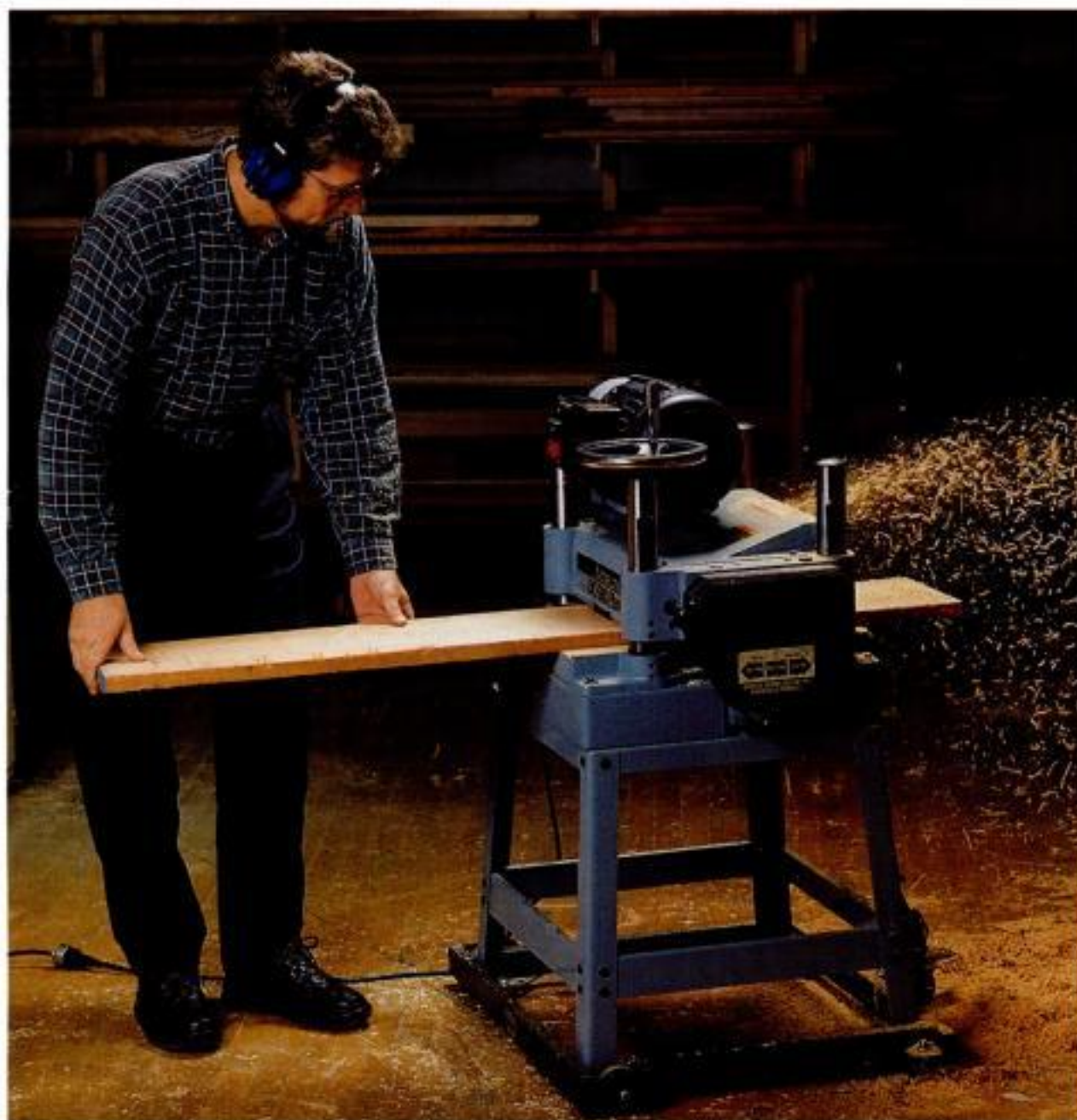
Shaving it down to size. A thickness planer allows you to mill lumber to the exact thickness you want for your project.
