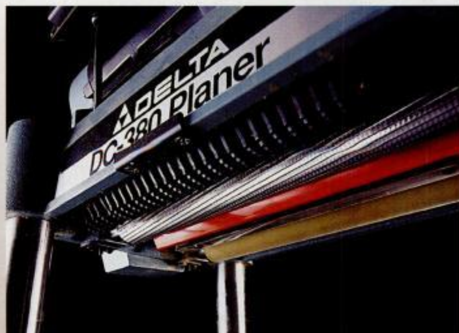
Infeed rollers. Serrated infeed rollers are effective in moving heavy boards through the machine.
