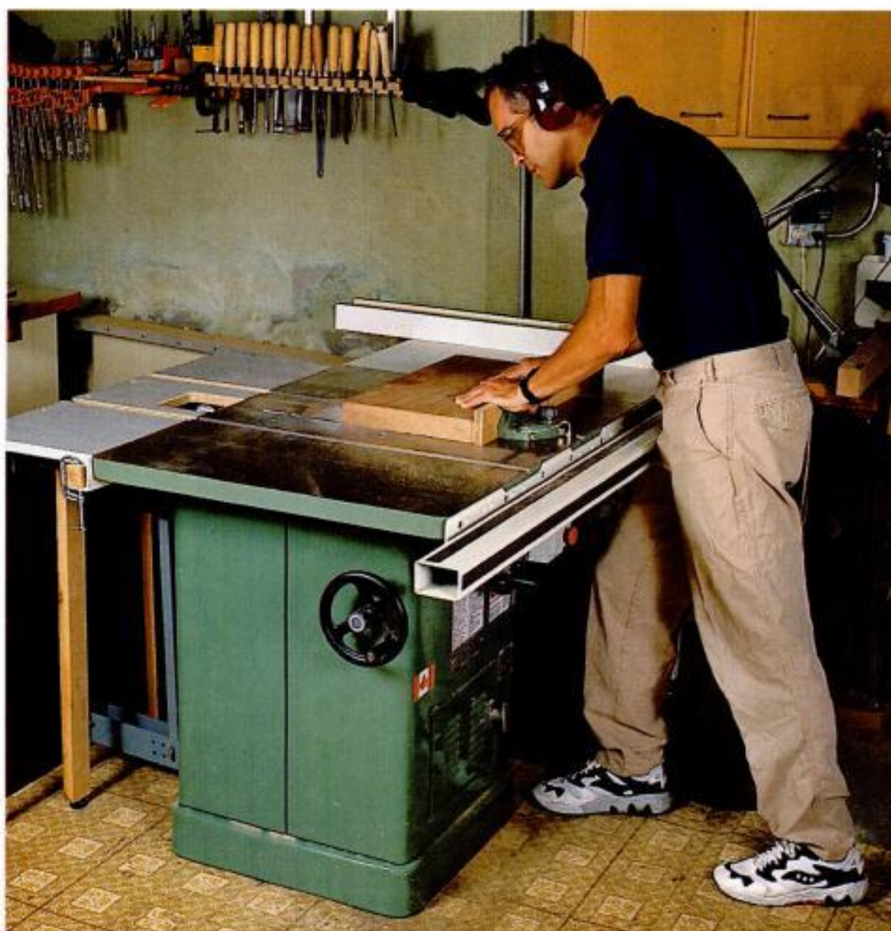
Shop workhorse. A tablesaw is the primary woodworking tool in many shops. No other machine can do so many jobs, from sizing material to cutting joints.
