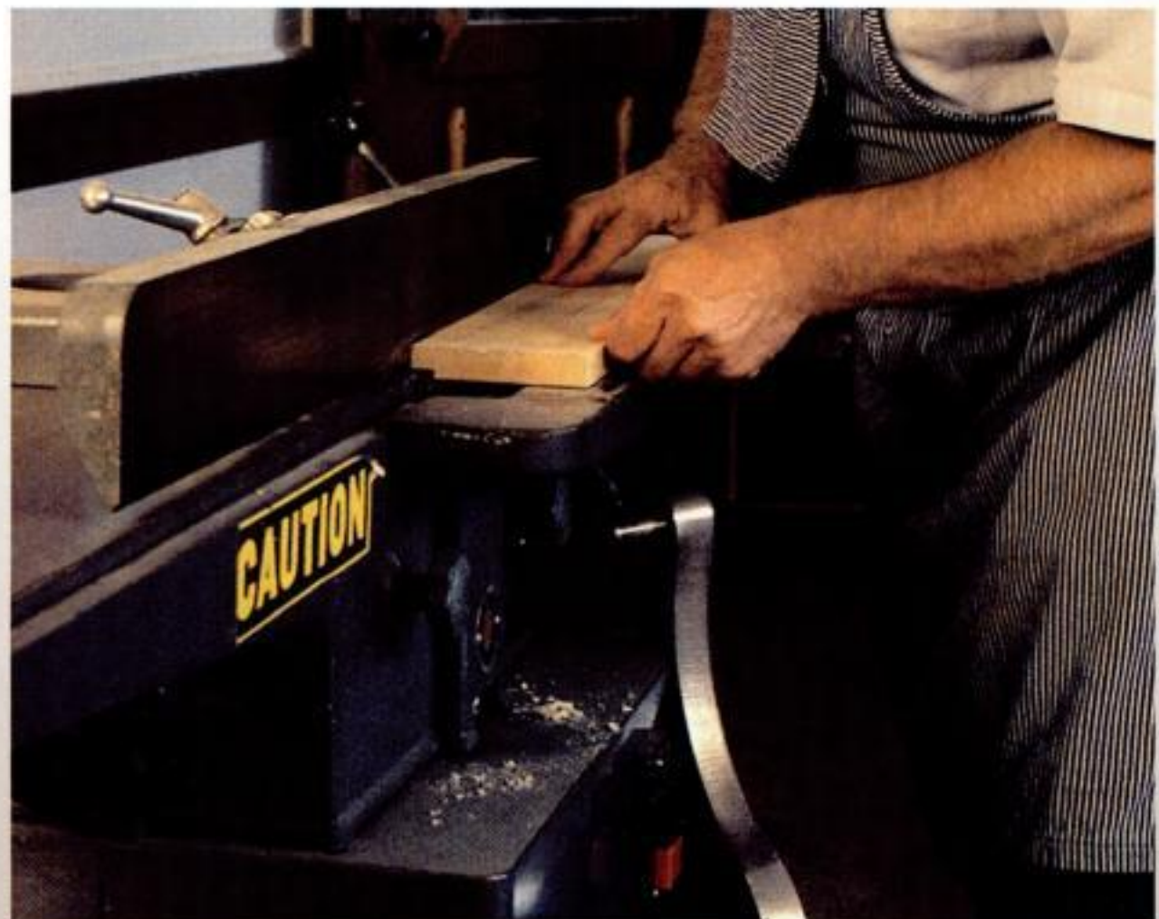
A ledge for rabbets. On a jointer equipped with a rabbeting ledge, you can quickly and easily mill rabbets and tongues.
