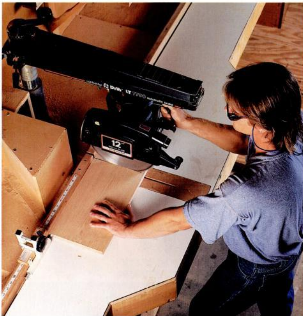
Radial revolution. The radial-arm saw is ideal for crosscutting or mitering large stock. It can also be a versatile tool for dimensioning and shaping wood.
