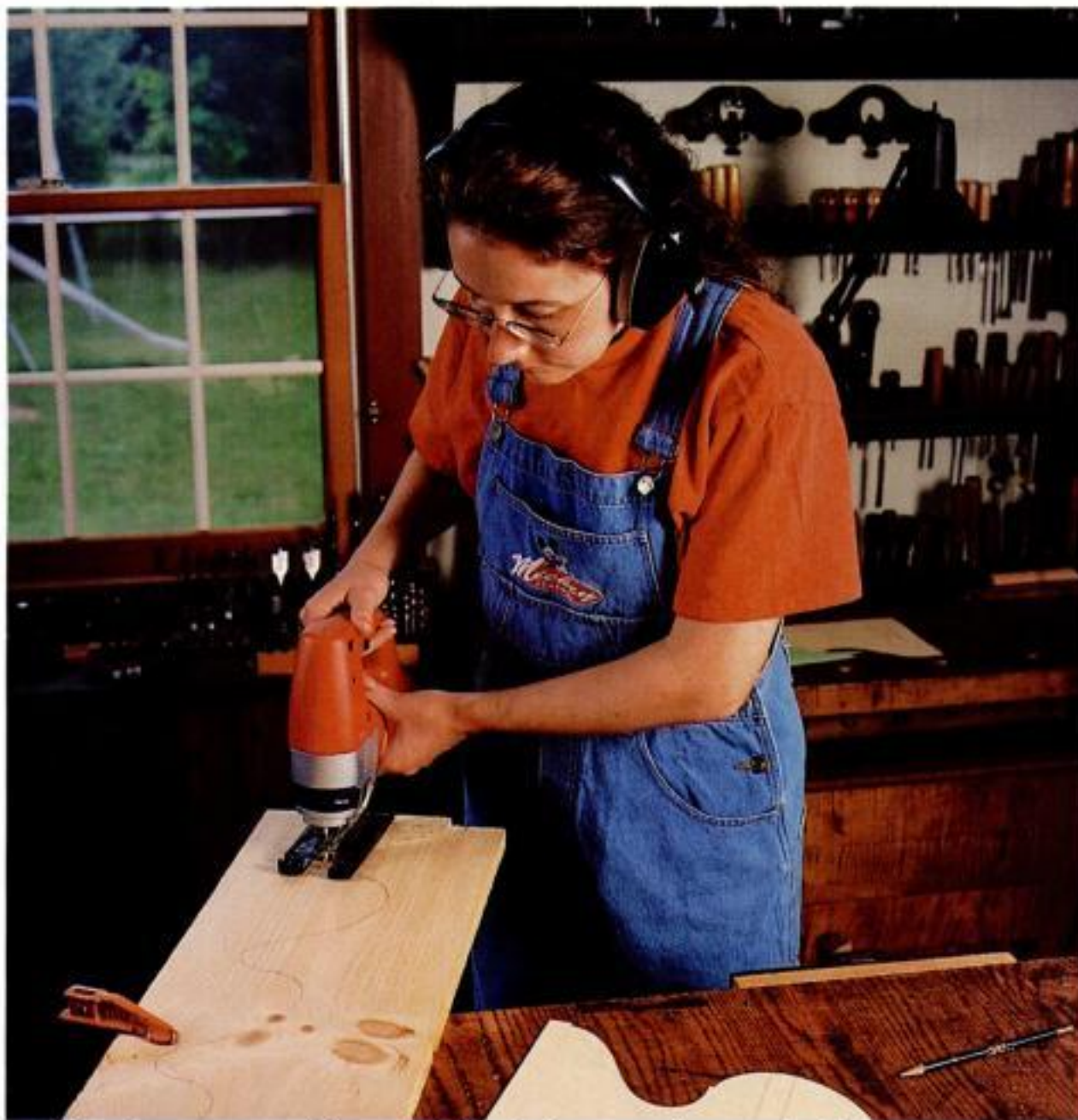
Making the cut. Portability, and the ability to make smooth, fast cuts in wood and other materials make the jigsaw a workshop and jobsite workhorse.
