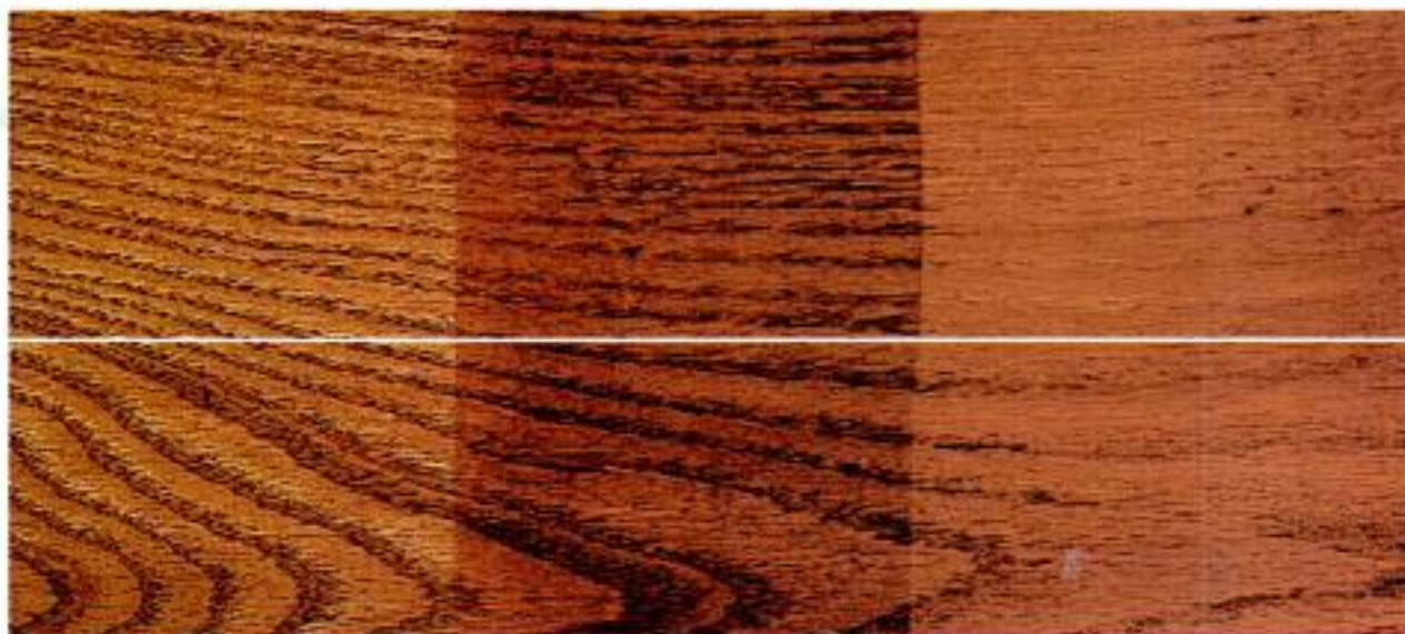
Dyes vs. pigments. Dye stain (top right) colors oak evenly, while pigment stain (top left) collects in the pores, emphasizing the grain. The overlapped section at center shows the combined effect. A coat of finish (bottom half of sample) saturates the color.
