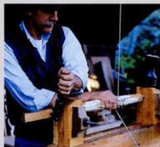
C: Adjusting the centers. Weber holds the spindle in place while screwing in the centers.
