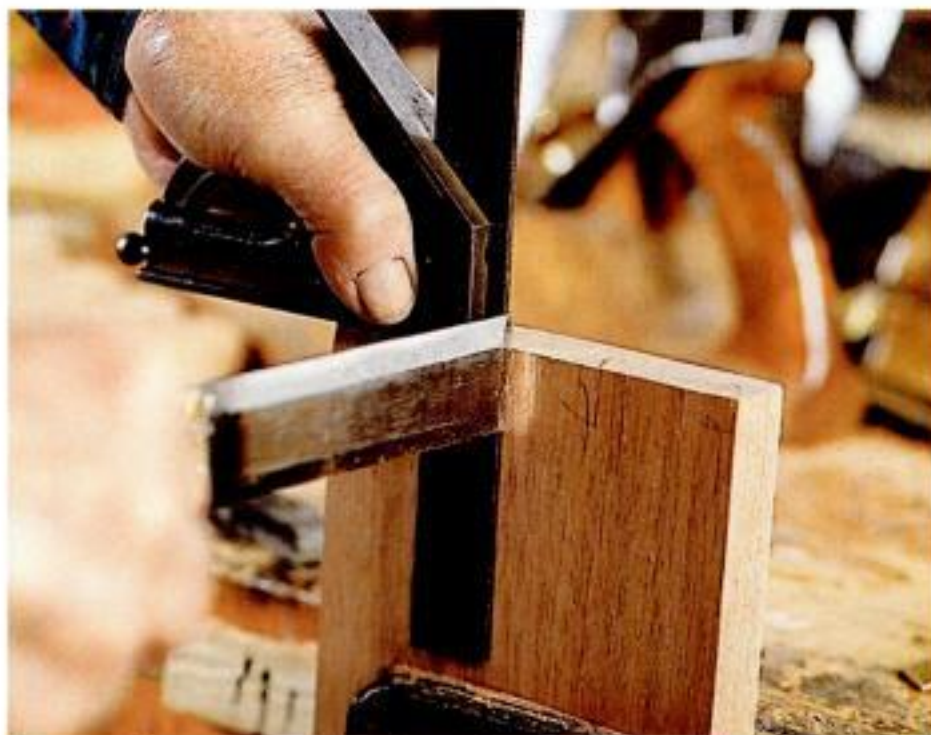
Square down. He completes the pin layout by extending his end-grain marks down to the baseline, using a square and a chisel.
