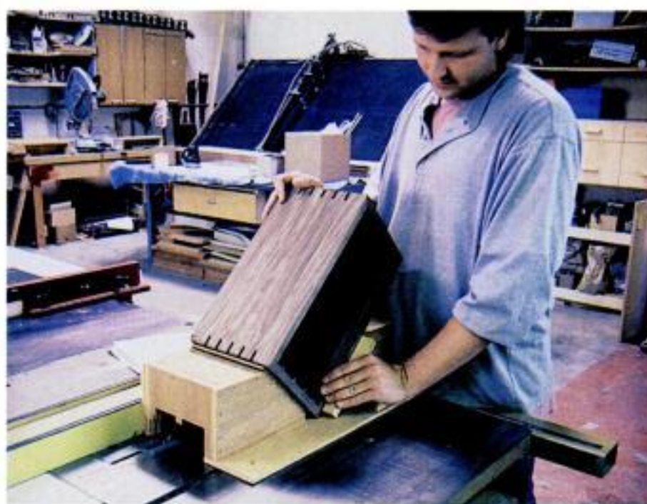
Grooves for keys. Use a carriage jig to hold the case corners at 45° when you're cutting grooves for keys.
