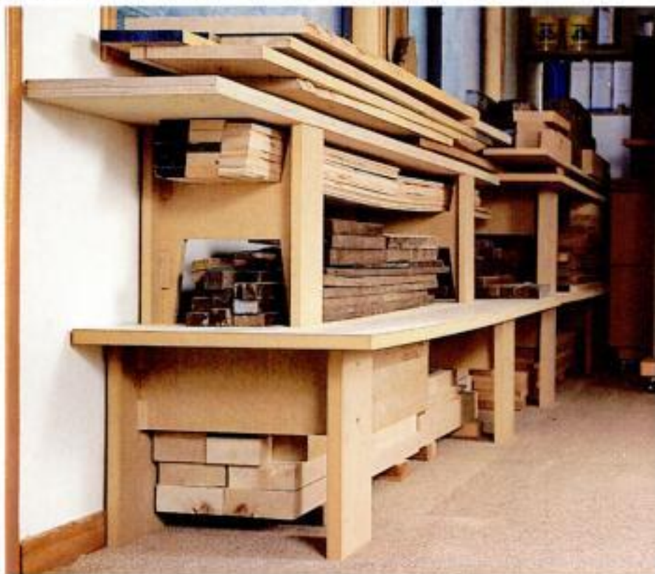
Storage modules that stack. Yeung Chan uses leg-and-beam assemblies to create platforms for storing lumber.
