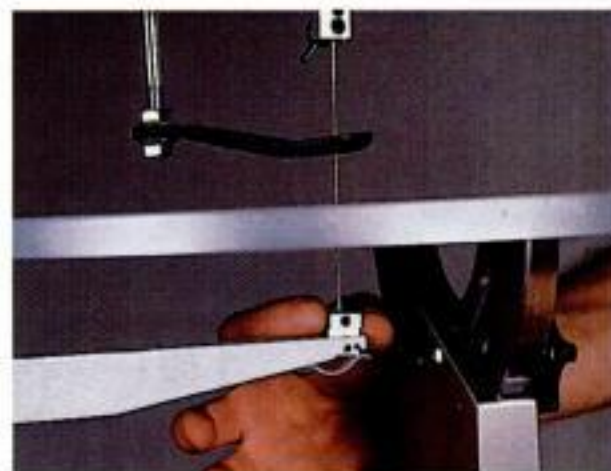
Aggressive or fine cuts. You can position the blade holder two ways on the RBI, for fine or aggressive cuts.
