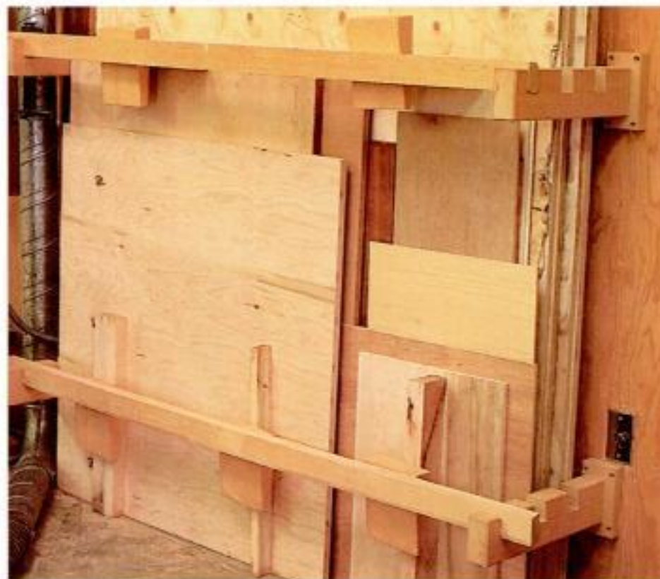
Flat storage for panel offcuts. This rack wedges plywood offcuts tightly together to keep them from warping.
