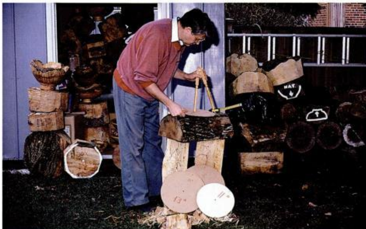
Laying out blanks. Cardboard templates make a quick size reference for laying out blanks in a log. Newlove uses a shop-made compass to establish the blank's rough diameter.
