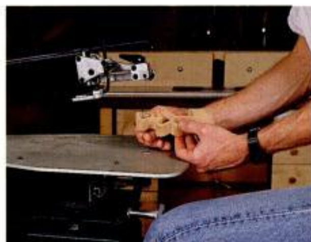
Easy inside cuts. An optional foot pedal on the Excalibur raises the upper arm for easier blade insertion.
