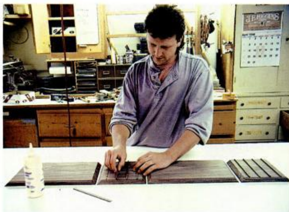
Grooves for runners. Groove the sides and install the drawer runners before assembling the case.
