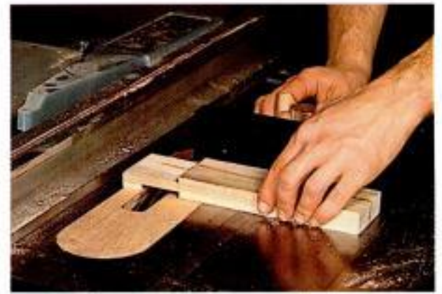
Multiple passes. Using a dado cutter, you cut tenon cheeks and shoulders with a series of overlapping cuts.
