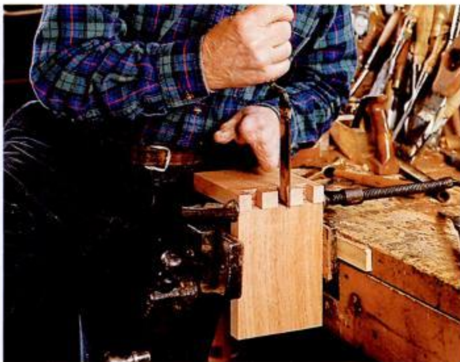
Transfer the tails. Pierce uses the tail piece as a template when laying out the pins. He presses down with a sharp chisel or plane iron.
