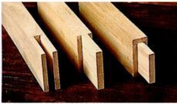
Not just tenons. You can cut tenons (right) and both halves of a bridle joint (left) with the author's jig.
