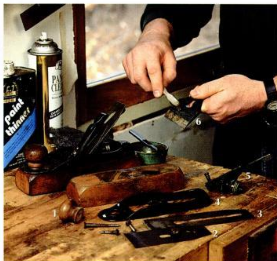
Take it apart. Clean the metal parts with an old toothbrush and some mineral spirits. Take care not to remove any original enamel. Parts of the plane include: 1 knob; 2 cap iron; 3 cutter or iron; 4 top casting; 5 frog, with thumbscrew and adjustment lever; and 6 lever cap.
