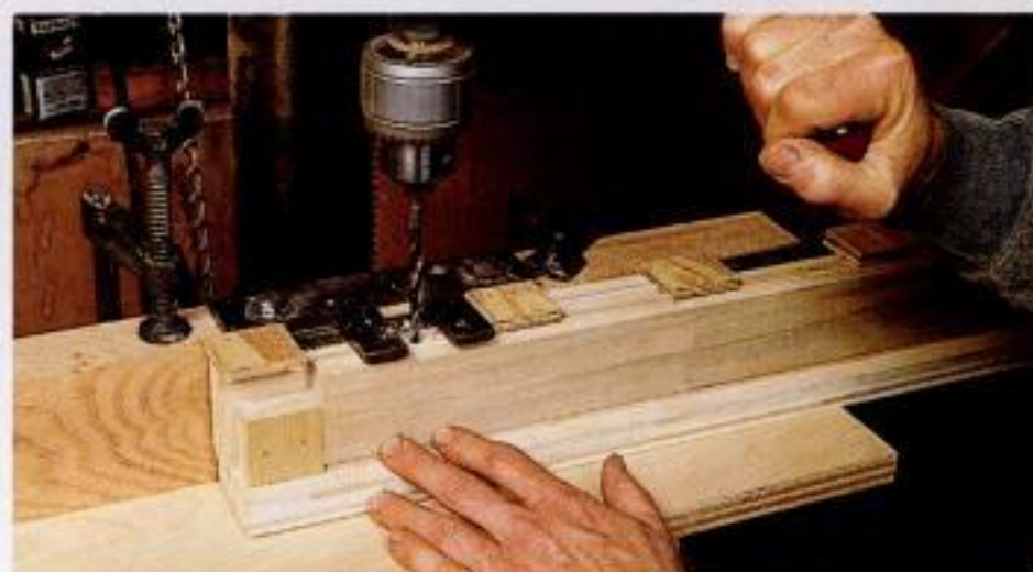
Foolproof mortise spacing. McCarthy's jig guarantees accurate mortises, time after time. You can use the jig on a drill press or a hollow-chisel mortiser.
