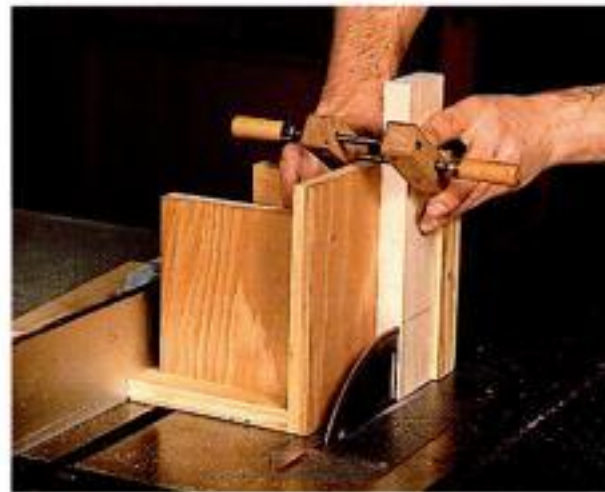
Cheek cuts. This jig cuts clean cheeks in a single pass. Set the blade height just below the shoulder line.
