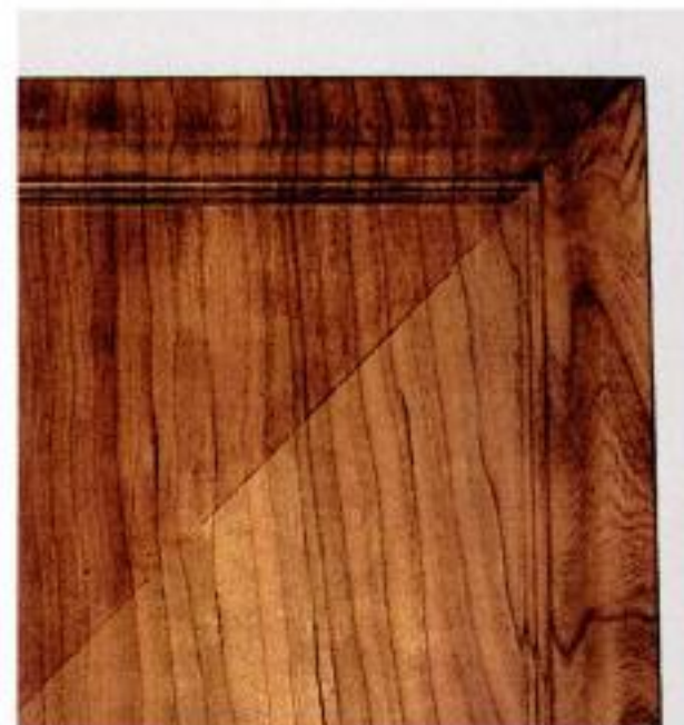
Glazed vs. unglazed. A coat of glaze (top left) adds depth and richness to this finished cherry panel.
