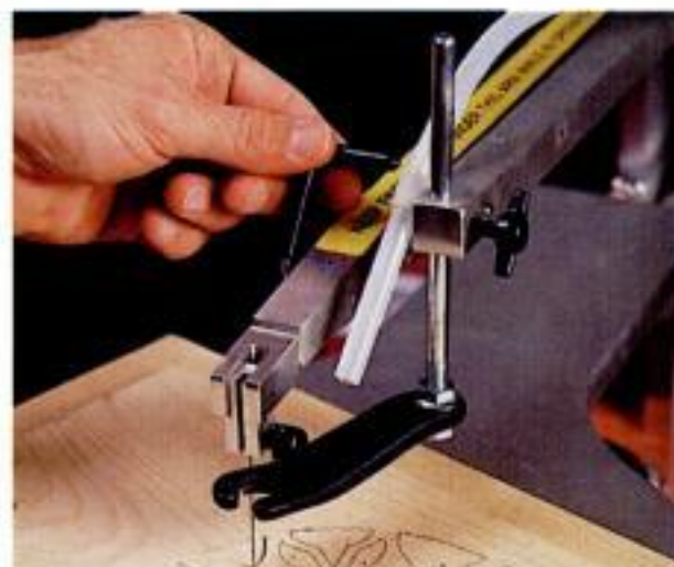
Fast blade tension. The RBI's quick-release device lets you tighten the blade with the flip of a lever.
