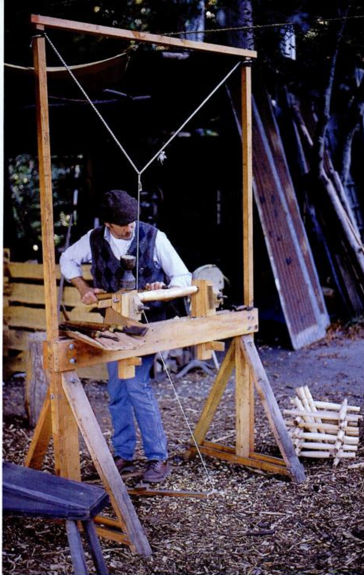
Pedal power. Turning chair parts is good exercise when you have a foot-powered lathe. On Weber's lathe, a bungee cord keeps the drive cord taut.
