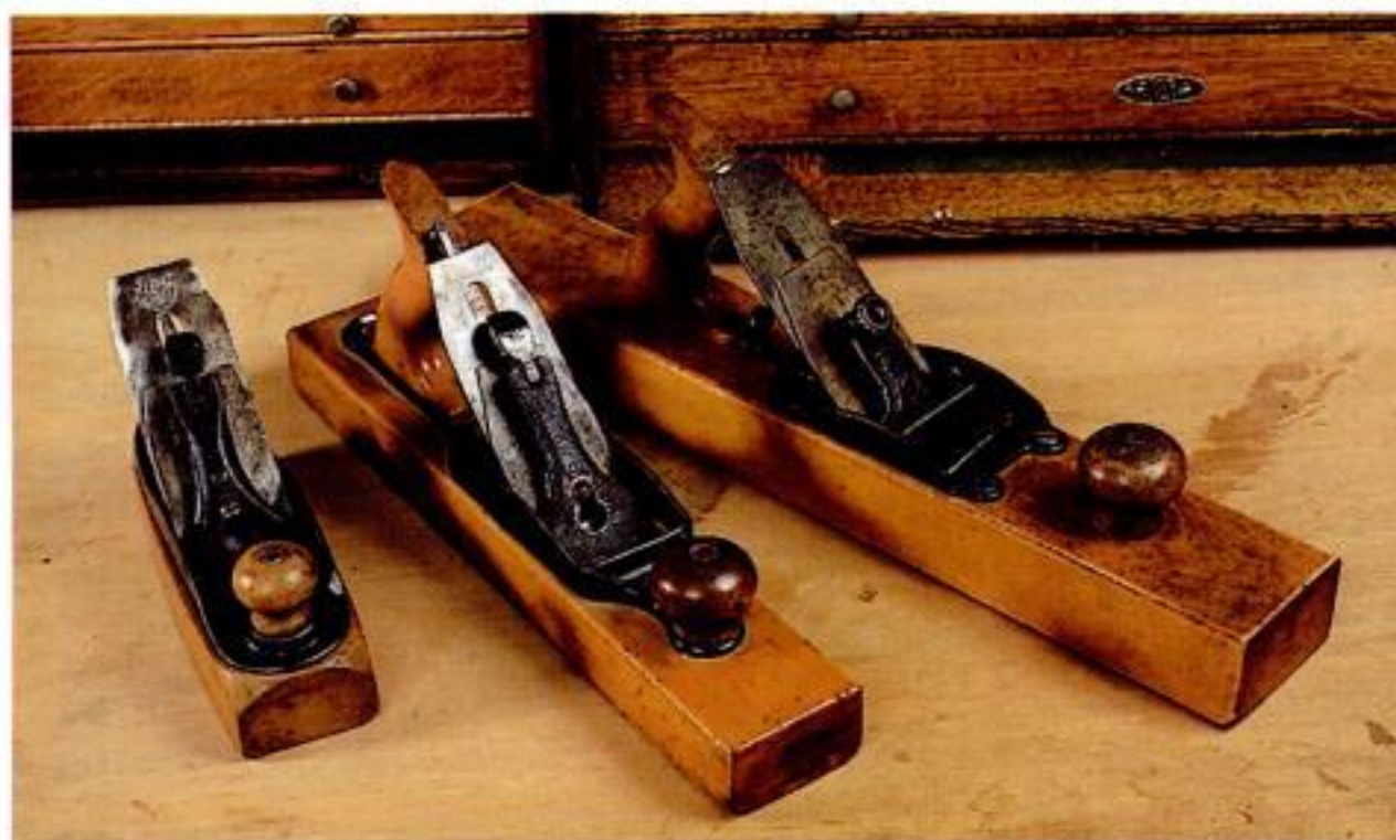
Benchful of beauties. The author's transitional collection includes (from left): a Bailey-type smooth plane made by the Ohio Tool Co., a Stanley Bailey No. 26 jack plane, and a No. 129 "Liberty Bell" fore plane.
