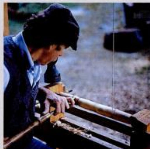
D: Making the cut. He moves the blade into the work each time he presses the foot treadle.
