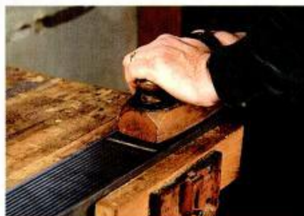
Flattening the sole. Stevens clamps a metal jointer plane upside down in his bench vise, to flatten the wooden sole of a transitional plane.
