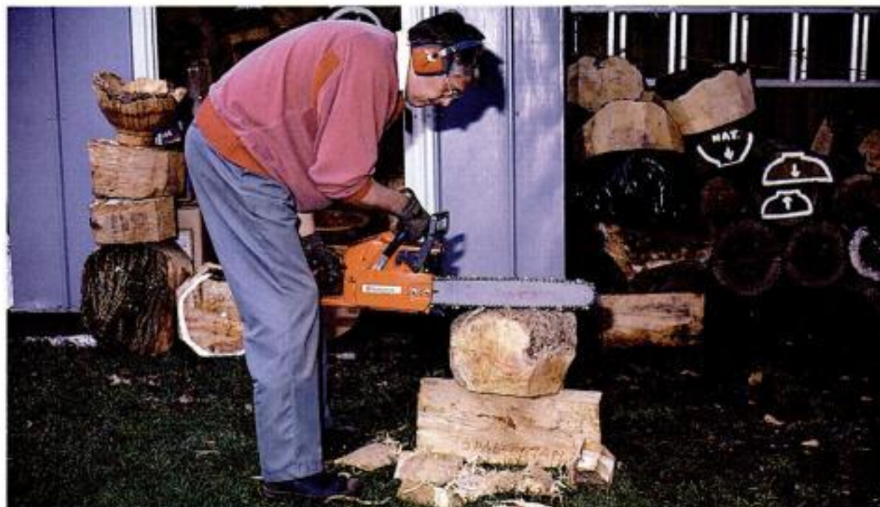
Sawing down to size. Newlove saws to a chalkline to remove excess stock. The stump makes a handy bench for trimming bowl blanks.
