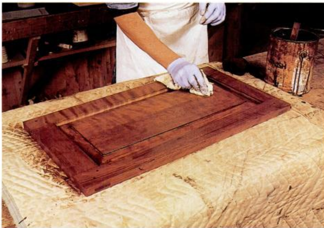
Wipe on some history. Burak's multi-step finish mimics the look of a well-worn antique. Here, he uses a rag to control the effect of a glazing coat.
