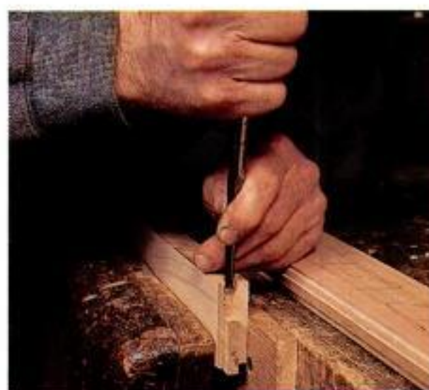
Trimming a tenon. The author chisels a rail tenon to finished width.
