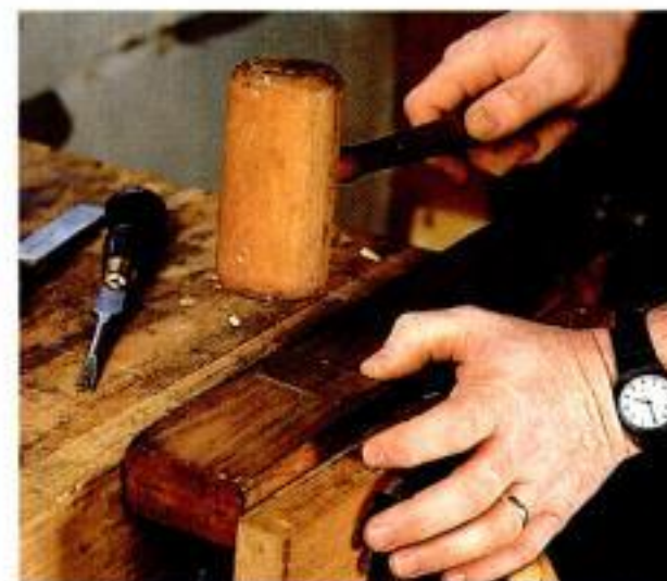
Tap in the patch. The installed patch should stand proud of the sole so it can be planed or scraped flush.
