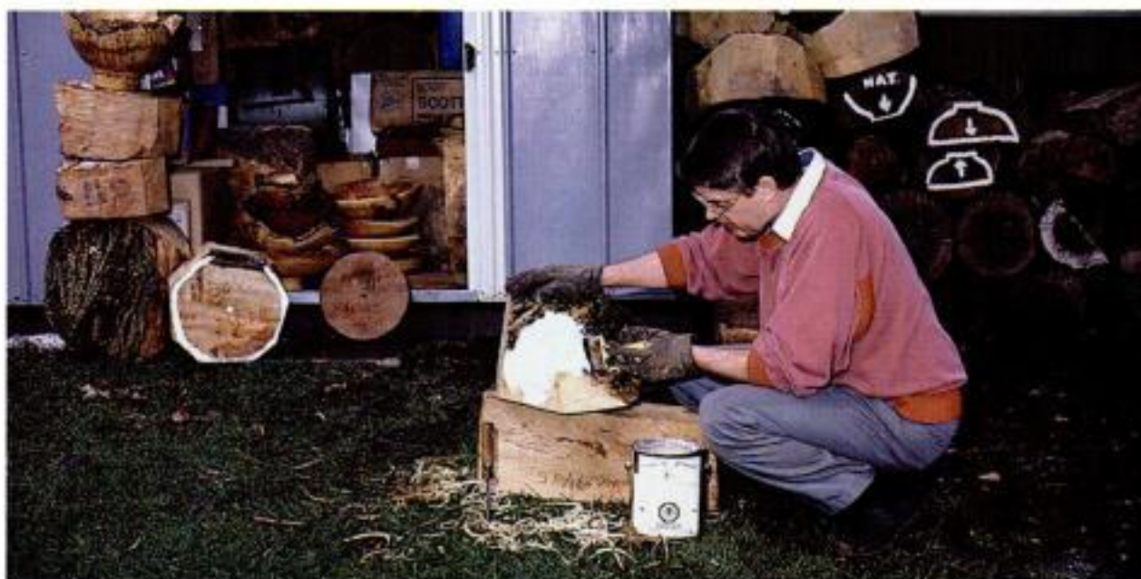
Sealing before storage. To control moisture loss and prevent checking, Newlove seals the cut surfaces before long-term storage.
