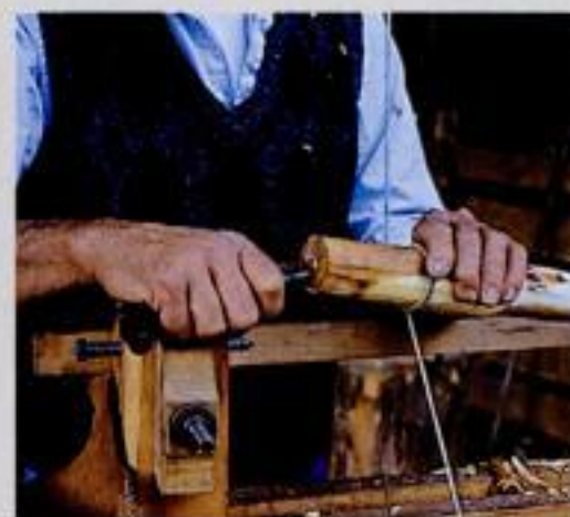
A: Making center holes. Weber uses a gimlet to poke holes for the lag-screw centers.
