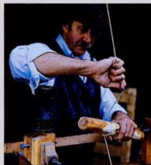
B: Wrapping the spindle. He wraps a spindle twice with the drive cord.
