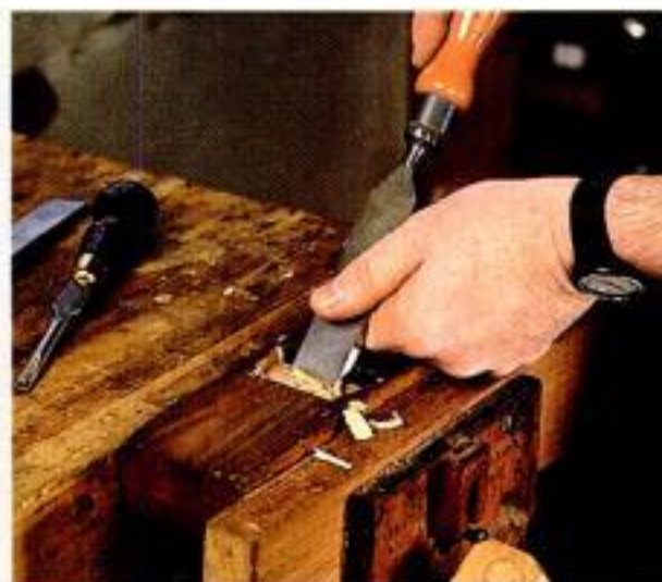
Chisel out the waste. Excavate the area inside the scribe lines with a sharp chisel.
