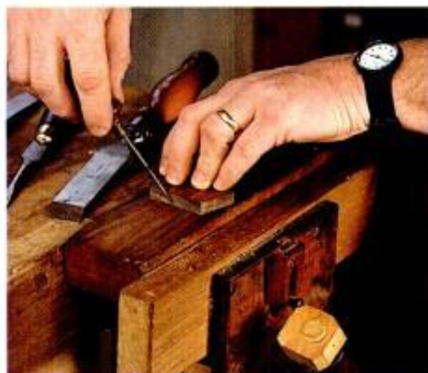
Scribe the sole. Outline the mortise by tracing around the patch piece with a sharp knife.
