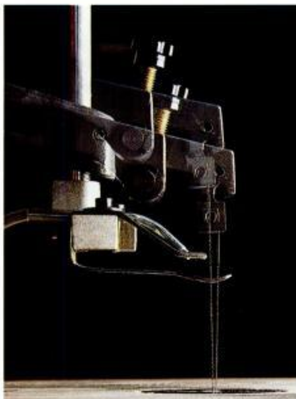
C-arm action. The C-arm design on the Craftsman moves the blade in a small arc, beveling the edge of the workpiece slightly.
