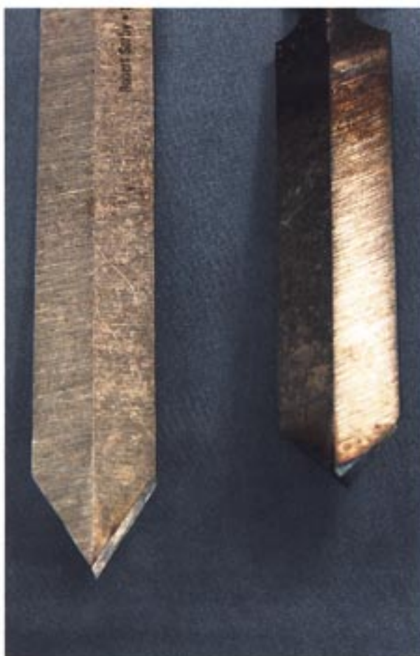
The diamond parting tool on the right is too blunt. The bevels need to be reground (lengthened) for the tool to be used properly.
