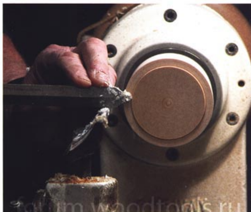
With the handle held too high, the wood is being scraped, not cut, with the tool.
