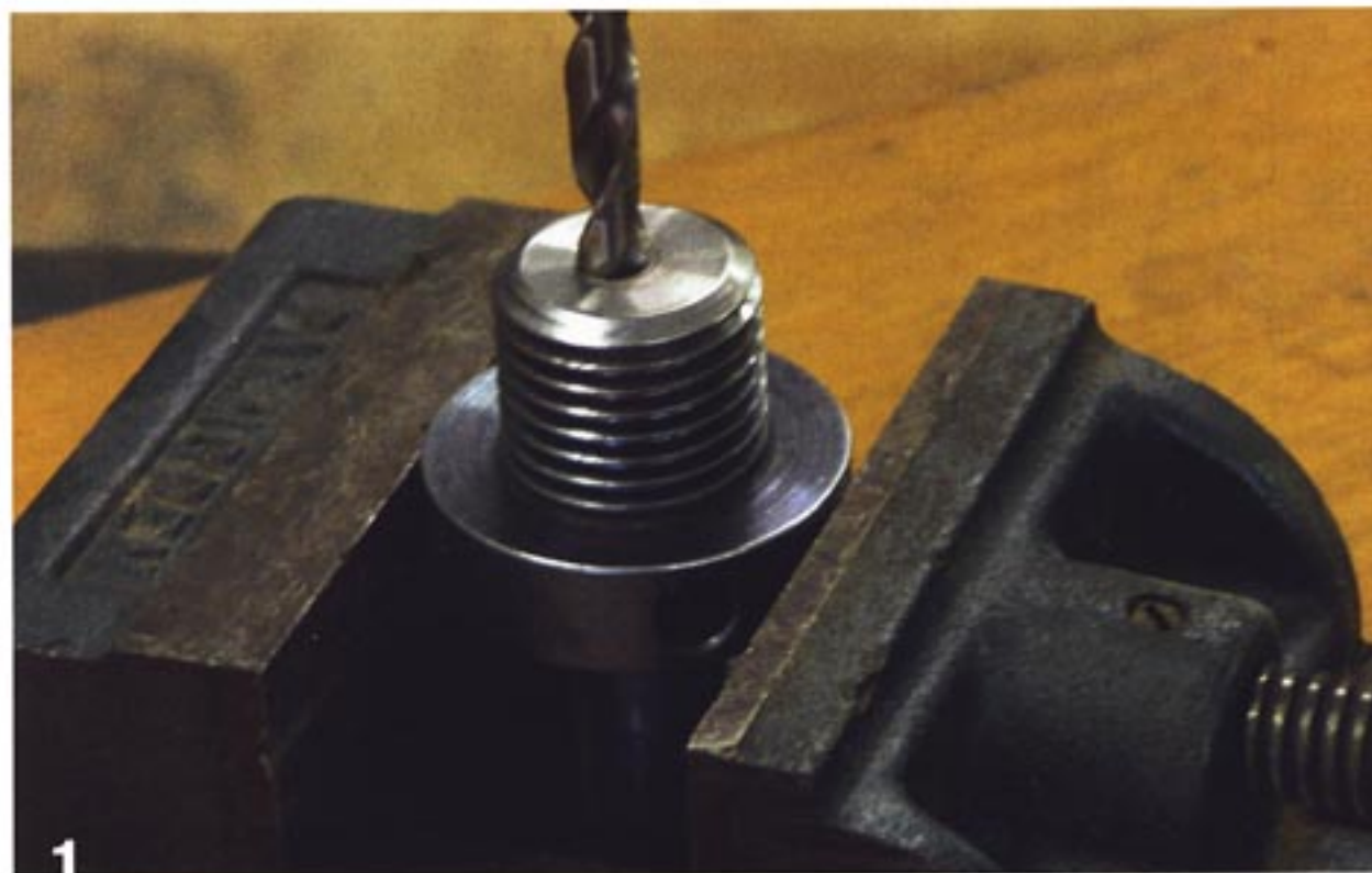
Drilling the first hole into the carving stand.
