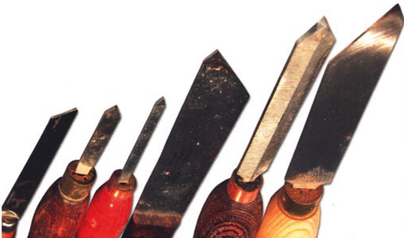
Shown here is an assortment of the author's parting tools. (Left to right) Nick Cook tool with a flute (Sorby), standard diamond parting tool (Sorby), standard thin-walled tool (no flute), shopmade mini tool, Bonnie Klein mini parting tool, and shopmade parting tool.
