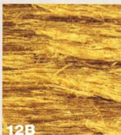
12B Resulting cut wood surface (100X).
