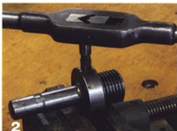
Threading the hole in the carving stand where the male pneumatic connector will attach.
