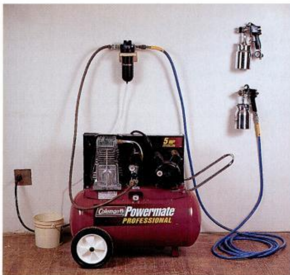
A compressor system. A compressor will power a conventional gun or an HVLP conversion gun. A coalescing filter (above the compressor) traps in-line oil, dirt and water.
