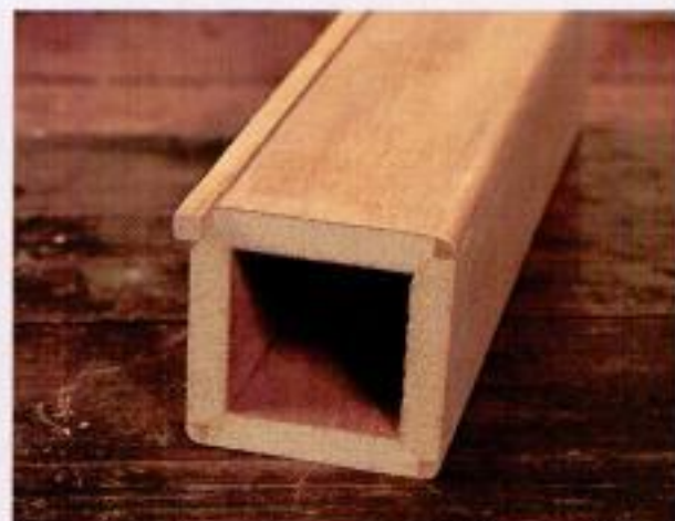
Protect the corner. A solid-wood corner insert protects man-made board from marring and lets you form a crisp edge at the corner.
