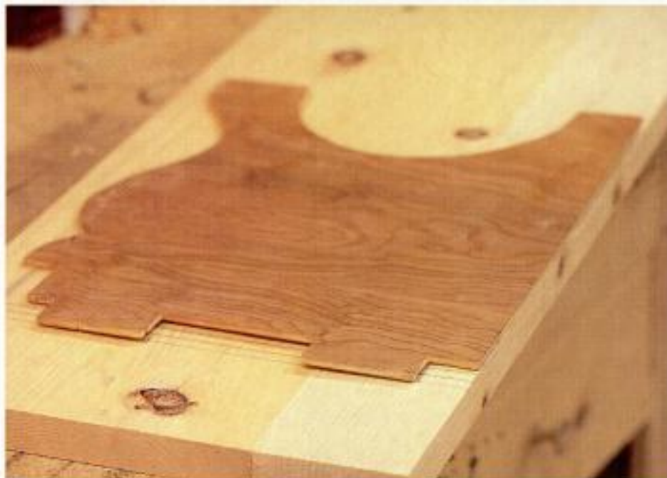
Seat mortises. Then use the template to mark mortises on the seat. Lay out the mortise widths across the centerlines.
