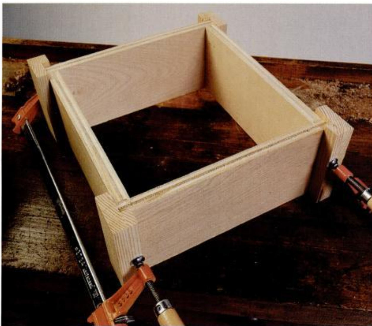
Clamping tongue-and-groove. Tongues and grooves work fine for corner joints. Shop-made blocks squeeze joints tight for glue-up.
