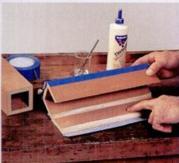
Glue it up. After brushing glue on the miters, roll up the box (left) and pull a strip of tape across the last corner (center). Remove the tape as soon as the glue sets.
