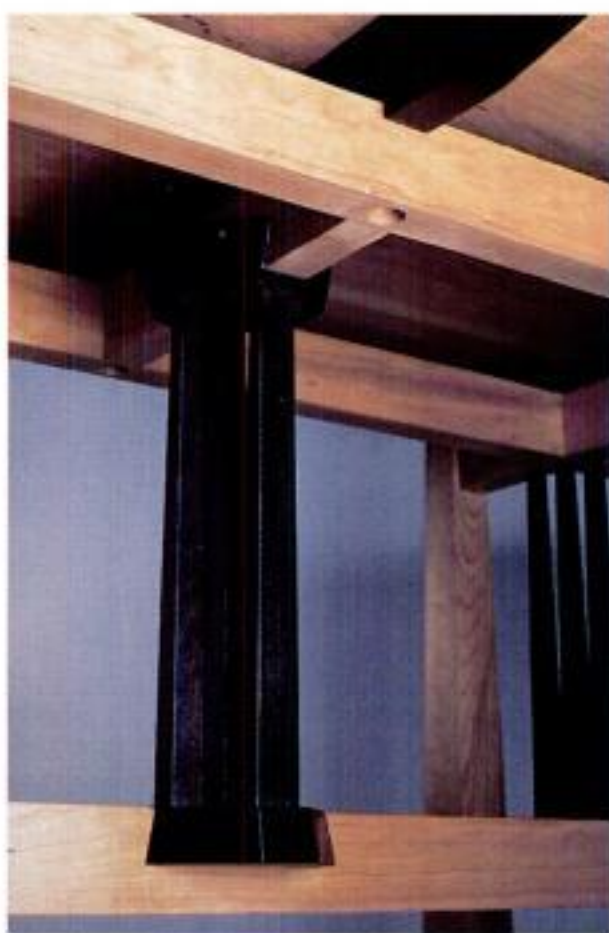
Center of attention. The centerpiece blocks fit into notches that are cut in the top and bottom stretchers. Screws hold the blocks in place.
