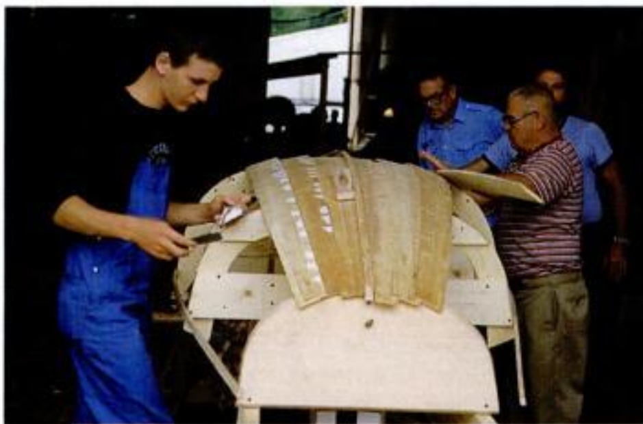
Whatever floats your boat. At left, Arques School students work on the bent-laminated hull of a traditional English boat. At right, David Gidmark pilots a 13-ft. Native American canoe made from a single sheet of birch bark.
