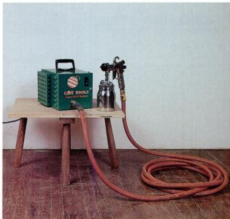
A turbine system. A turbine is more portable and often less expensive than a compressor system. It uses a turbine gun, usually sold as part of the system.
