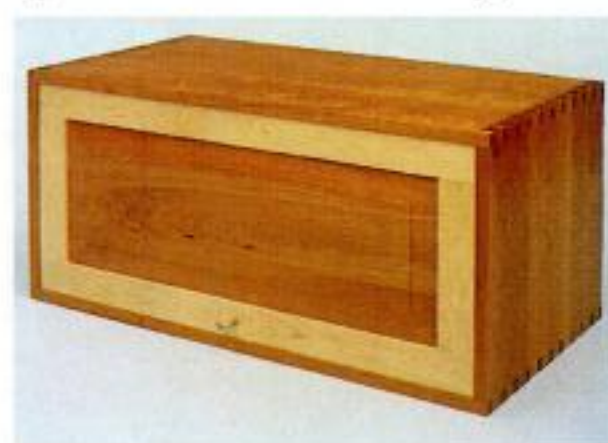
Basic but beautiful. Designed and built by Claire Fruitman, this cherry and maple tool chest fits under a workbench. A pull-out door locks in front of the drawers, keeping them in place when the chest is moved.
