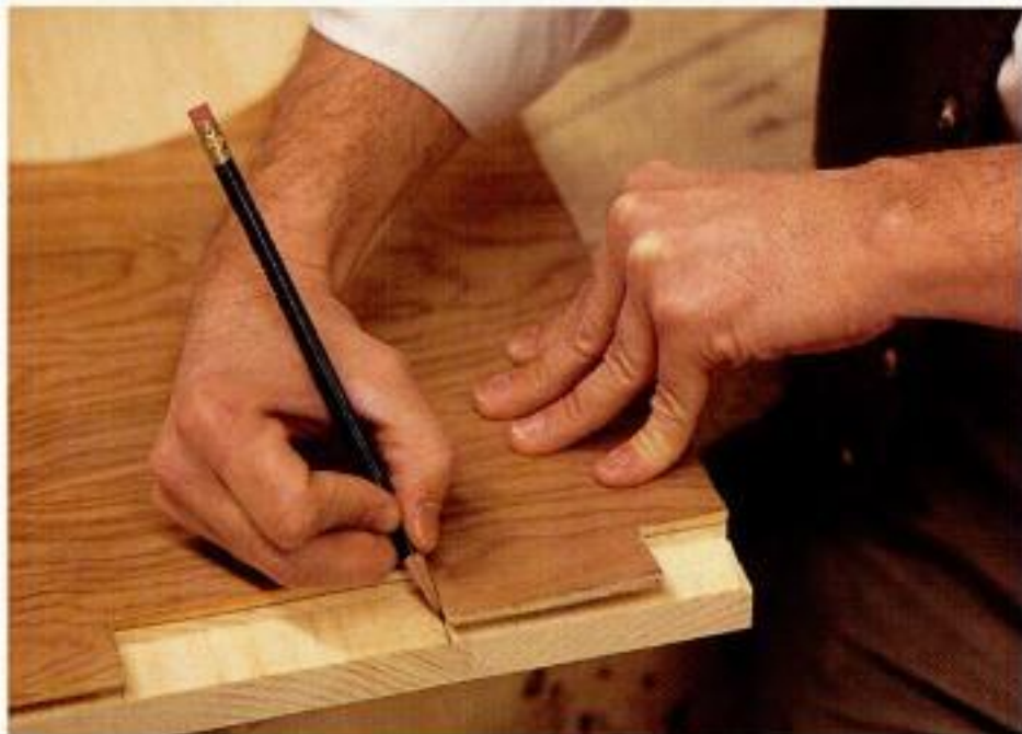
Legs and tenons. First use the plywood template to transfer the leg and tenon profile to your workpiece.
