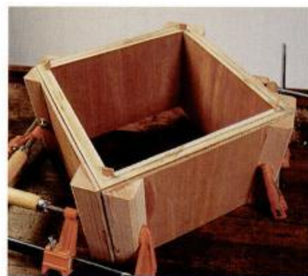
Clamping miters. Spline miters are another corner option. Clamp with pairs of 45° blocks.
