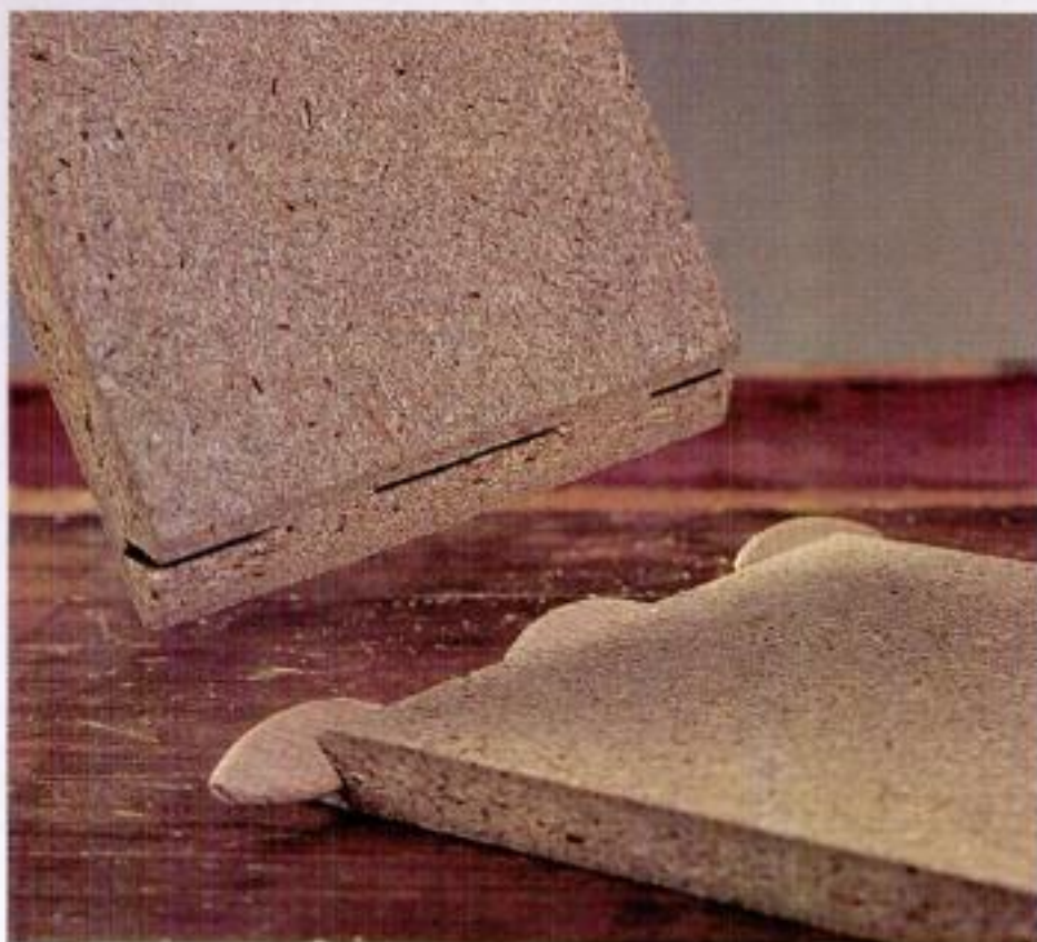
Mitered corners. Biscuits (left) and splines (right) make the simplest and strongest mitered corners in man-made board. To avoid weakening the board, splines are located near the inside face.
