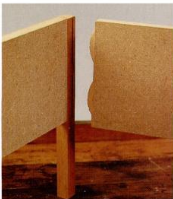
Solid-wood corner blocks. Biscuits and glue join solid-wood corner blocks to man-made panels for a strong joint. Here, the lengthened corner block will form a cabinet leg.
