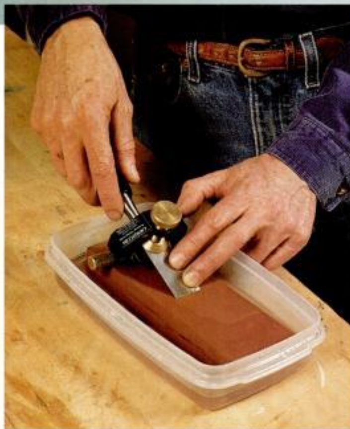
Guiding the edge. Using a honing guide, you can set and hold exact angles for honing both the bevel and microbevel.
