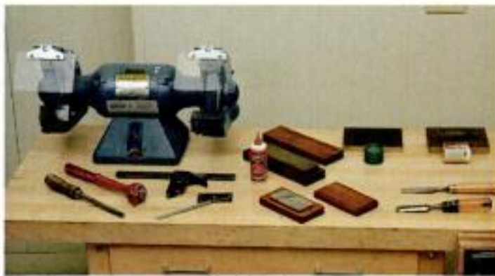
Strops, stones and wheels. Neptune's sharpening system begins with a Baldor grinder and ends with super-fine oilstones and leather strops.
