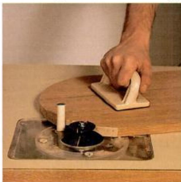
Around the curve. Horizontal bits can also raise curved panels. The stock pivots on the pin to control the cut. A back cutter relieves the panel back in the same pass.
