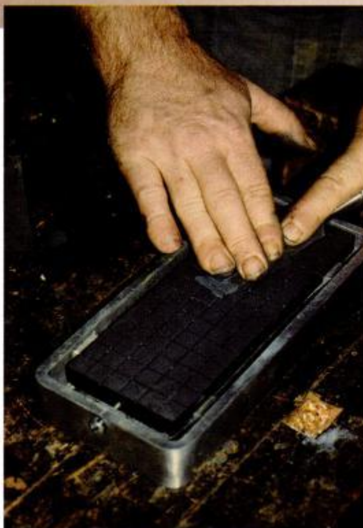
Lapping the back. Working on the coarse grooved plate, Biesanz applies even pressure over the back of the chisel to make it flat.
