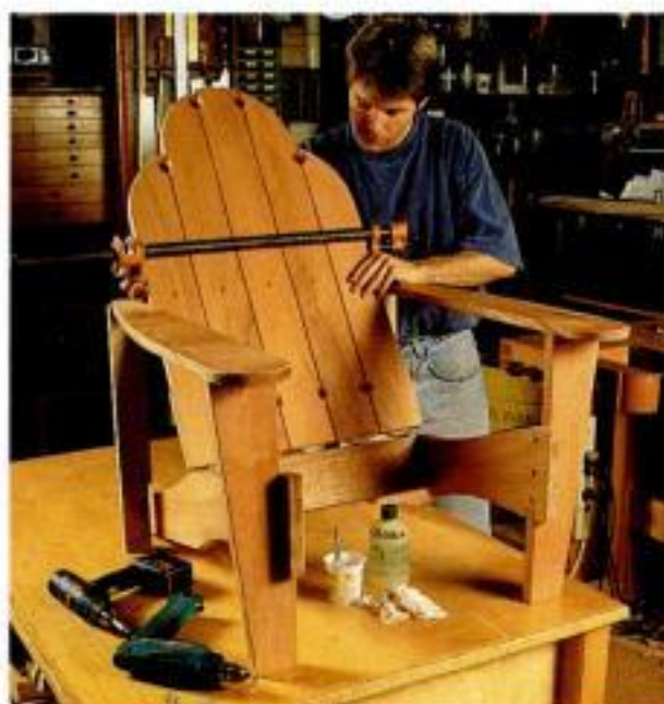
Gluing the back slats. Use a pipe clamp and spacers to hold the back slats in position while you join the slats to the stretcher.
