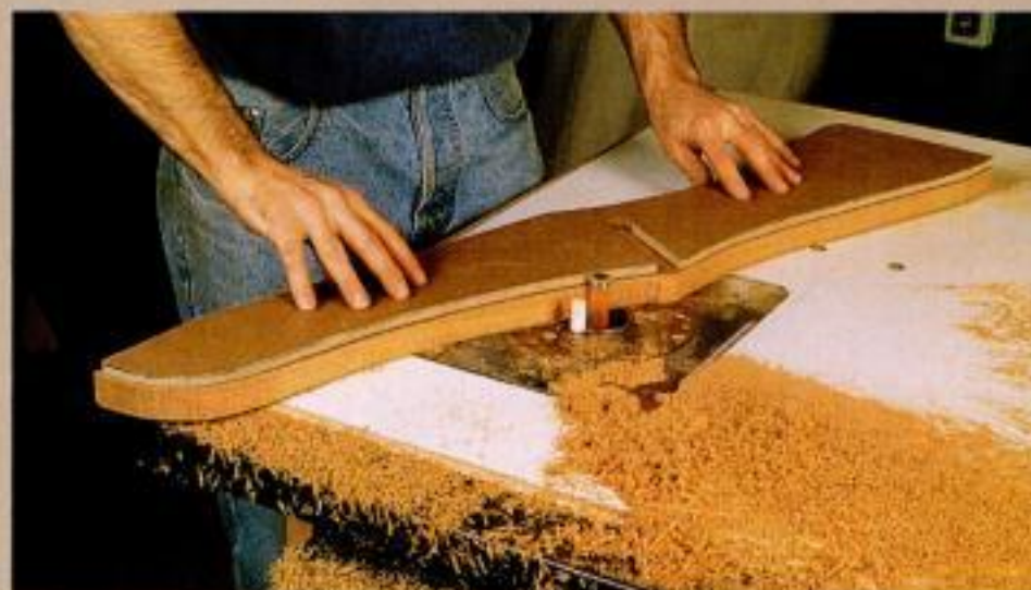
Routing a shape. Template rout an irregular shape by riding the template against the ball bearing of a flush-cutting bit. A starting pin in the router table allows the author to begin the cut safely.
