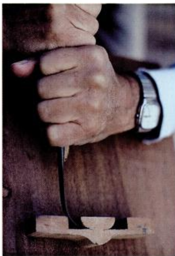
Handmade knives. Straight and curved blades are used for kerfing and decorative carving. Long handles allow for two-handed use.
