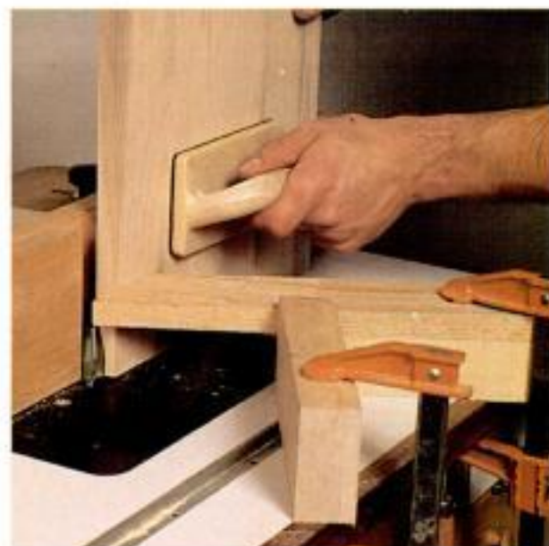
Raising on edge. Vertical bits enable small routers to make wide reveals. A feather board positioned above the bit holds the panel flat against the fence.
