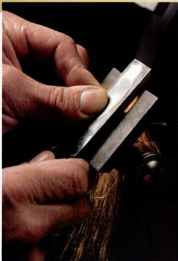
Wheel work. Hollow-grinding creates a concave bevel that minimizes the amount of metal you need to remove when honing.
