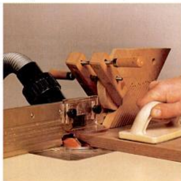
On the flat. Horizontal bits allow the panel to lie flat on the table. The panel edge runs against the fence or the bit's bearing. A feather board helps to hold the panel down.
