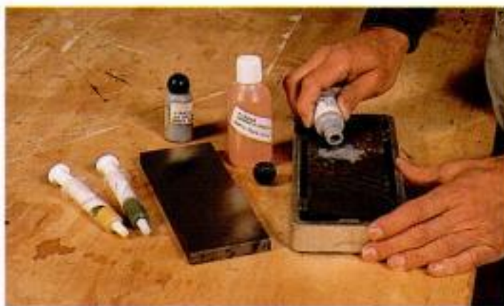
Plates, powder and diamond paste. Charging the flat iron plates with abrasives makes them work like sharpening stones. The syringes hold diamond paste; silicon carbide powder comes in vials.
