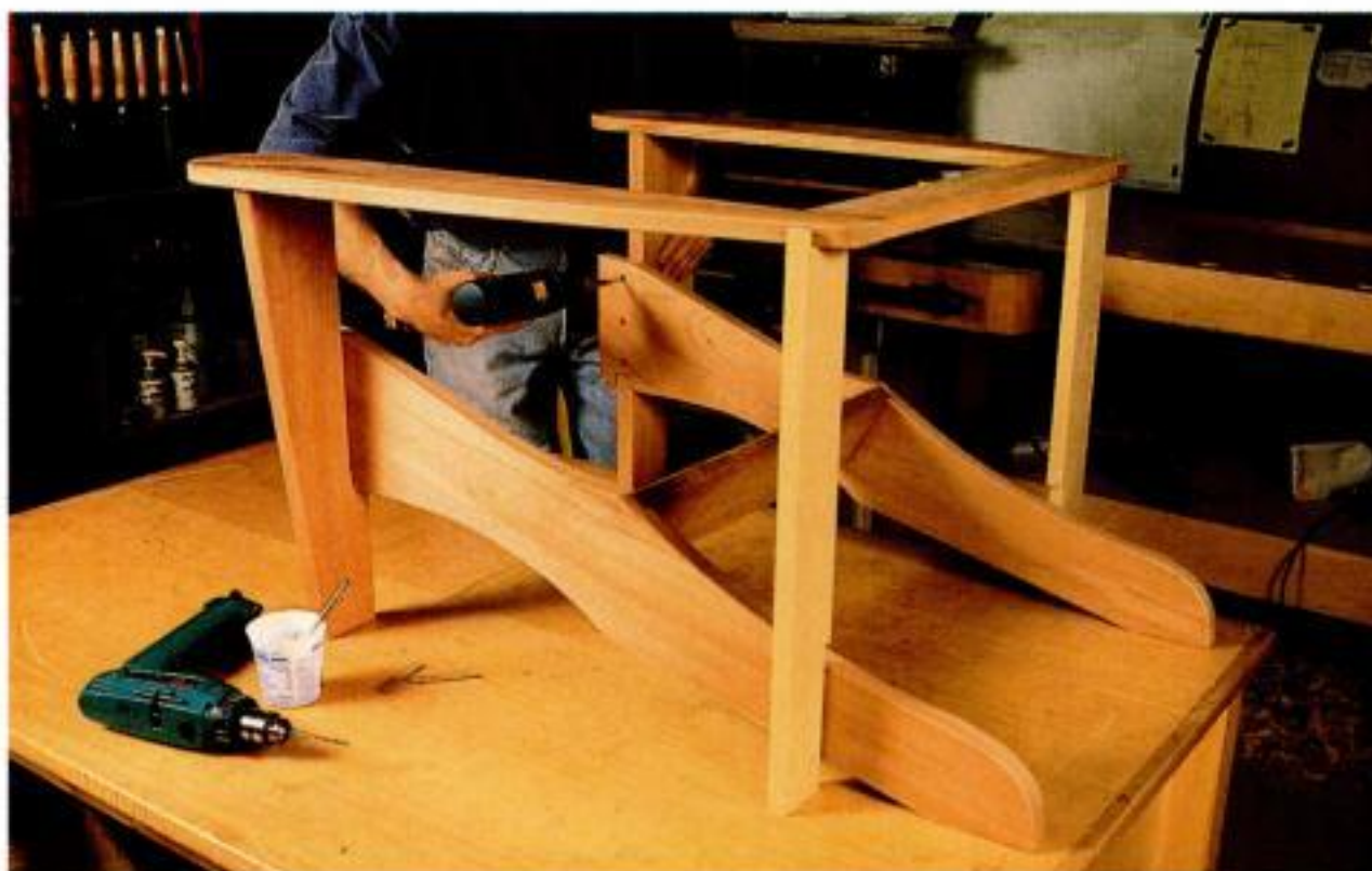
Supporting the assembly. Bandsaw two scrap sticks to support the backs of the arms level with the fronts of the arms during assembly.
