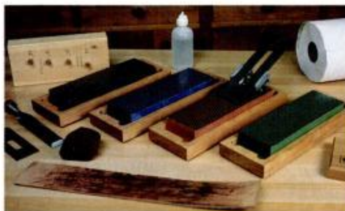
Four stones and a strop. Diamond stones are color coded by grit. A water bottle, paper towels and a bevel-setting jig complete the kit.
