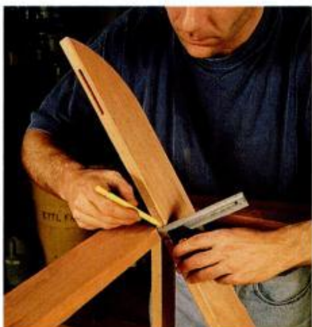
Marking for screw holes. Determine the location of the screw hole in the back slat by holding an adjustable square against the back rail.
