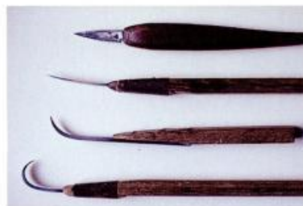
Handmade knives. Straight and curved blades are used for kerfing and decorative carving. Long handles allow for two-handed use.
