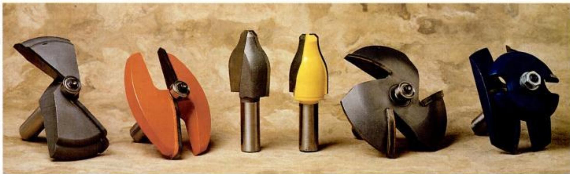
Raised-panel bit list. Left to right: standard horizontal, anti-kickback horizontal, standard vertical, anti-kickback vertical, three-wing horizontal, horizontal with back cutter.
