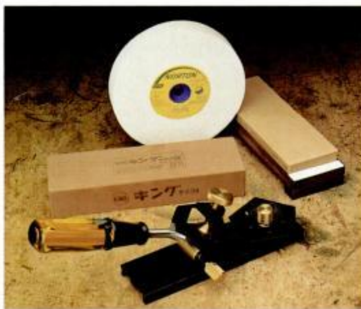
Three-stone system. Lee uses an 80-grit Norton wheel to hollow-grind the bevel. For flattening and honing, he relies on 800- and 6,000-grit waterstones.
