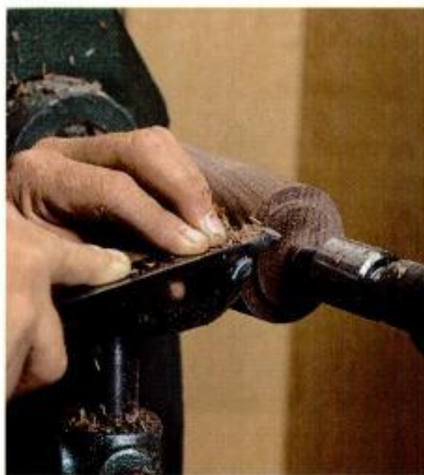
Start with the blank. With the blank turning between centers (left), cut a shoulder at each end of the blank to fit in a self-centering chuck. At right, Raffan uses a parting tool to cut the base of the box free of its lid.
