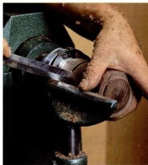
Start with the blank. With the blank turning between centers (left), cut a shoulder at each end of the blank to fit in a self-centering chuck. At right, Raffan uses a parting tool to cut the base of the box free of its lid.
