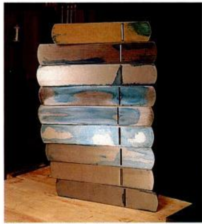
Test of sole. Right out of the box, plane soles were tested for flatness on a surfacing plate (left). At right, blue dye shows where the sole contacted the plate. The more blue, the flatter the sole. From top: AMT, Anant, new Stanley Bailey, vintage Stanley Bed Rock, vintage Stanley Bailey, Record, Footprint, Great Neck, Stanley Contractor.
