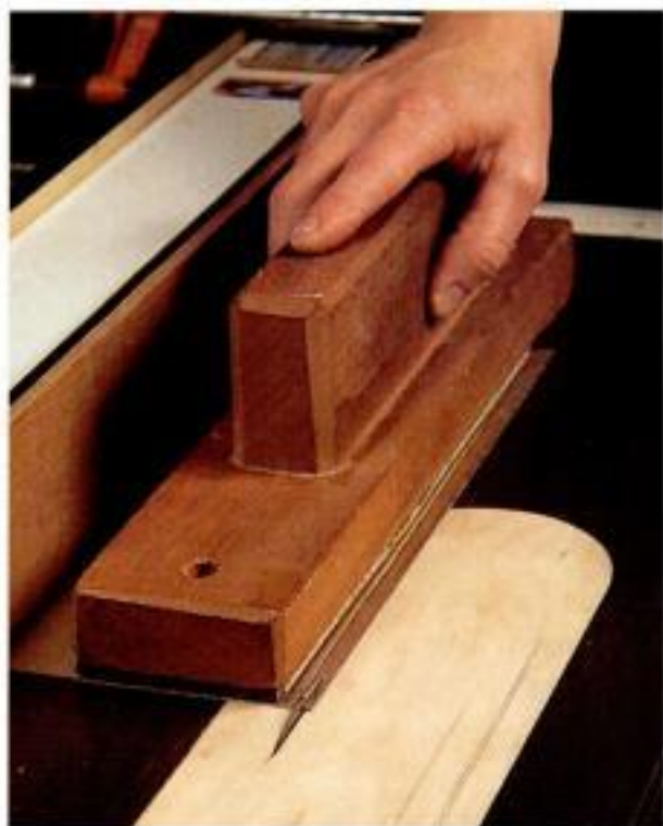
Cutting metal strips. The author rips a thin inlay strip from a sheet of pewter, using a metal-cutting blade. A zero-clearance throat plate, an auxiliary fence and a push stick make for safe, accurate cuts.
