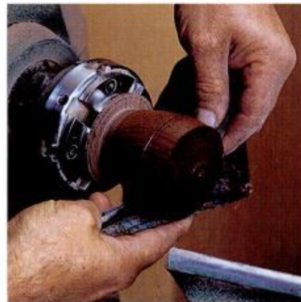
Turning base and lid together. With the lid fit tightly on the base, turn the final detail on the top of the lid (left). Form the beads on both sides of the opening with a skew (center). Buff on a beeswax finish after sanding the profiled sides (right).
