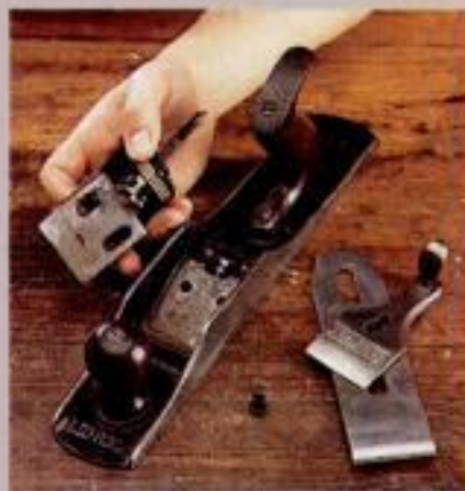
Back to Bed Rock. The flat-milled frog on this old Stanley Bed Rock plane beds itself against a milled ramp in the sole for solid, chatterless performance.
