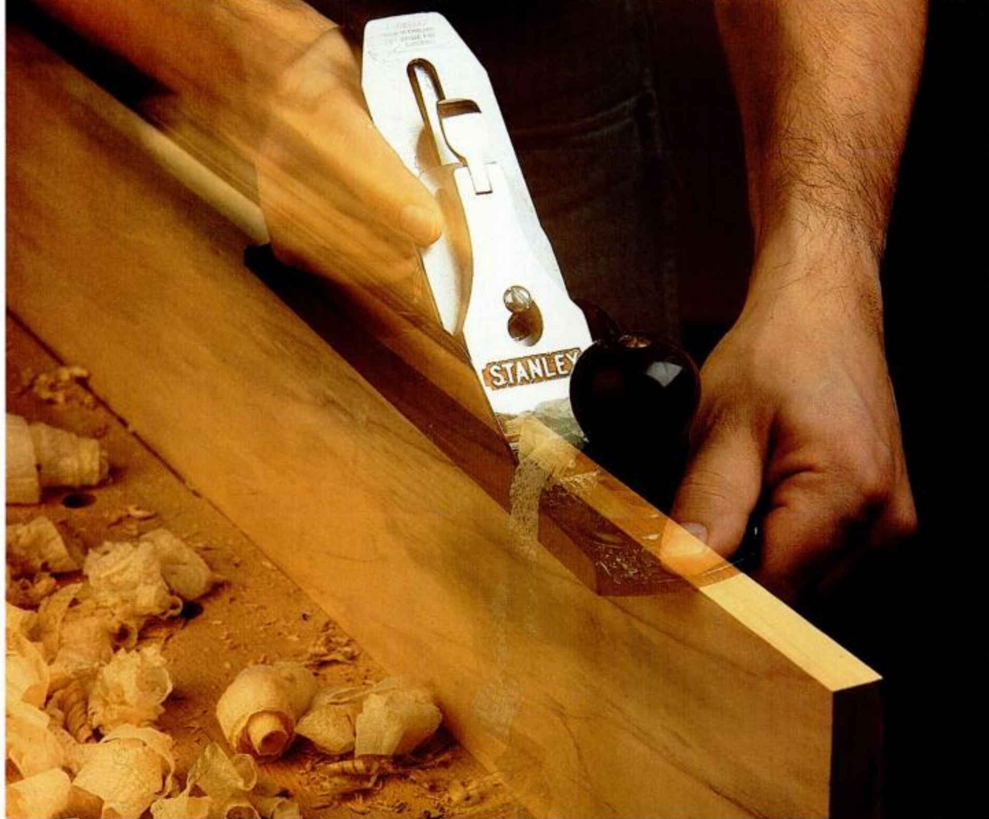
Plane portrait. The do-it-all jack plane is equally useful for jointing edges and general smoothing.
