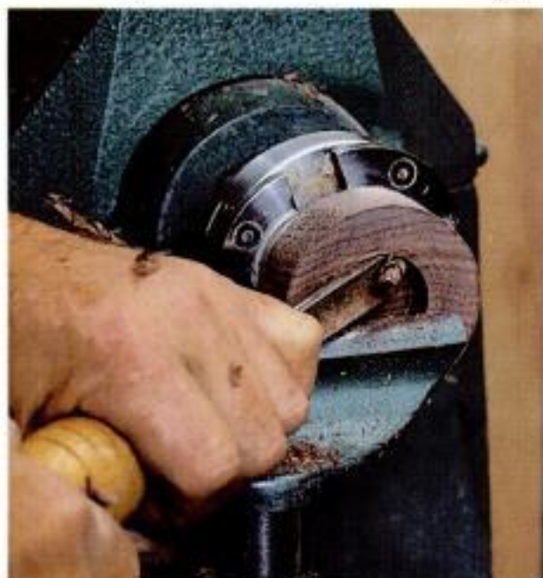
Lid work. Start by "back hollowing" the lid with a 1/2-in. gouge (left). Cut the flange that will fit over the base with a square-end scraper, making sure to make the flange parallel to the turning axis (center). After turning and sanding the inside of the lid, apply a coat of beeswax and buff it out (right).
