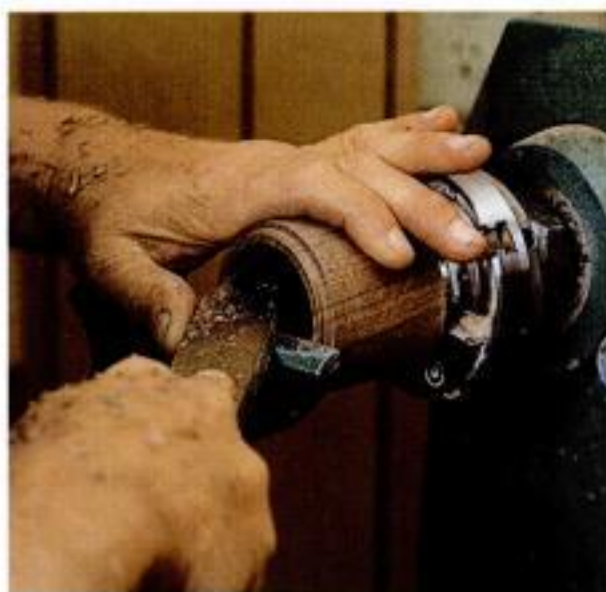
Shaping the base. Rough out the interior with a gouge after turning a shoulder for a rough fit with the lid (left). Then refine the interior shape with a scraper (center). After finishing the interior, turn the flange for a tight fit with the lid (right).
