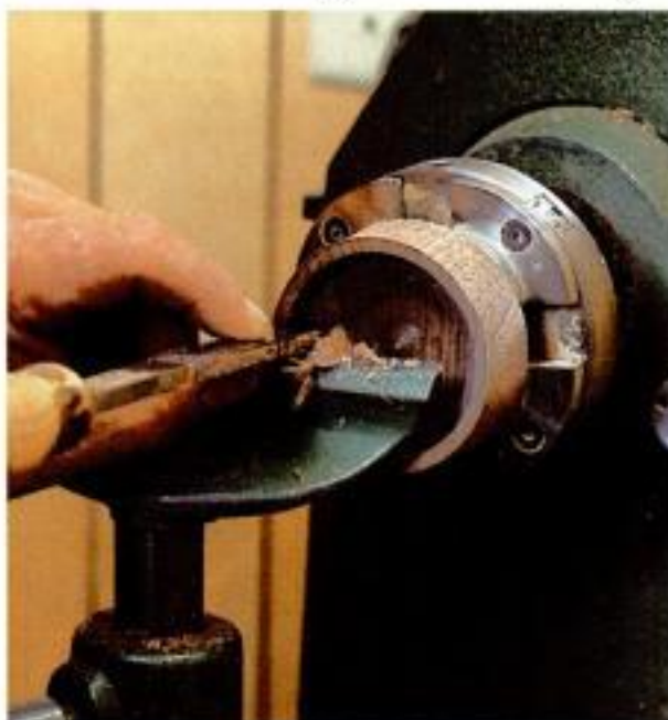
Lid work. Start by "back hollowing" the lid with a 1/2-in. gouge (left). Cut the flange that will fit over the base with a square-end scraper, making sure to make the flange parallel to the turning axis (center). After turning and sanding the inside of the lid, apply a coat of beeswax and buff it out (right).
