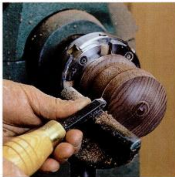
Turning base and lid together. With the lid fit tightly on the base, turn the final detail on the top of the lid (left). Form the beads on both sides of the opening with a skew (center). Buff on a beeswax finish after sanding the profiled sides (right).
