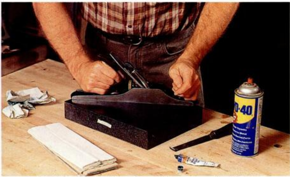
Test of sole. Right out of the box, plane soles were tested for flatness on a surfacing plate (left). At right, blue dye shows where the sole contacted the plate. The more blue, the flatter the sole. From top: AMT, Anant, new Stanley Bailey, vintage Stanley Bed Rock, vintage Stanley Bailey, Record, Footprint, Great Neck, Stanley Contractor.
