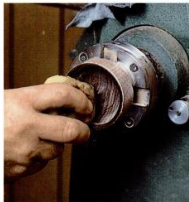
Lid work. Start by "back hollowing" the lid with a 1/2-in. gouge (left). Cut the flange that will fit over the base with a square-end scraper, making sure to make the flange parallel to the turning axis (center). After turning and sanding the inside of the lid, apply a coat of beeswax and buff it out (right).
