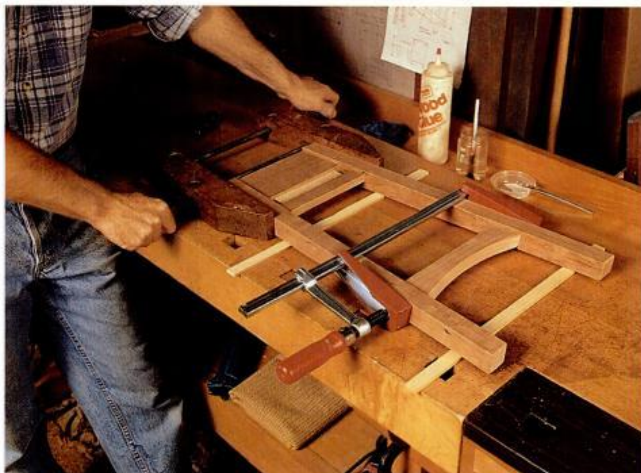
Angled clamping. A flat surface and clamps with adjustable jaws ensure that the side assembly glues together without slippage or twist. The author uses a scrap block between the upper and lower rails to keep the spacing correct (left). Make sure the entire assembly is true by gluing it together upright on the bench (right).
