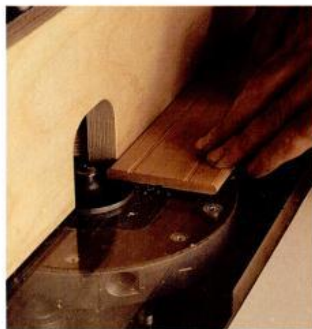
Rounding tenons. Round over the edges of the loose tenon stock on the router table to fit the curved ends of the mortises.
