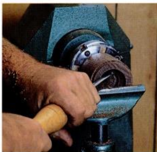
Shaping the base. Rough out the interior with a gouge after turning a shoulder for a rough fit with the lid (left). Then refine the interior shape with a scraper (center). After finishing the interior, turn the flange for a tight fit with the lid (right).
