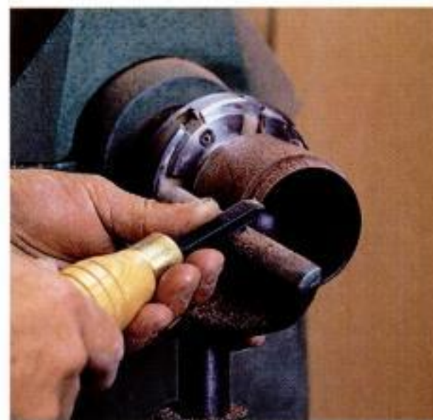
Shaping the base. Rough out the interior with a gouge after turning a shoulder for a rough fit with the lid (left). Then refine the interior shape with a scraper (center). After finishing the interior, turn the flange for a tight fit with the lid (right).
