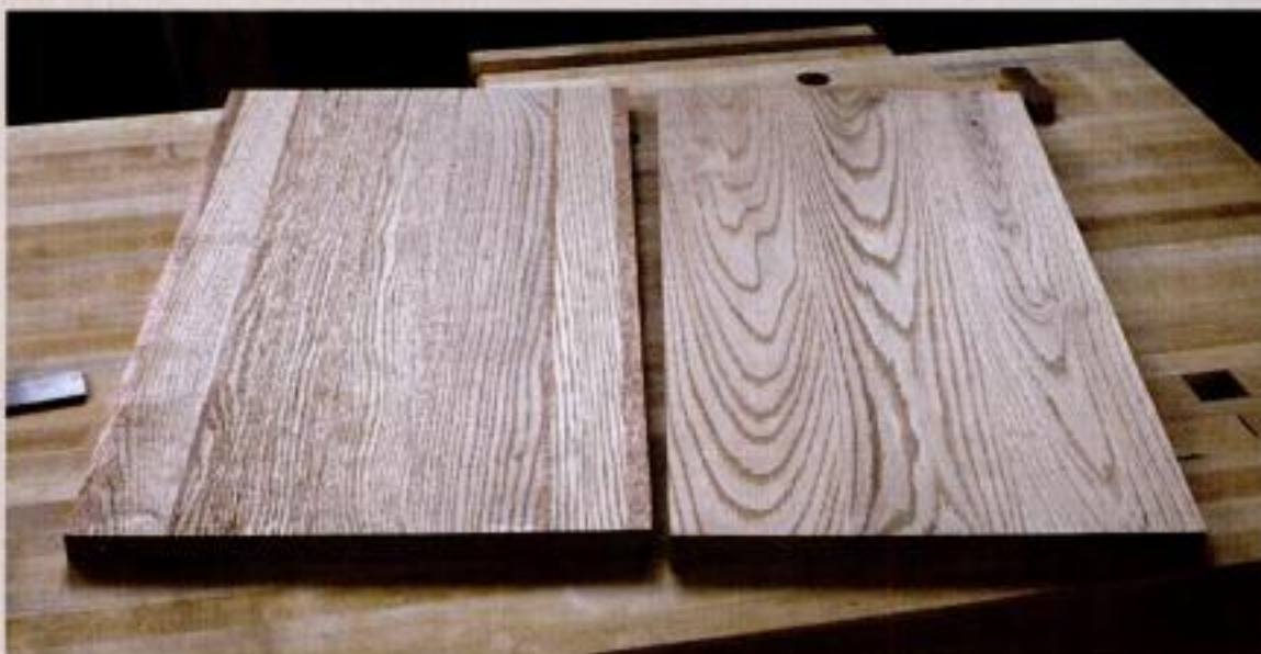
Fancy panels. At left, a quartersawn panel with solid inserts. At right, a flatsawn panel with cathedrals.
