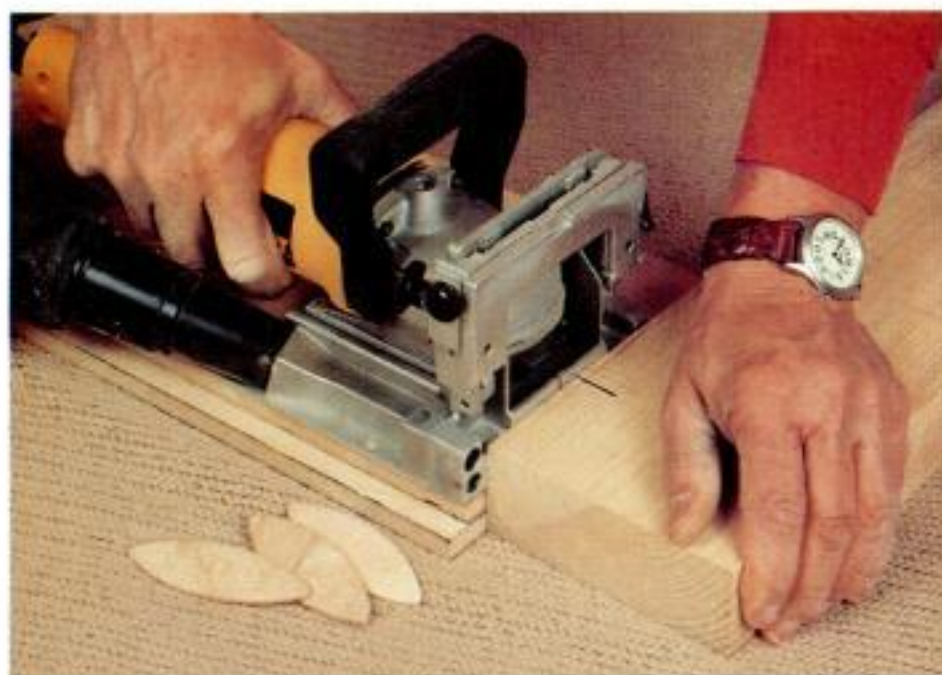
Slot machine. Hanson mills the topmost biscuit slot in a door stile, using two 1/2-in.-thick spacers beneath the joiner to keep the slots parallel and evenly spaced.
