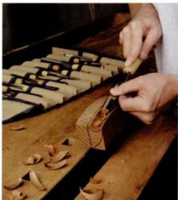
Carving a cove by hand. Clamp the crest rail in a bench vise and carve from the center of the rail toward each end to avoid tearout.
