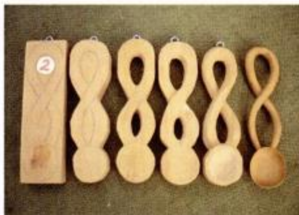
Spoon with a twist. With its figure-of-eight handle, this spoon is first cut with a fretsaw and then shaped with carving tools.
