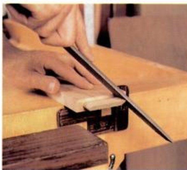
Tenon two-step. Form the tenons on the tablesaw with a carbide-tipped dado blade (left). At the bench, Rae rounds the edges of the tenons with a patternmaker's rasp (right).
