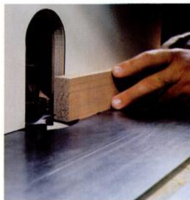
Profile work. Bird runs a stile through the shaper to mill the quirk-and-bead sticking profile.
