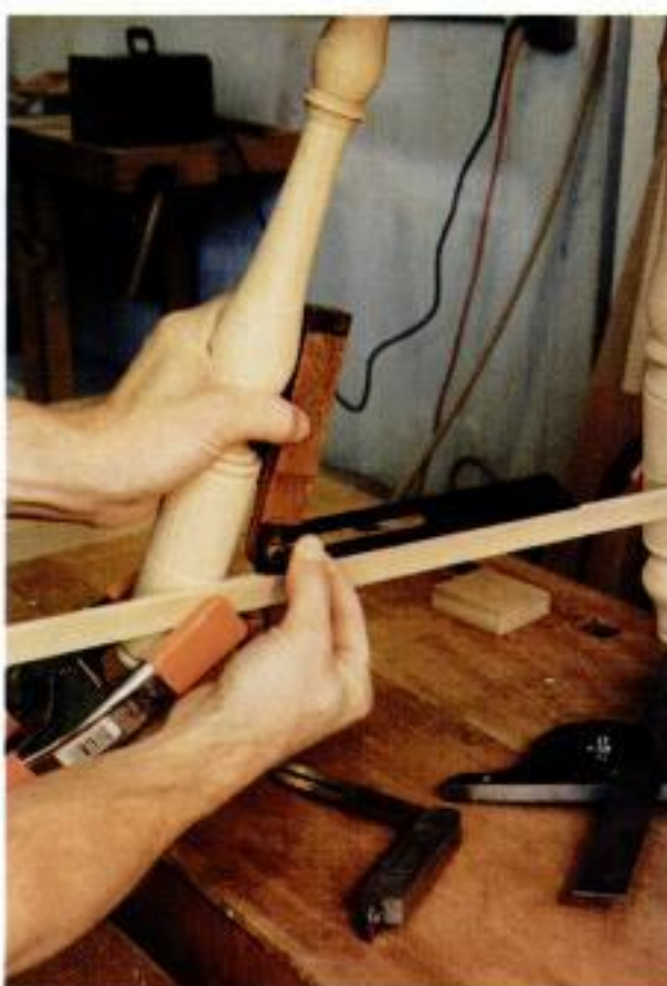
Stretcher work. Find the correct angle of the stretcher holes in the legs with a bevel gauge (left). Then use the gauge as a guide when boring the stretcher holes (above).
