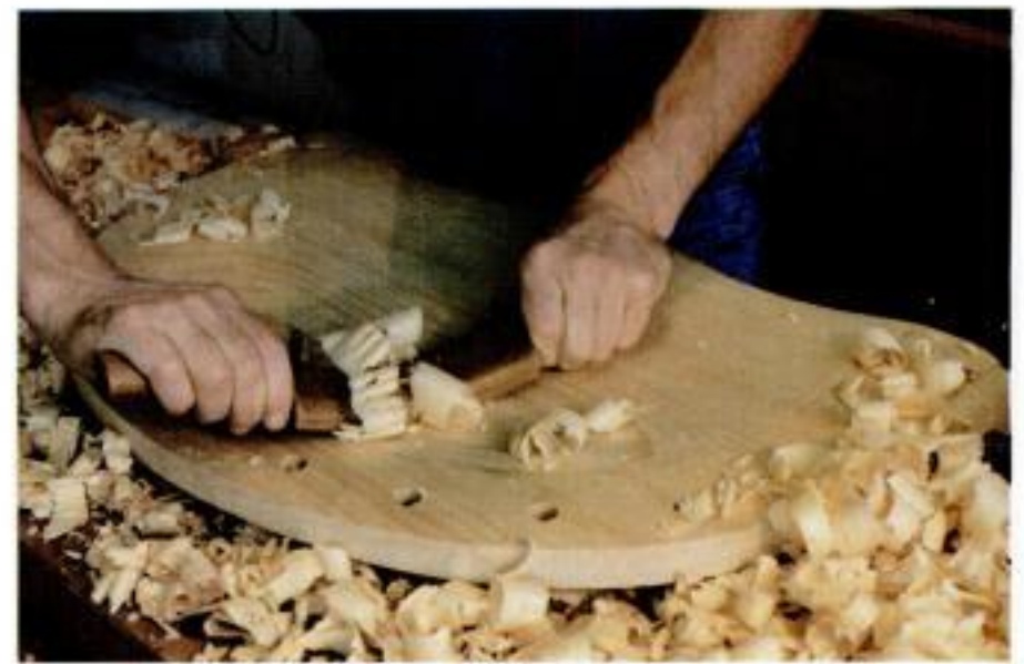
Saddling the seat. A scorp makes quick work of roughing out the contours of the seat (left). Treanor then smooths and refines the surface with a travisher (right).
