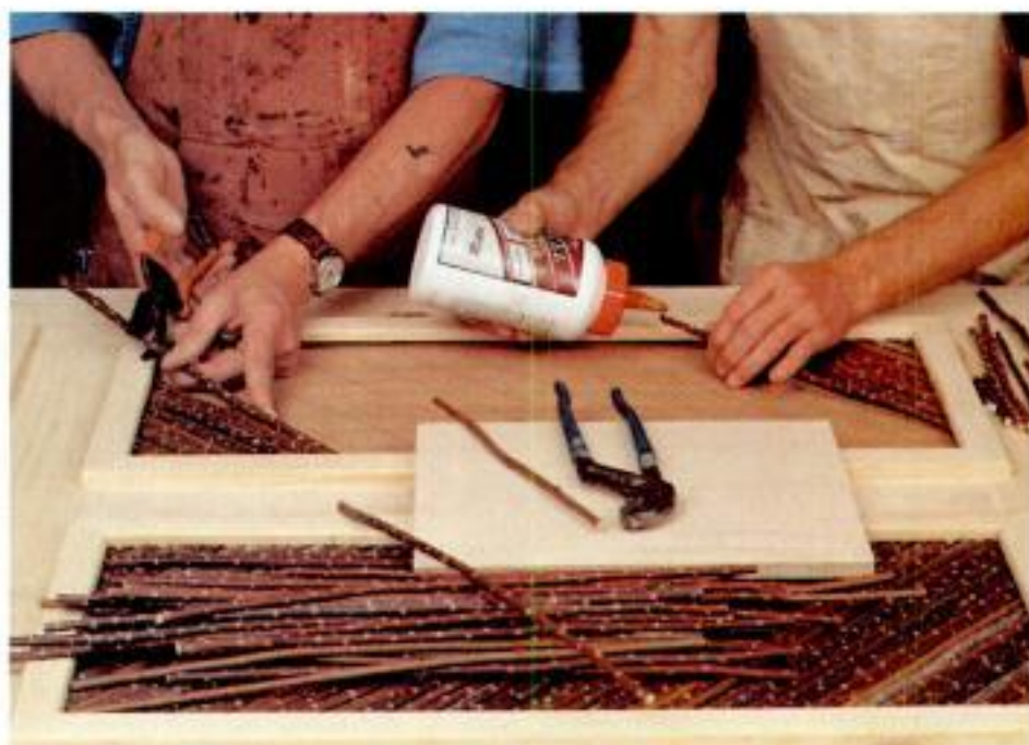
Twig infill. Working toward the center from opposite corners, Hanson and Ring cover a plywood panel with tamarisk twigs. After being snipped to length, twig ends are wedged between the panel and the interior molding.
