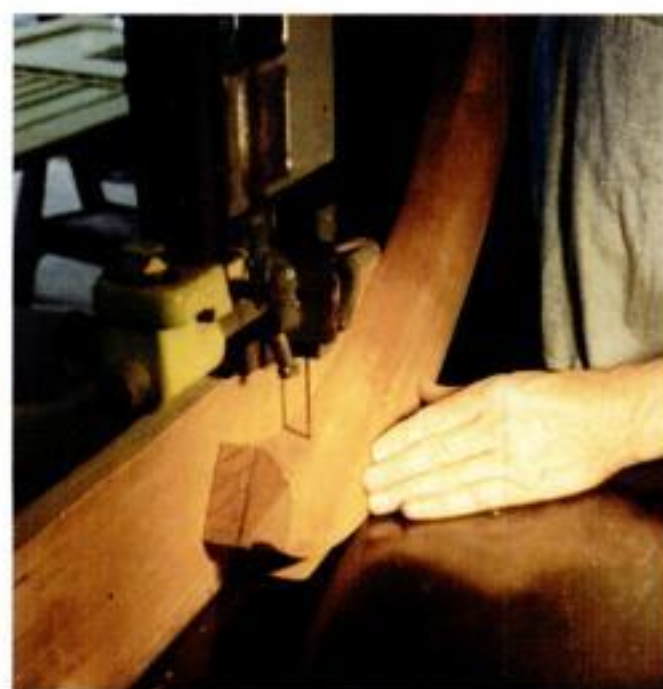
Sawing the lap joint. Cut the half-lap in the crest rail on the bandsaw. Guide the workpiece against a fence to keep the cut straight.
