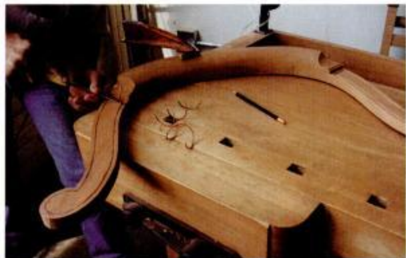
Carving the details. Use a sharp chisel to carve the transitional thumbnail on the end of the crest rail (center). Then, use a narrow gouge to cut the shallow cove on the arm (right).
