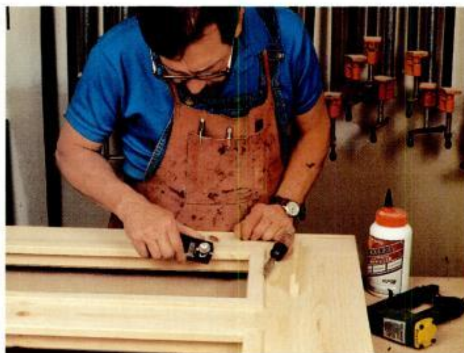
Trimmed out. Ring uses a block plane to touch up a chamfer on the exterior trim.
