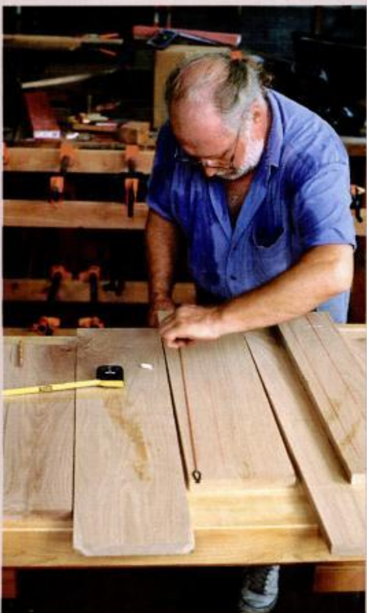
Draw the board. The first chalk line locates the center of the "V"-shaped figures, or "cathedrals." Measuring equal distances to both sides defines the selections.
