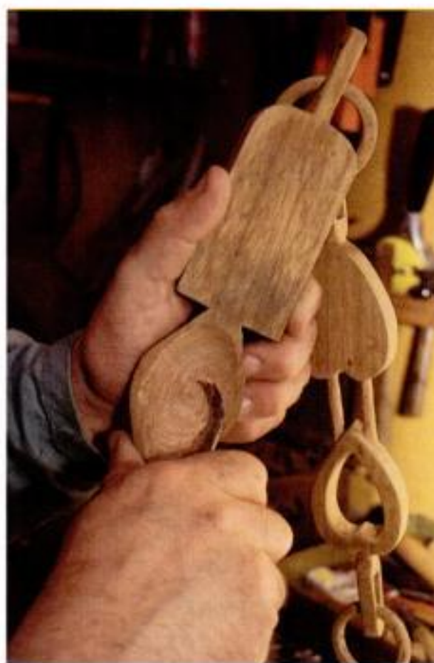
Getting the scoop. Hentall uses a specially made bent knife, called a twca cam (pronounced took'-ur-cam), to hollow out the spoon bowl.
