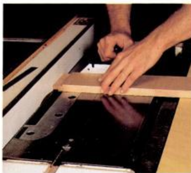
Tenon two-step. Form the tenons on the tablesaw with a carbide-tipped dado blade (left). At the bench, Rae rounds the edges of the tenons with a patternmaker's rasp (right).
