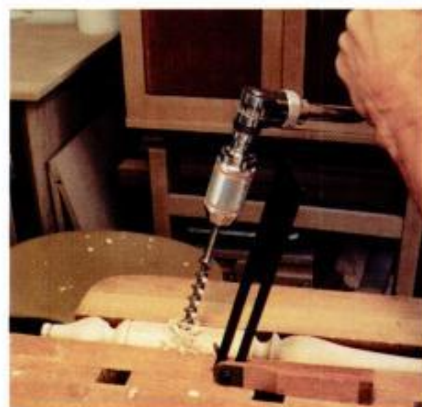
Stretcher work. Find the correct angle of the stretcher holes in the legs with a bevel gauge (left). Then use the gauge as a guide when boring the stretcher holes (above).
