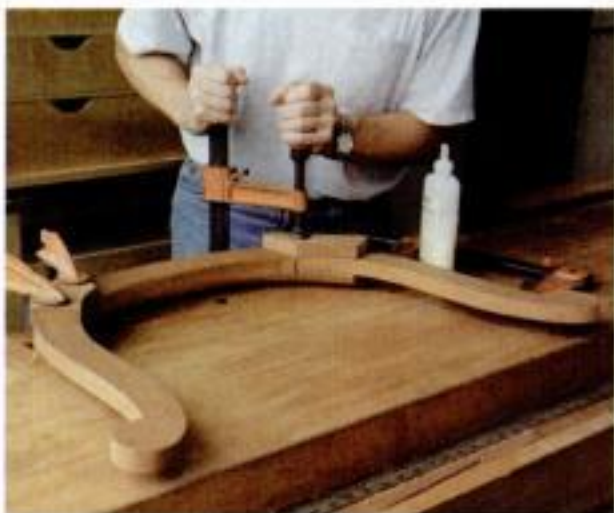
Clamping the arm. Treanor glues up the arm assembly with the parts upside down on his bench.
