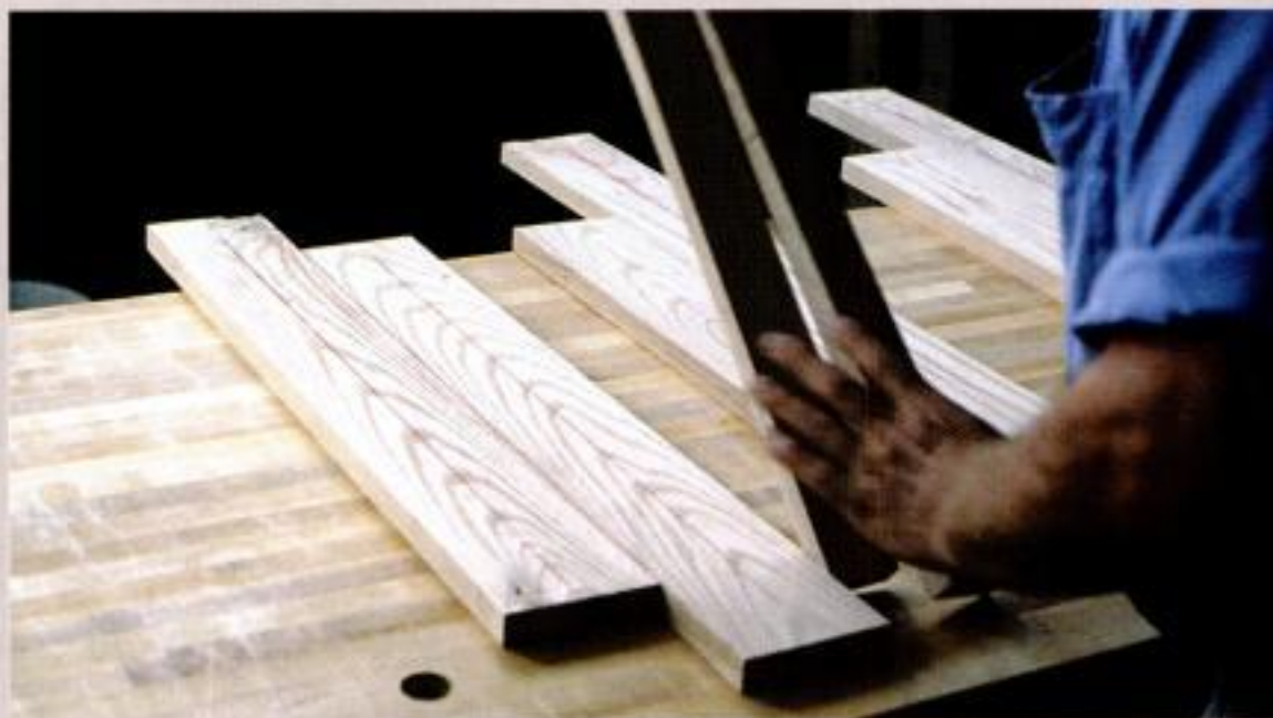
Rip and sort. After you rip the board on the bandsaw, you can sort the wood into flatsawn cathedrals and the straight figure of quartersawn and rift-sawn wood.
