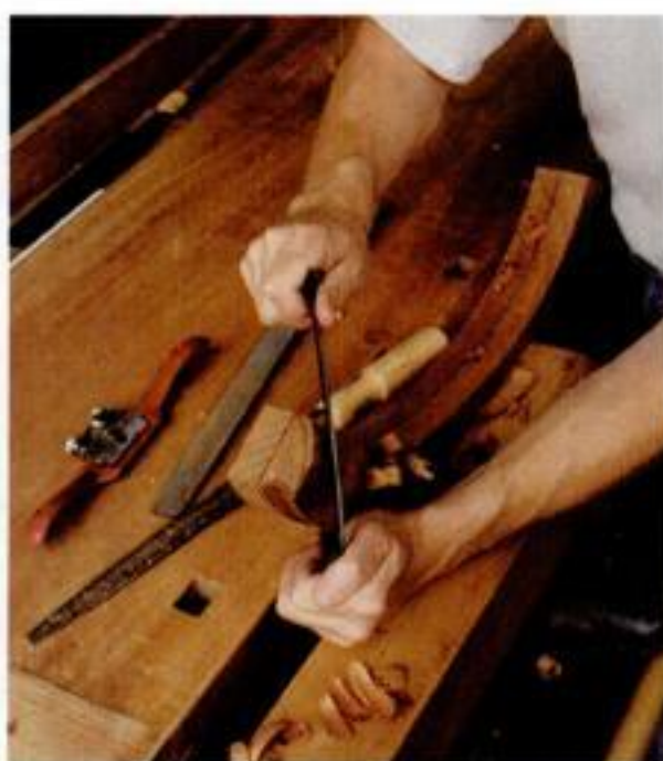
Shaping the round-over. Treanor uses a drawknife to round the edge of the crest rail. A spokeshave and rasps help to refine the curved surface.
