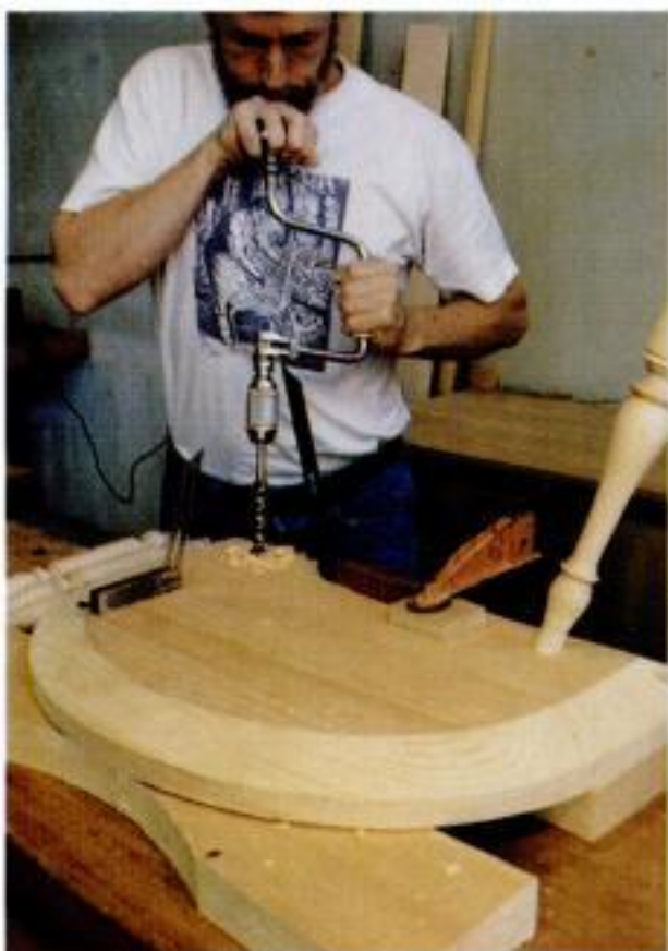
Boring the leg holes. Treanor drills the angled hole for the front leg by eyeballing two bevel gauges set to the correct splay of the leg.
