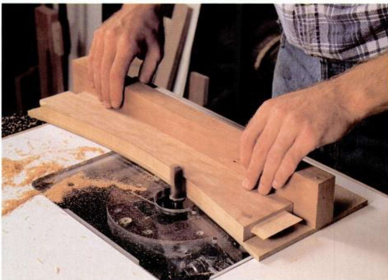
Routing a curve. Rae shapes the lower rail on the router table by guiding a curved template against the bearing of a pattern bit. Double-faced tape holds the workpiece to the jig.
