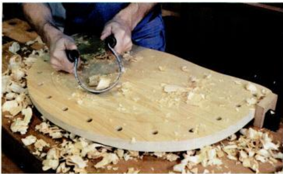
Saddling the seat. A scorp makes quick work of roughing out the contours of the seat (left). Treanor then smooths and refines the surface with a travisher (right).
