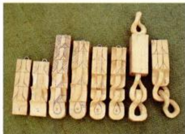
Pieces of eight. The figure-of-eight links shown here feature links that have a 90° twist. Careful carving frees them from the blank.
