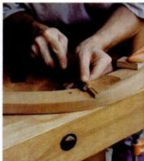
Carving the details. Use a sharp chisel to carve the transitional thumbnail on the end of the crest rail (center). Then, use a narrow gouge to cut the shallow cove on the arm (right).
