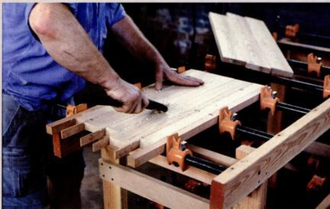
Solid inserts. Inserts of solid mahogany enhance the proportional pattern created by quartersawn rippings of various widths. Kirby scrapes off the glue squeeze-out before it sets hard.
