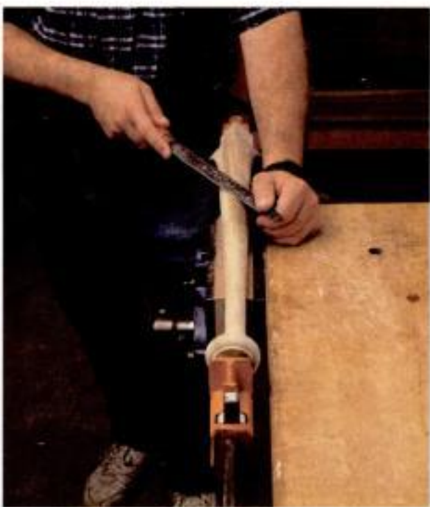
Filing it fair. Legs gain their final form with hand work. Bird starts with a rasp and file, then moves on to scrapers and sandpaper.
