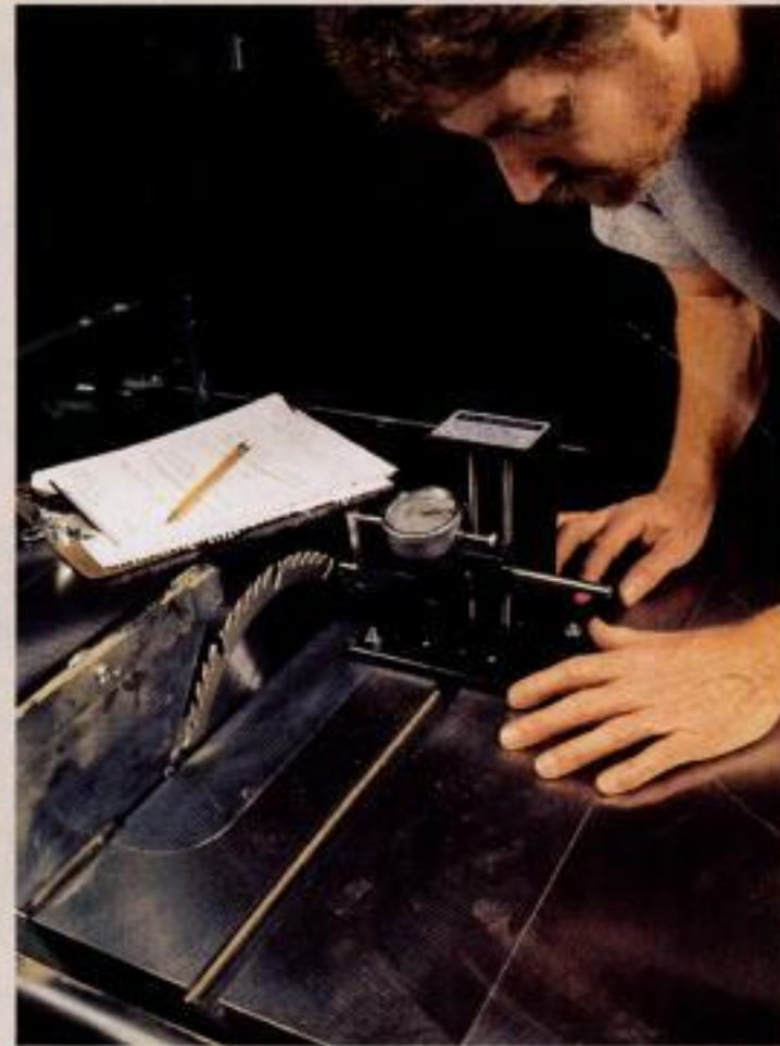
Getting in tune. To align the miter slots parallel to the blade, Dave Sellers uses a TS-Aligner gauge.
