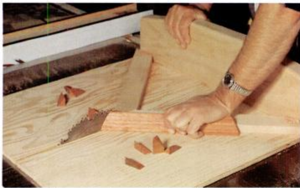
Sawing miters. Greef uses a homemade mitering jig to miter the ends of the sides. The jig has wooden runners that ride in the table saw's miter grooves.
