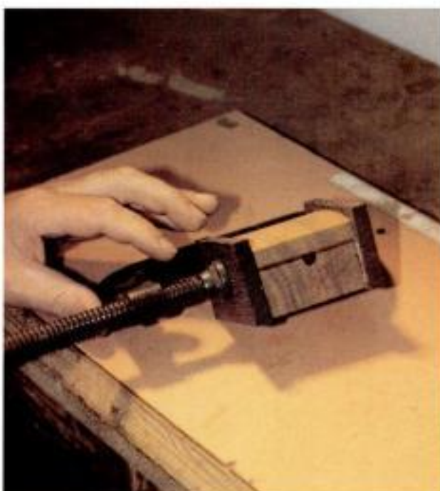
A single C-clamp. Taking care to keep the lid free of glue, join the sides to the box body. Glued up oversize, the sides will be sanded flush after the glue dries.
