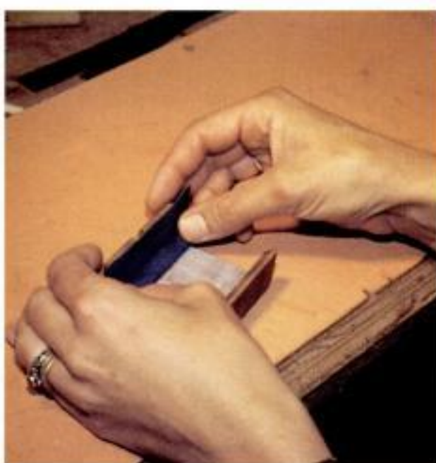
Suede lining. Janet O'Rourke glues suede fabric in the U-shaped cavity of the box body. Excess suede is razored off after the glue dries.
