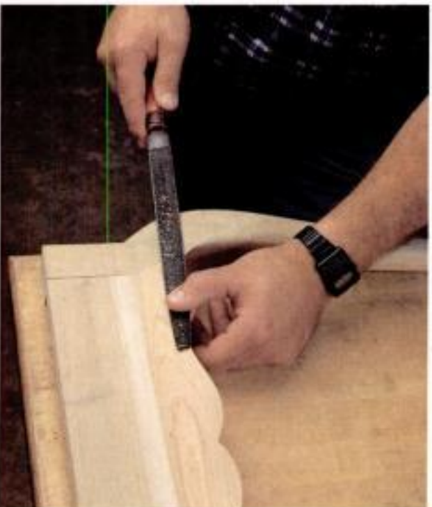
Blending the curves. Bird uses a patternmaker's rasp to smooth the leg flush with the knee block.
