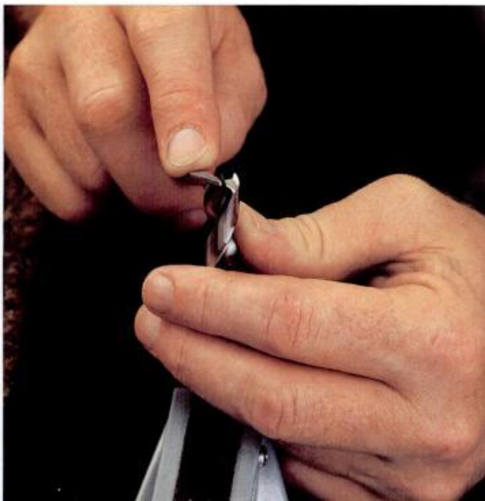
A few good strokes. The author uses a diamond file to sharpen the bevels of a spurred brad-point bit (left). He hones the insides of the spurs with a wooden stick covered with 600-grit abrasive (above).
