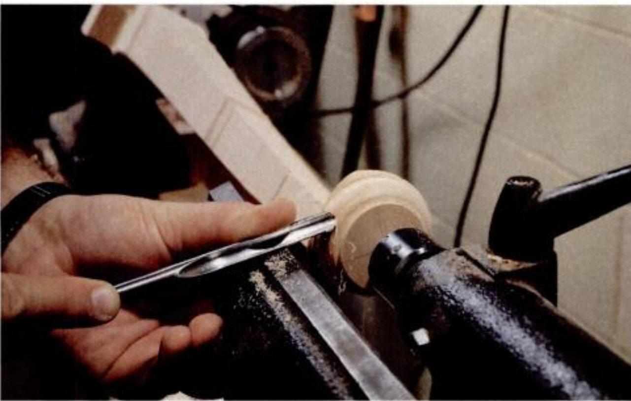
Turning the foot. Using a \frac{3}{8} -in. spindle gouge, the author turns the curve of the foot, starting at the top of the foot and working toward the pad.
