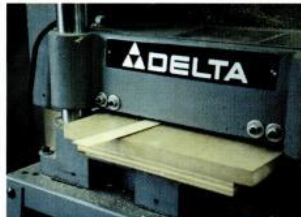
Closing the gap. A planer board effectively raises the planer bed, allowing you to mill stock as thin as 1/16 in.
