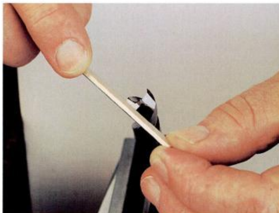
A few good strokes. The author uses a diamond file to sharpen the bevels of a spurred brad-point bit (left). He hones the insides of the spurs with a wooden stick covered with 600-grit abrasive (above).
