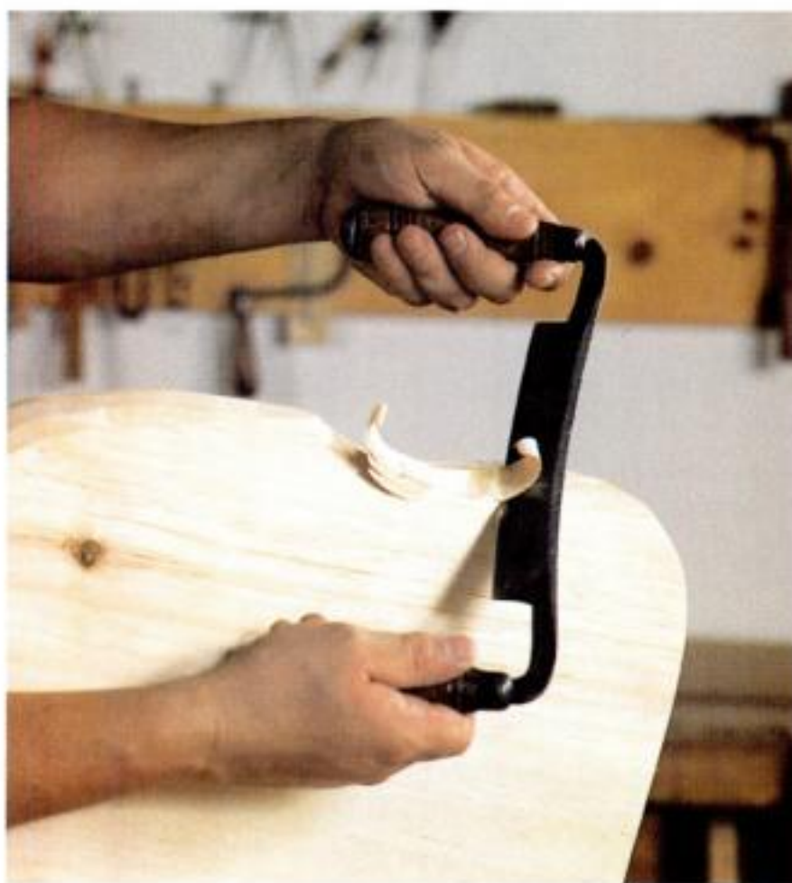
Making a concave cut. Slice in from opposing ends of a concave cut to prevent cutting against the grain. The small bezel on the back of the blade allows the drawknife to follow the curve smoothly without diving into the wood.
