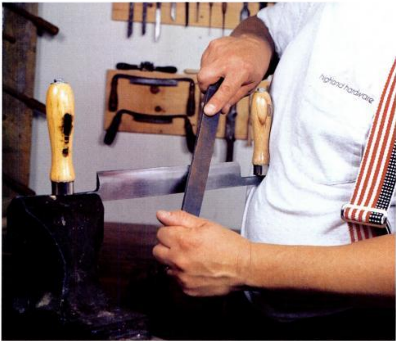
Reshaping a bezel. Dunbar drawfiles the edge of a modern drawknife to convert its factory-ground bezel to a smooth, rounded shape.
