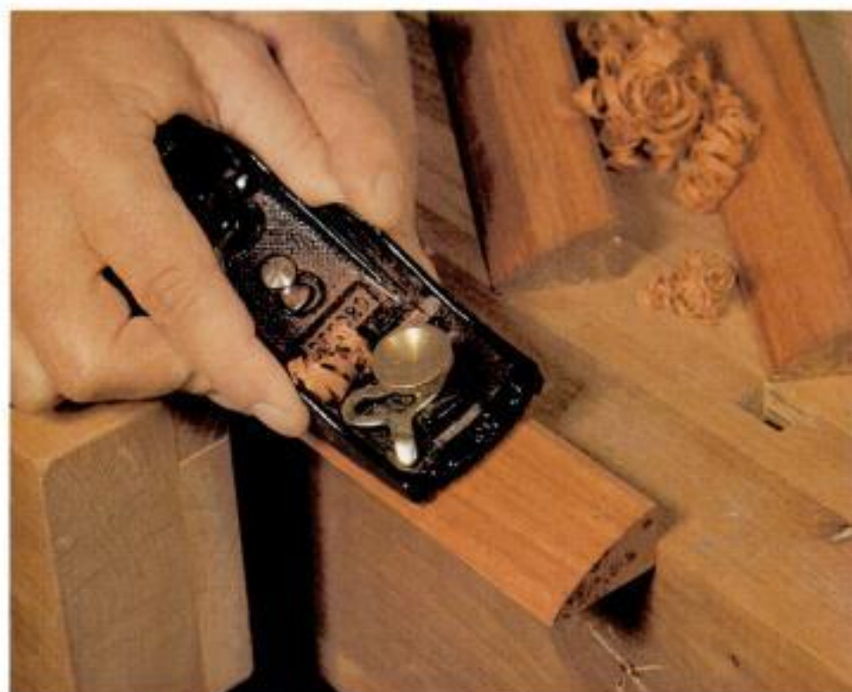
Shaping the curves. Greef uses a block plane to round the bevel-cut faces of the tray sides.
