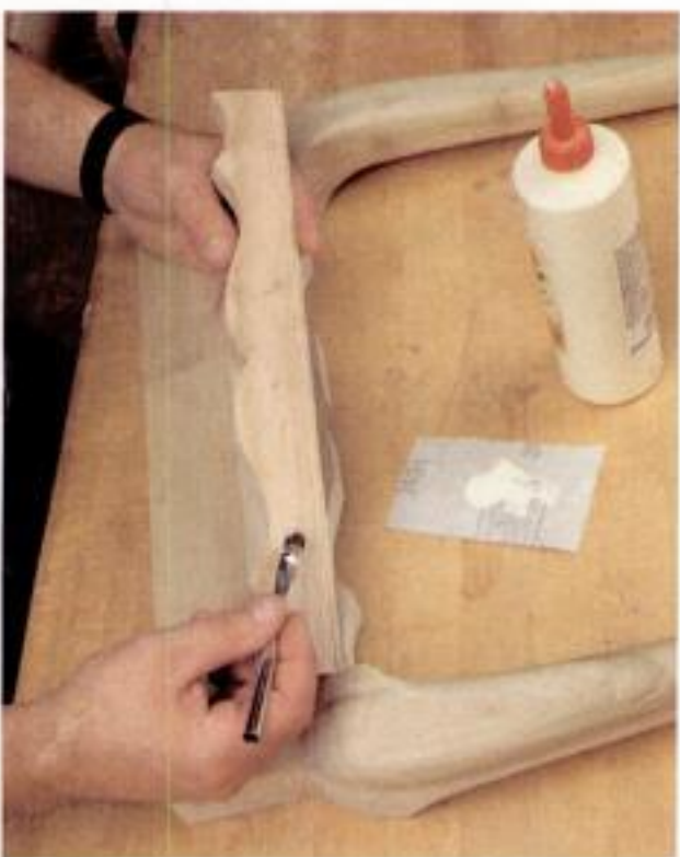
Glue-up. A brush helps to spread an even coat of glue on the back of the knee block. The groove along the back edge will catch excess glue, helping to prevent squeeze-out.
