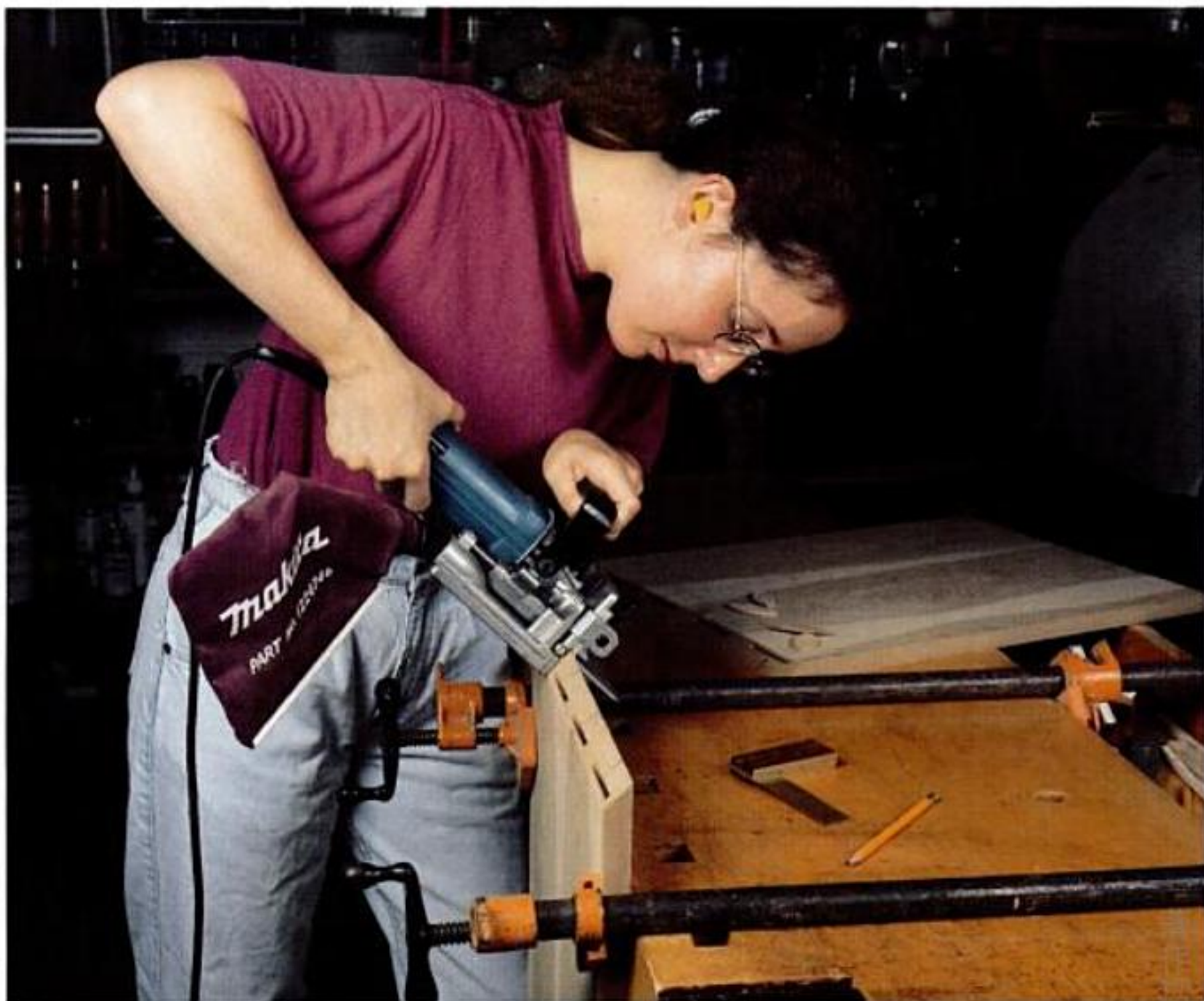
Redefining splining. Biscuit joiners cut arced slots that accept flat, football-shaped biscuits of compressed wood which swell when glued to make strong, accurate joints.
