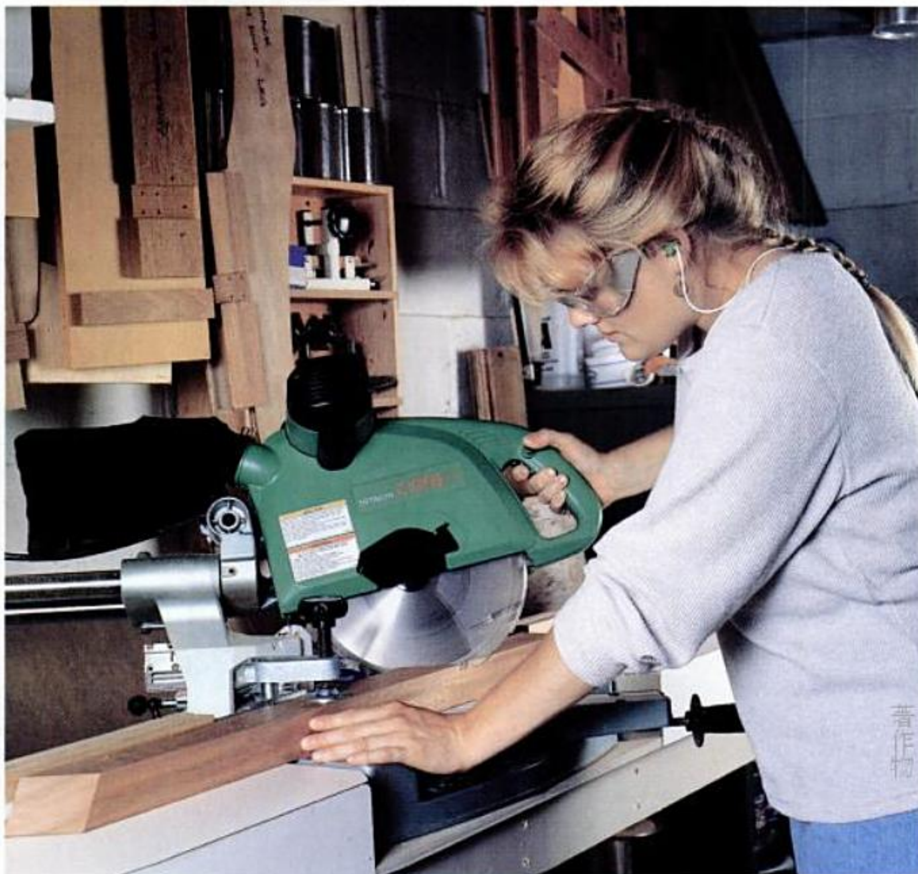
Fast and precise. Miter saws make glass-smooth miter cuts in moldings and narrow stock. The sliding compound saw shown above can crosscut wider stock and also make compound-angle cuts.
