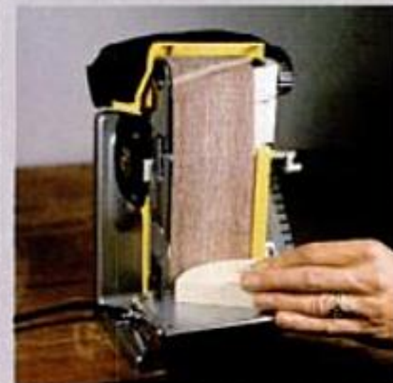
Stationary use. With an accessory stand, you can mount the sander horizontally or vertically on your workbench.
