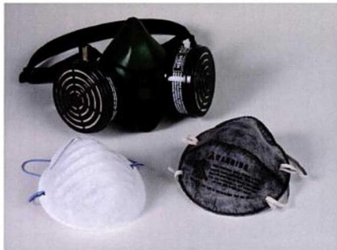
Breathing easy. Disposable filter masks, shown in the foreground, are inexpensive, and they offer good general protection against airborne dust. A cartridge-type mask can trap finer dust.
