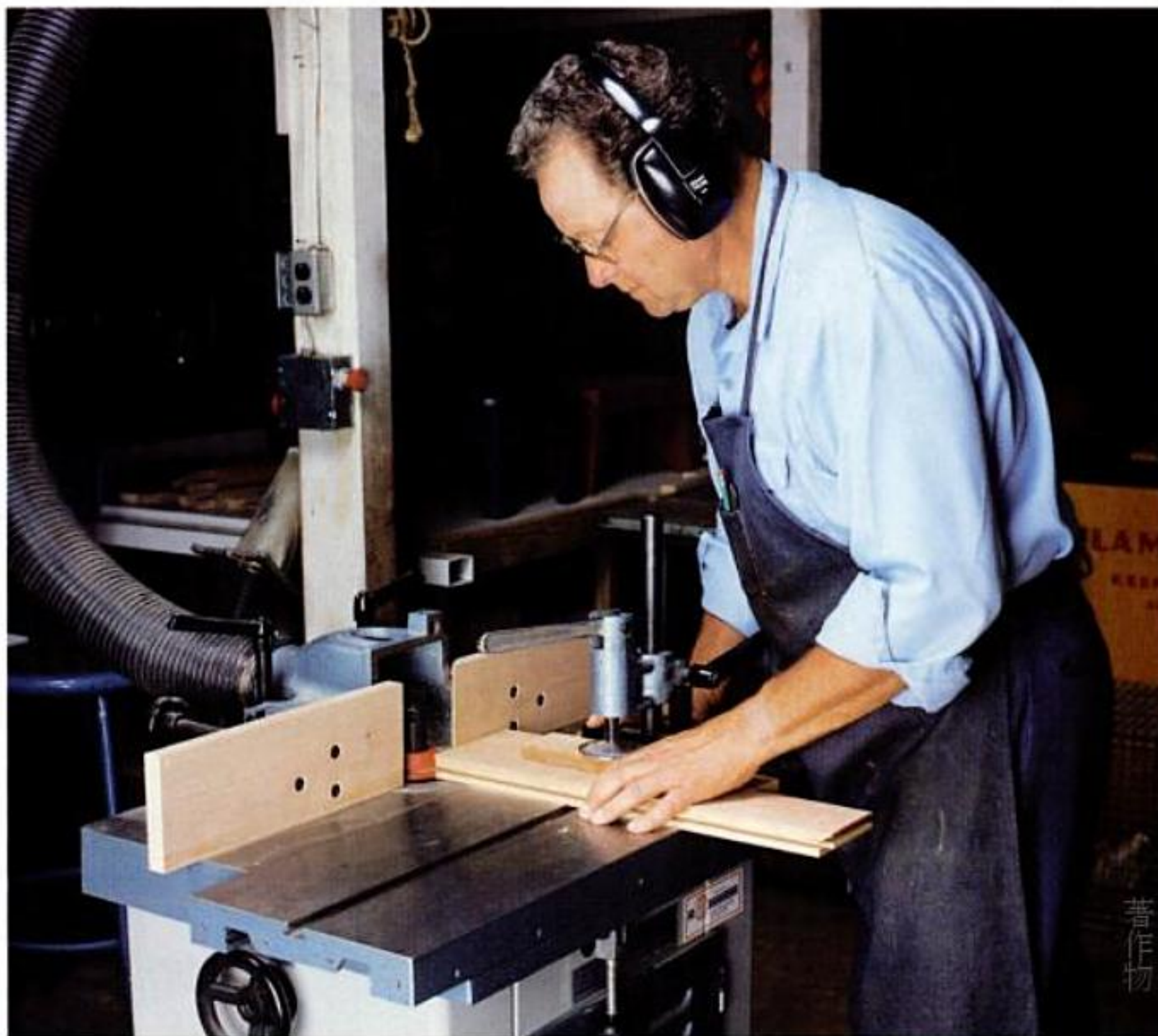
Get in shape. Buying a shaper opens the door to architectural woodworking. This heavy-weight can handle large or intricate work like raised panels and cope-and-stick joinery.
