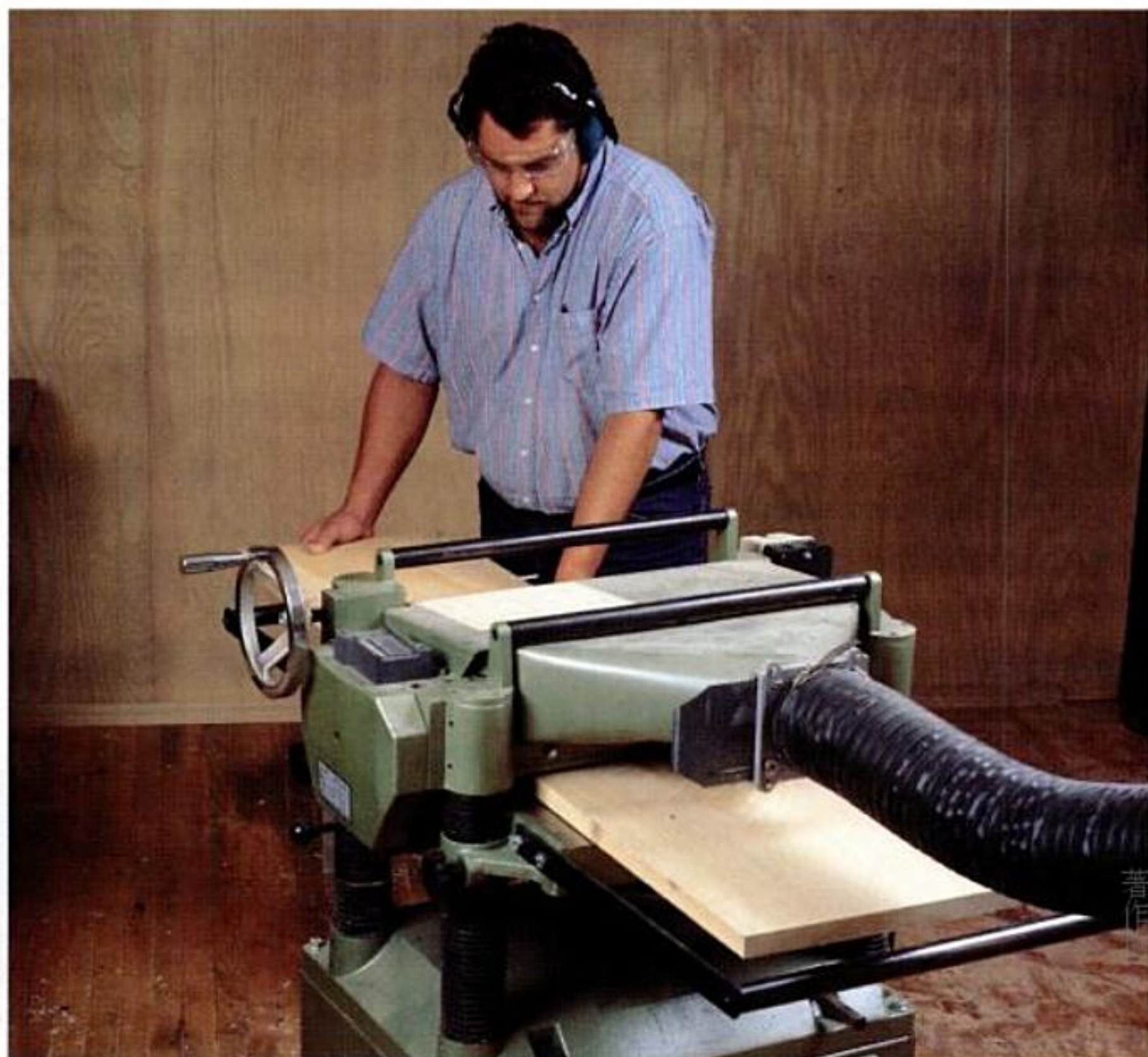
Shaving it down to size. A thickness planer allows you to mill lumber to the exact thickness you want for your project.
