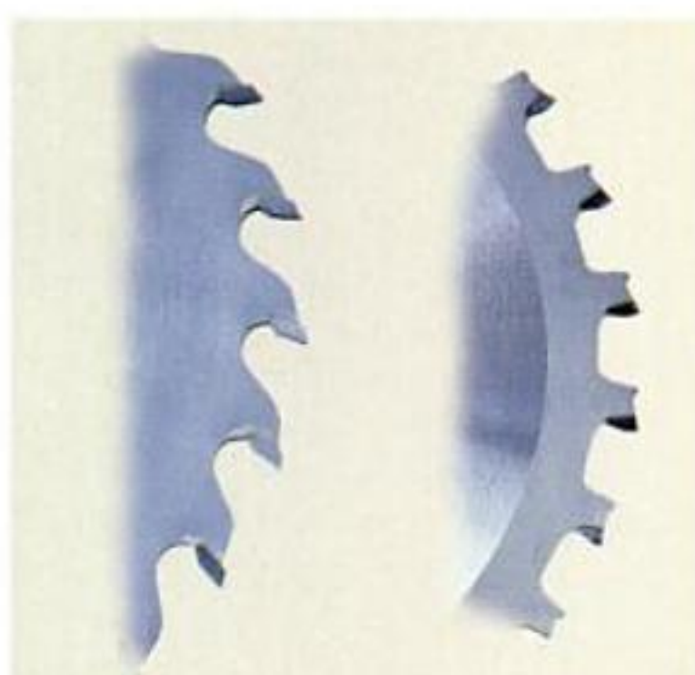
Anti-kickback cutters. A conventional circular saw blade (left) is more prone to kickback than one engineered with kickback-limiting shoulders (right).
