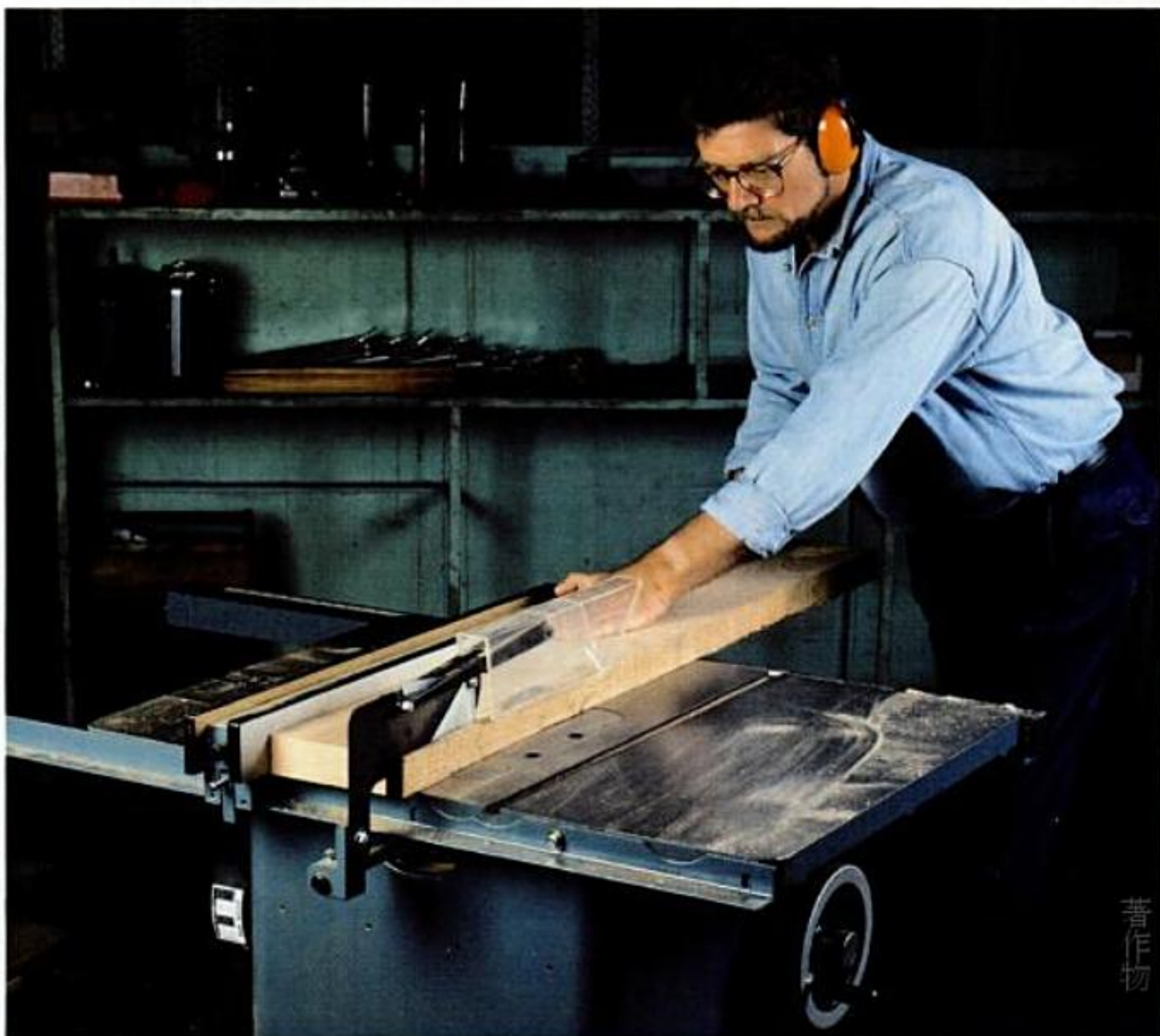
Shop workhorse. A tablesaw is the primary woodworking tool in many shops. No other machine can do so many jobs, from sizing material to cutting joints.
