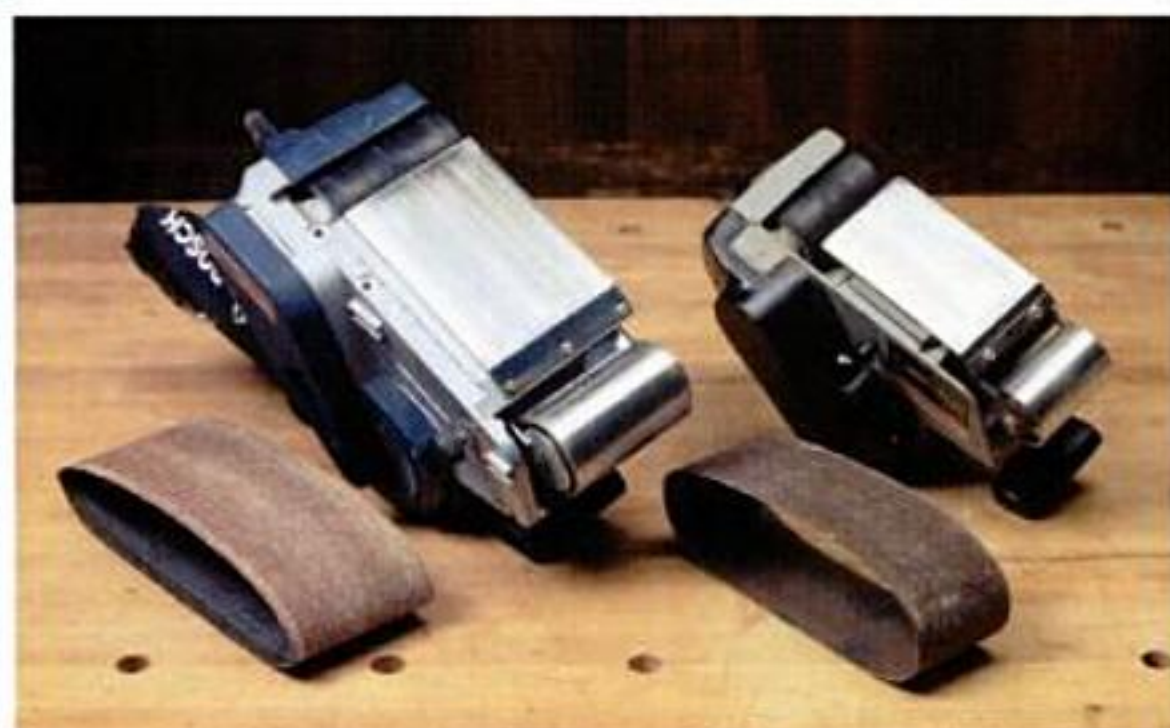
Sanding surface. Larger platens put more of the belt surface in contact with the wood, for faster stock removal.
