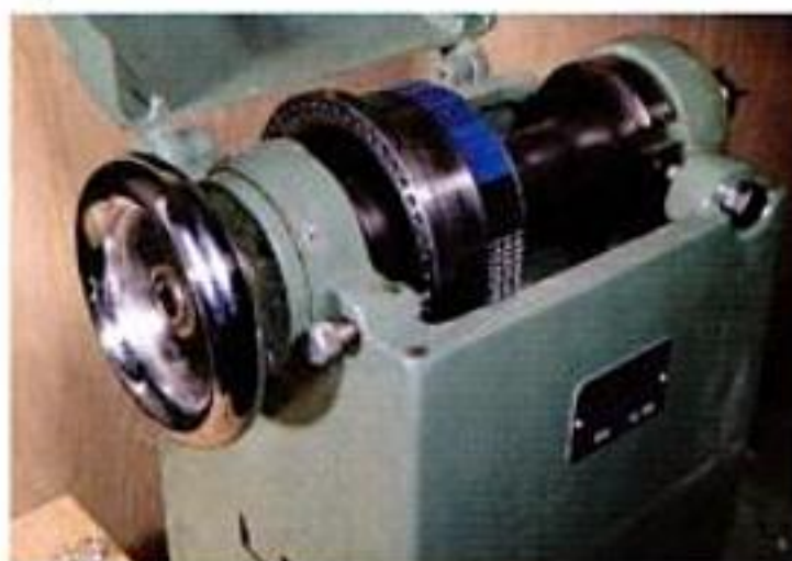
Indexing head. An indexing pin (on left end of housing) allows you to lay out turnings in equal increments for decorative work.
