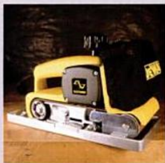
Frame it. Attached to the belt sander, a rectangular sanding frame promotes flat, even sanding on broad surfaces.
