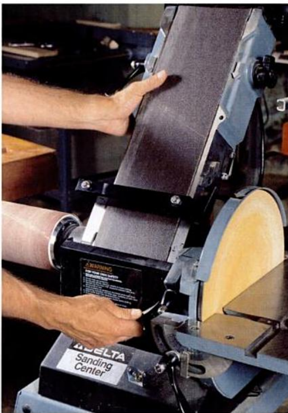
Angling the belt. With some belt-disc sanders, you can work with the belt adjusted between horizontal and vertical positions.
