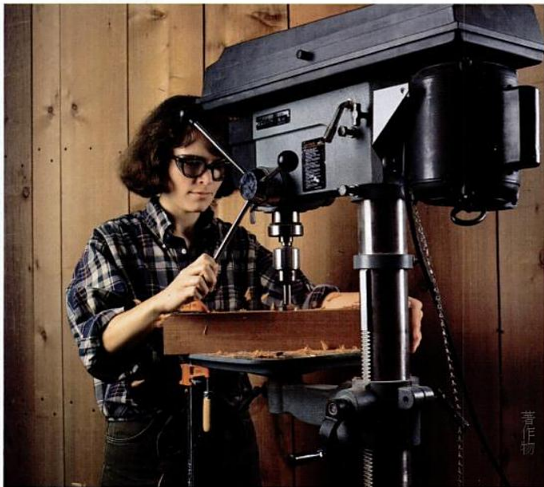
The hole story. No workshop would be complete without a drill press. This multipurpose tool drills holes, cuts plugs, chops mortises, and powers other accessories.
