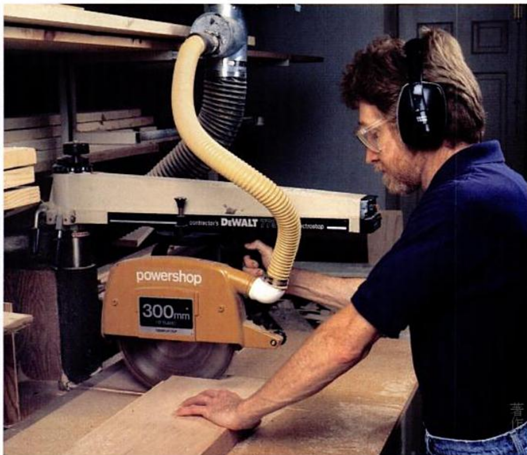
Radial revolution. The radial-arm saw is ideal for crosscutting or mitering large stock. With the right accessories, it can be a versatile tool for dimensioning and shaping wood.
