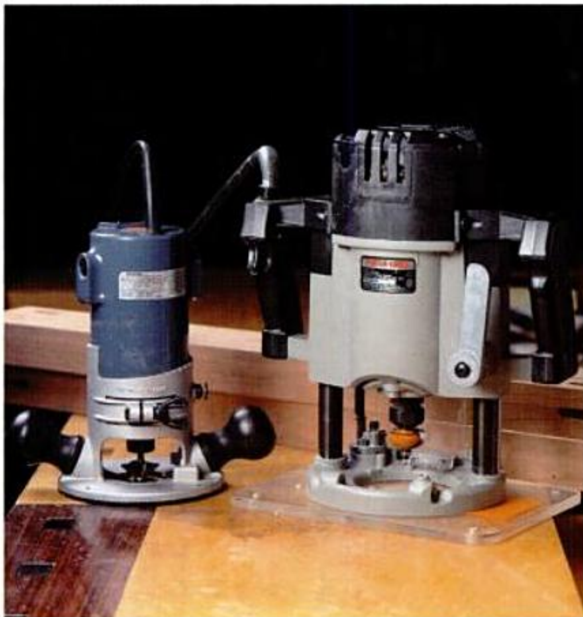
Little and big. For hand-held operations, a small router like the Bosch 1604A has the edge in maneuverability. More powerful routers like the Porter-Cable 7539 do their best work in a router table, for heavy-duty shaping.
