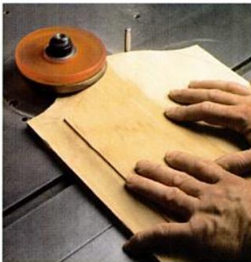
No-fence work. Shape curved parts without a fence by supporting the workpiece against a starting pin and rub collar.
