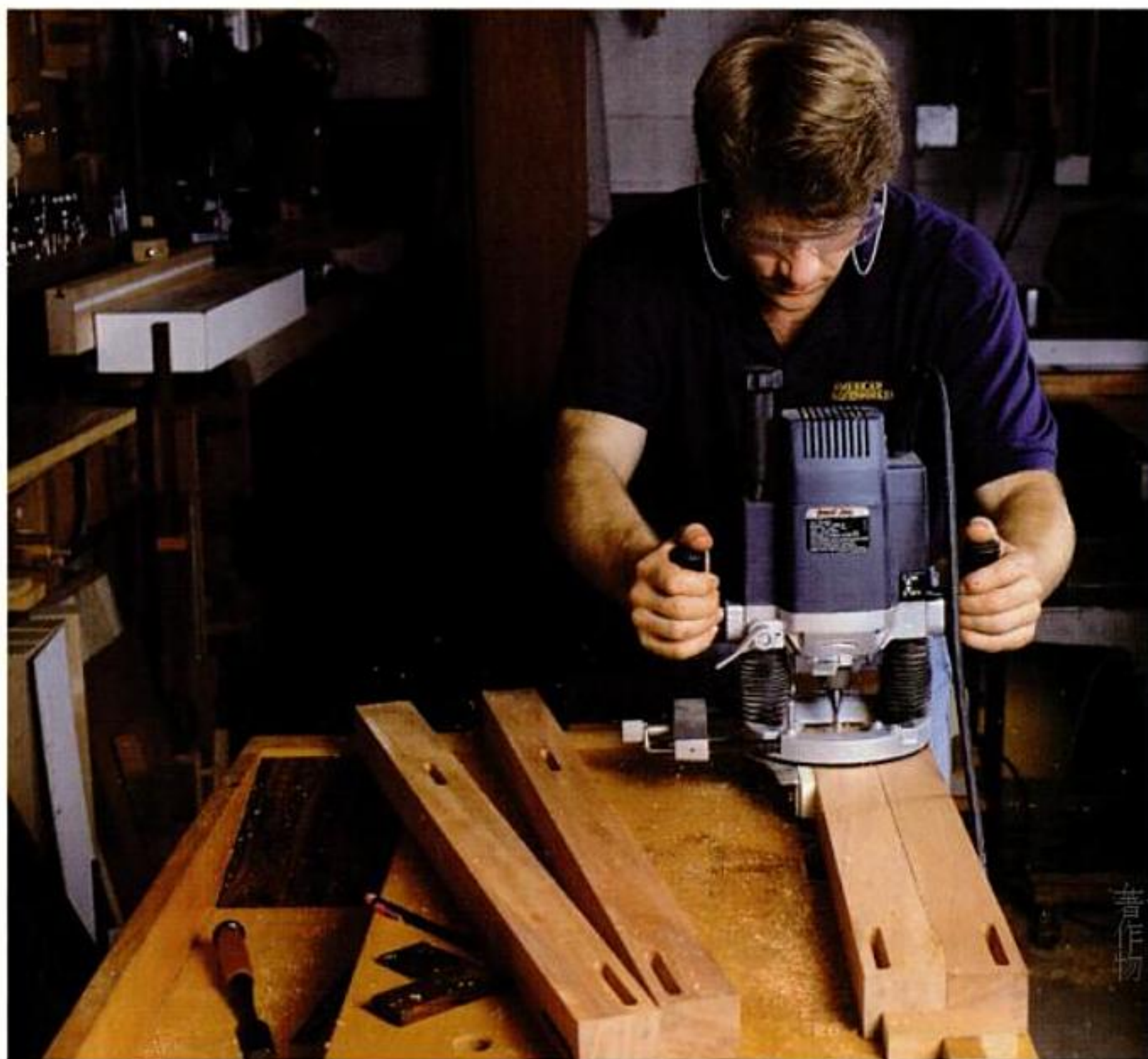
Plenty of possibilities. From edge treatments and joinery to pattern routing and panel raising, routers are packed with woodworking potential.
