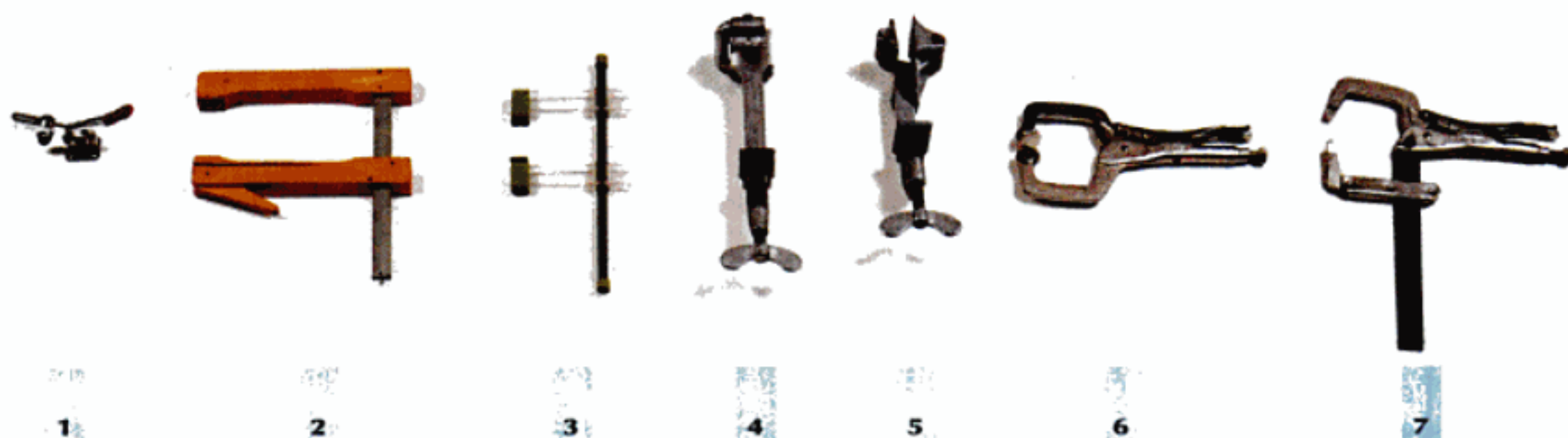
Specialty clamps. 1: Toggle clamp (DE-STA-CO). 2: Cam-action clamp (available from Garrett Wade). 3: Berna Assemblers model-maker’s clamp (Zona). 4 and 5: No Scuff right-angle clamp and Shelf and Corner right-angle clamp (Universal). 6 and 7: Locking-jaw plier clamps (American Tool).
