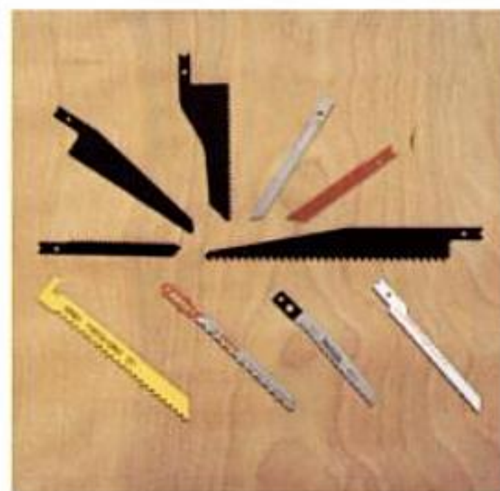
Choose your weapon. Jigsaw blades come in many sizes, and there's a blade for cutting just about any material. However, some saws have blade-holding mechanisms that accept only a specific type of blade.
