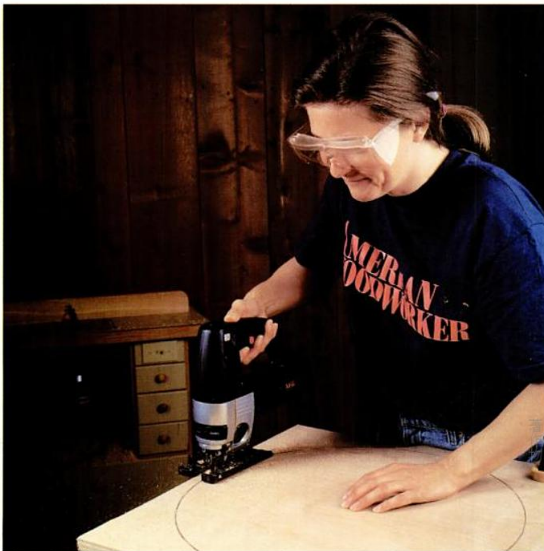
The jig is up... and down. Today's jigsaws make smooth, fast cuts in wood and other materials up to 2 3 / 4 in. thick.
