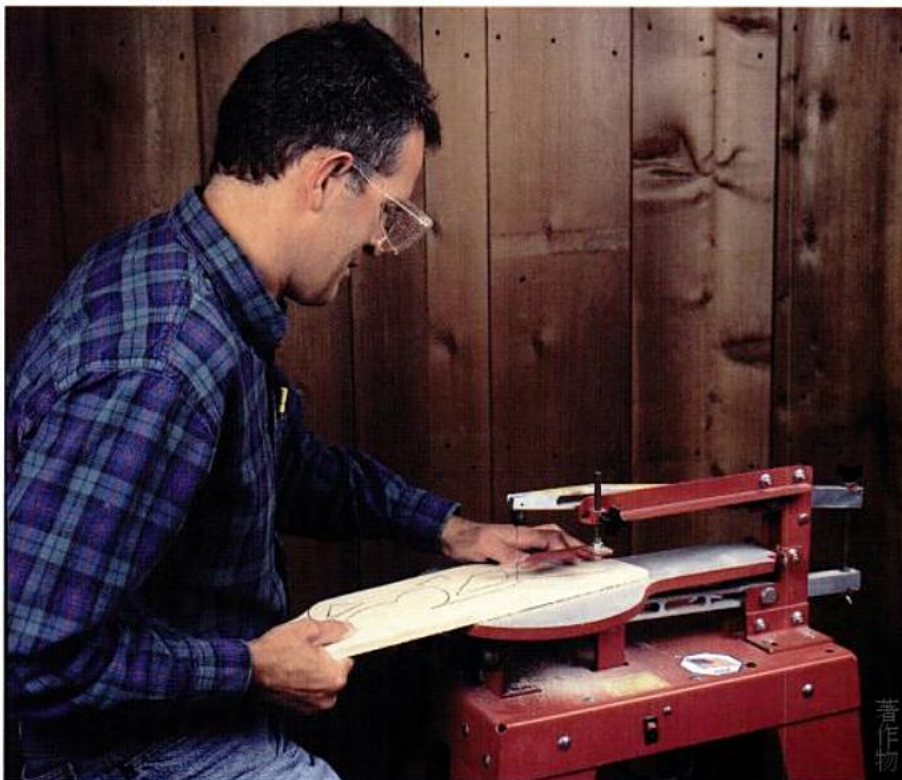
Intricate curves. For fretwork, marquetry, puzzlemaking and inside cuts, no tool does it better than the scrollsaw.
