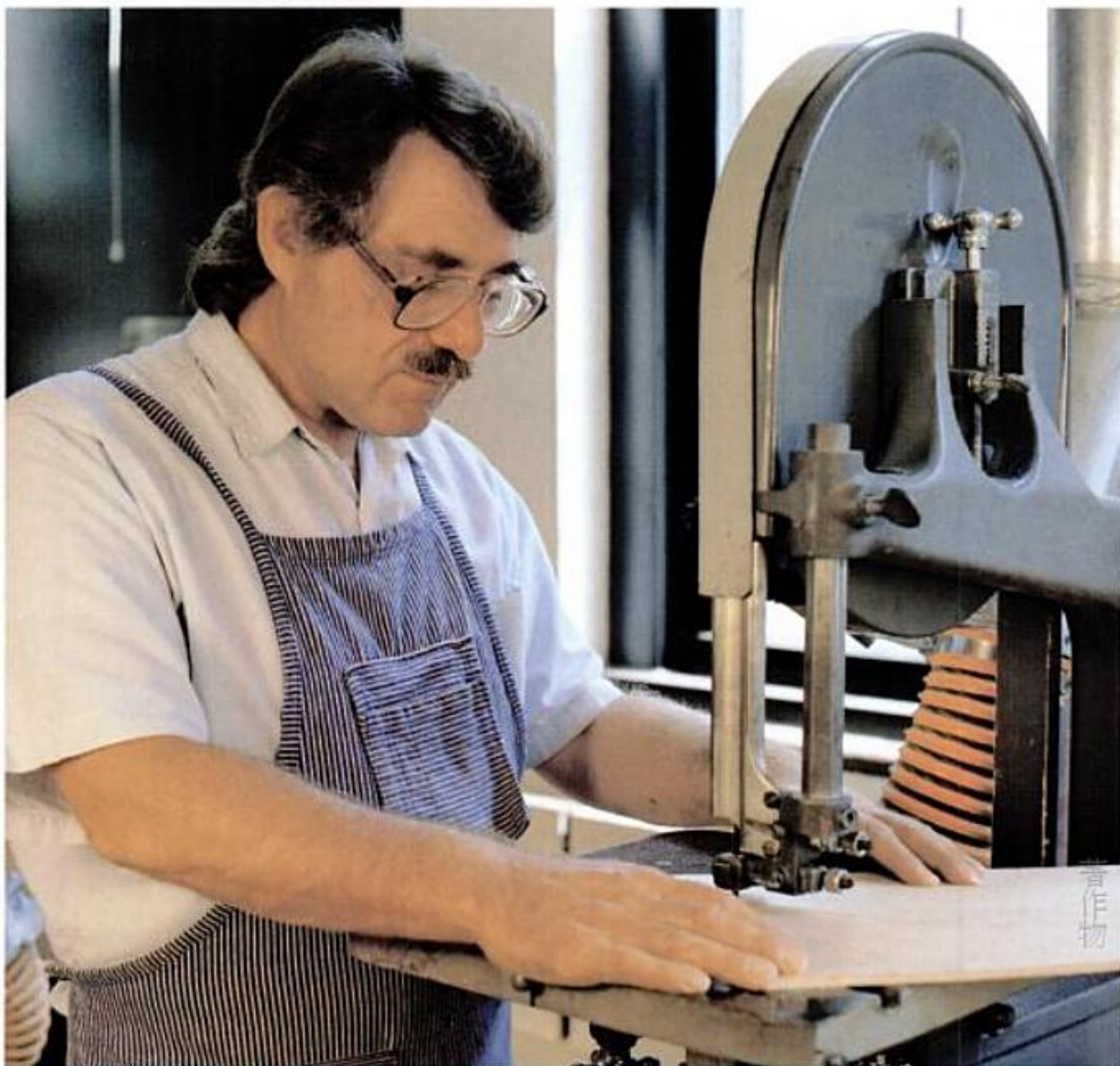
Curves, resawing and straight cuts. The bandsaw takes up where the tablesaw leaves off, performing general-purpose work and specialized cutting.
