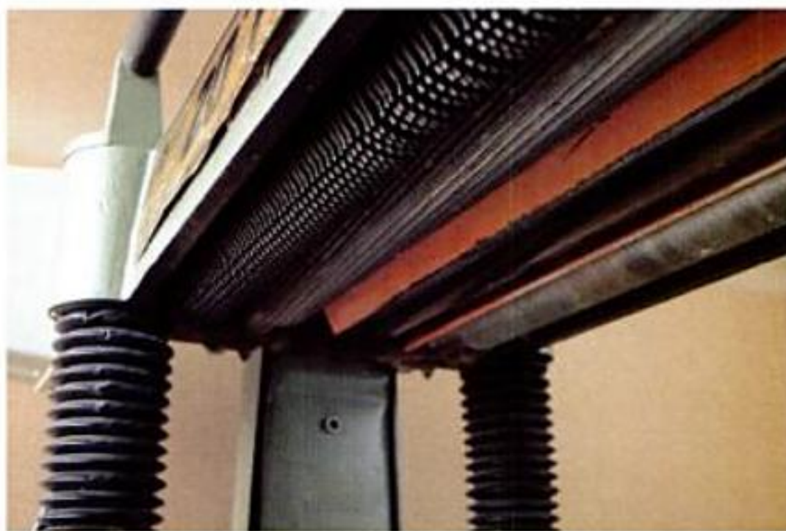
Infeed rollers. Serrated infeed rollers are effective in moving heavy boards through the machine.
