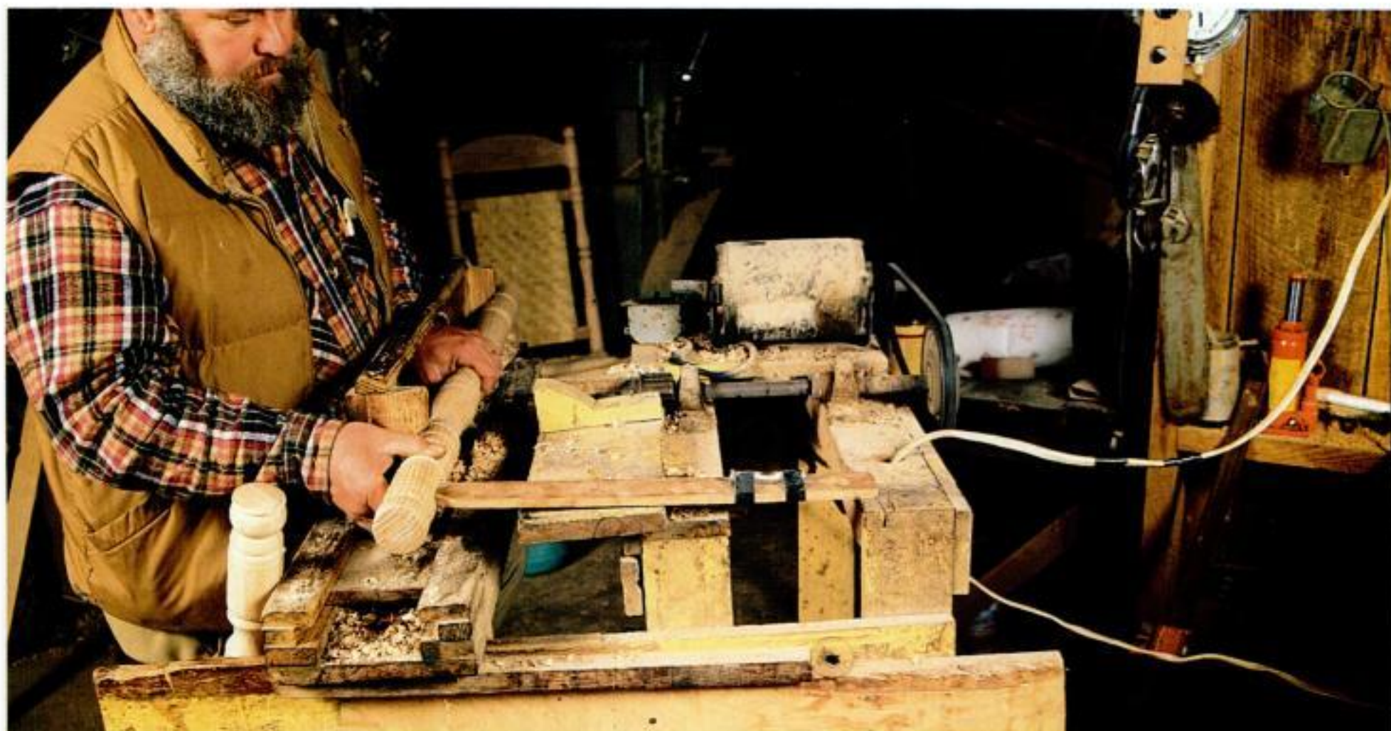
Drilling the holes. Harkins uses a shop-made drilling machine he calls a “belly punch” to drill the holes in the posts. To keep the holes aligned, he inserts a board into the headpiece mortise and reads a small level taped to the board.
