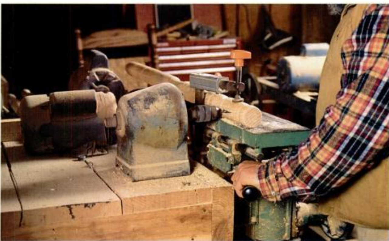
Slot mortising. Harkins cuts the mortise for the rocker's headpiece on a home-made slot mortiser. To provide maximum strength for opposing joints, Harkins orients the grain of the post at 45° to the axis of the mortise.
