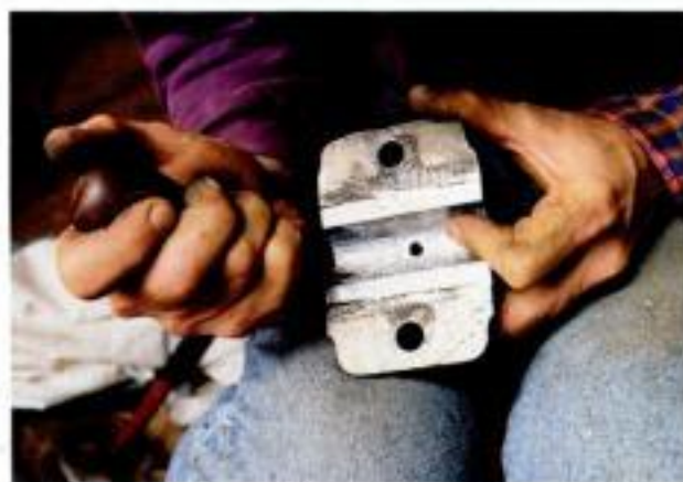
Letting it flow. Shallow channels carved into the top bearing will distribute oil evenly when the machine is running.
