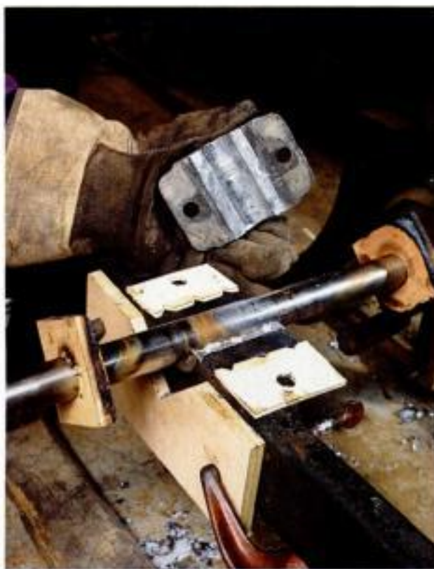
Moment of truth. When the metal hardens, McCarthy removes the top cap and files off the triangular sprues left by the notches in the cardboard.
