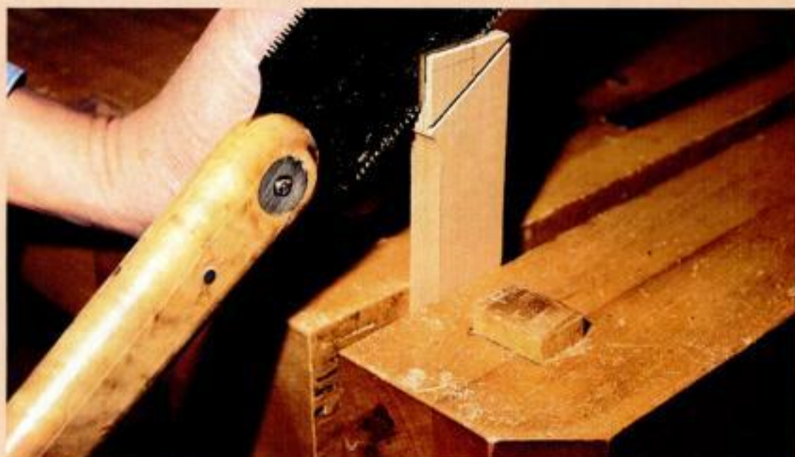
Thin-kerf work. Chan uses a Japanese ryoba saw to cut the tenon cheeks on a chair rail.
