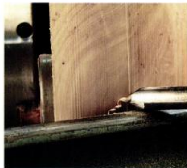
Shear cutting. Whether you're turning a foot (center), a cove or a bowl profile (right), start the shear cut with the gouge rolled over so the flute is facing sideways. Once you're in the wood, roll the tool slightly in the direction of the cut to get a larger shaving (right).
