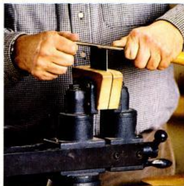
Form the hook. Draw the burnisher across the angled edge at a 15° angle.
