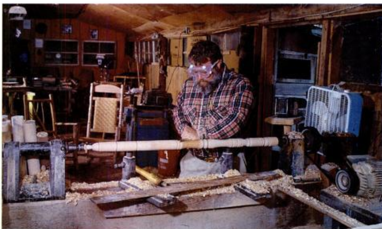
Turning post patterns. Harkins uses a skew to shape the hollows and bellies.
