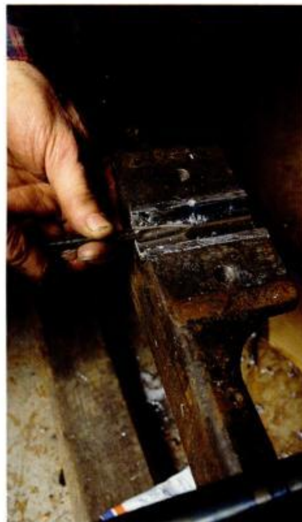
Tuning the fit. McCarthy carefully scrapes the blue high spots with a triangular scraper.
