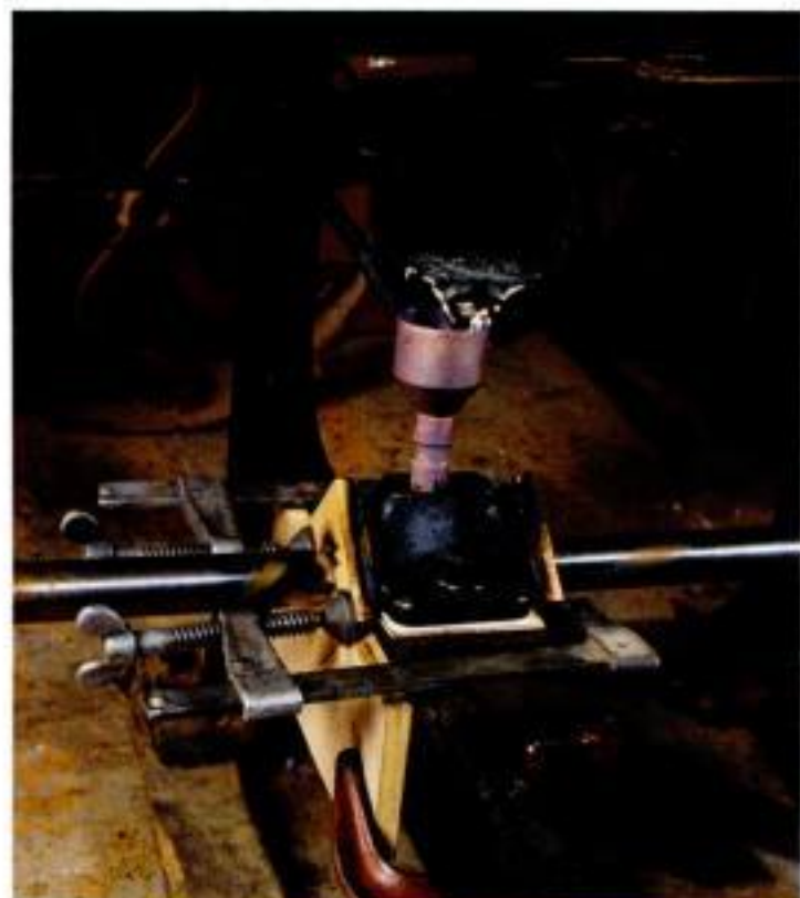
Page 50 Replacing Babbitt Bearings
