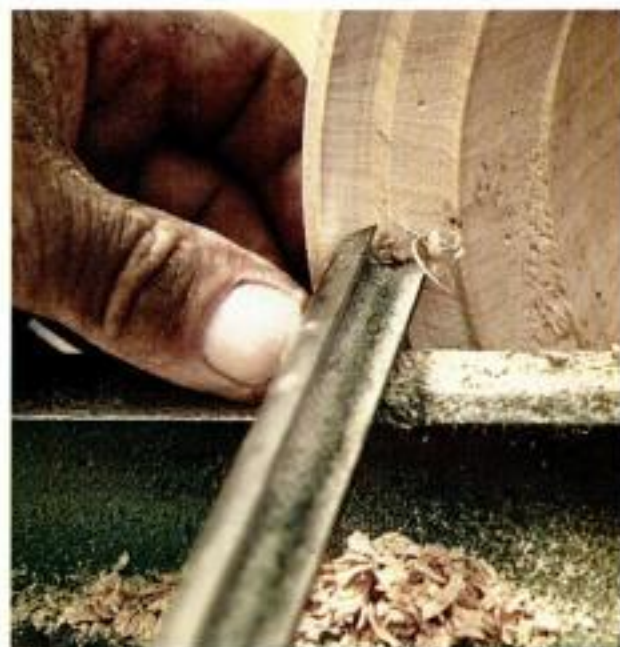
Standard hollowing cut. When hollowing the inside of a bowl with the deep-fluted gouge, keep the corner of the tool clear of the wood. Always cut from the rim inward.
