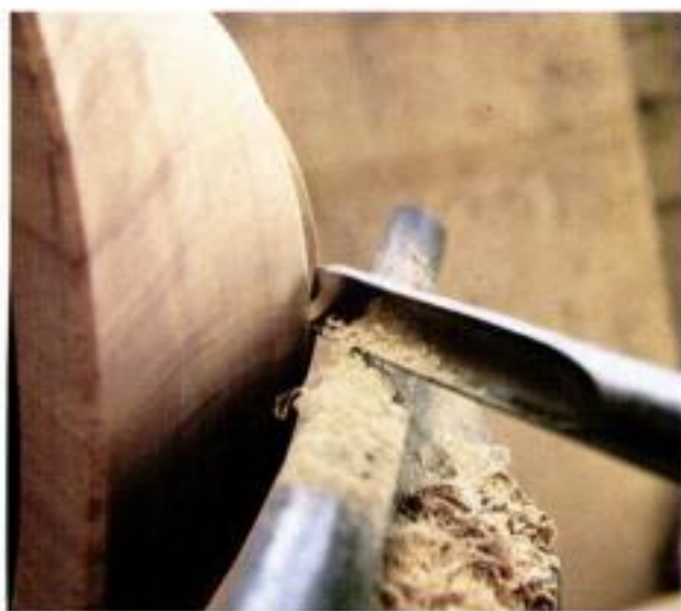
Shear scraping. With the flute of the shallow gouge facing the wood, shear scrape by brushing the edge lightly across the surface.
