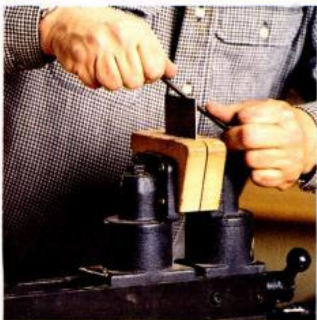
File at 45°. Use a mill file to create a straight edge at a 45° angle.
