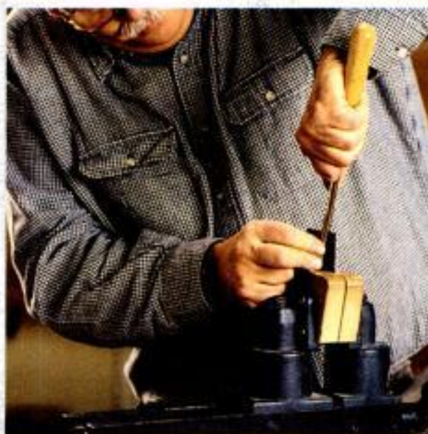
Burnish the back edge. Flatten the back of the blade with the burnisher.
