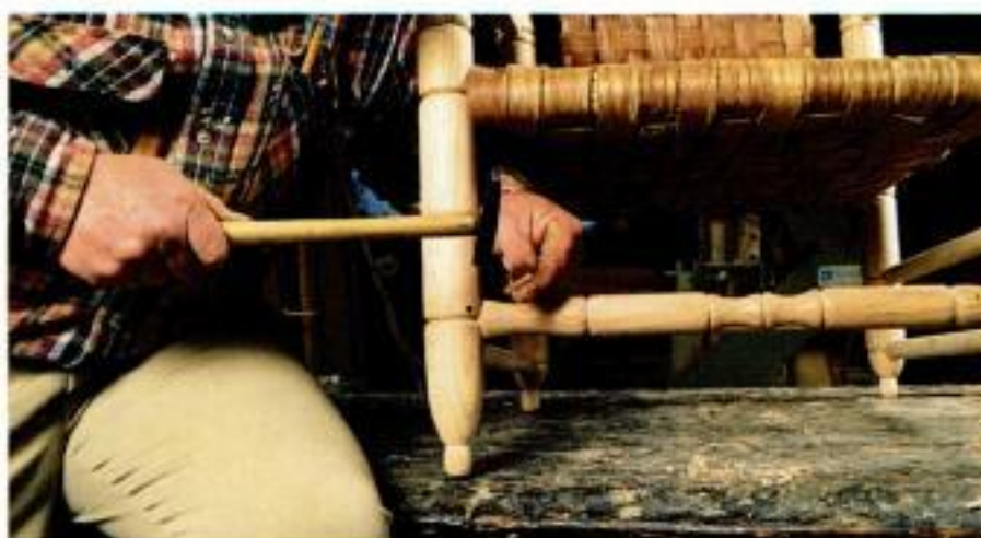
Pegging the joints. Harkins taps a wooden peg into a predrilled hole to lock the foot round to the front post.
