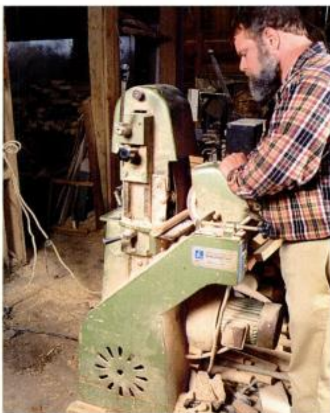
Sanding round. Rough-turned chair rounds are fed through this dowel sander, using 80-grit followed by 220-grit belts. A rotating wheel turns the spindle steadily against the sanding belt for a perfectly round, smooth surface.
