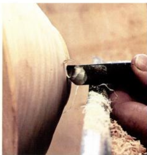
Back-cutting. With a deep-fluted gouge, make a back-cut using the inside cutting edge, supporting the tool with the steep side bevel. Don't let the inside shoulder of the edge roll into the wood or it will catch.
