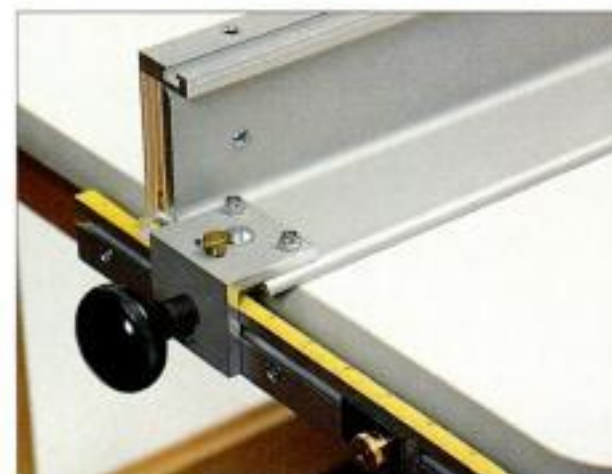
Optional adjuster. Woodhaven's optional fence adjuster accessory works like a table-saw fence. A scale and cursor let you locate the fence precisely and lock it parallel to previous settings.
