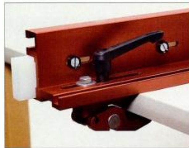
Tight-gripping cam clamp. A half-turn of the handle locks Woodsmith's fence securely.
