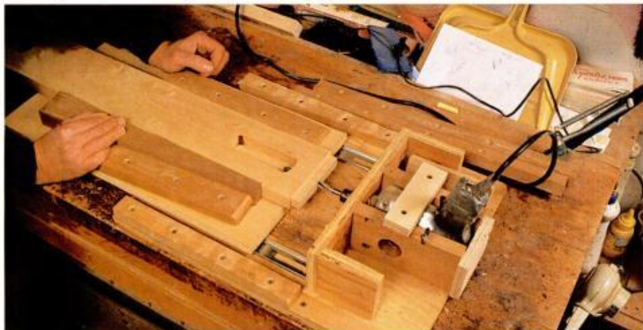
Boring the bolt holes. The author's $23 shop-made boring jig makes short work of drilling bolt holes in the ends of the front and back rails.
