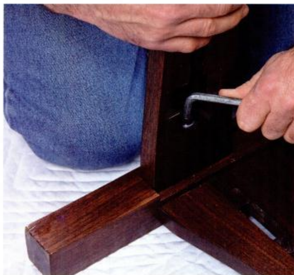
Putting it together. To assemble the knockdown rail joint, insert the tenon into the mortise and tighten the bolt.
