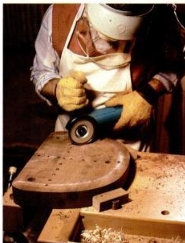
Shaping the seat. First the author drills a series of holes in the top of the seat, using a depth-gauge jig cut to approximate the finished contours (left). Then he carves to the depth of the holes, using a right-angle grinder fitted with a carving wheel (right).
