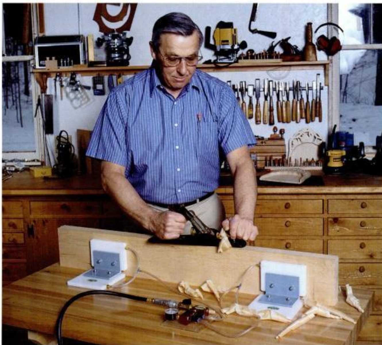
One-sided clamping. Spielman planes a board held by a pair of right-angle vacuum-clamping fixtures. Suction holds the fixtures to the bench and to the workpiece. The small venturi vacuum pump on the bench is driven by compressed air.
