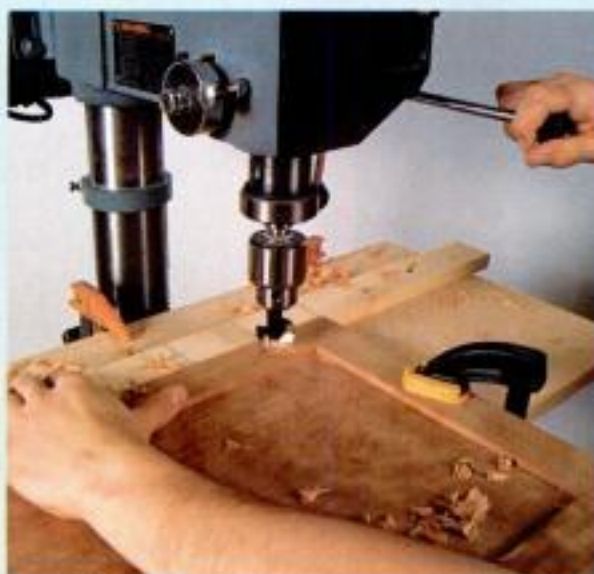
Drilling the door. Using a 35mm bit, Levine bores the hole for the hinge cup. Driving a pair of screws will install the hinge mechanism.
