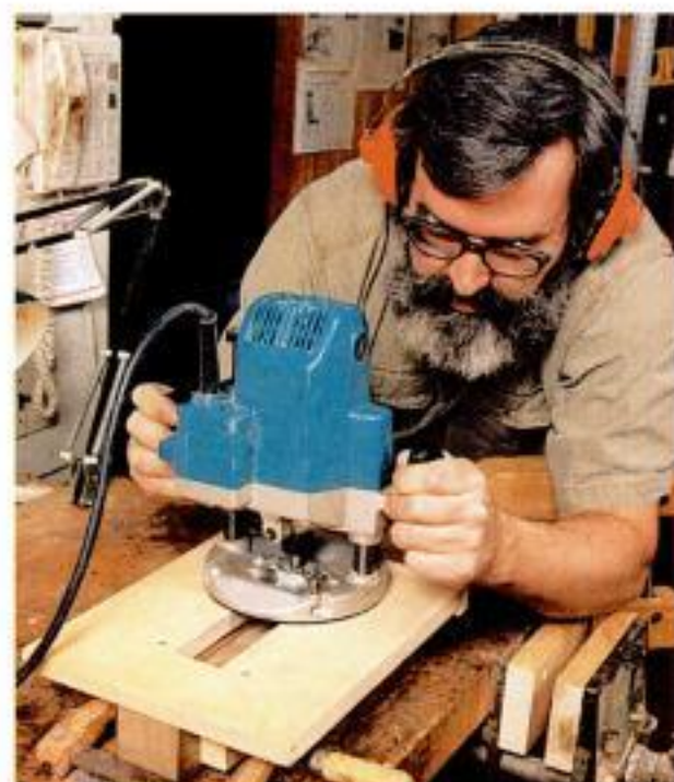
Routing tapered recesses. Lohr routs the recessed foot details on the posts using a wedged template to create the taper.
