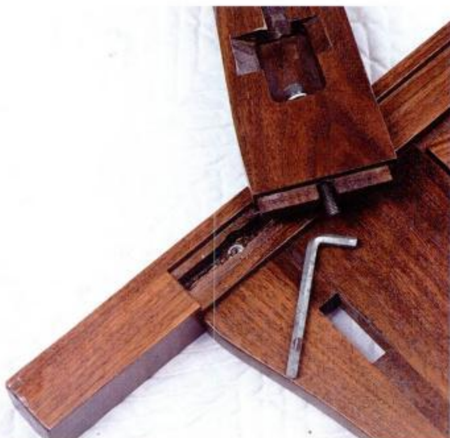
Putting it together. To assemble the knockdown rail joint, insert the tenon into the mortise and tighten the bolt.
