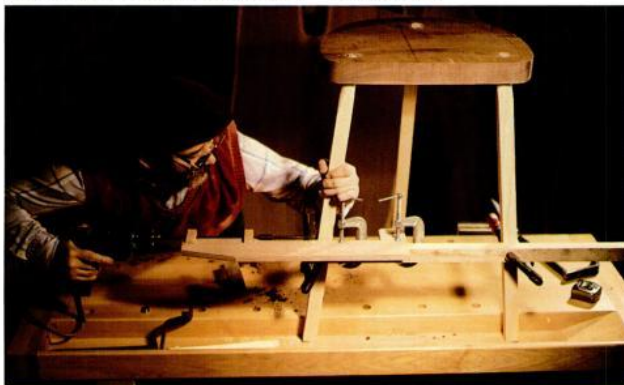
Drilling the legs. To bore the angled holes for the stretchers, the author clamps the arm of the drilling jig in position to guide his drill.
