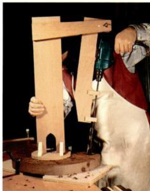
Drilling the seat. Marian's shop-made drilling jig is clamped to the underside of the seat to bore the three leg holes. The jig guides an extension bit chucked in a portable electric drill.
