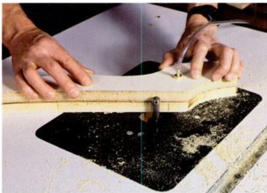
Easy-on, easy-off. A vacuum template lets you pattern-route with a flush-trim bit without marring your workpiece with fasteners.
