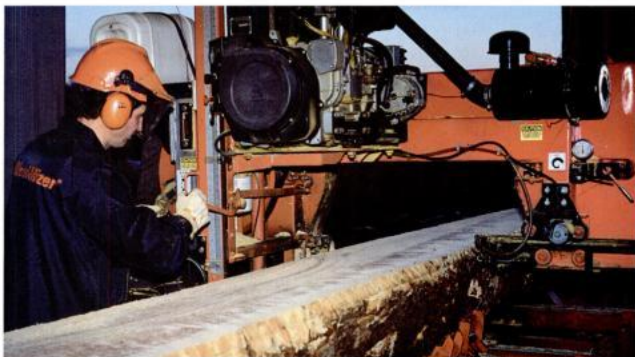
Custom cutting. Albert Bartel, a sawyer at Groff & Hearne, cuts a 5/4 slab of curly cherry with his diesel-powered bandmill. On-site cutting enables lumber dealers to fill custom orders and get the best lumber out of each log.
