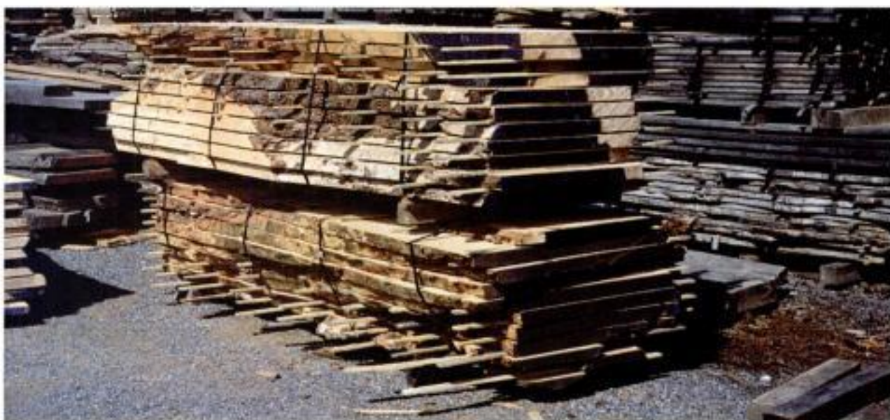
A log's-worth of lumber. Specialty lumber dealers can cut and sticker a log "in the boule," so that boards hold the same relative position they had before milling. This enables woodworkers to build a project using wood from the same tree—an important consideration when wood grain and color need to match.
