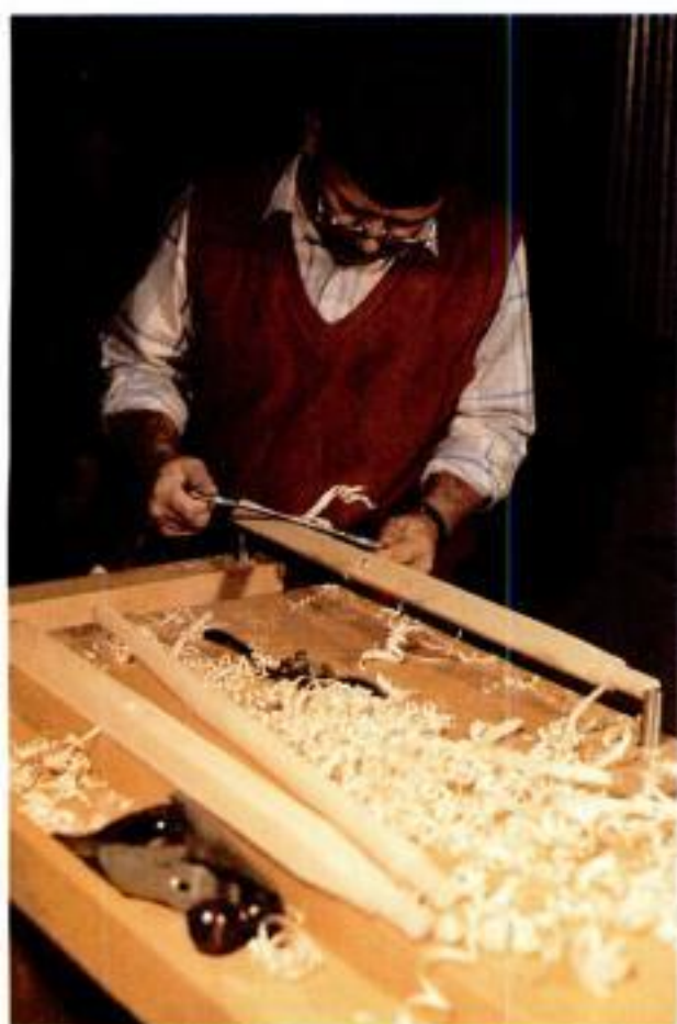
Shaving the legs. With the workpiece clamped between bench dogs, Marian uses a drawknife to shape the legs.
