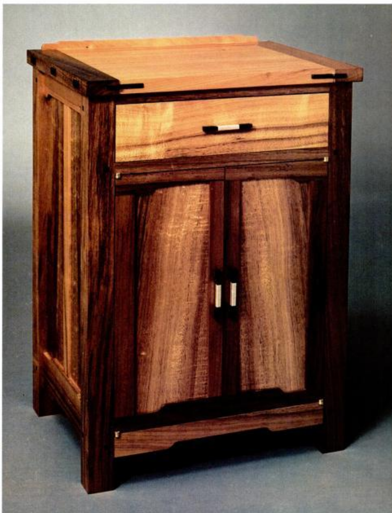
Interpreting a tradition. Accented joinery, curved "cloud-lift" frame rails and handmade handles are details inspired by the work of turn-of-the-century architects Charles and Henry Greene.
