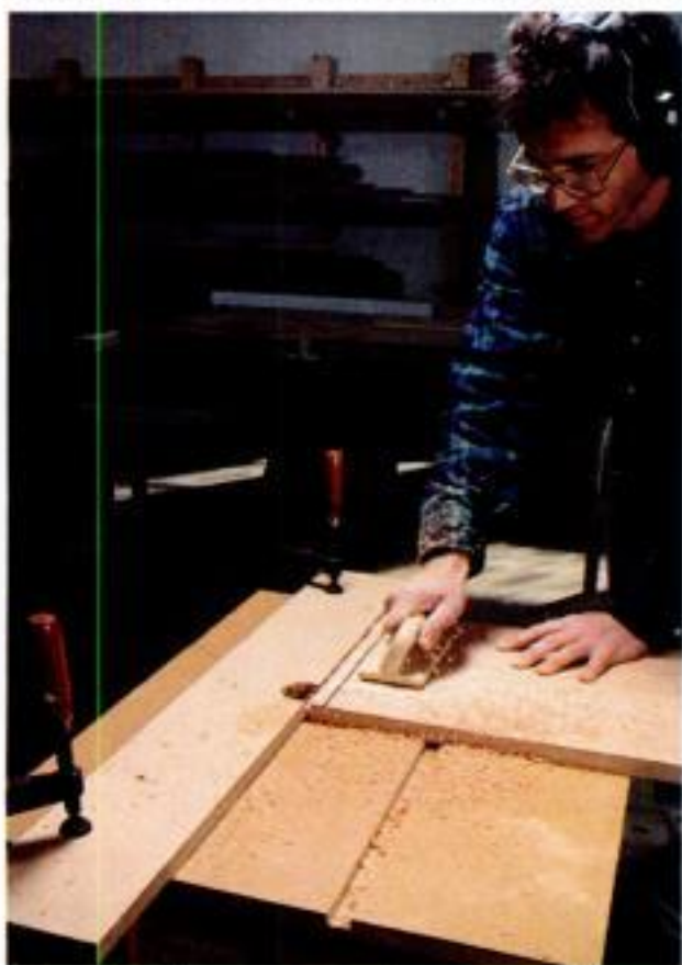
Routing the tongue. Korn routs both sides of each tongue, removing \frac{5}{16} in. of wood with each pass before repositioning the fence.
