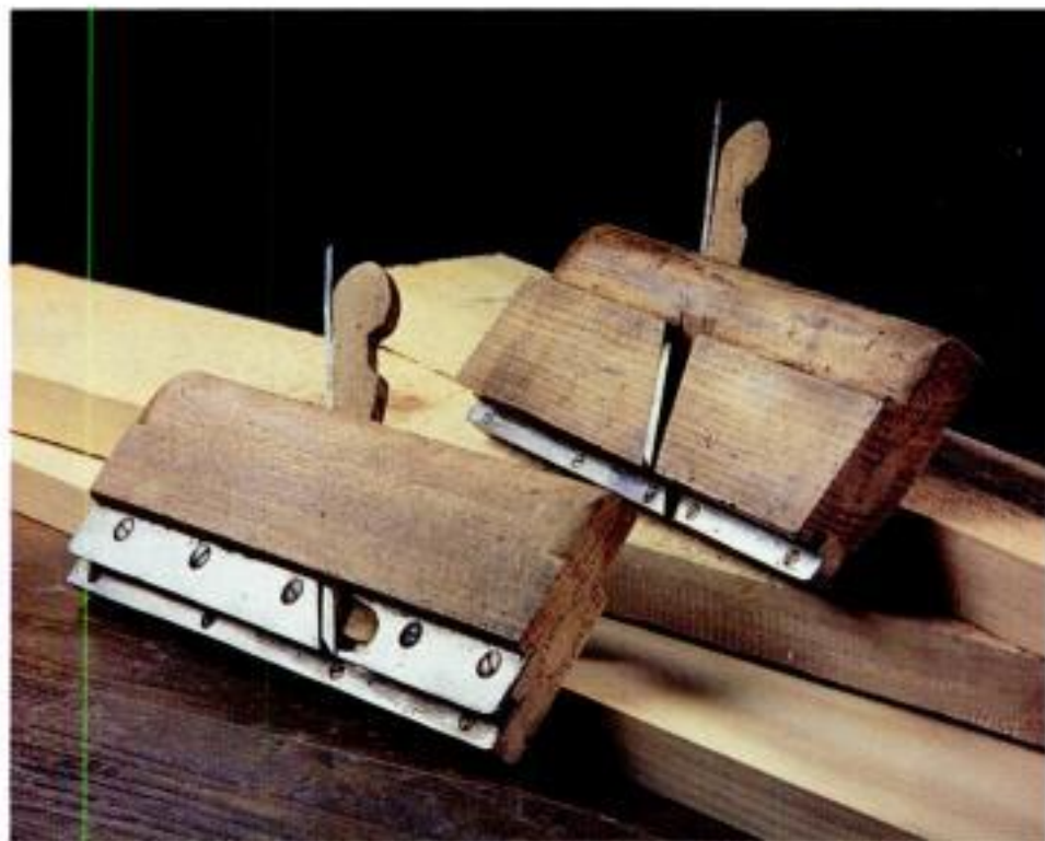
A matched set. Fitted with steel plates to eliminate wear, these wooden match planes were made by Casey, Clark & Co. around 1880.
