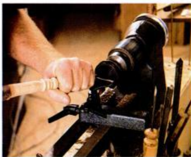
"Chattering" the inside. Pulling from the center out, Paulsen cuts a ring of chatter that resembles beaten metal on the inside of a bowl.
