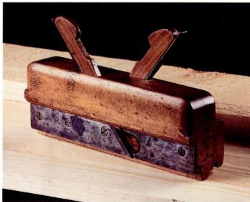
Two in one. Made during the late 1800s, this wooden combination match plane by Mockridge & Francis contains both tongue and groove cutters.
