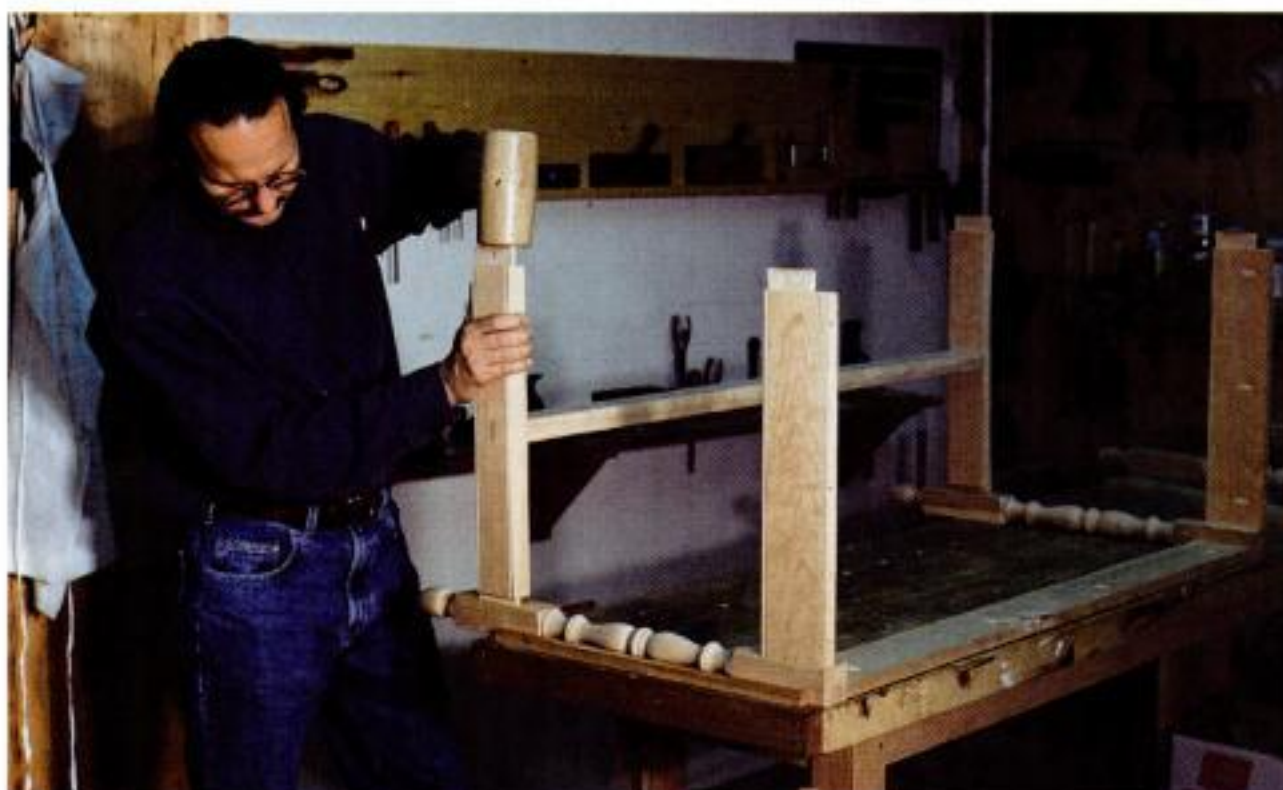
Tapping the tenons home. With one base side assembly flat on the bench, Burak installs the end aprons and stretcher assembly. The remaining side assembly will go on last.
