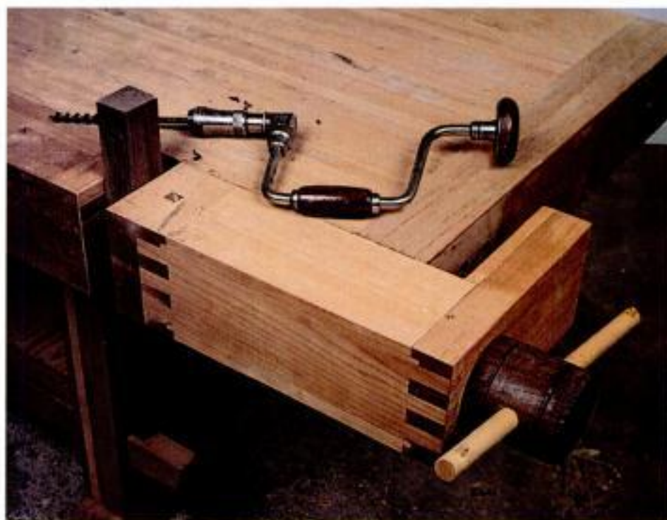
Put on the squeeze. Add European-style stock-holding capabilities to any sturdy workbench with this shop-made tail vise.
