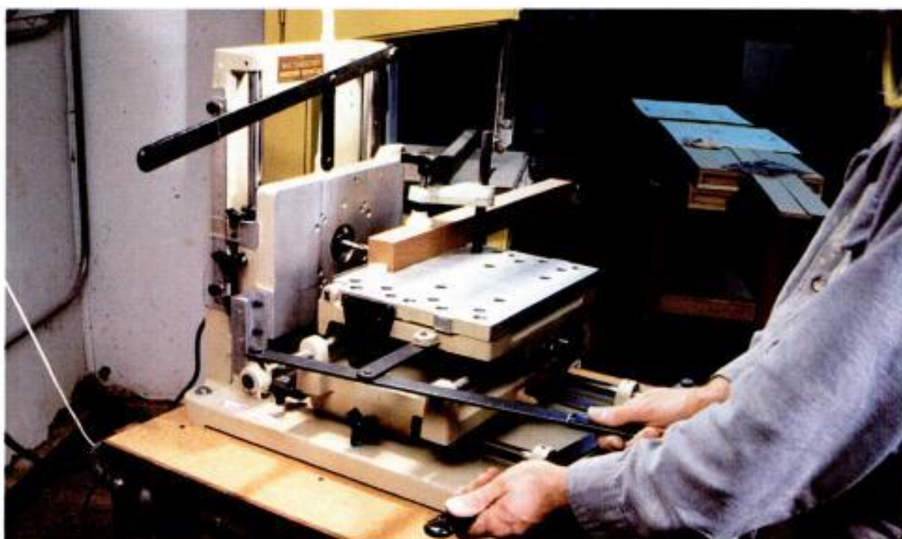
"Multi-Routed" mortises. The author cuts mortises using a Multi-Router, a machine that lets you rout slots in wood precisely.
