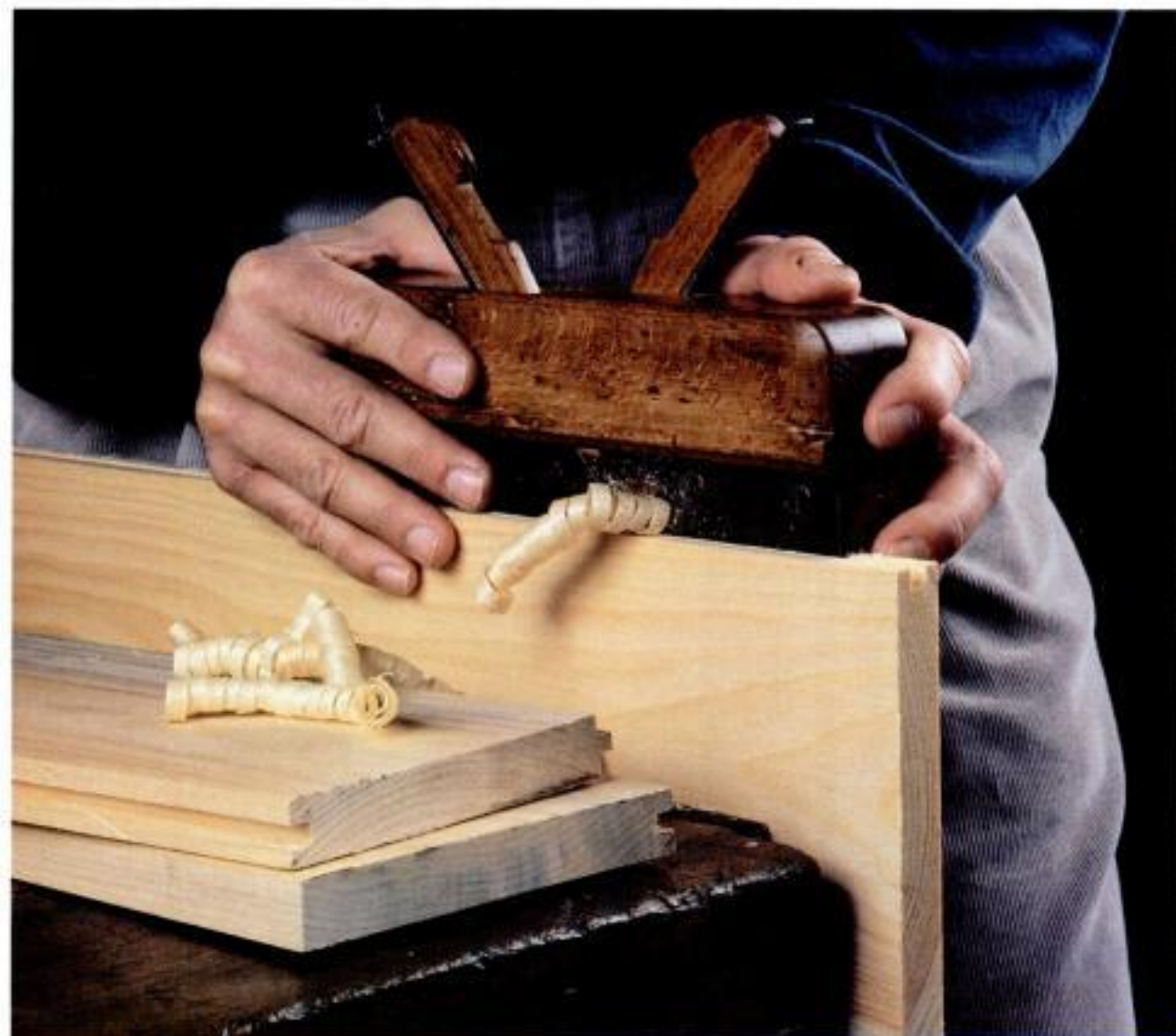
Works like new. Passed through generations of woodworkers, this century-old combination match plane still cuts a first-rate joint.
