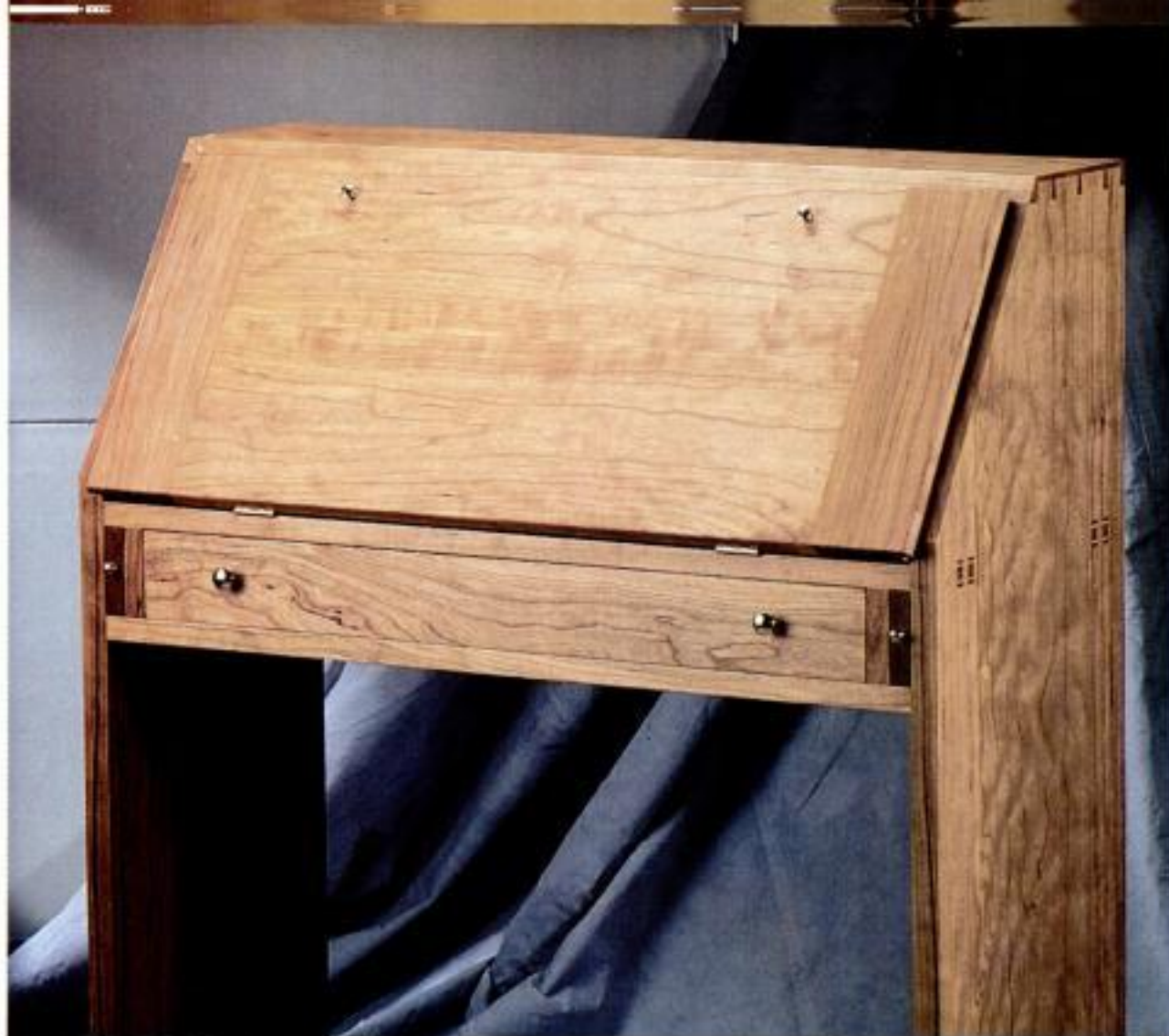
No cupping here. Breadboard ends on the author's fall-front desk lid keep the solid-wood panel from cupping.
