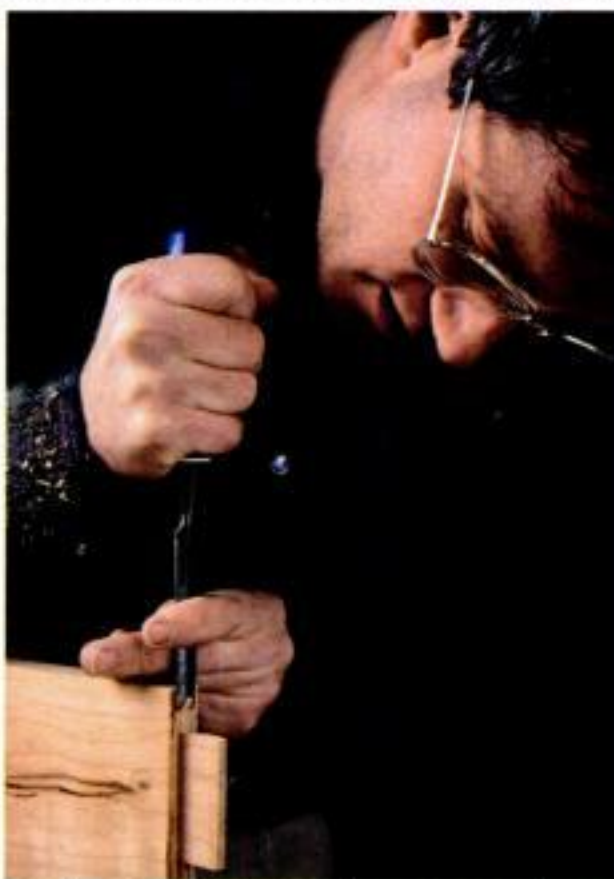
Paring the tongue. After cutting the tenons on the bandsaw, Korn pares off the tongue near the edges of the panel.
