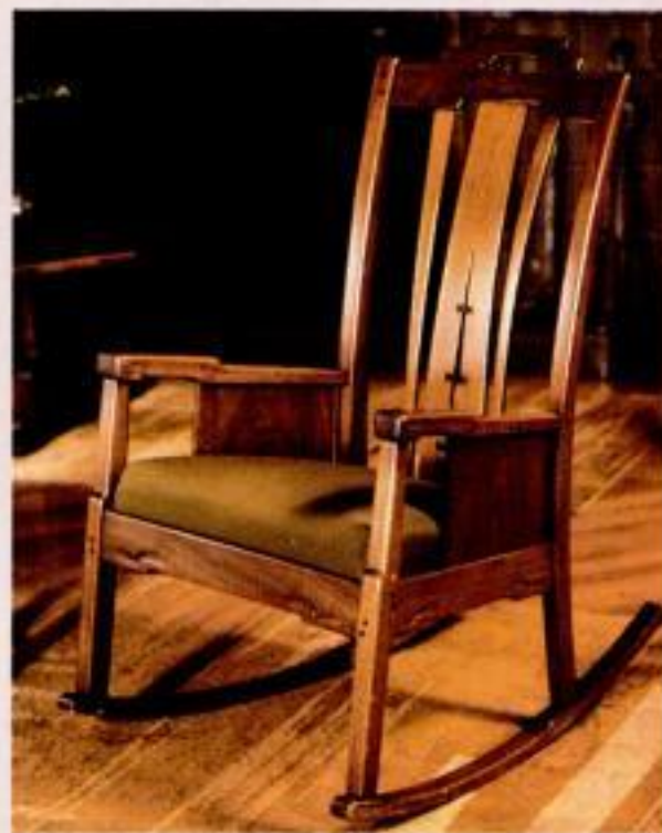
Integrated elements. This rocking chair combines pegged through tenons, Oriental "cloud lifts" on the arms, and ebony splines.
