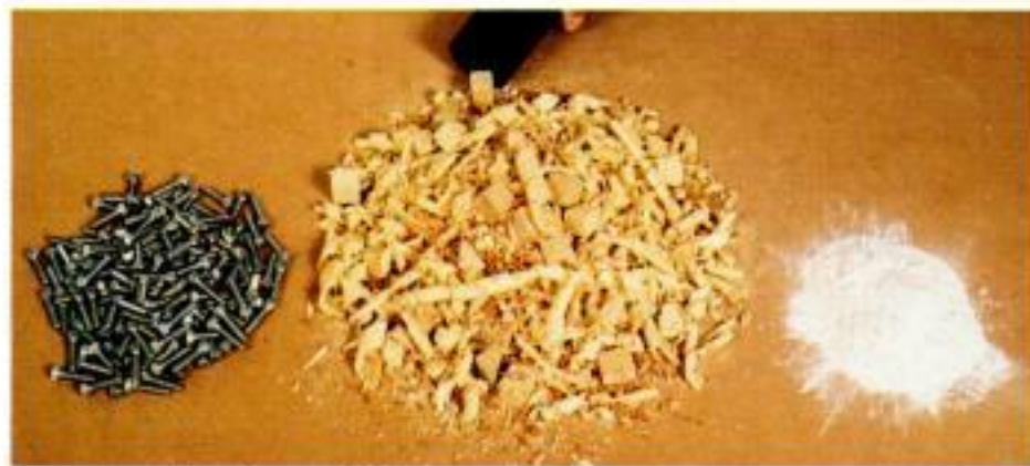
Heavy, chunky and fine. To test performance and filtering efficiency, we picked up piles of mixed debris, 1-in. bolts, and fine drywall dust.
