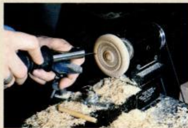
Vibrating chisel. The tip of this tool flexes as it presses against the spinning work, creating a pattern of chatterwork.
