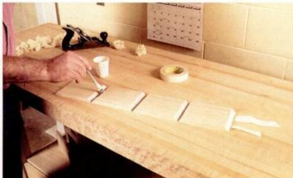
Taping it tight. To glue up a small box with mitered corners, Bird lays the mitered sides end-to-end onto the sticky side of masking tape. Then he applies glue, folds the sides together and draws the miters tight with the tape.
