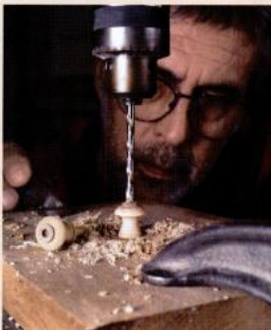
Second hole. After gluing a walnut plug in the knob, Layport bores the hole for a 3/16-in.-dia. maple plug.
