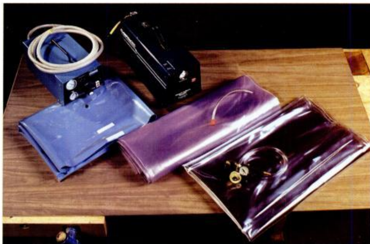
Pumps, bags and fittings. There are three different types of pumps for vacuum pressing. All three use similar vacuum bags and fittings. Left to right: a 5-cfm automatic venturi, a 5-cfm electric pump, and a 2.2-cfm manual venturi.
