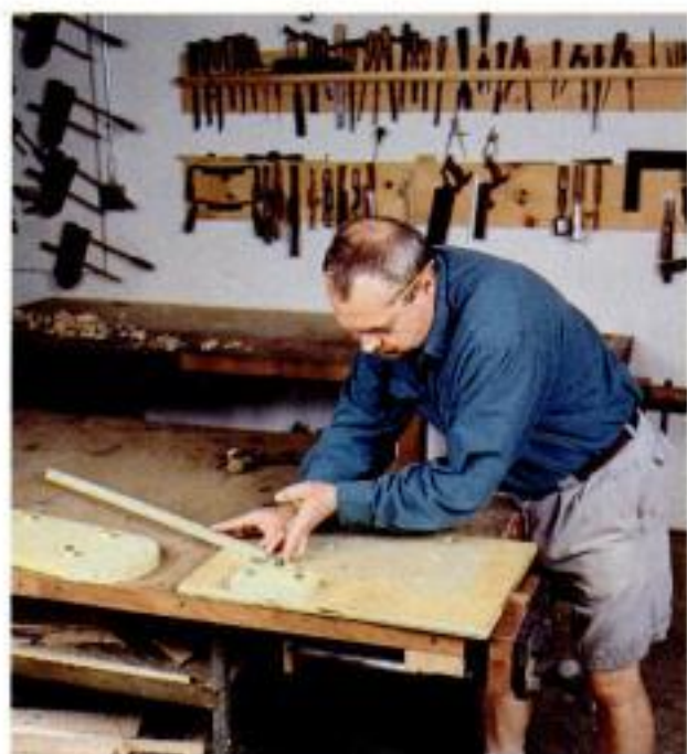
Small bend. With the tip of the workpiece clamped, Dunbar lifts the free end up to make the small bend.
