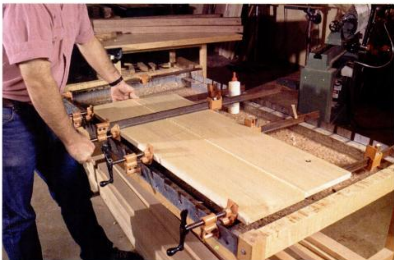
Over and under. Alternating clamps on both sides of an edge-to-edge joint prevents the panel from cupping.
