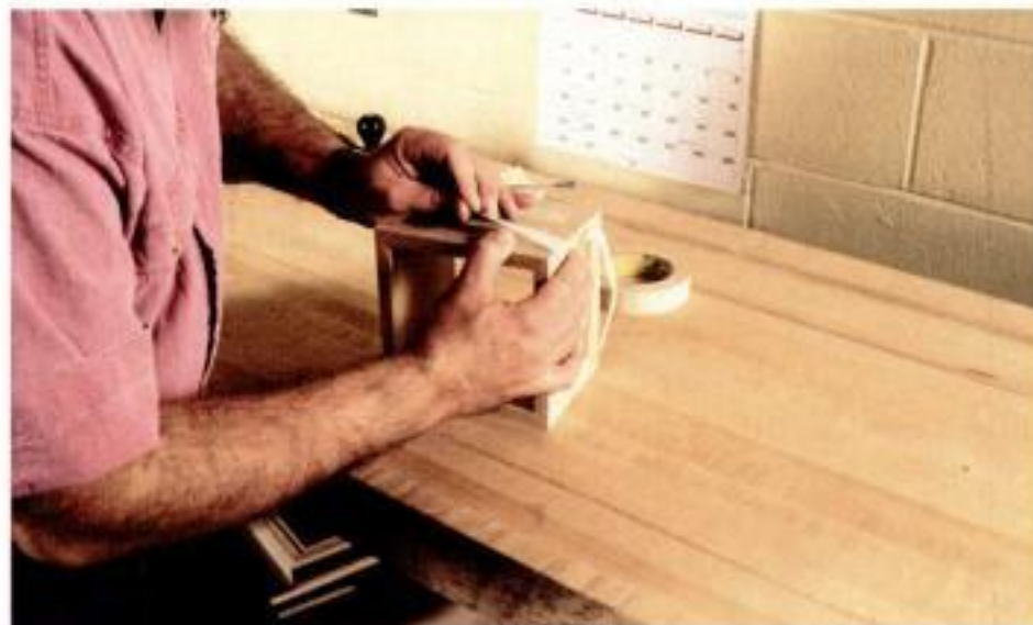
Taping it tight. To glue up a small box with mitered corners, Bird lays the mitered sides end-to-end onto the sticky side of masking tape. Then he applies glue, folds the sides together and draws the miters tight with the tape.
