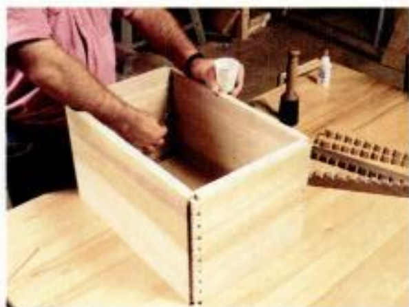
Good brushwork. With the corner joints partially assembled, Bird uses a flux brush to coat the dovetail pins with glue.
