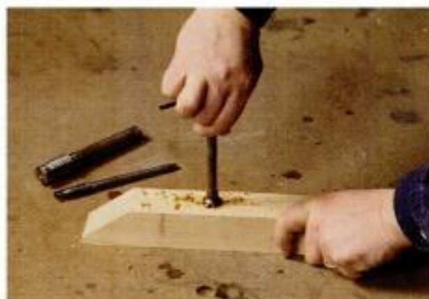
Tapping the jaw. Holding the tap vertical, Dunbar starts the thread with firm downward pressure.
