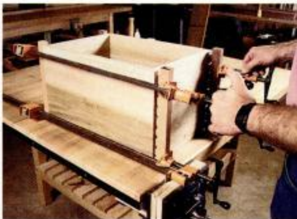
Notched blocks. Positioned at the corners, notched clamping blocks allow the pins to protrude but ensure that the tails are clamped tightly.
