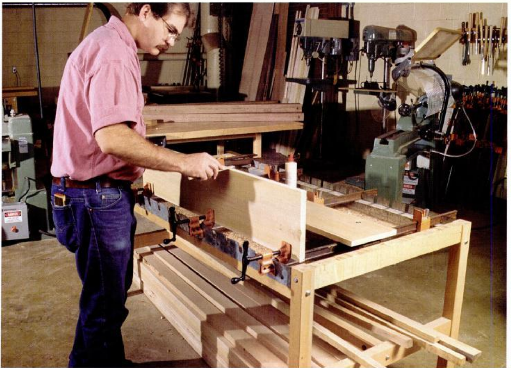
Good preparation. A rack holds clamps at the ready as the author begins spreading glue on the edge of a board.
