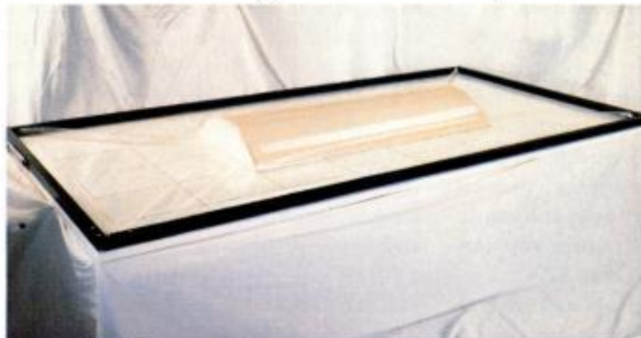
The membrane press from Mercury Vacuum Presses has a silicone rubber membrane.
