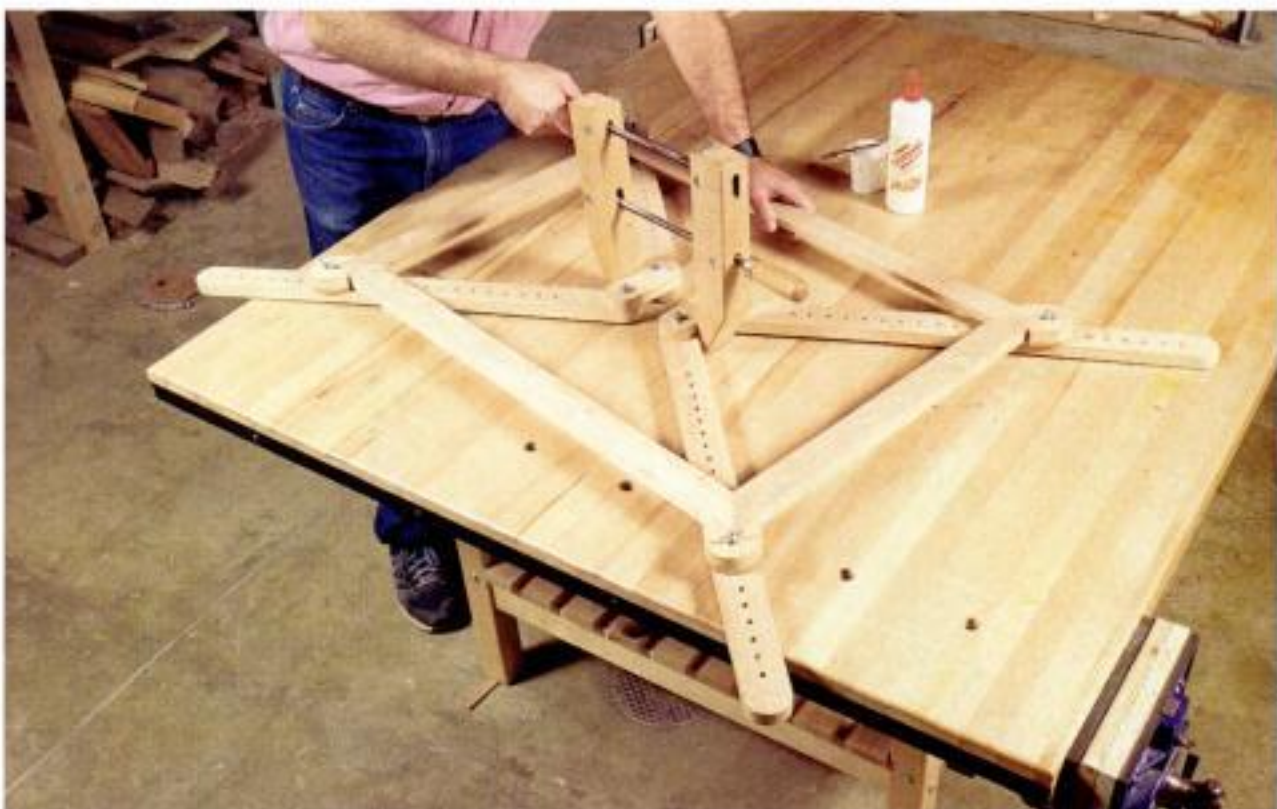
Tight miters. This shop-made jig pulls miters tight and square with pressure from a single handscrew clamp.
