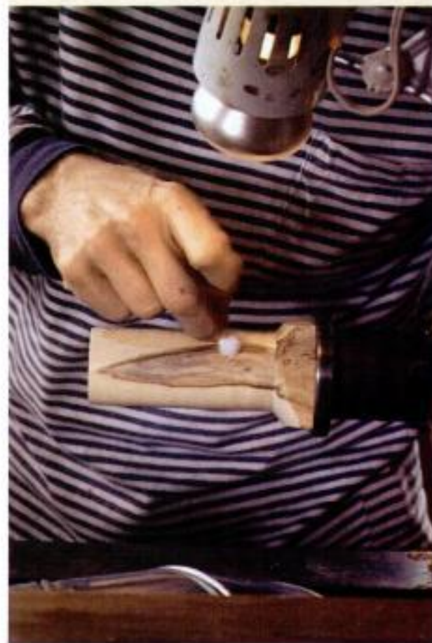
Super sealer. With the lathe turned off, the author applies cyanoacrylate sealer to a maple practice piece that he has sanded to 320 grit.
