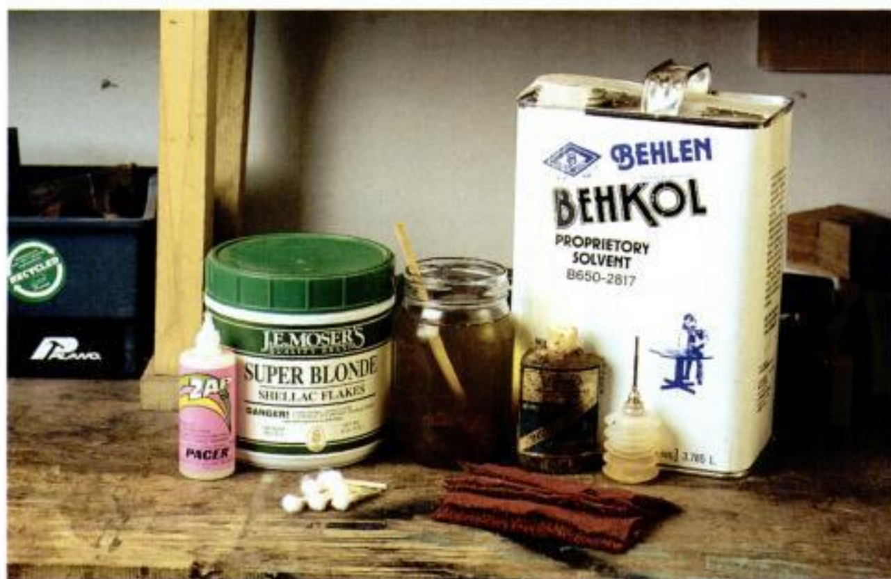
Finish, pads and brushes. Mode uses squeeze bottles to apply shellac and linseed oil to his cotton-velour French polishing pads. He applies his cyanoacrylate glue "sealer" with tiny shop-made glue brushes.
