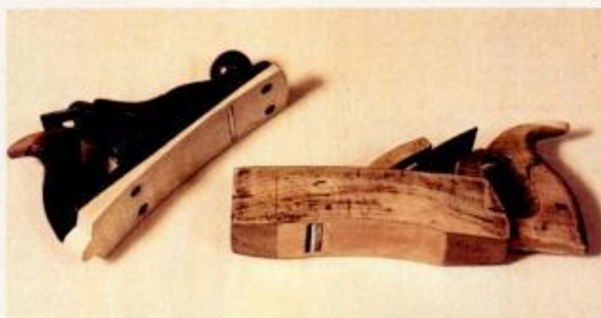
Customized for curves. Planemaker Cecil Pierce modified a "clunker" Stanley No. 4 plane to accept interchangeable wooden soles of various radii. The old wooden plane at right was shaped to a dedicated 14-in. radius.
