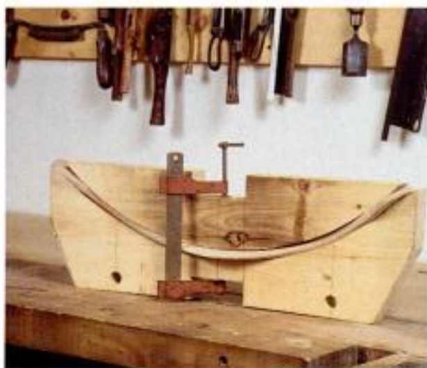
Two-part form. Designed to bend the crest of a Windsor chair, this form can be pulled tight and held with a single bar clamp.
