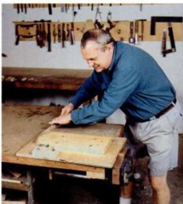
Big bend. After fitting the large form member to the base, the author pulls the workpiece around it.
