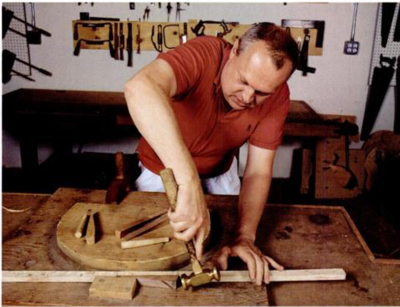
Beginning the bend. Fresh from the steam box, the oak workpiece is secured with its midpoint positioned against the centerline of the bend. Wedges and pegs stand ready to secure the oak against the form.
