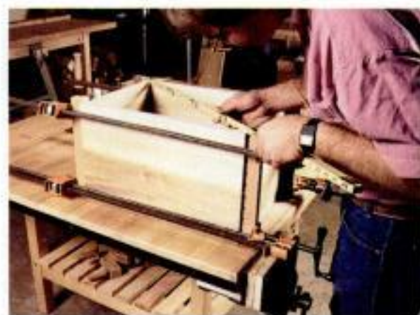
Measuring for square. Once the case is clamped, Bird uses a folding rule to check for square by comparing diagonal measurements.
