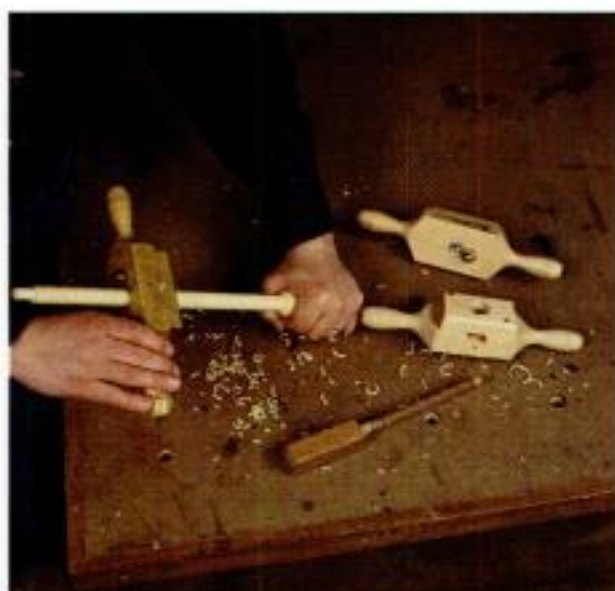
Threading the rod. Once the thread is started, Dunbar removes the screw handle from the vise and completes the thread by turning the die.
