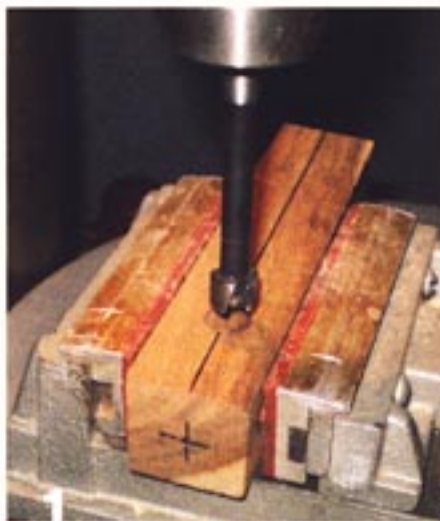
Drilling the 1/2" hole.
