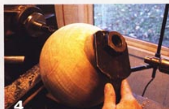
4 Slightly thread the faceplate onto the tenon.
