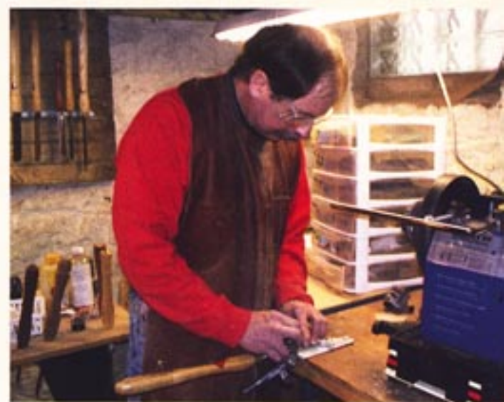
Dennis setting up a turning tool in a jig for sharpening on the Tormek.
