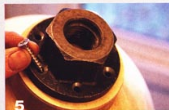
5 I'm using #12, 1¼" screws (SPAX brand) to secure this particular faceplate to the vessel.
