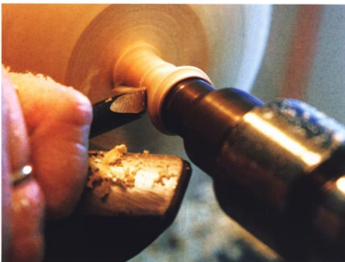
The vessel's bottom is made slightly concave and the nub is turned smaller.
