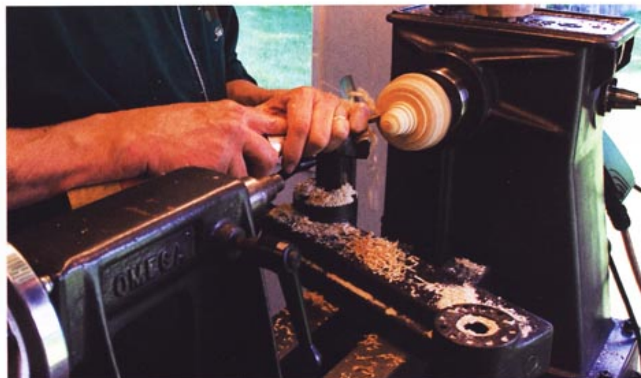
Turning a tenon and shoulder on a waste block to fit the vessel's opening.
