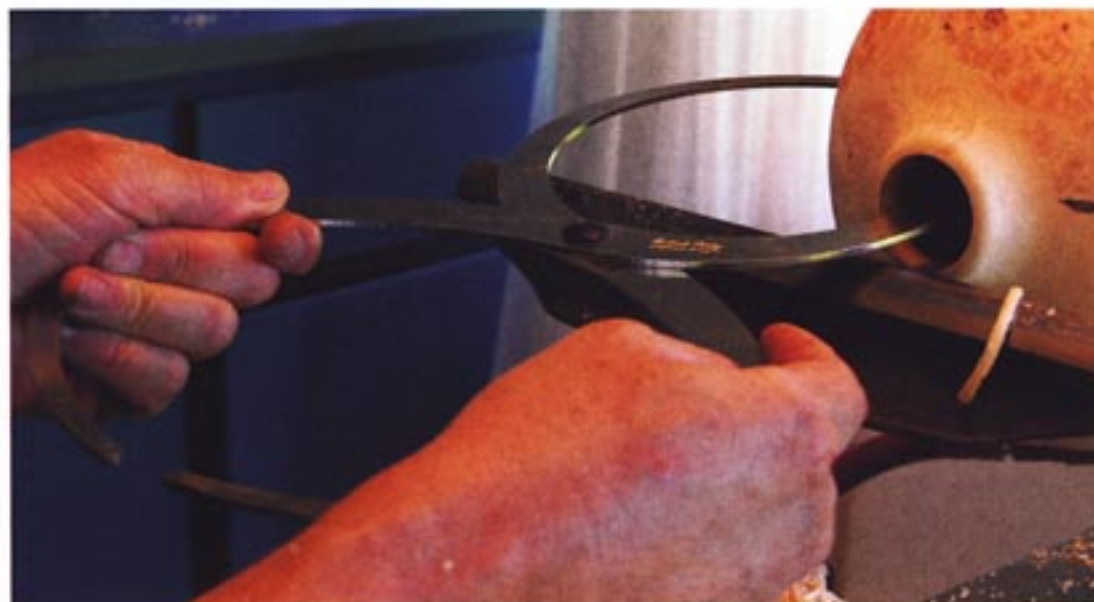
Measuring wall thickness with calipers.
