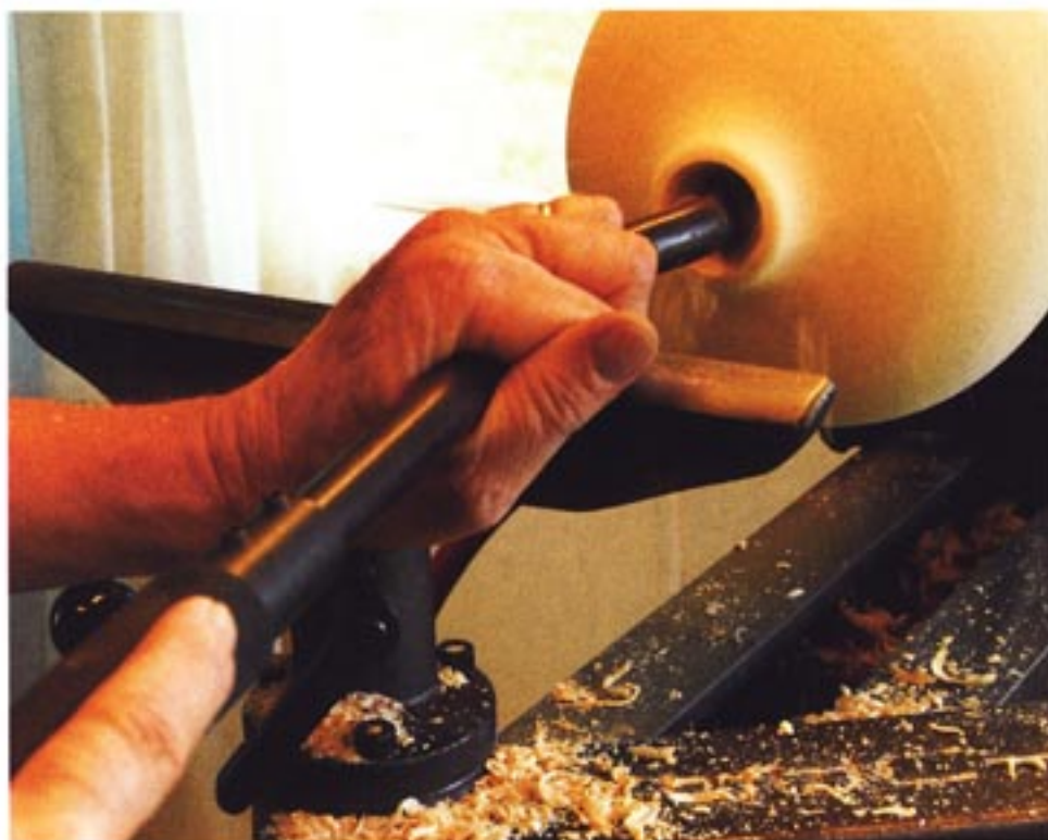
First cuts with a hook tool to open the shoulder.
