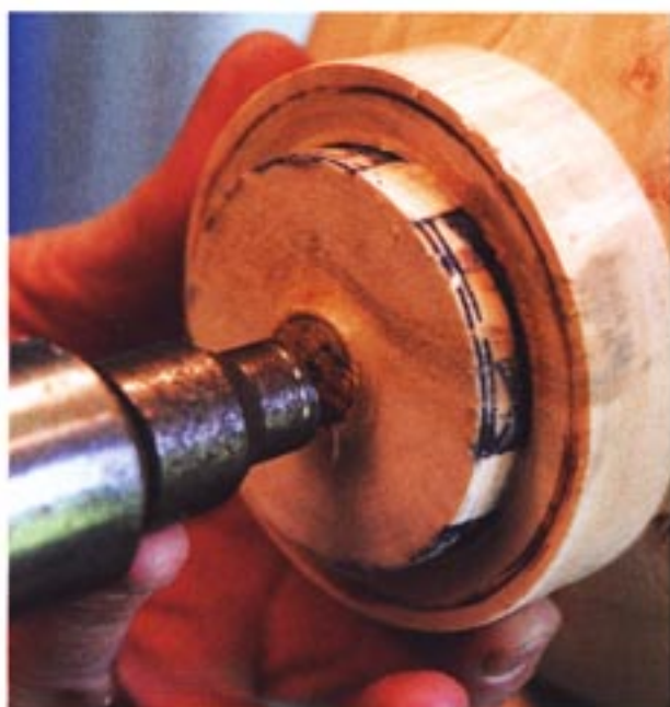
Revolving tailstock center is used to put light pressure on the vessel against the waste block.
