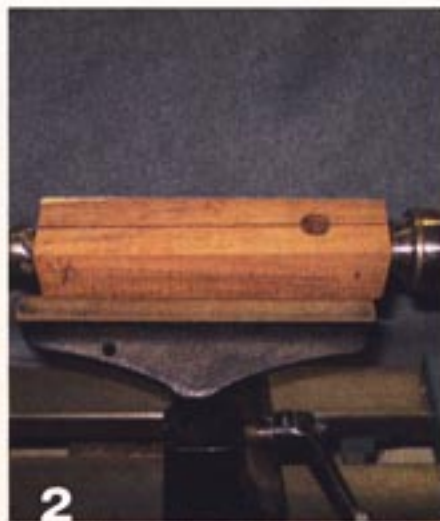
The turning blank mounted on the lathe. Note the smaller 1/8" hole located on the wood, positioned just above the right-hand side of the toolrest.
