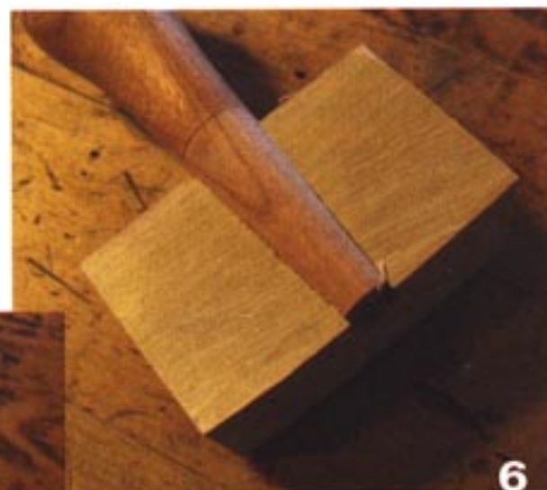
(Above) The tenon in the test block shows a snug fit.
