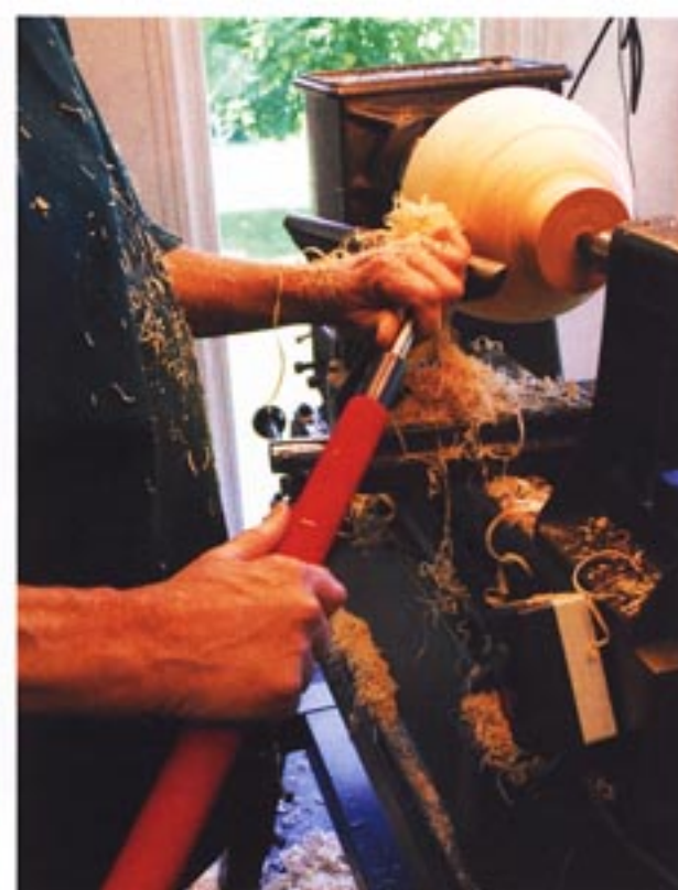
Rough shaping between centers.
