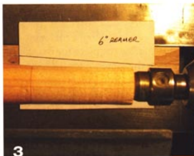
(Right) The angle of the tenon is now parallel to the line on the template showing that the tenon now has the correct taper.
