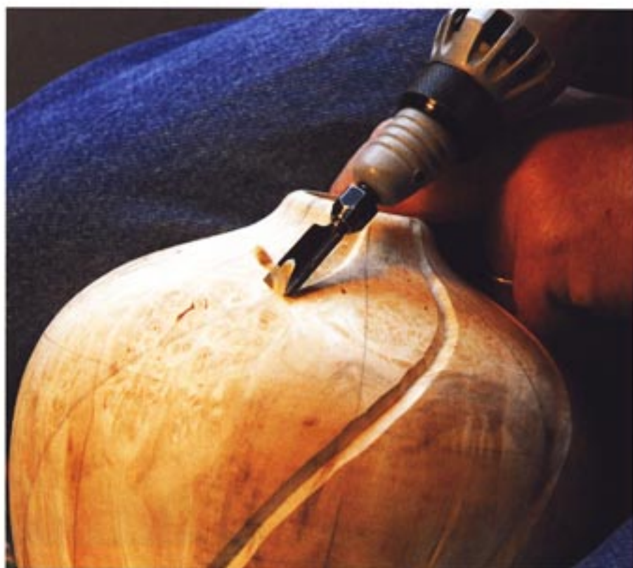
Initial carving is done with a reciprocating carver and V-gouge.
