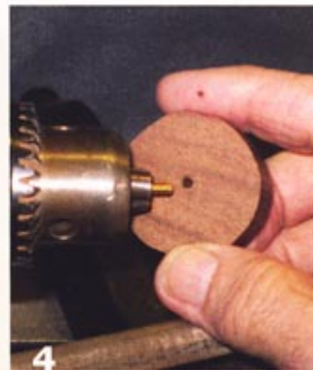
The brass rod mounted in a Jacobs chuck. Mount the wheel blank onto the brass rod, then bring up the live center of the tailstock before turning the shape of the wheel.
