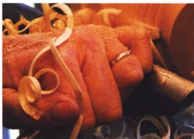
Rough shaping between centers using a 1/2" side-ground bowl gouge to establish a tenon for mounting in a chuck.
