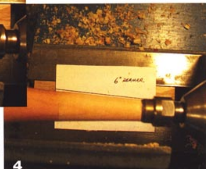
(Right) The angle of the tenon is now parallel to the line on the template showing that the tenon now has the correct taper.
