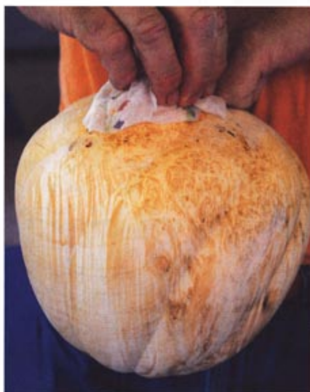
The surface of the vessel is wetted between each round of sanding and detailing.
