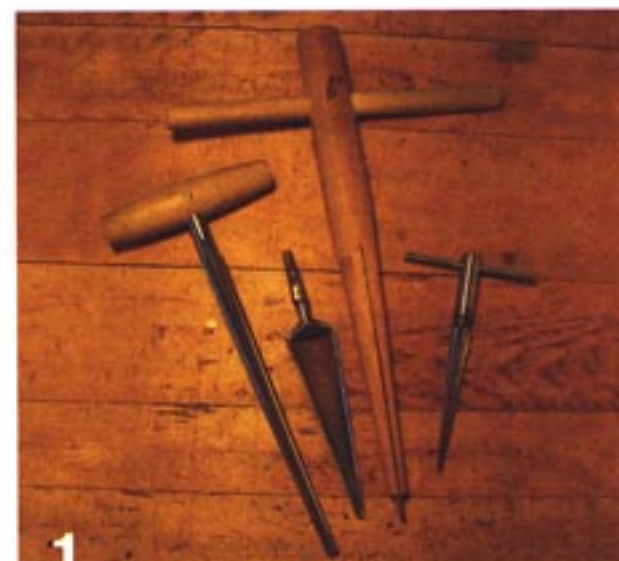
1 Reamers come in a variety of angles, sizes and types. From left to right: A cello reamer, a spoon bit style reamer for use in a brace, a shopmade wooden reamer and a hardware store plumbers reamer.
