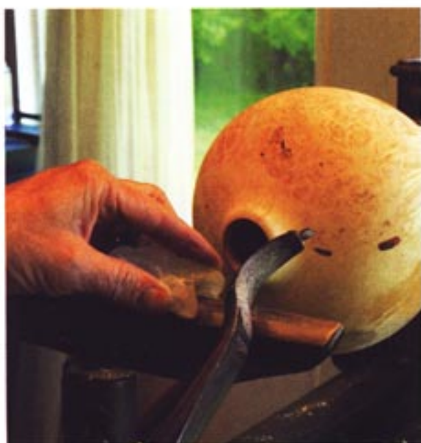
Wiping paraffin (wax) on toolrest and tool to reduce friction before final cuts are made.
