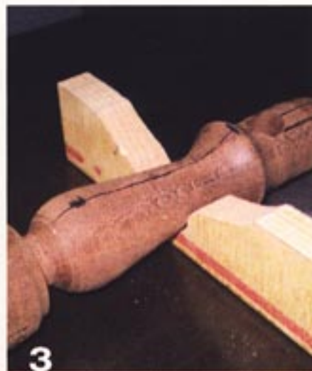
Handle of the crimper turned and mounted in a block, ready to have the waste removed for the slot.
