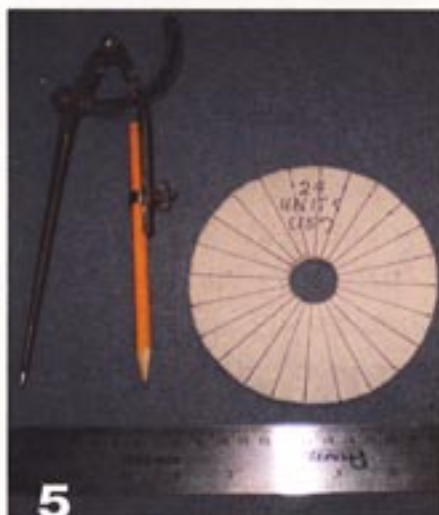
5 Shopmade indexing wheel with the tools needed to create it.
