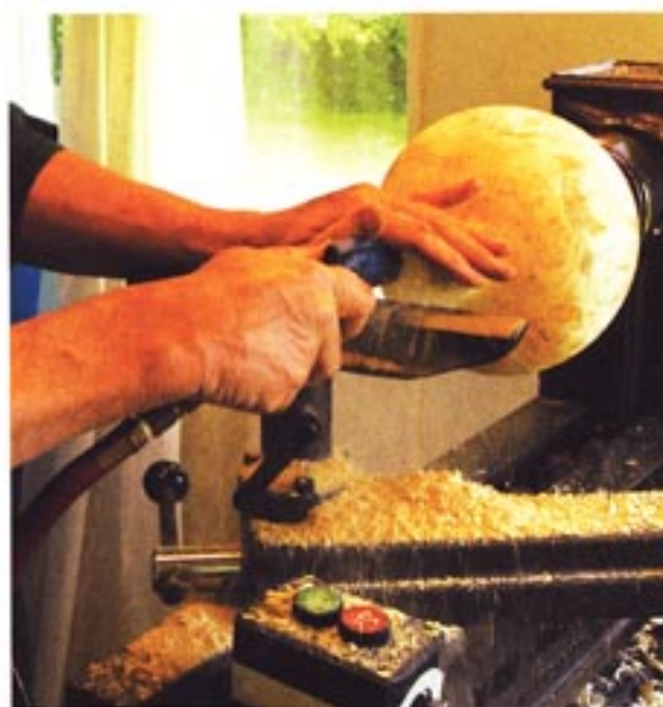
Blowing out shavings with compressed air.
