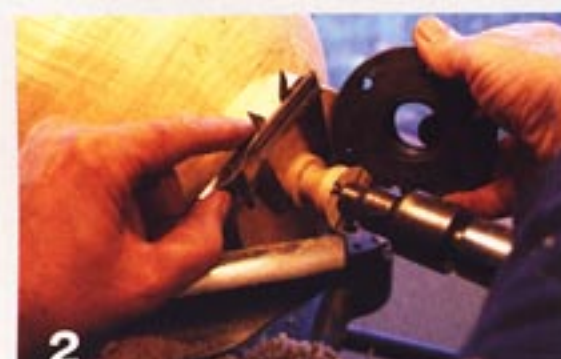
2 Add a few thousandths of an inch and turn and measure a short tenon on the bottom of your vessel.
