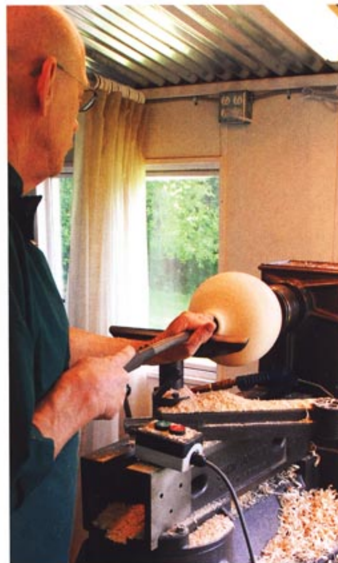
Body position is upright and relaxed, tool handle next to body.
