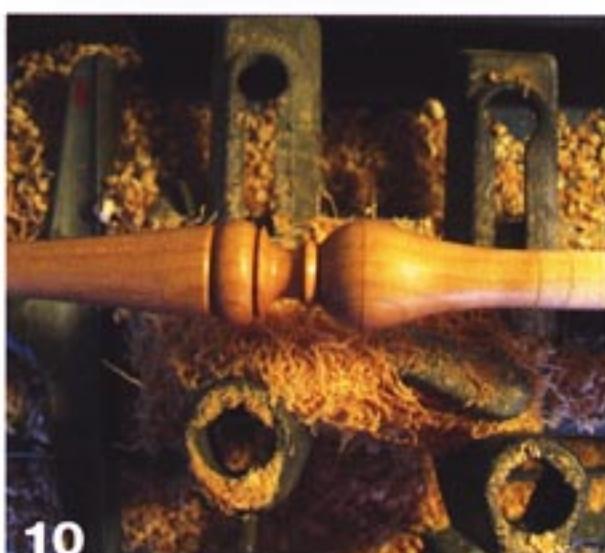
10 Except for the tenon, the leg is finished and oiled. Note that the tenon has been left cylindrical. After drying in the kiln, it will be turned to the correct taper.
