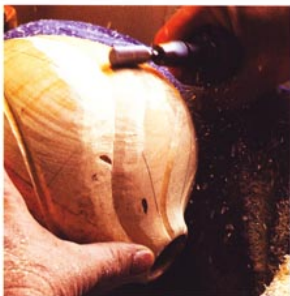
Rough shaping with pneumatic die grinder and carbide burr.
