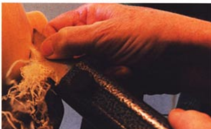
The newly turned area is finished with a shear scraper.
