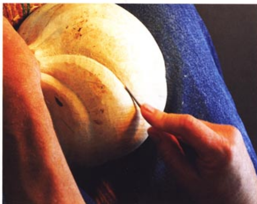
Defining the spiral lines with a small round rasp.
