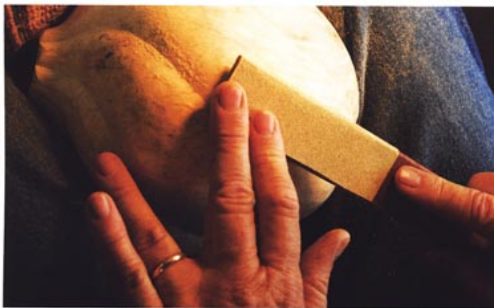
Sanding, using a flexible, leather-padded stick.
