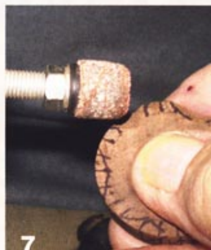
7 Notching the wheel using a small sanding drum. Follow the "Vs" inscribed on the side of the wheel.
