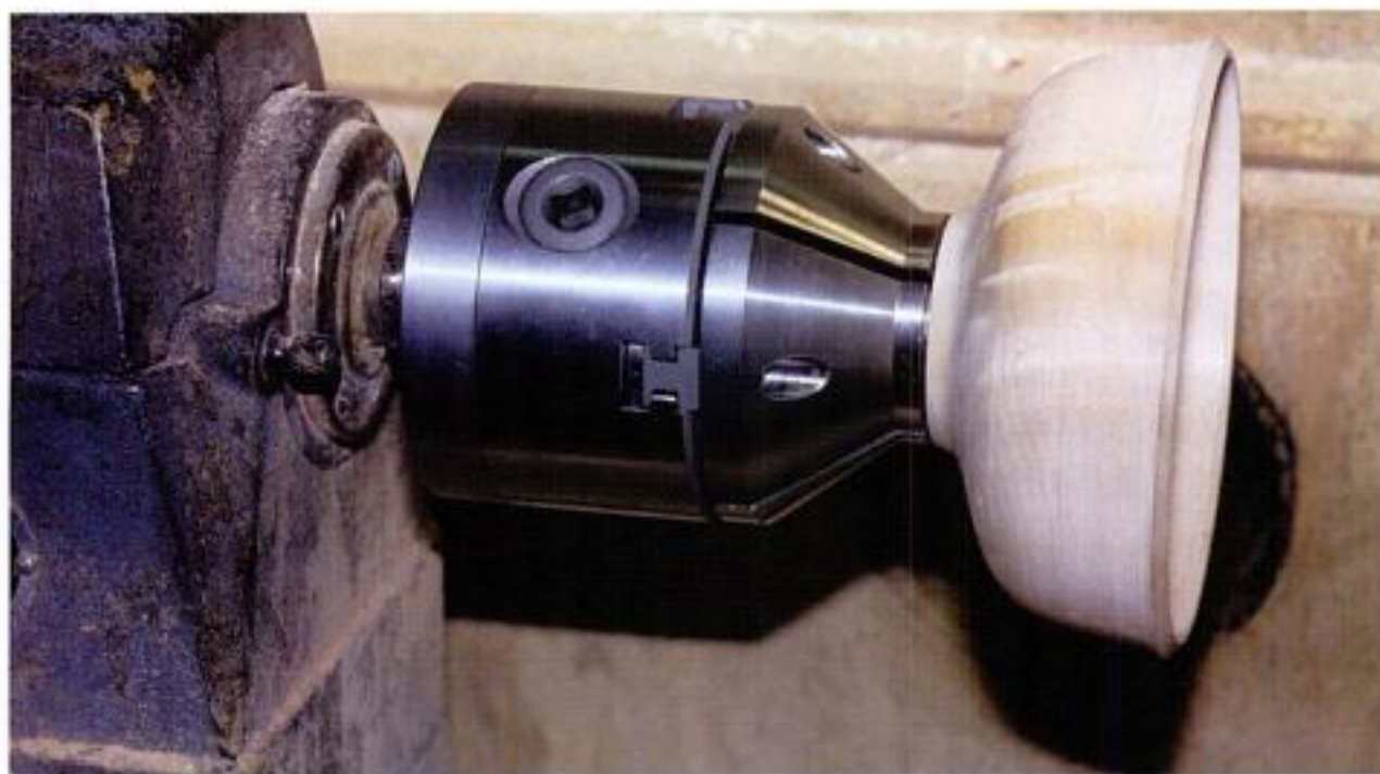
O'Donnell Jaws. The long jaws on this Axminster chuck accessory give you unrestricted access around the bottom of a bowl, but installing them is difficult.
