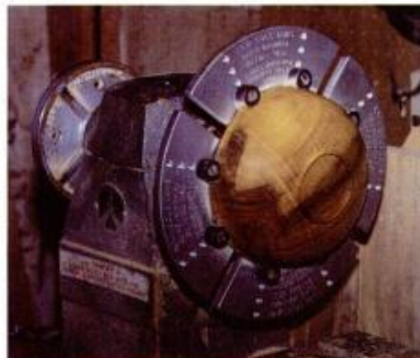
Around the rim. With oversize jaws like the Cole Jaws on this Nova chuck, you can grip a bowl by its rim in order to finish the base.
