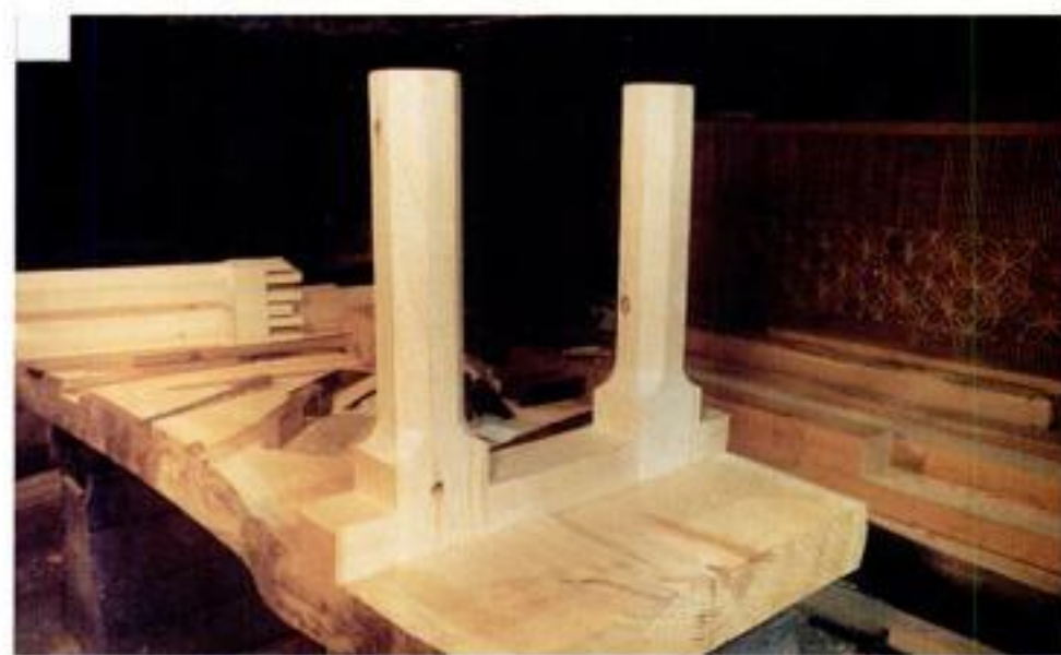
Final steps. After driving the dovetailed beams into place, Odate assembles the legs to the beams with rice glue. He wipes one coat of Watco oil on the completed table to even out the color and help protect the surface.
