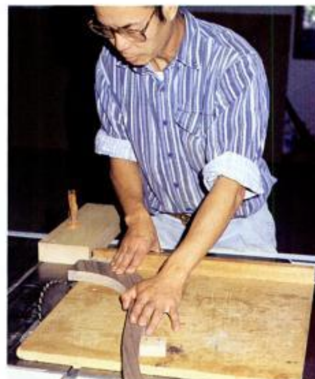
60° cut off. Alignment blocks enable Chan to make bevel cuts in the legs.
