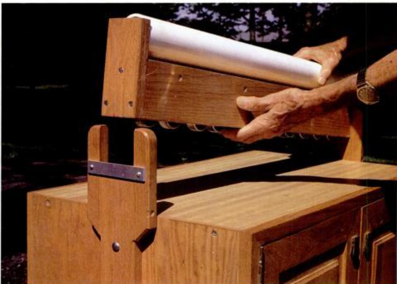
Quick change. Switching from wheels to outfeed roller is simply a matter of flipping the support over in its yokes.
