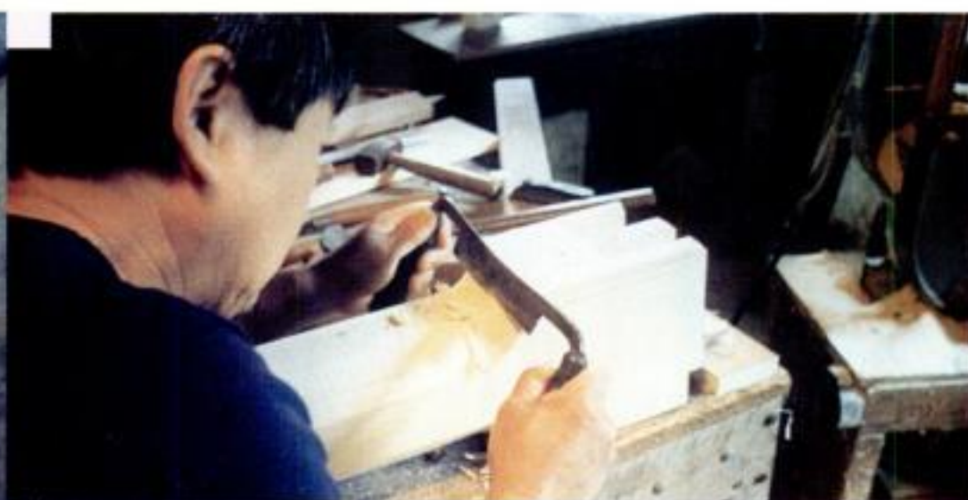
The joinery complete, Odate cuts the octagonal profiles on the legs. After bandsawing the legs square, he makes 45° saw cuts to his layout lines (left), then removes the waste on the beveled edges with a drawknife (above).
