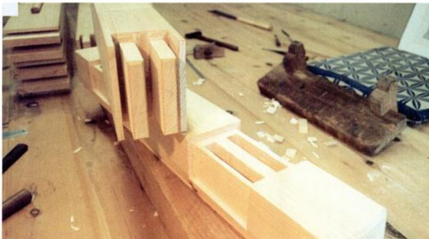
The finished joint has many shoulders to add strength. When assembled, none of the complicated joinery is visible from the outside.
