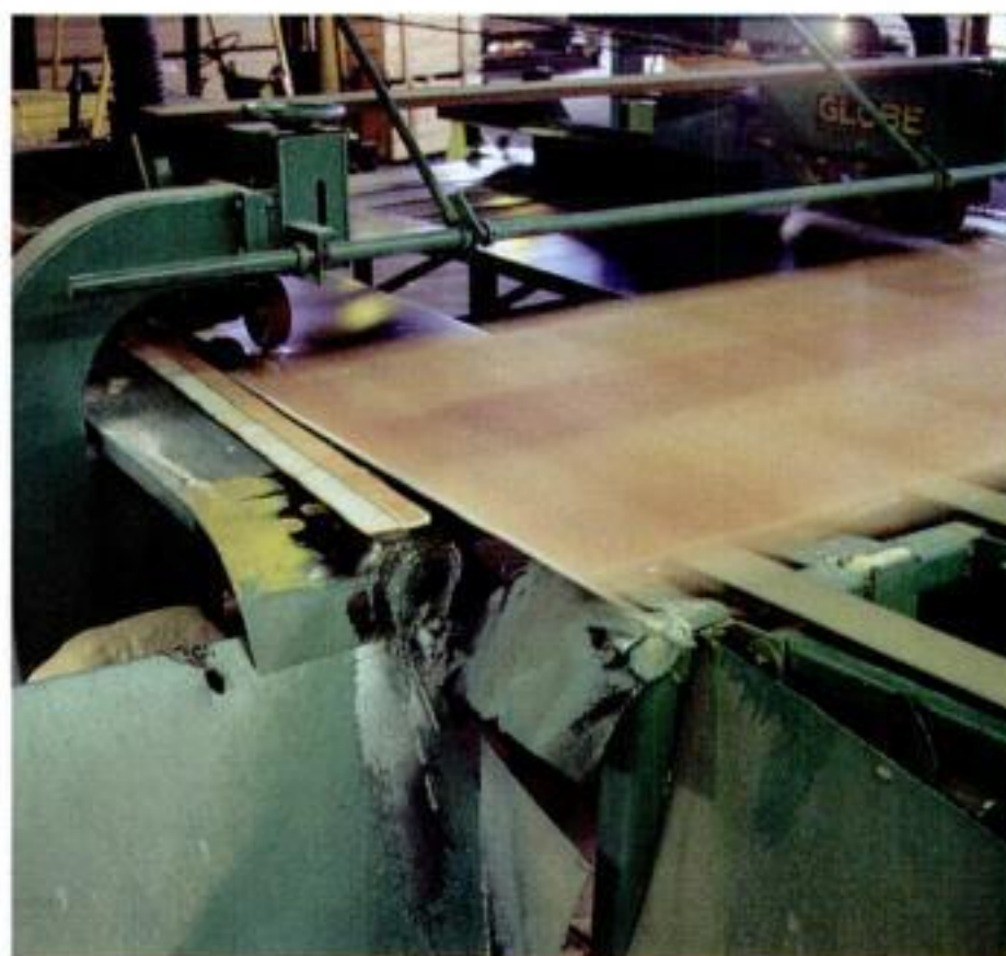
Quick saw. Two saw blades trim the ends of panels square to the sides.
