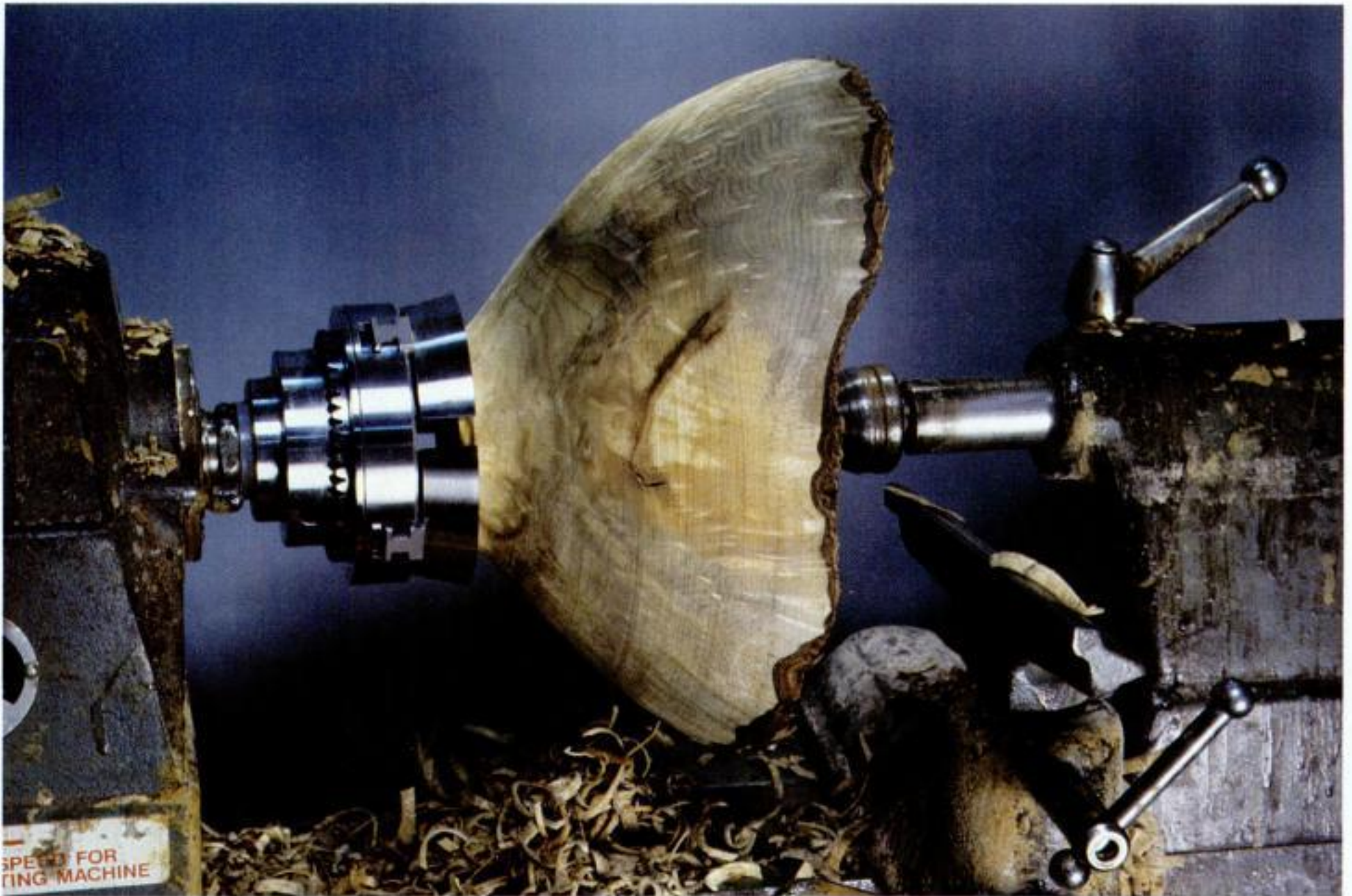
A good turn. A scroll-type chuck is great for gripping bowls and hollow vessels for turning on the lathe.
