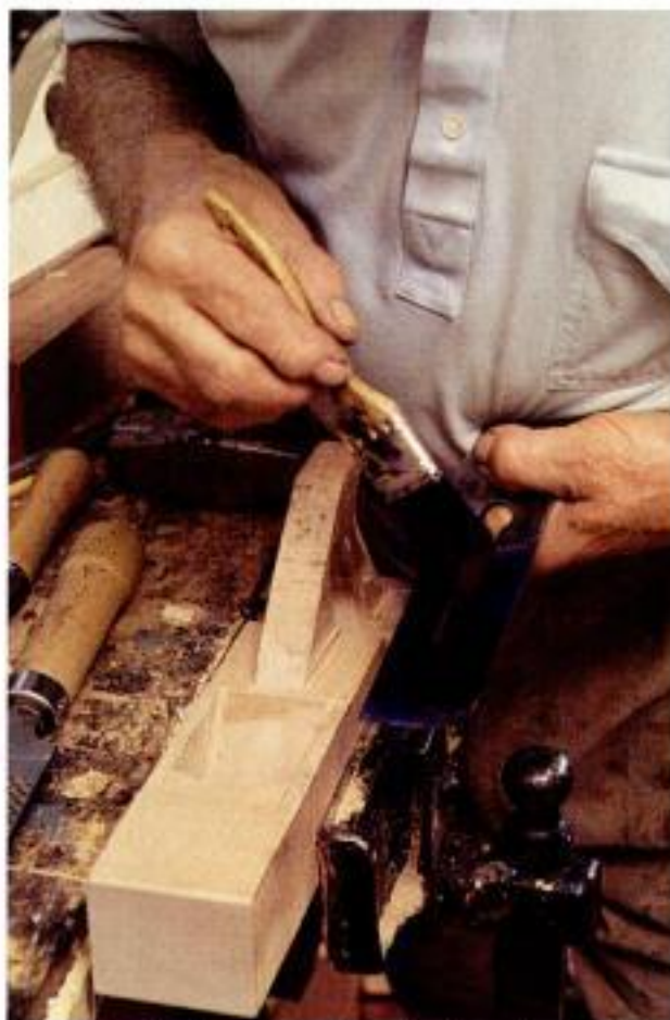
Getting it flat. To check the throat's blade-bearing ramp for flat, Pierce coats a plane blade with machinist's fluid and rubs it on the ramp. High spots show up as blue marks and are removed with chisels or scrapers.
