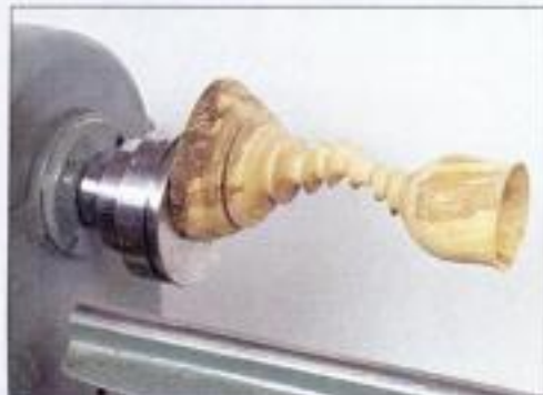
How did he do that? Sorby's new Eccentri-Chuck turns tricky creations by offsetting the turning axis from the lathe's axis.
