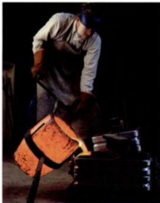
Molten manganese-bronze. In the Lie-Nielsen foundry, the molten alloy, known for its strength and beauty,
