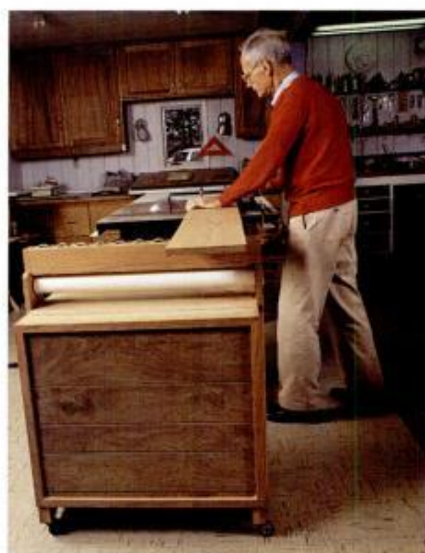
Infeed mode. Skate wheels support long boards for crosscutting.
