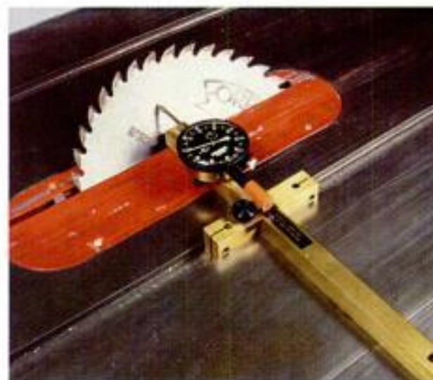
The Infinitii AAG-100 measures distance at 1 in. above the table. The removable brass fence fits in the miter slot.
