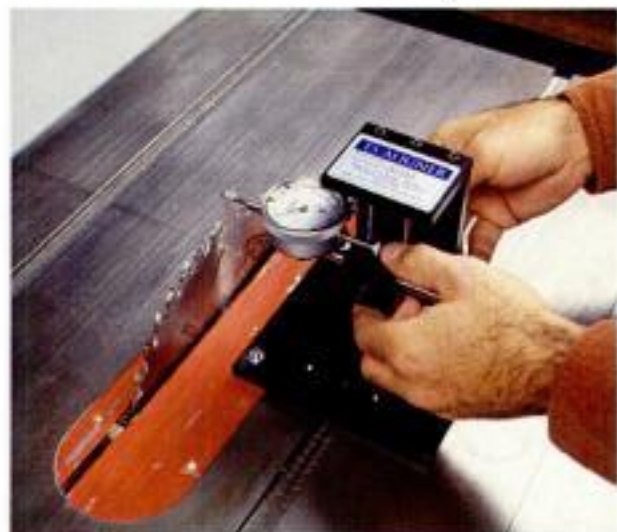
The TS-Aligner can measure vertically and horizontally. Offset tip allows measurements close to the table.
