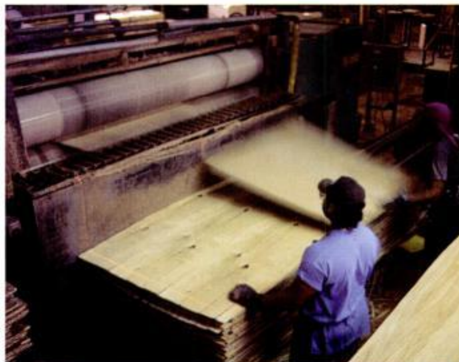
Rolling the glue. Workers catch glue-covered plies and arrange them in alternating grain directions to make a stack of plywood sheets.
