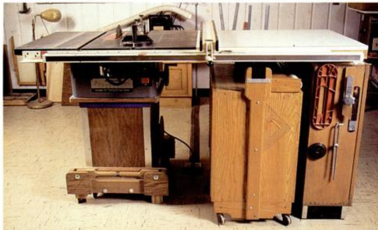
Storage mode. When not in use, the mobile cart and its roller support stow underneath the table saw's extension table.
