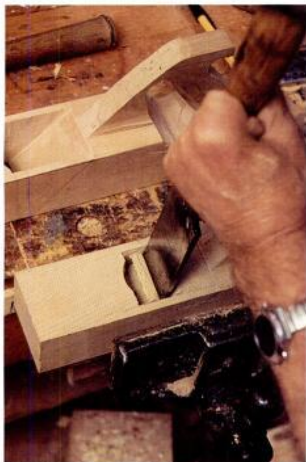
Clearing the throat. Major waste removal in the throat is done with a 2-in. firmer chisel and a gouge. An integral handle, shown roughed out on the plane in the background, is a standard feature on all Pierce planes.
