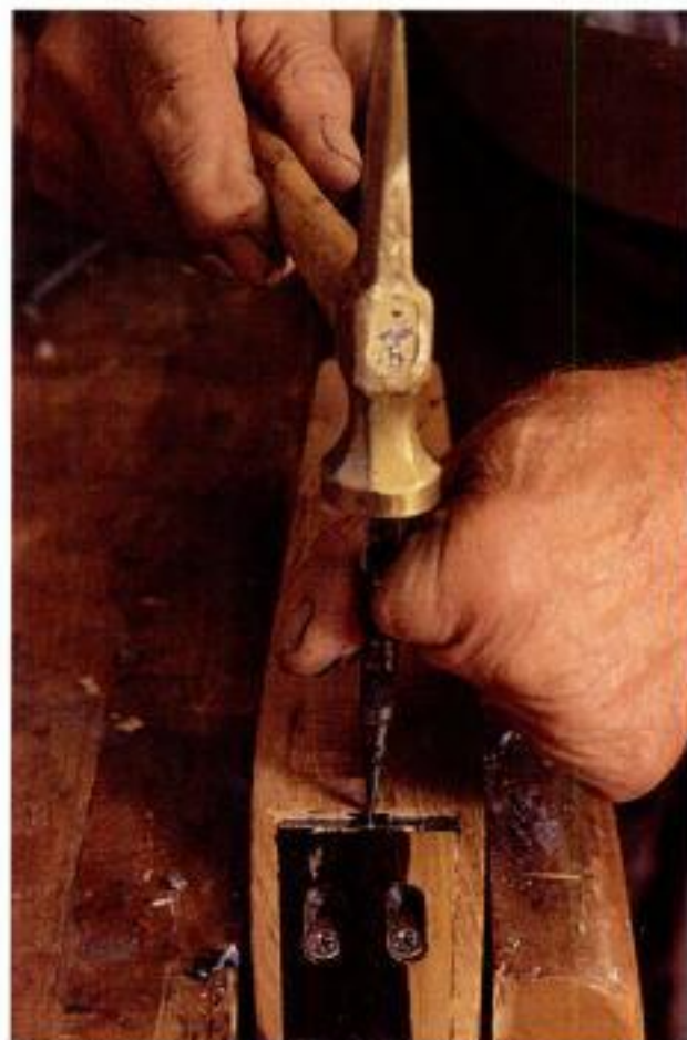
Making adjustments. A small pocket, ground into the plane iron just below its bevel, provides a recess for the nailset as Pierce fine-tunes cutting depth with a few light taps. Note the adjustable throat plate.
