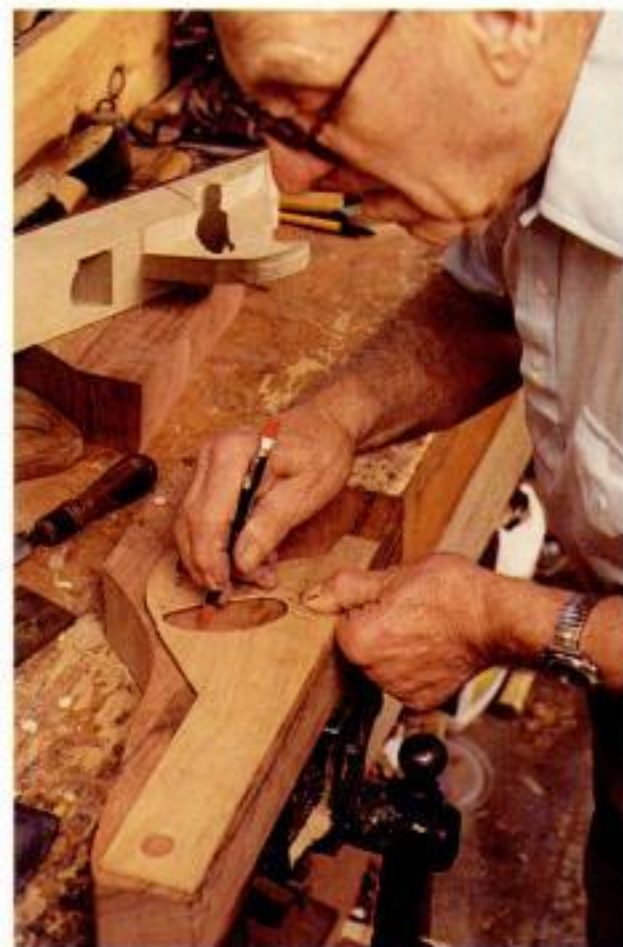
▲ Tracing the pattern. Using a simple template, Pierce marks up a blank that will be shaped into a wooden plane.
